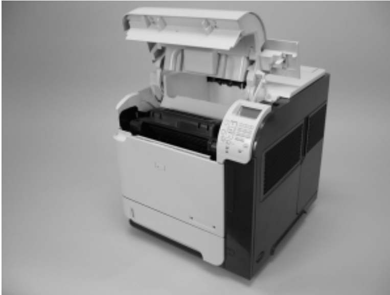
Figure 2-2 Remove the print cartridge (1 of 2)
