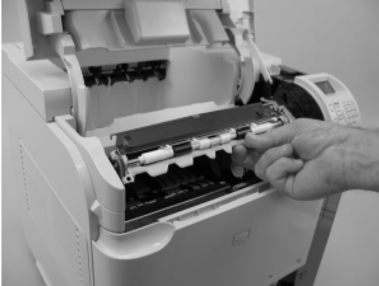
Figure 2-62 Remove the registration assembly (3 of 4)
