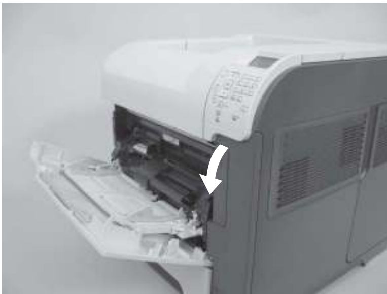
Figure 2-36 Remove the front accessory covers (2 of 2)
