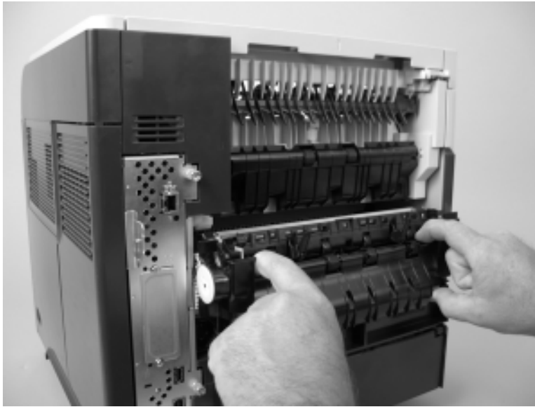
Figure 2-11 Remove the fuser (2 of 2)
