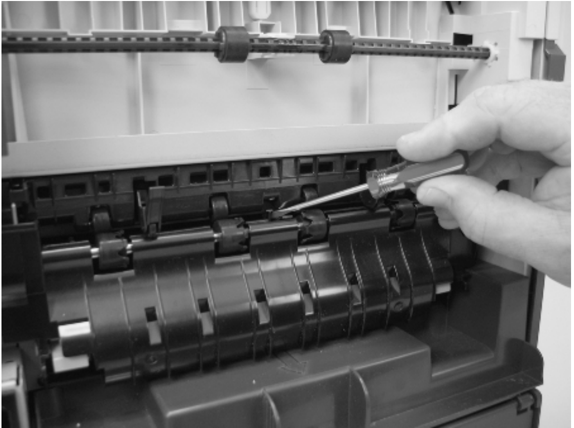
Figure 3-6 Test the fuser delivery sensor (PS700)
