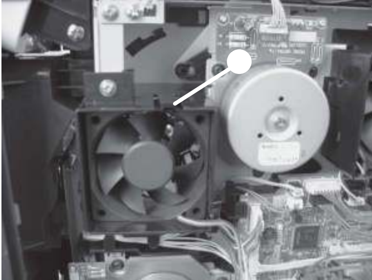
Figure 2-78 Remove fan FN103 (2 of 2)
