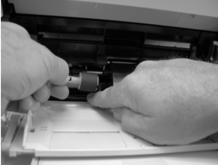
Figure 2-31 Remove the Tray 1 separation roller (3 of 3)
