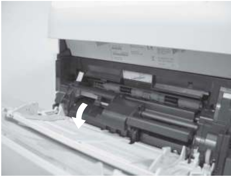
Figure 2-29 Remove the Tray 1 separation roller (1 of 3)
