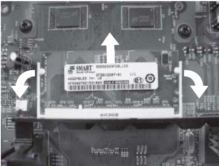
Figure 2-22 Remove the memory DIMM
