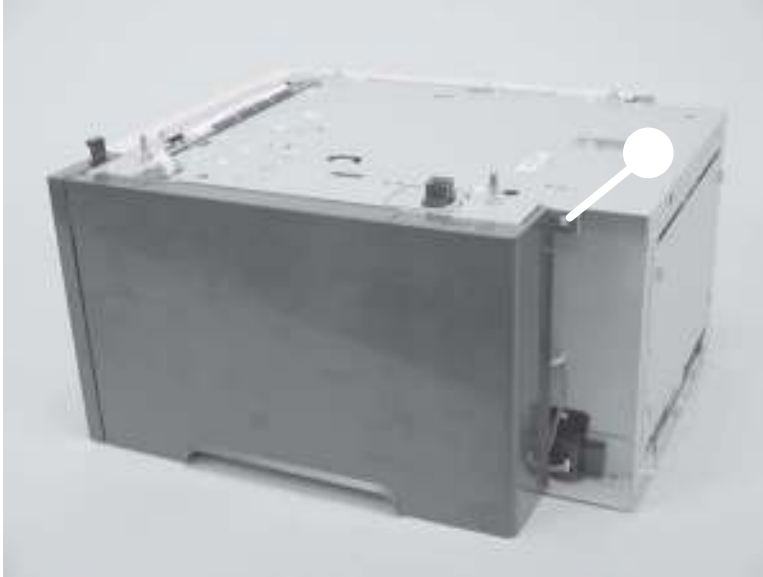
Figure 2-141 Remove the right-side cover (PD; 1 of 2)
