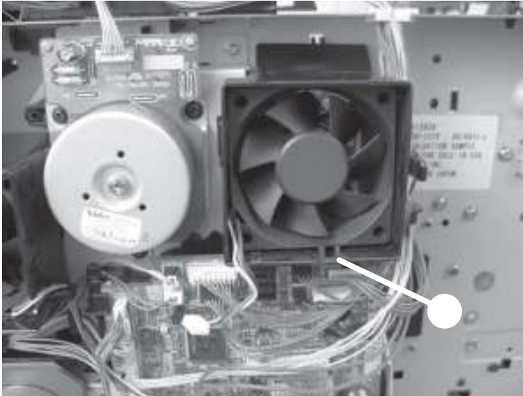
Figure 2-76 Remove fan FN102 (2 of 2)
