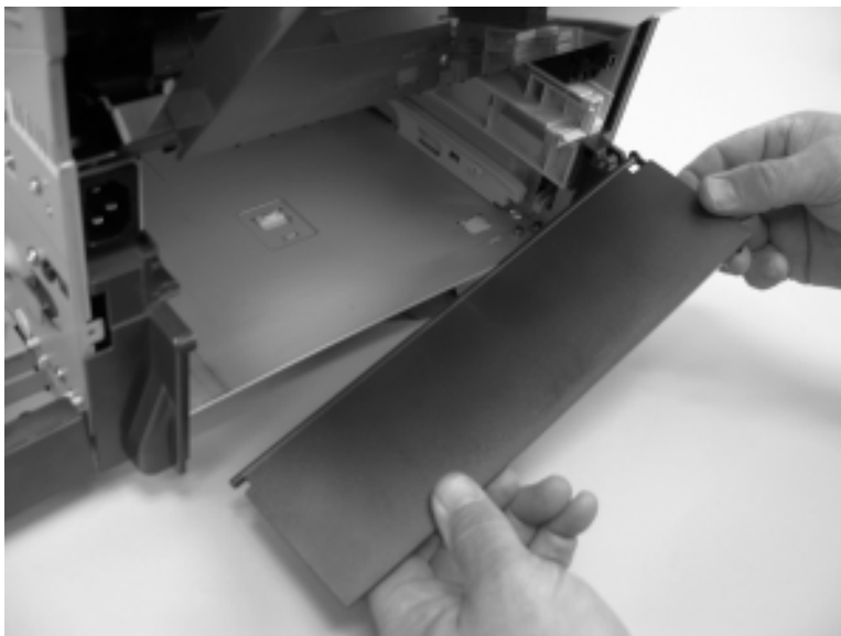
Figure 2-40 Remove the Tray 2 extension door (2 of 2)
