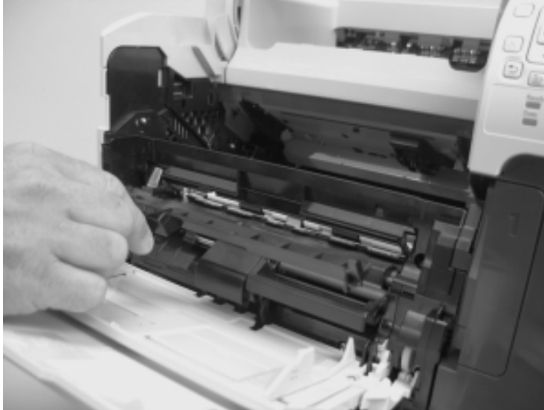
Figure 2-35 Remove the front accessory covers (1 of 2)
