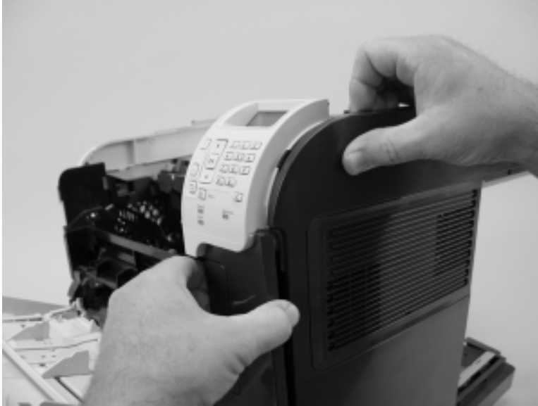
Figure 2-46 Remove the right-side cover (2 of 3)
