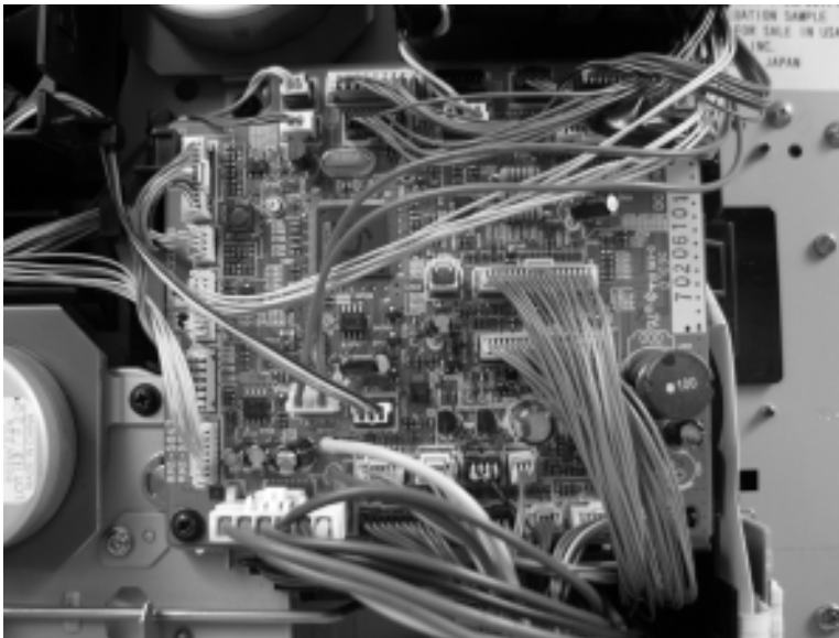
Figure 2-87 Remove the DC controller PCA (1 of 4)
