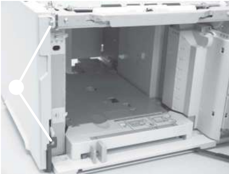
Figure 2-145 Remove the left-side cover (PD; 3 of 5)
