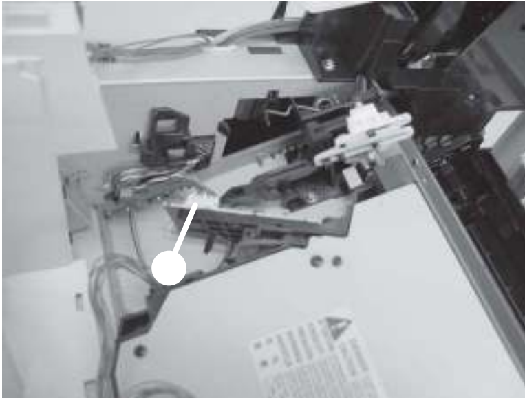
Figure 2-131 Remove the laser/scanner assembly (4 of 4)
