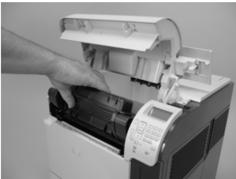
Figure 2-3 Remove the print cartridge (2 of 2)
