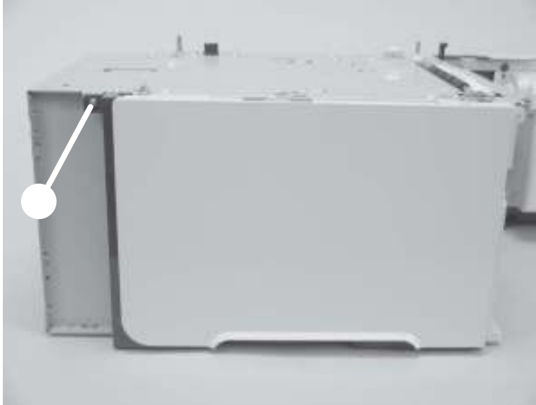
Figure 2-146 Remove the left-side cover (PD; 4 of 5)
