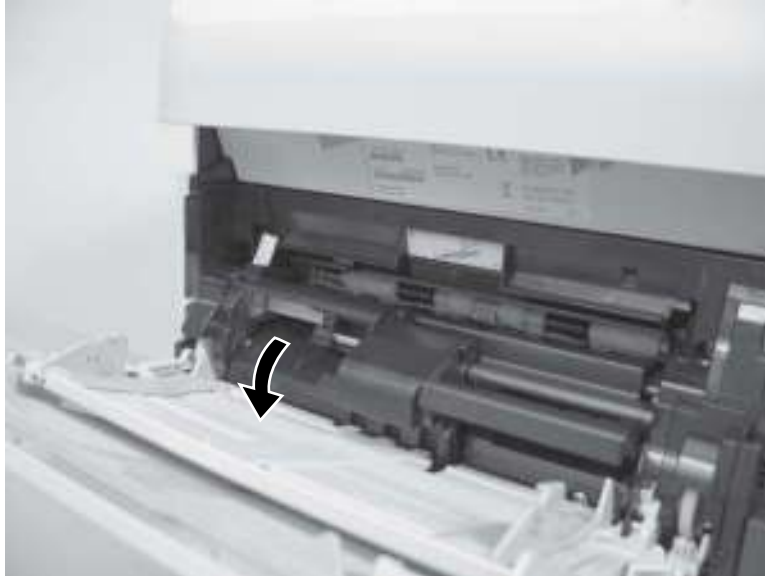
Figure 2-118 Open the separation roller cover
