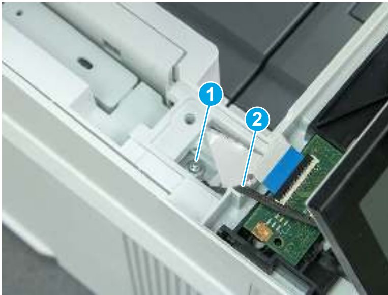
Figure 5-228 Remove one screw
