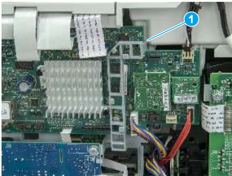
Figure 5-627 Release one tab
