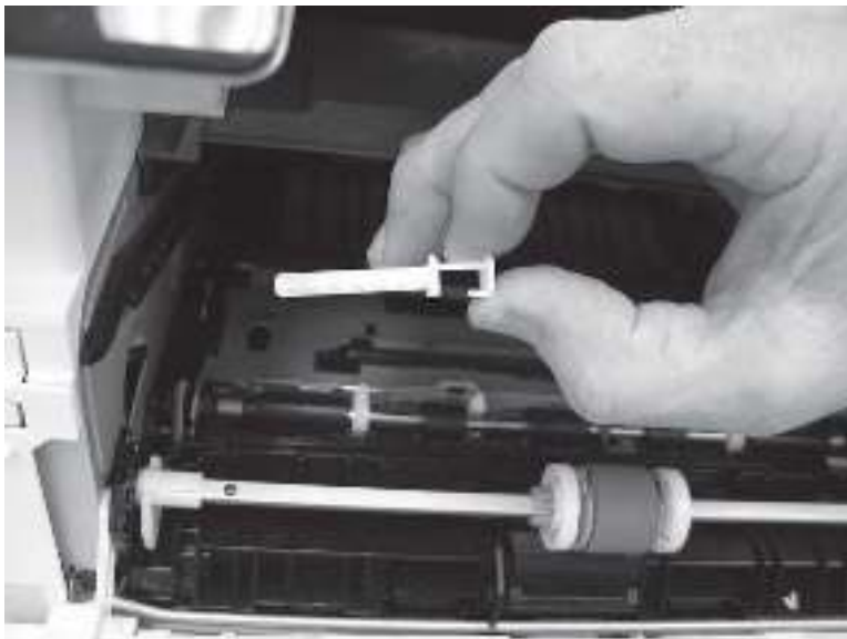
Figure 5-341 Remove the support shaft
