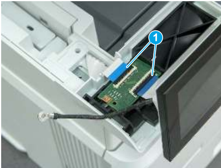
Figure 5-191 Disconnect two FFC
