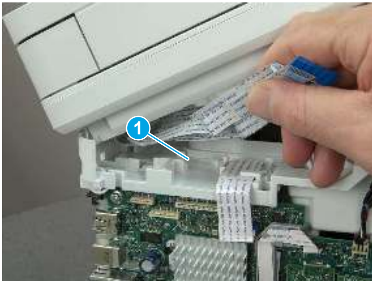
Figure 5-666 Release the tape
