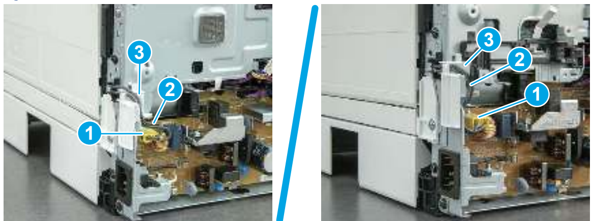
Figure 5-861 SFP/MFP: Remove the wire harness
