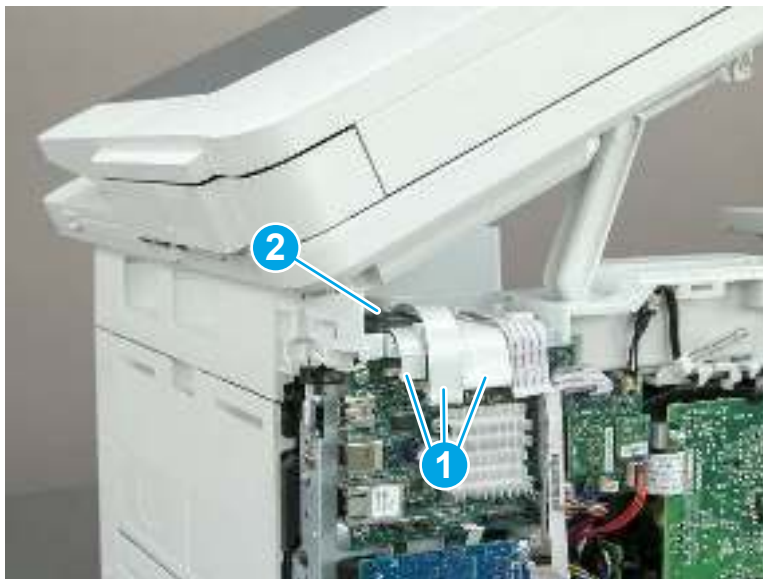
Figure 5-76 Disconnect three FFCs
