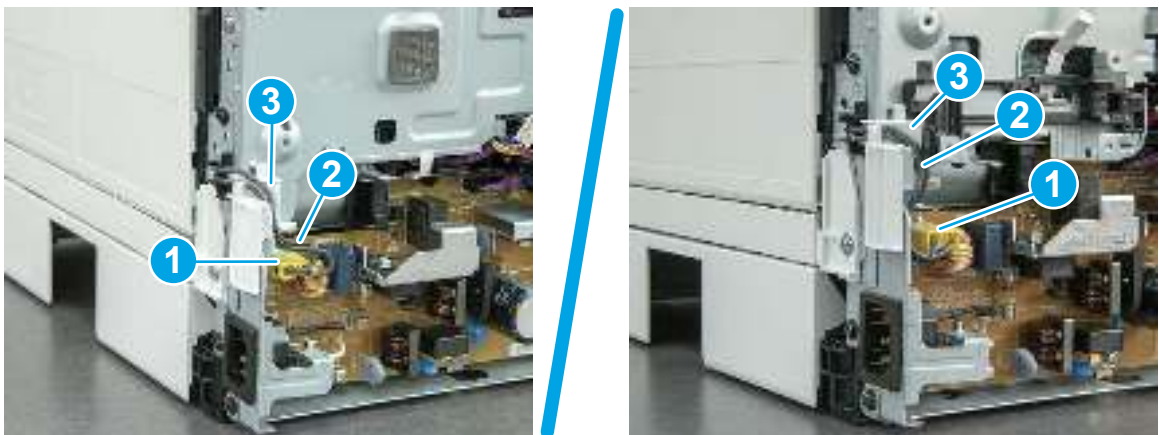
Figure 5-633 SFP/MFP: Remove the wire harness
