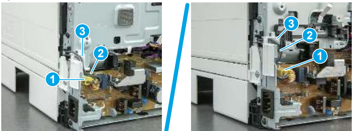
Figure 5-687 SFP/MFP: Remove the wire harness
