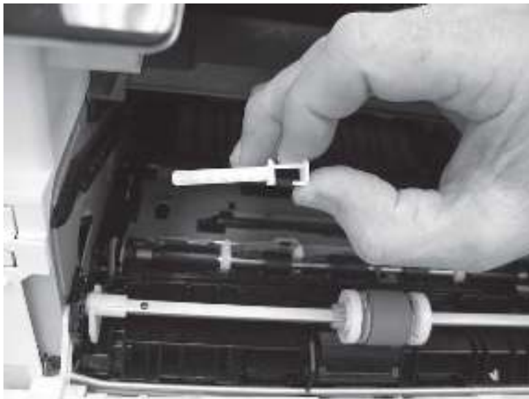
Figure 5-451 Remove the support shaft
