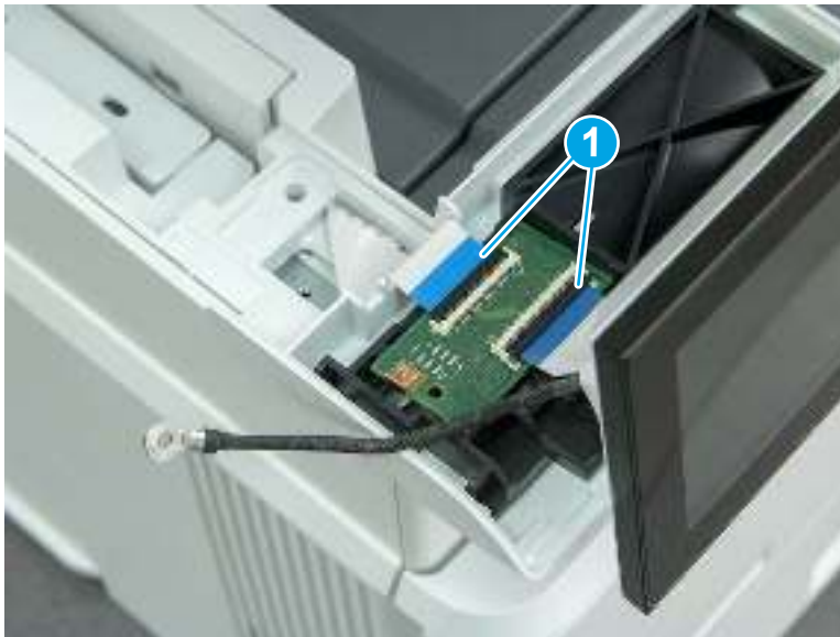
Figure 5-888 Disconnect two FFC
