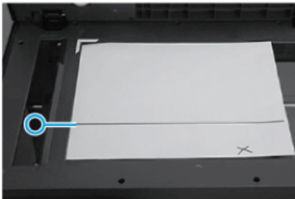
Figure 4-92 Place the copy on the flatbed
