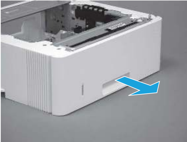
Figure 5-33 Pull the tray out of the printer
