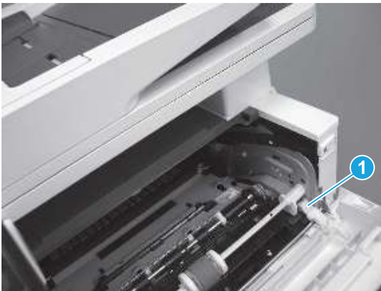
Figure 5-466 Release the pressure-release link
