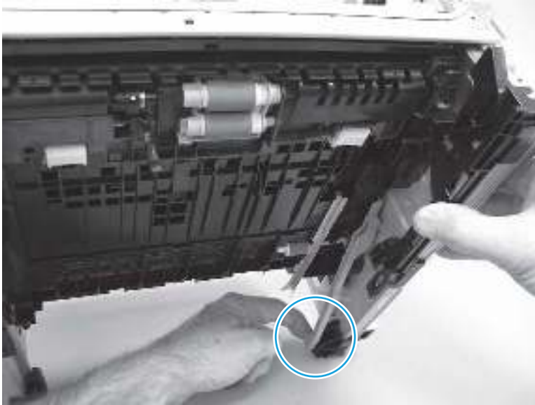
Figure 5-391 Move the link arm out of the way
