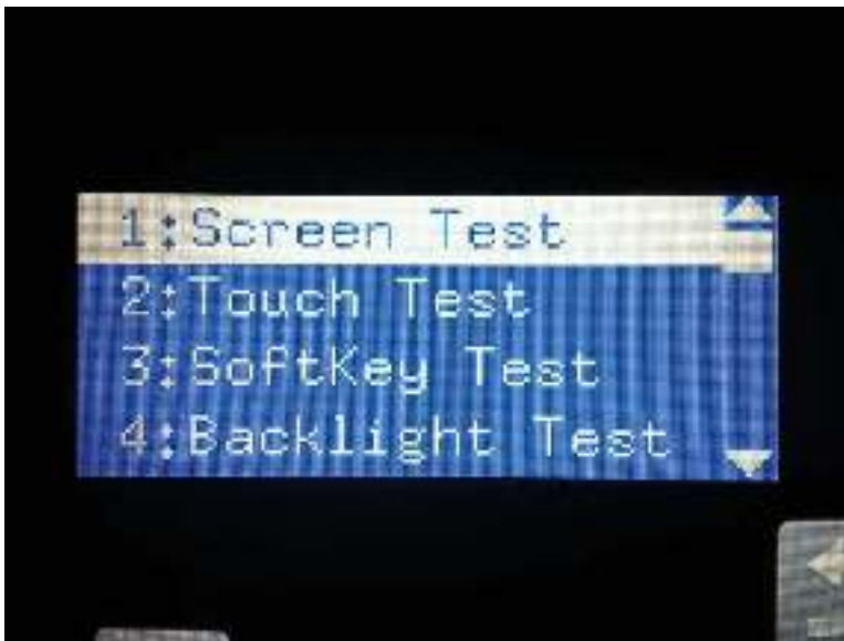
Figure 4-49 Open the screen test
