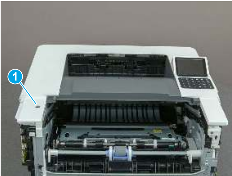
Figure 5-943 Remove one screw
