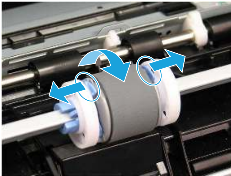
Figure 4-62 Release the roller
