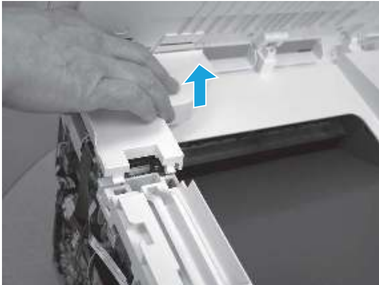
Figure 5-61 Remove the scanner cable cover
