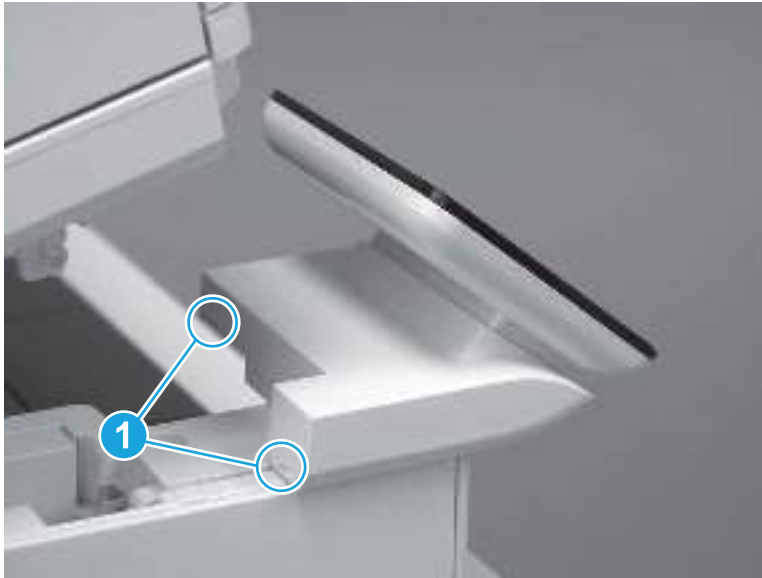
Figure 5-226 Release two tabs
