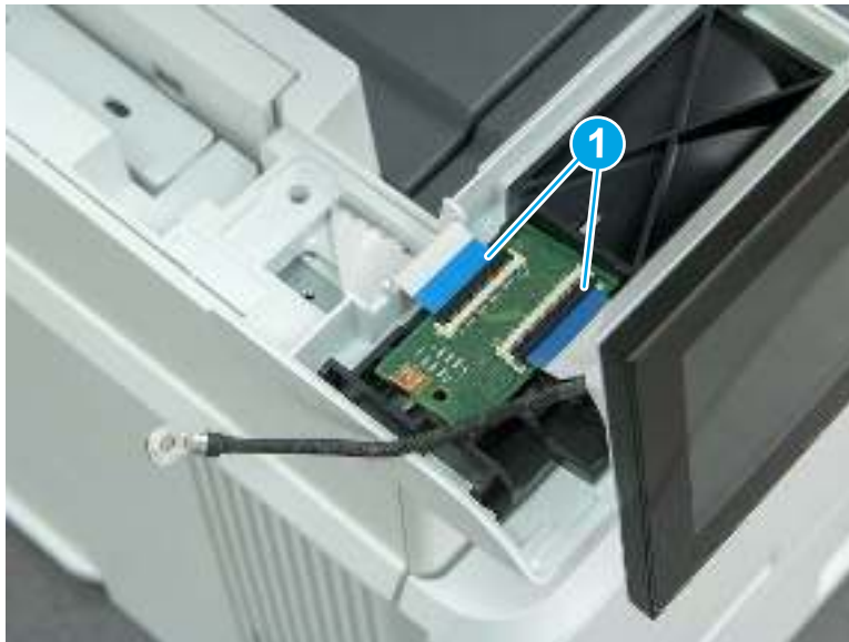
Figure 5-359 Disconnect two FFC
