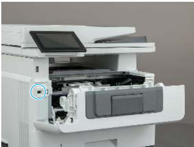
Figure 4-43 Defeat the front (cartridge) door interlock
