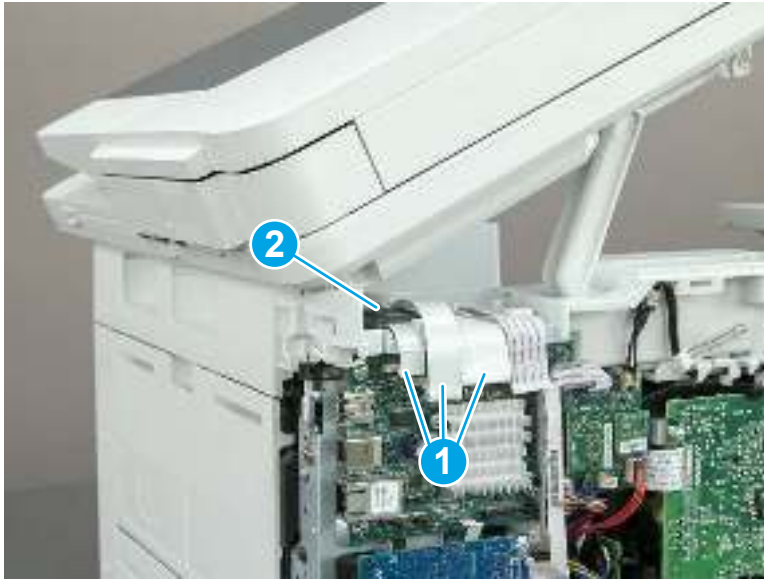
Figure 5-364 Disconnect three FFCs
