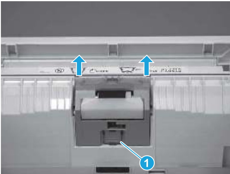
Figure 5-28 Release the assembly
