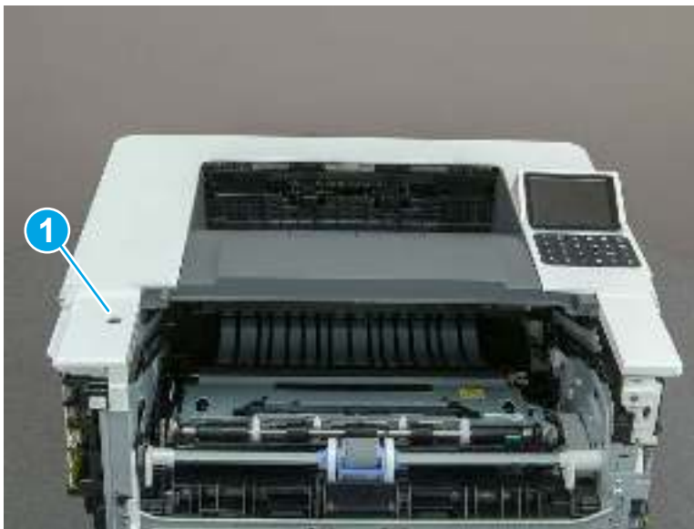
Figure 5-270 Remove one screw
