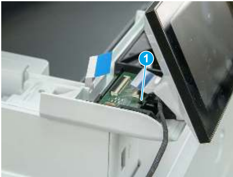
Figure 5-604 Remove the ICB
