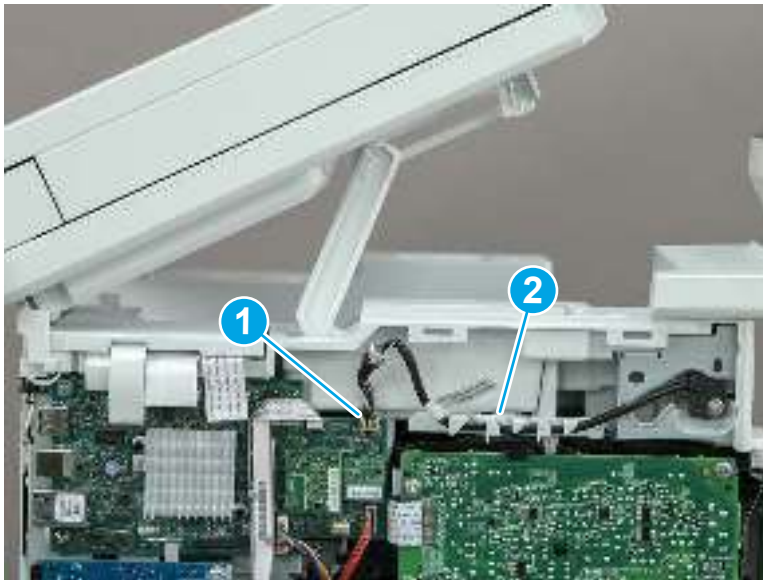
Figure 5-460 Disconnect one connector
