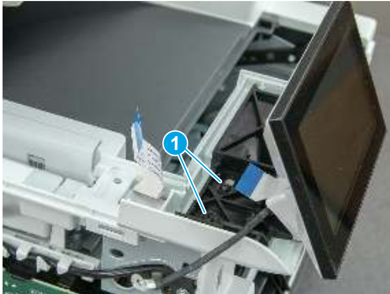
Figure 5-231 Remove two screws and remove the control panel assembly
