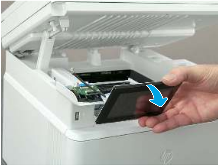
Figure 5-974 Remove the control-panel assembly
