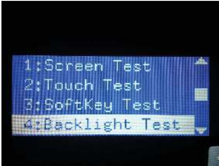
Figure 4-57 Open the backlight test
