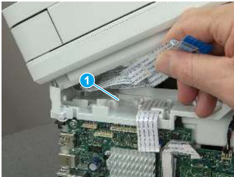
Figure 5-894 Release the tape
