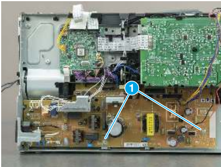
Figure 5-928 Remove two screws
