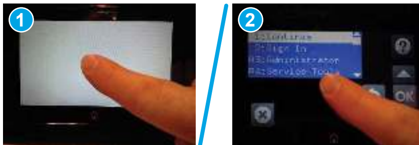
Figure 4-41 Open the Pre-boot menu (MFP)
