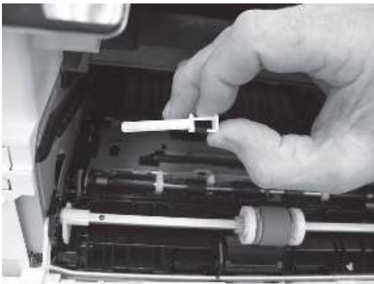
Figure 5-423 Remove the support shaft
