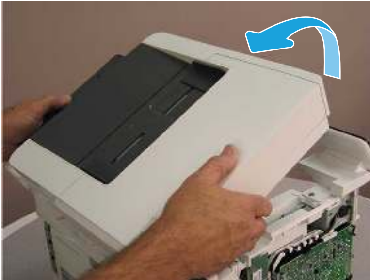
Figure 5-221 Rotate the ISA towards the rear of the printer
