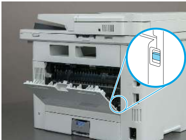
Figure 4-44 Defeat the rear door interlock
