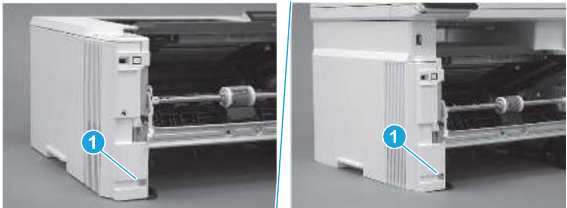
Figure 5-593 Remove one screw
