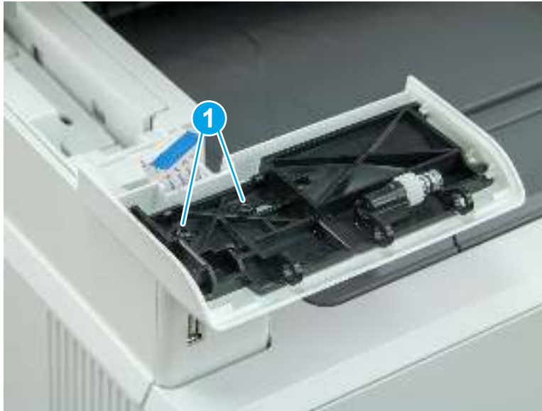
Figure 5-976 Remove two screws
