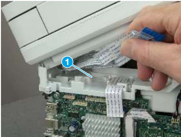
Figure 5-216 Release the tape
