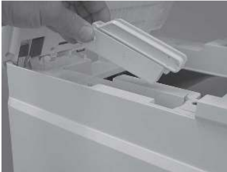
Figure 5-62 Remove the support arm
