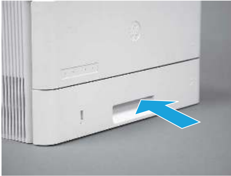
Figure 5-32 Install the tray
