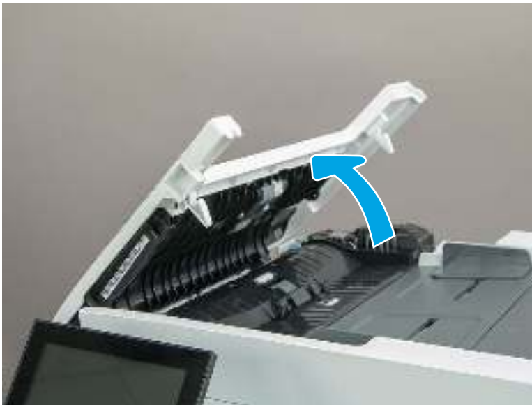
Figure 5-52 Open the document feeder top cover
