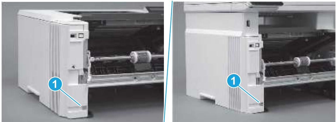
Figure 5-516 Remove one screw
