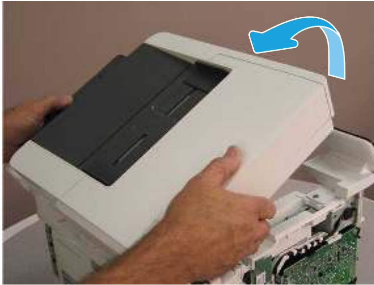
Figure 5-370 Rotate the ISA towards the rear of the printer
