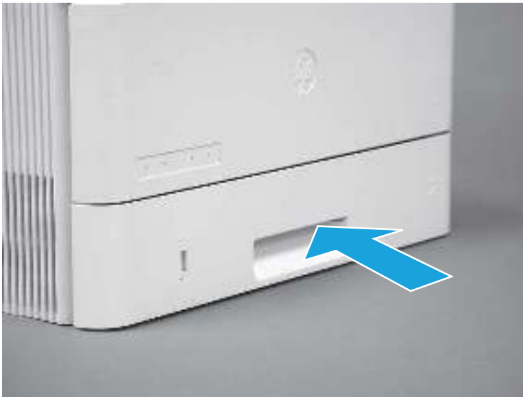
Figure 2-18 Install the tray
