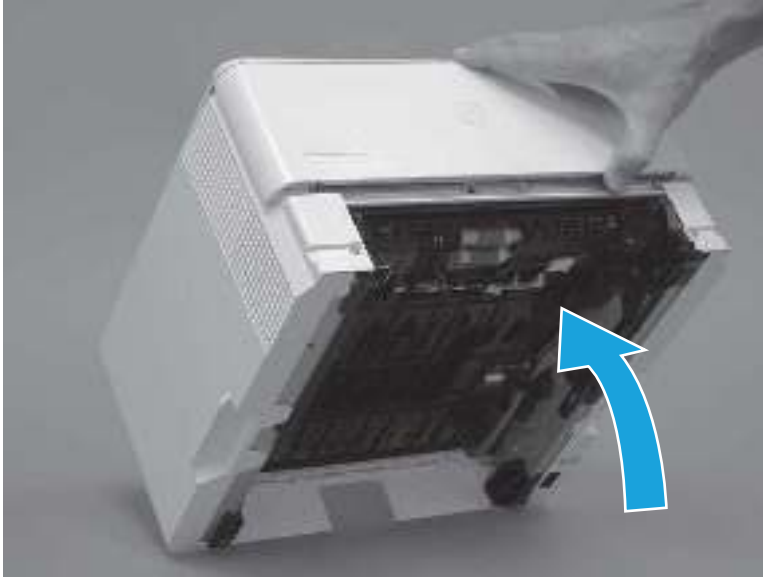
Figure 5-18 Tilt the printer backward
