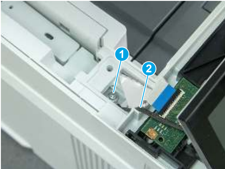
Figure 5-830 Remove one screw
