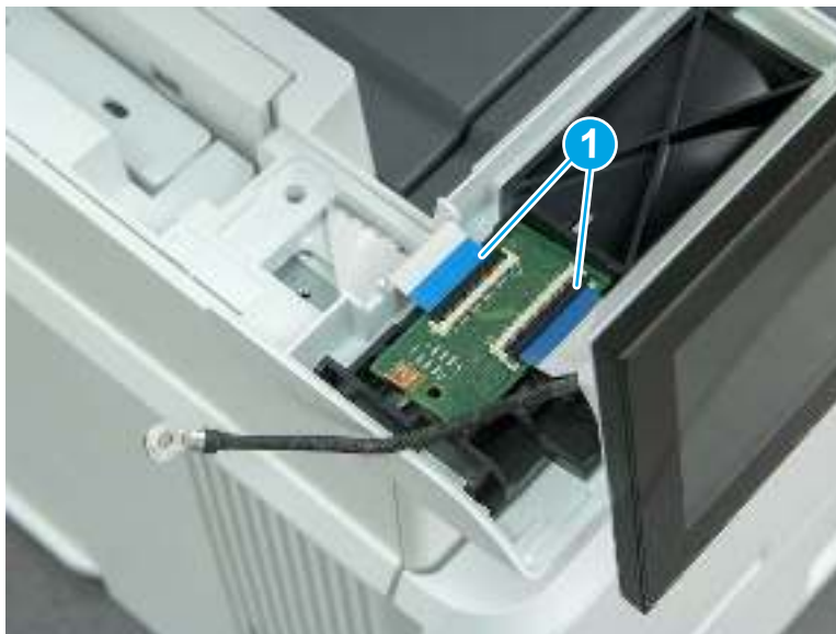
Figure 5-603 Disconnect two FFC
