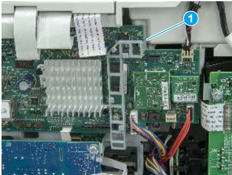
Figure 5-501 Release one tab
