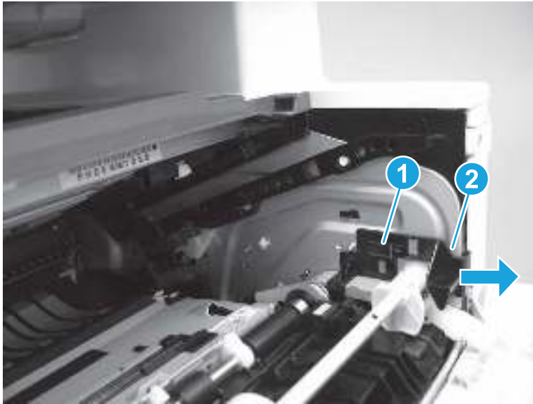
Figure 5-452 Remove the guide
