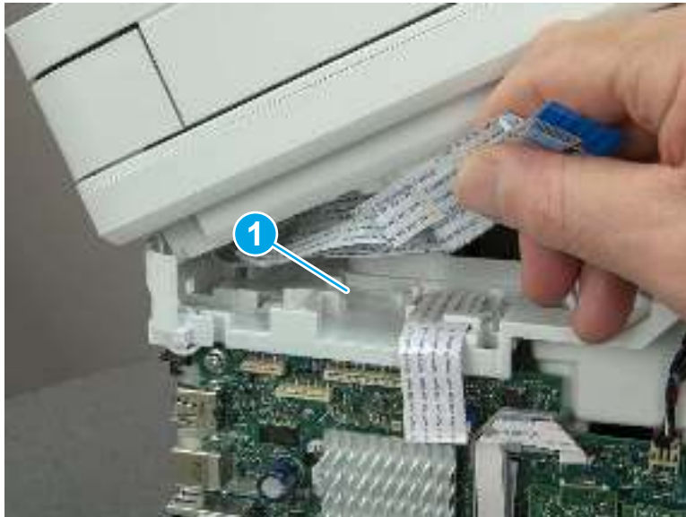
Figure 5-178 Release the tape
