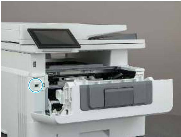
Figure 4-22 Defeat the front (cartridge) door interlock
