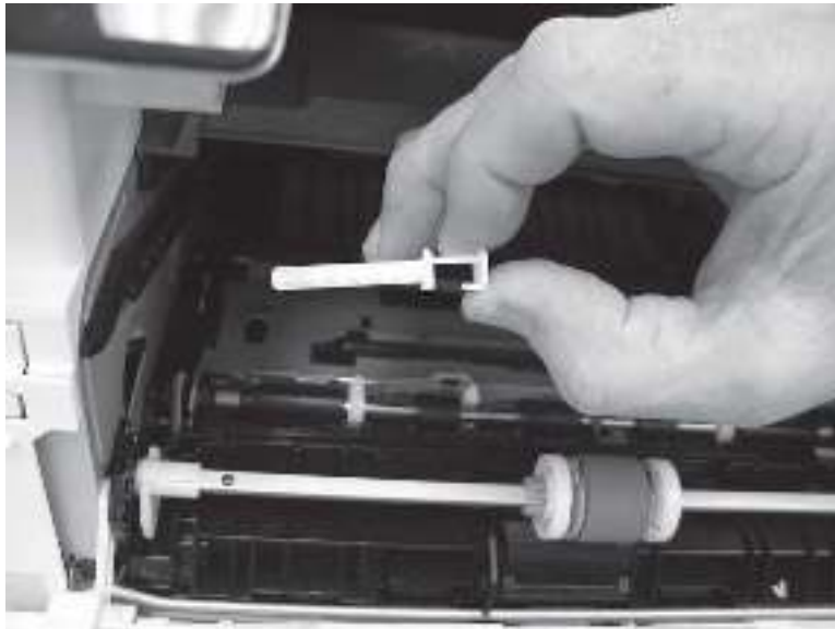
Figure 5-96 Remove the support shaft
