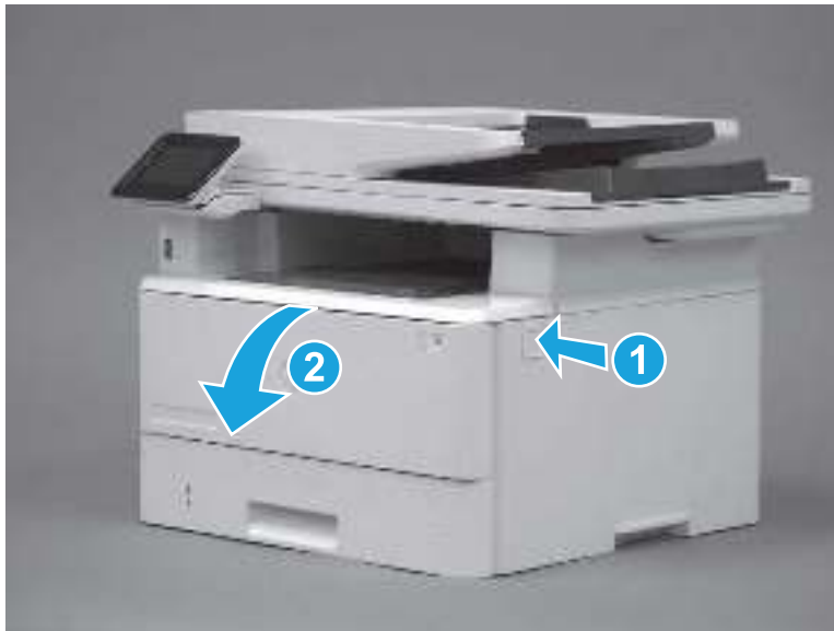
Figure 2-1 Open the toner-cartridge door
