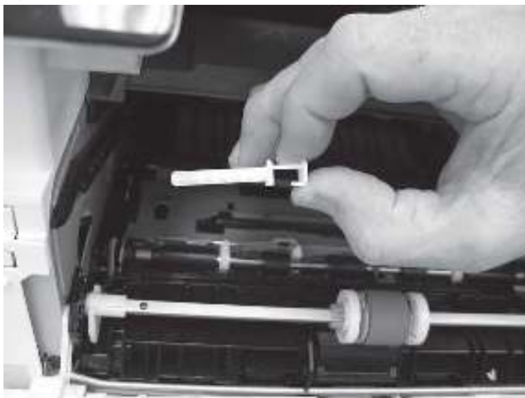
Figure 5-587 Remove the support shaft
