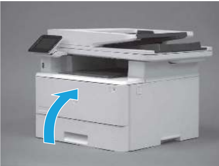
Figure 2-7 Close the toner-cartridge door
