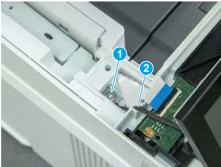
Figure 5-190 Remove one screw
