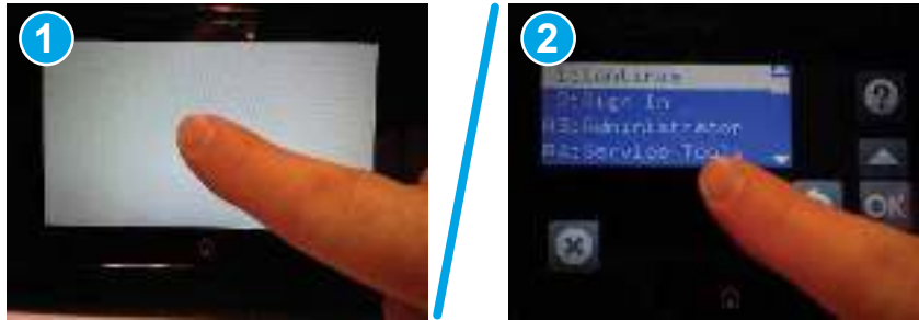
Figure 4-40 Open the Pre-boot menu (MFP)
