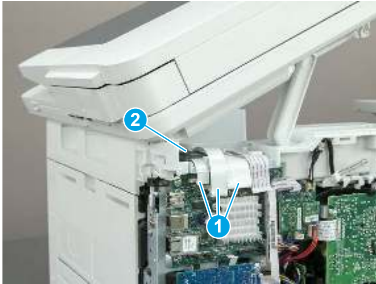
Figure 5-721 Disconnect three FFCs
