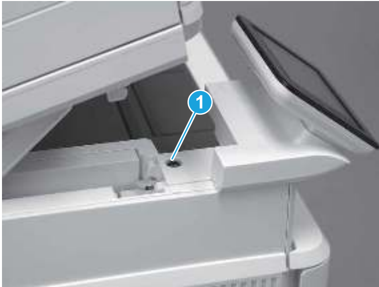
Figure 5-709 Remove one screw
