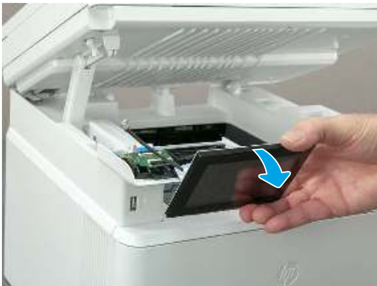
Figure 5-957 Remove the control-panel assembly
