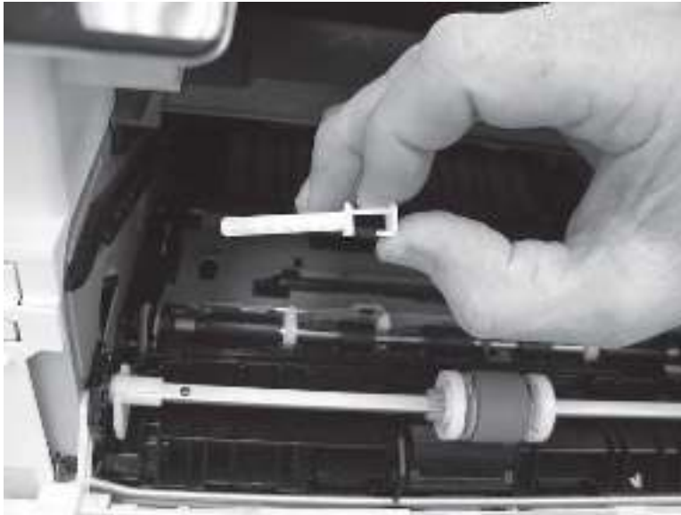
Figure 5-117 Remove the support shaft
