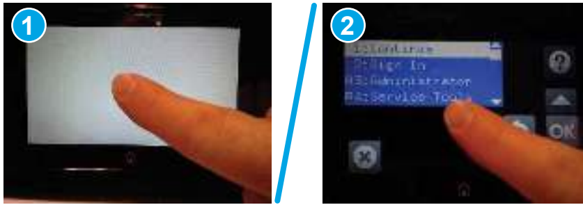
Figure 4-42 Open the Pre-boot menu (MFP)
