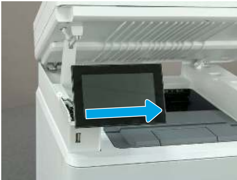
Figure 5-956 Slide the control panel display
