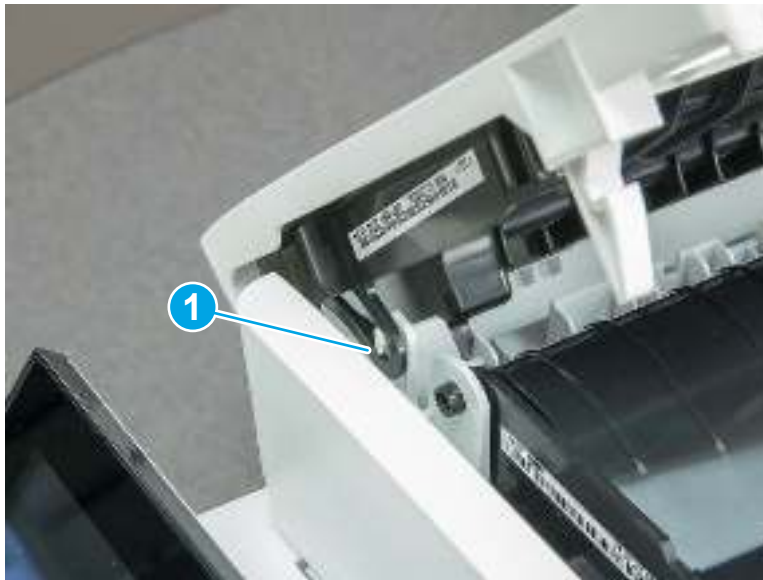
Figure 5-53 Release one hinge pin
