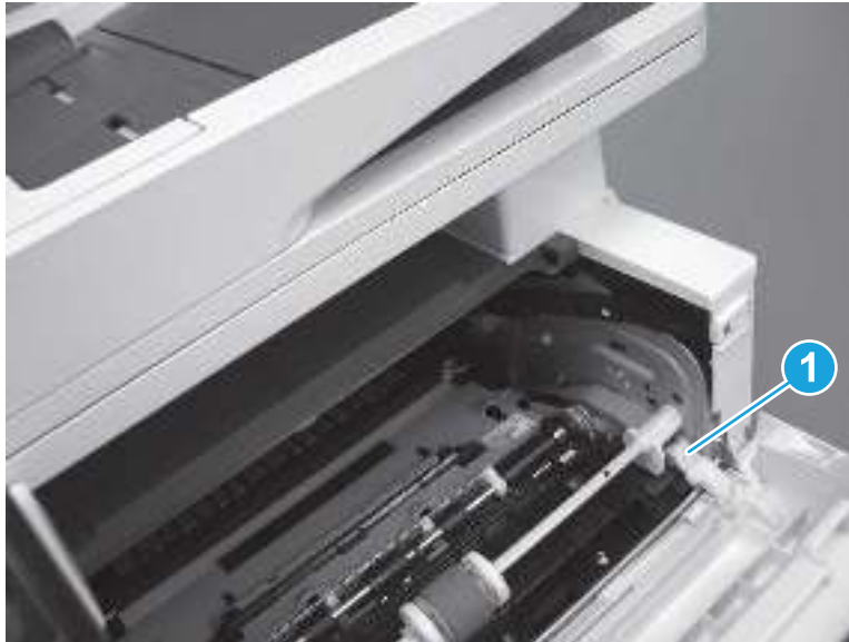
Figure 5-322 Release the pressure-release link
