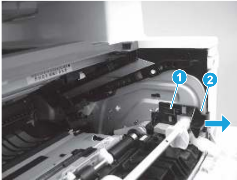
Figure 5-90 Remove the guide
