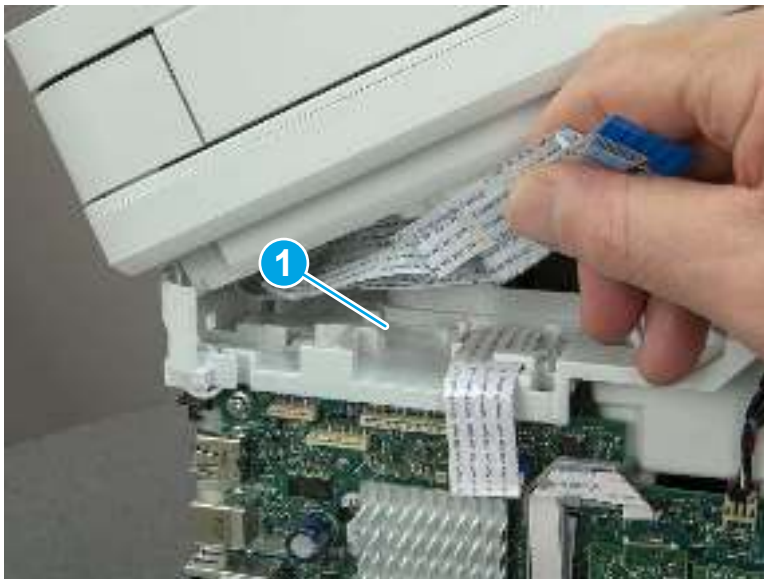
Figure 5-365 Release the tape
