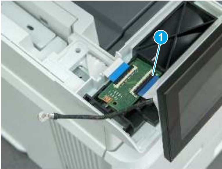
Figure 5-972 Disconnect one flat cable
