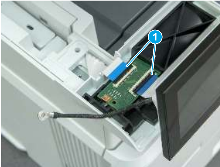
Figure 5-713 Disconnect two FFC
