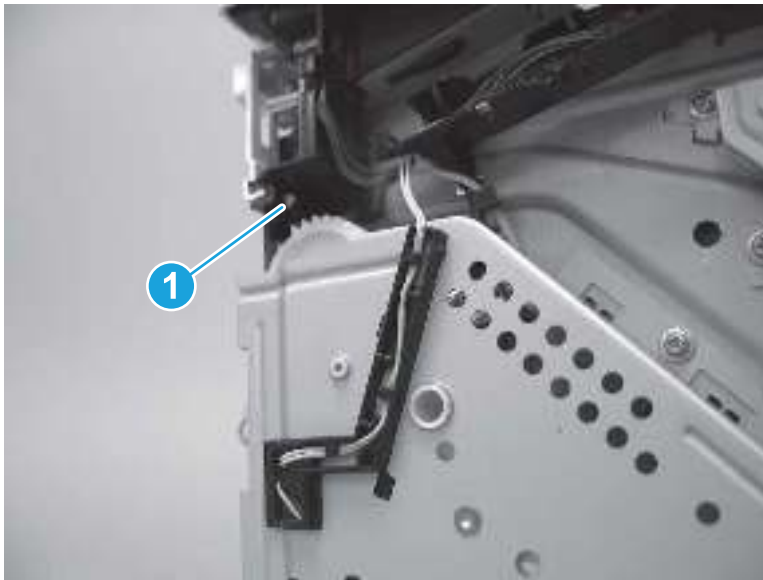
Figure 5-417 Release one tab
