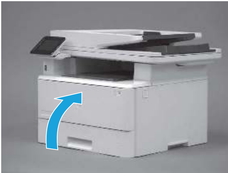
Figure 5-16 Close the toner-cartridge door
