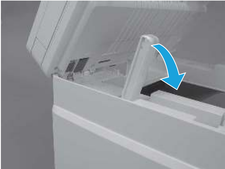
Figure 5-57 Lower the support arm
