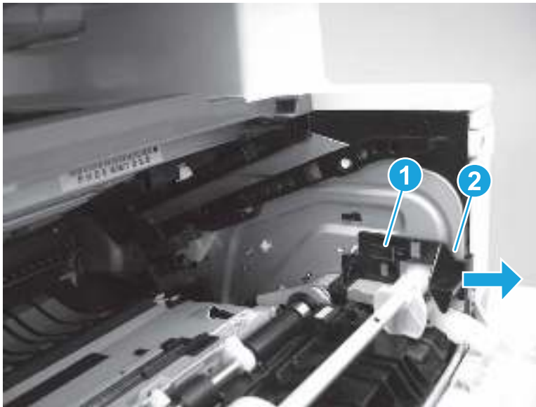
Figure 5-588 Remove the guide
