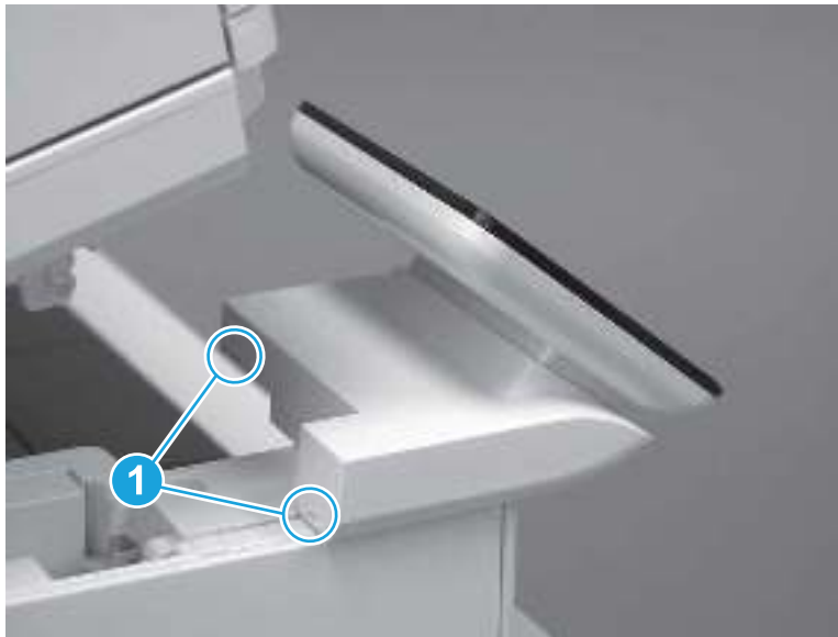
Figure 5-160 Release two tabs
