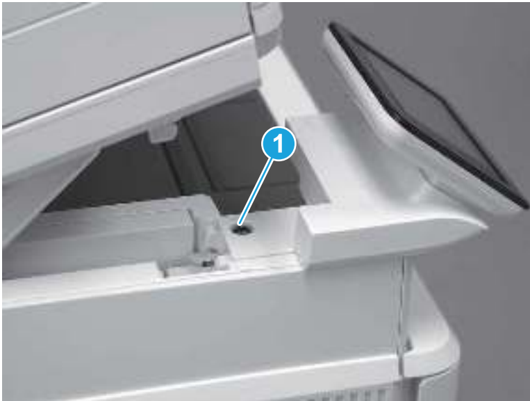
Figure 5-159 Remove one screw
