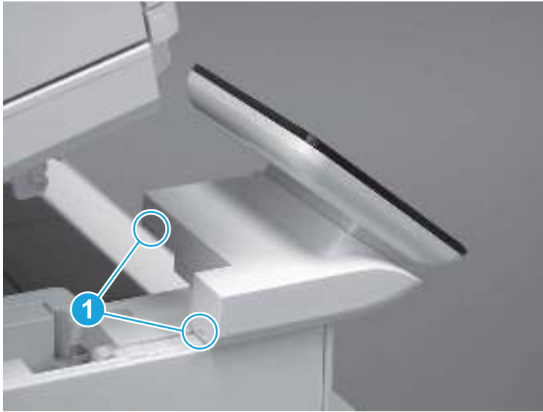
Figure 5-302 Release two tabs
