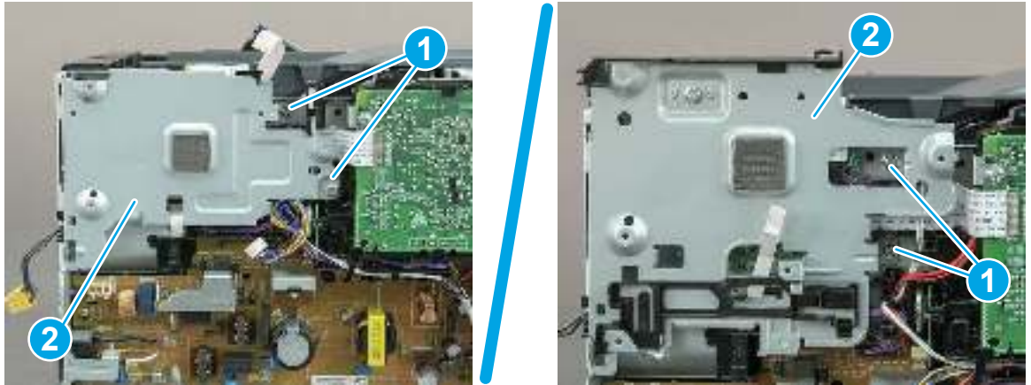
Figure 5-921 Remove two screws
