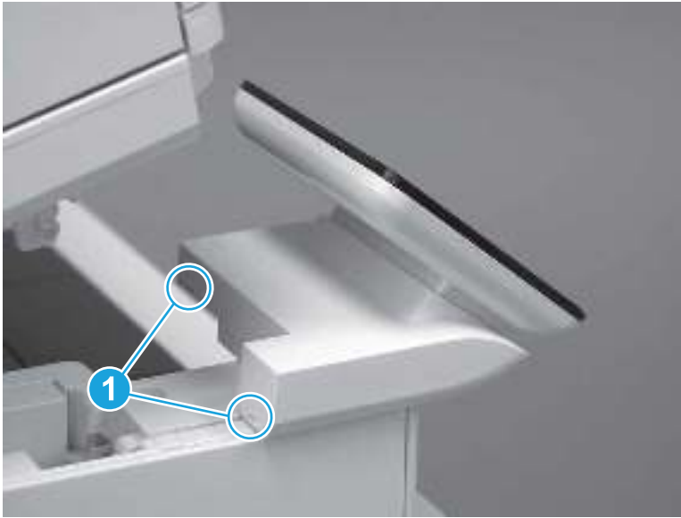
Figure 5-356 Release two tabs
