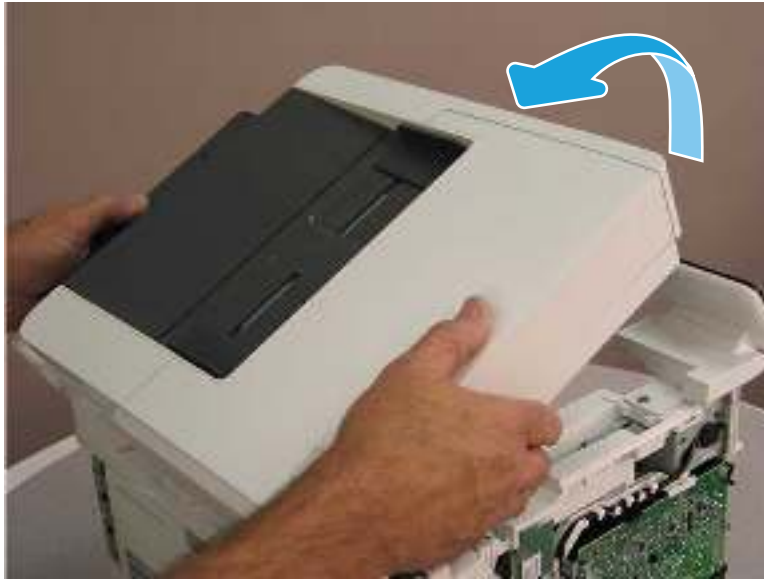
Figure 5-784 Rotate the ISA towards the rear of the printer
