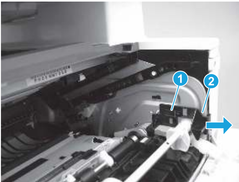
Figure 5-933 Remove the guide
