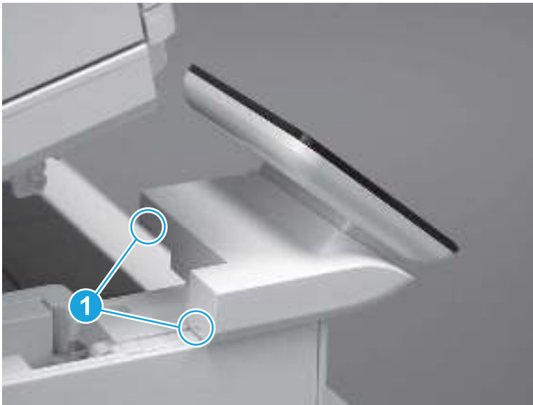
Figure 5-767 Release two tabs
