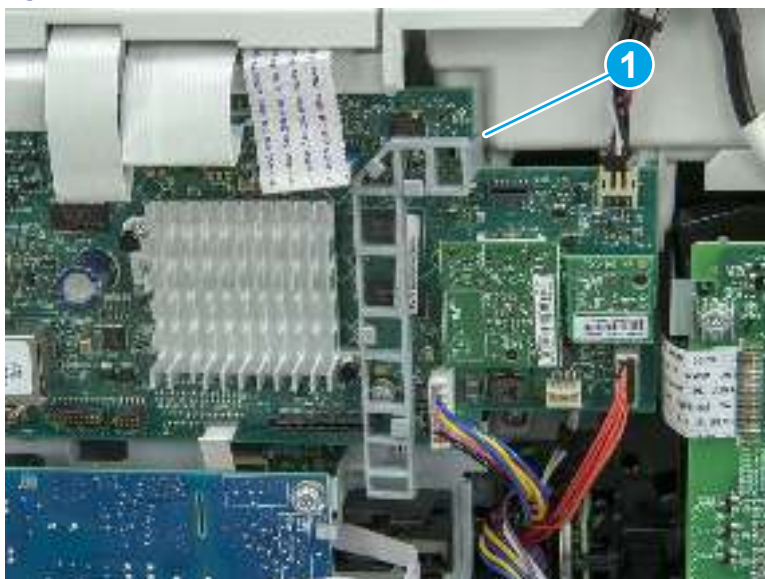
Figure 5-795 Release one tab
