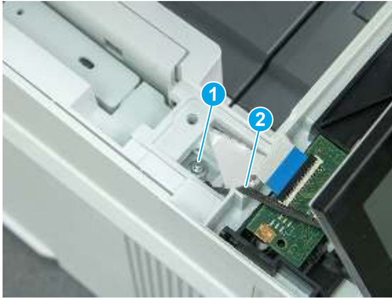
Figure 5-963 Remove one screw
