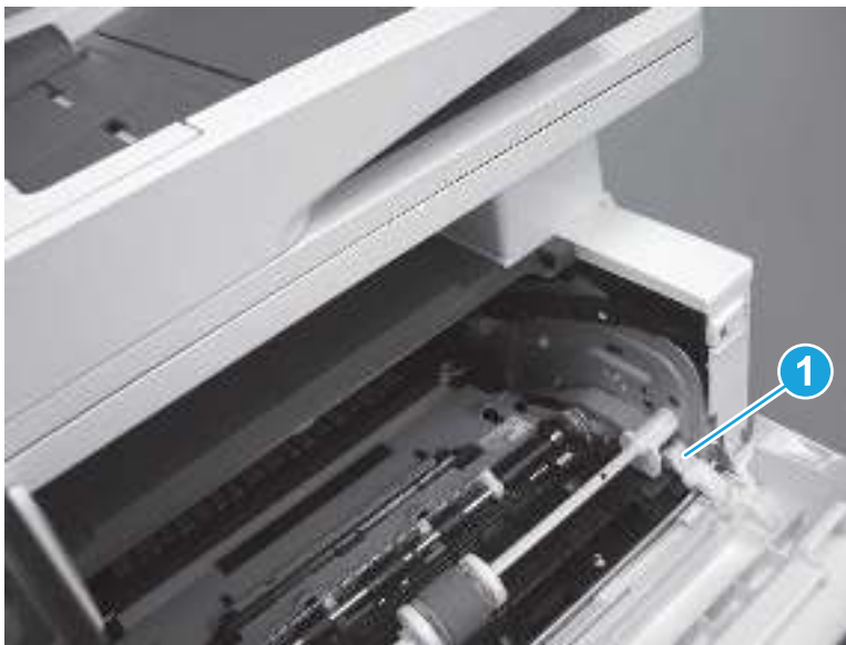
Figure 5-129 Release the pressure-release link
