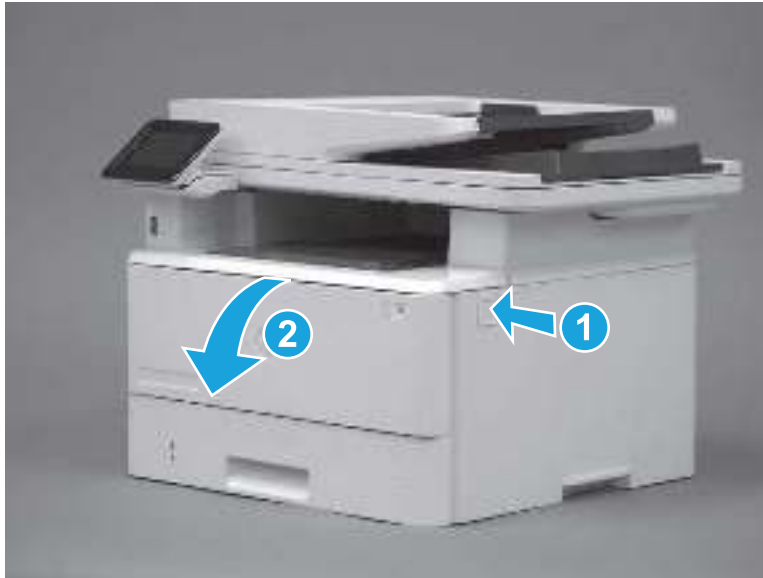
Figure 5-11 Open the toner-cartridge door
