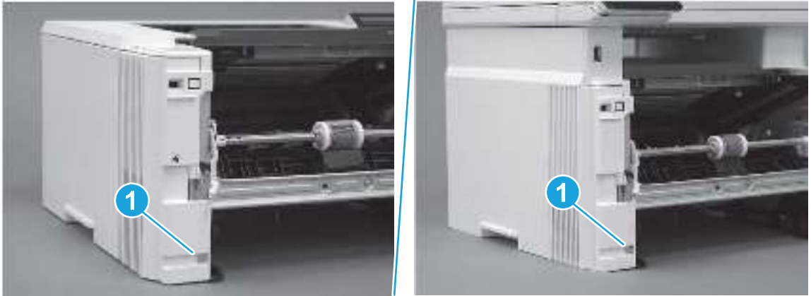
Figure 5-703 Remove one screw
