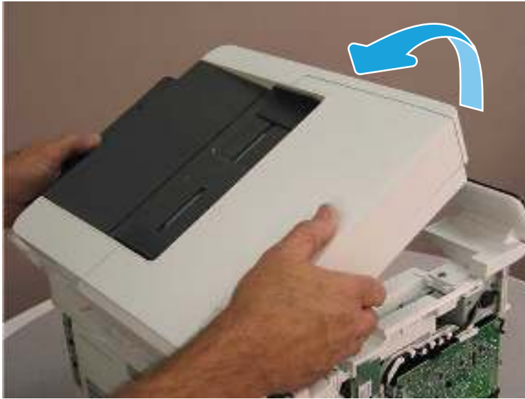
Figure 5-899 Rotate the ISA towards the rear of the printer
