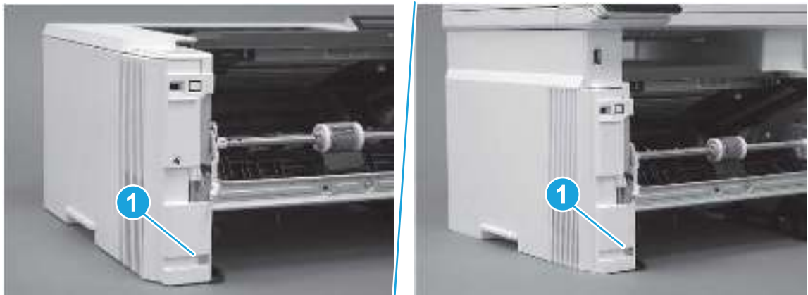
Figure 5-251 Remove one screw
