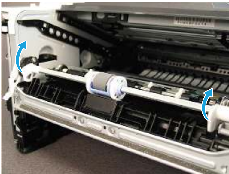
Figure 5-1019 Rotate the Tray 1 pickup roller shaft
