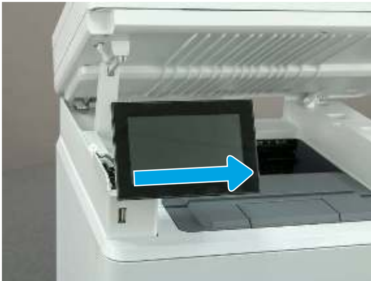
Figure 5-973 Slide the control panel display
