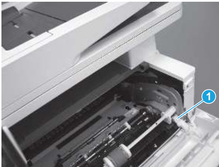
Figure 5-343 Release the pressure-release link
