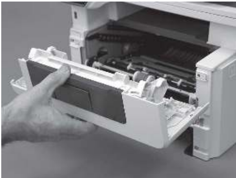
Figure 5-548 Remove the door
