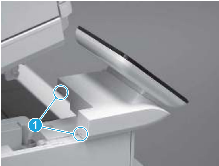
Figure 5-600 Release two tabs
