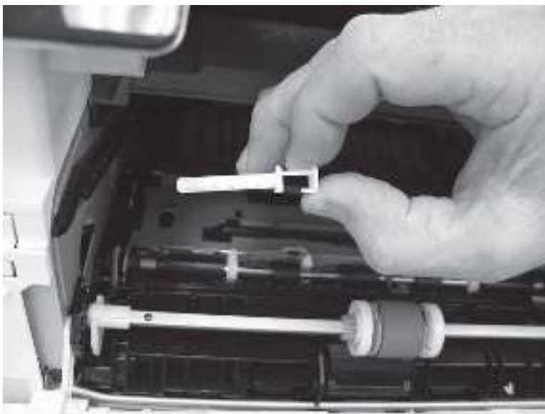
Figure 5-320 Remove the support shaft
