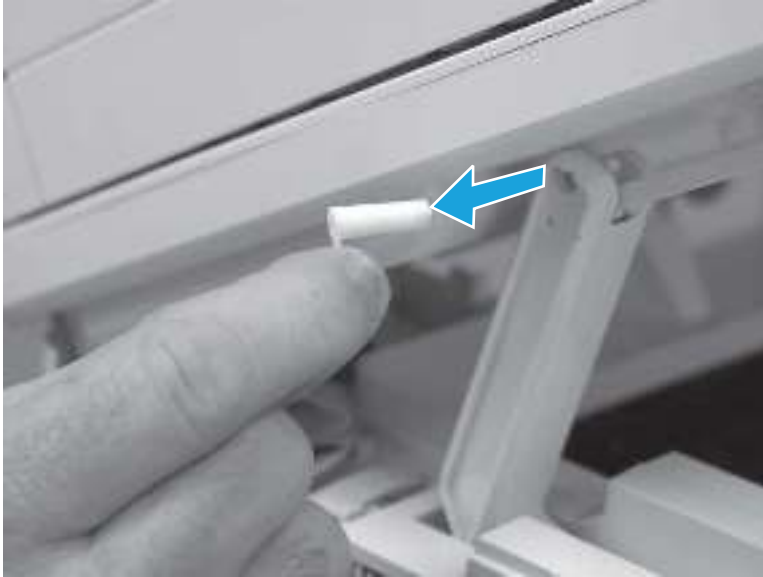
Figure 5-220 Remove the slider pin
