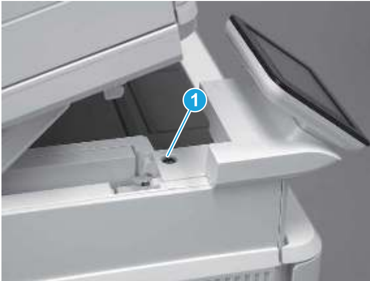
Figure 5-766 Remove one screw
