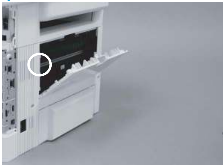
Figure 2-53 Defeat the rear door interlock
