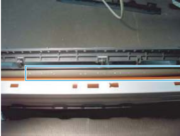
Figure 2-116 Contaminated fuser film
