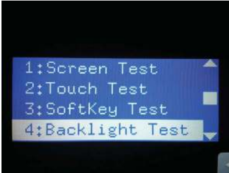
Figure 2-41 Open the backlight test
