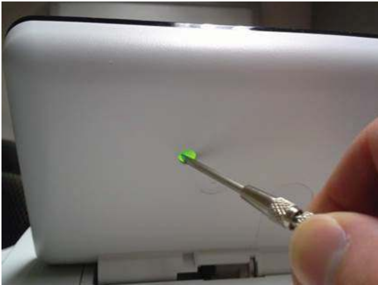
Figure 2-28 Press the diagnostics-access button (M507x and E50145dn)
