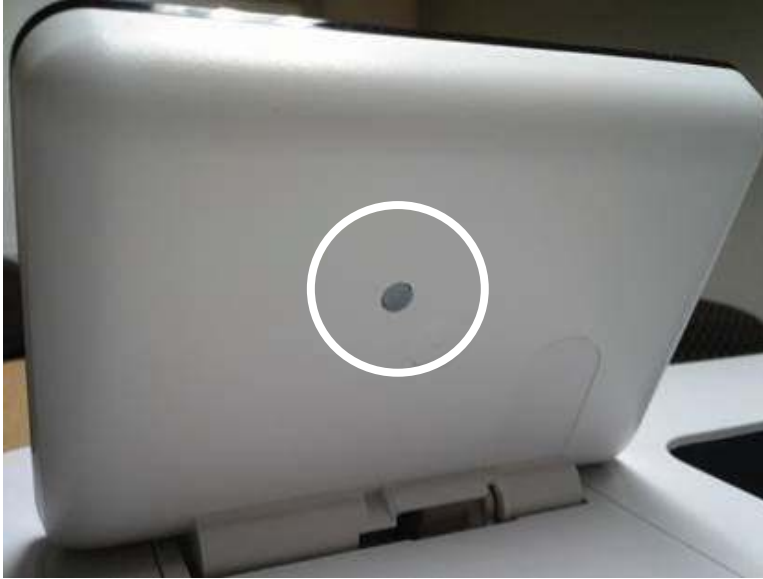
Figure 2-27 Diagnostic-tests access button (M507x and E50145dn)
