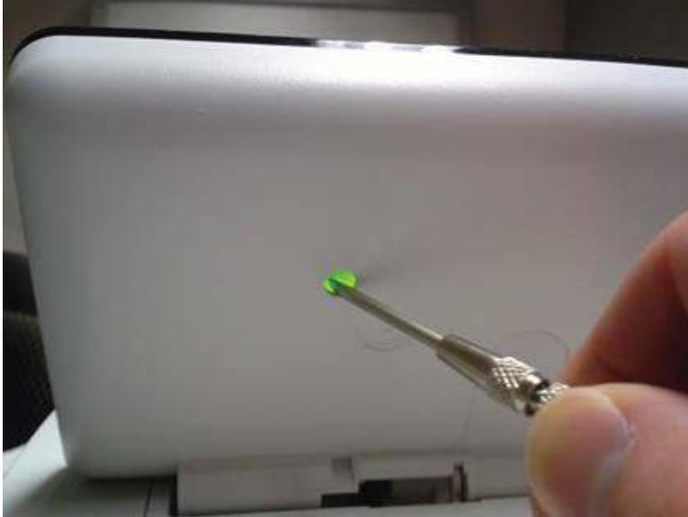
Figure 2-22 Press the diagnostics-access button (M506x)
