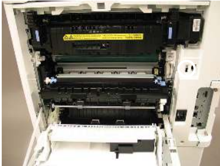
Figure 2-52 Defeat the right or rear door interlock
