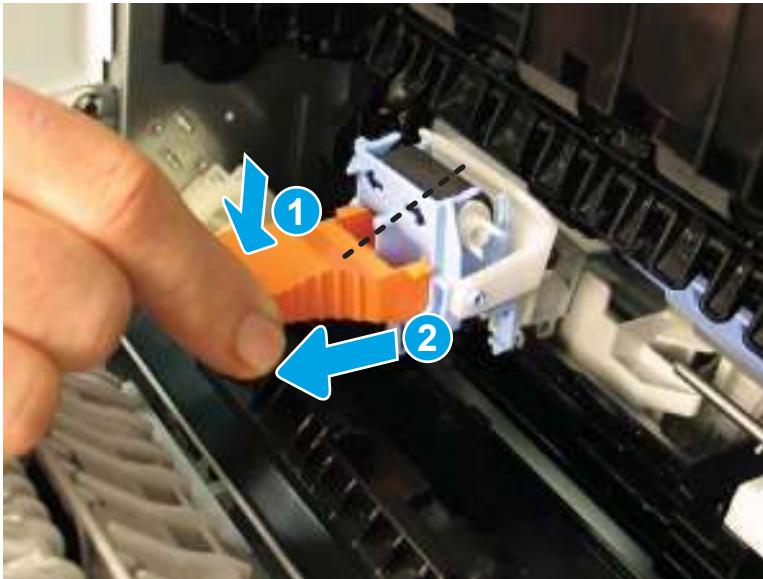
Figure 2-139 Remove the roller
