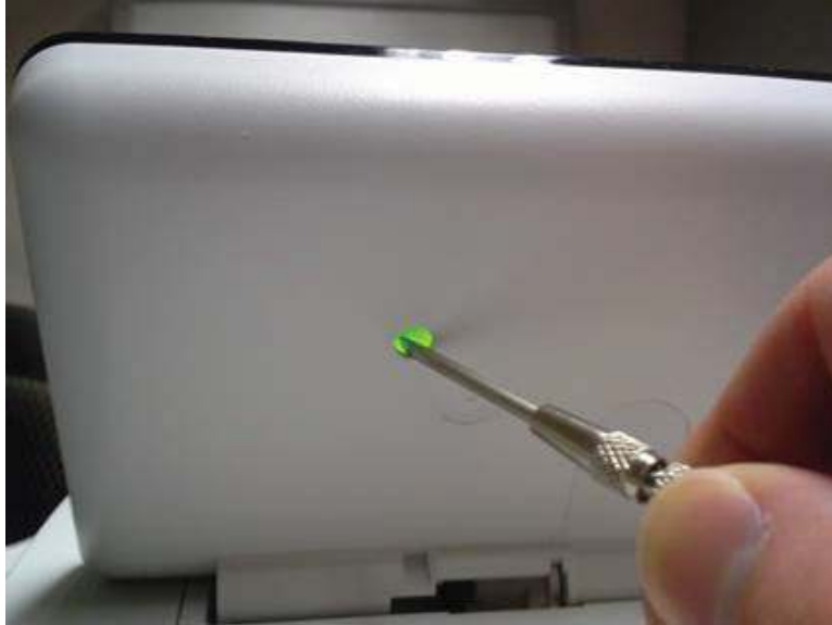
Figure 2-24 Press the diagnostics-access button (small touchscreen)
