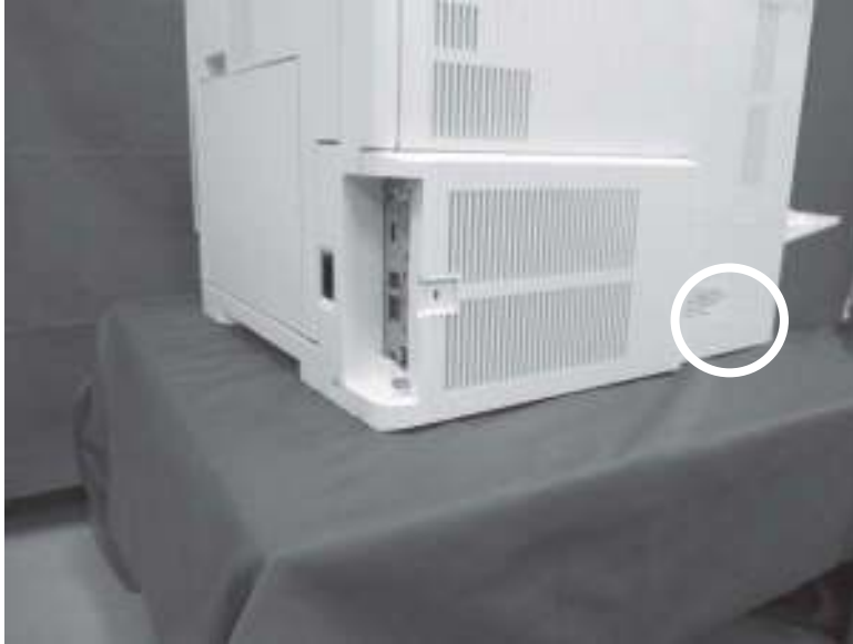
Figure 2-50 Engine test button (2 of 2)
