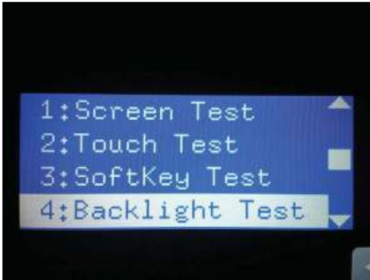
Figure 2-40 Open the backlight test
