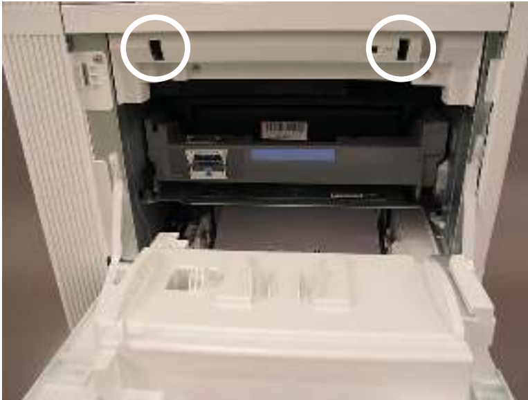
Figure 2-51 Defeat the toner cartridge door interlocks
