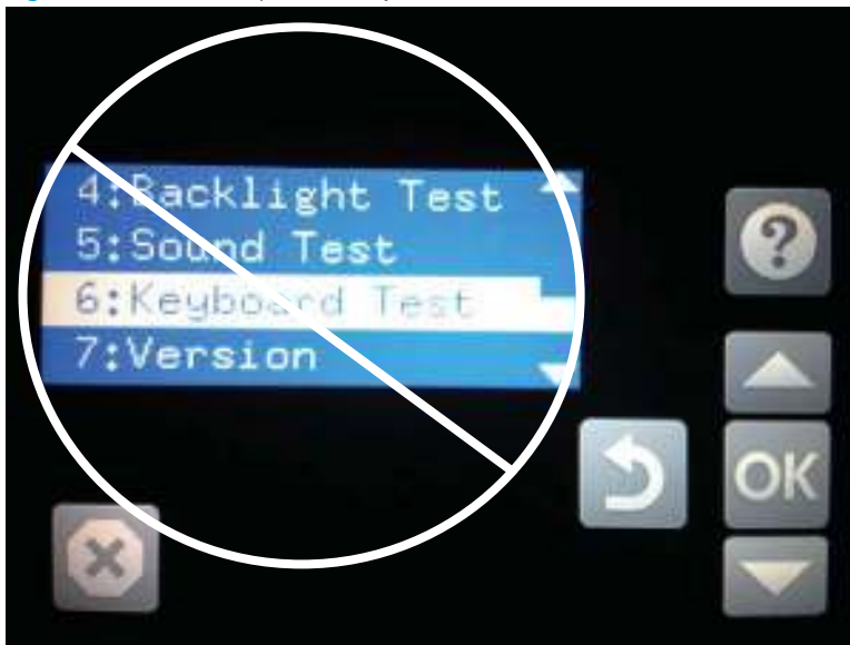
Figure 2-42 Do not open the keyboard test
