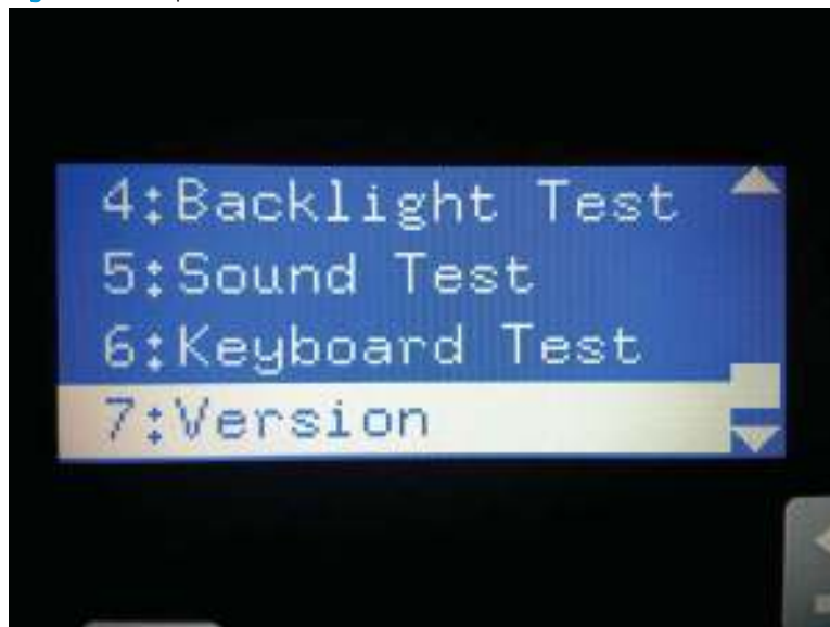
Figure 2-43 Open the sound test
