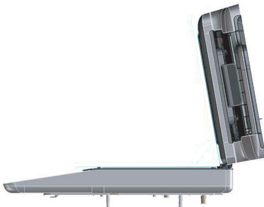
Figure 1-52 Document feeder open (60° to 80°)
