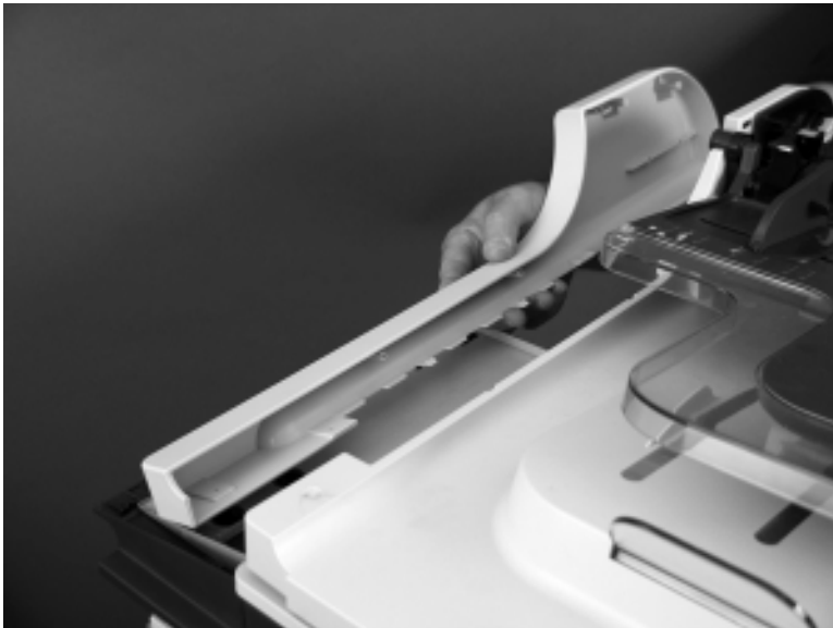
Figure 1-323 Remove the document feeder front cover (8 of 8)
