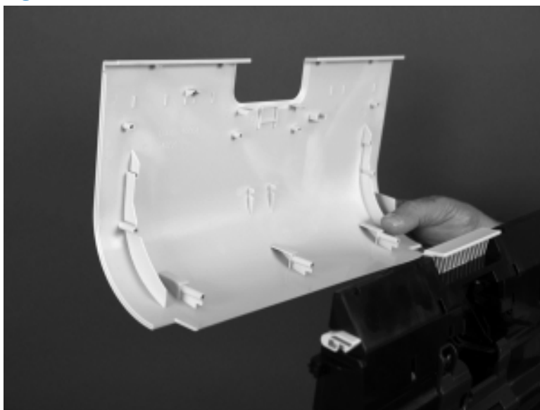
Figure 1-325 Remove the document feeder hatch cover (2 of 2)
