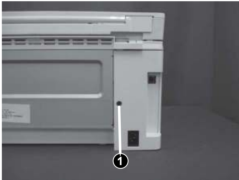
Figure 1-91 Install one screw (MFP)
