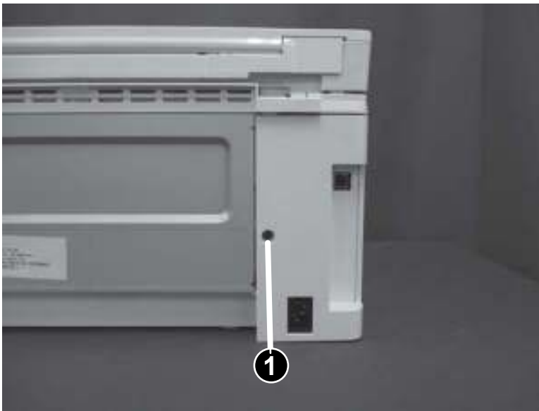
Figure 1-103 Install one screw
