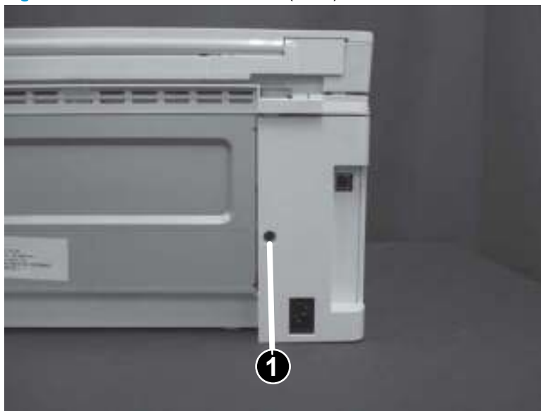
Figure 1-325 Remove one screw (MFP)
