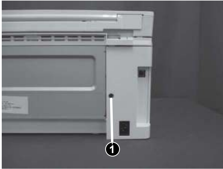
Figure 1-540 Install one screw (MFP)
