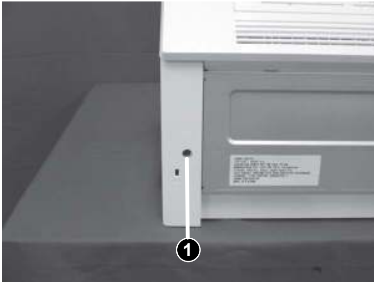
Figure 1-181 Install one screw (SFP)
