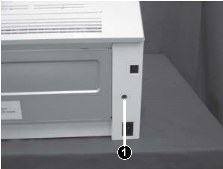
Figure 1-238 Install one screw (SFP)
