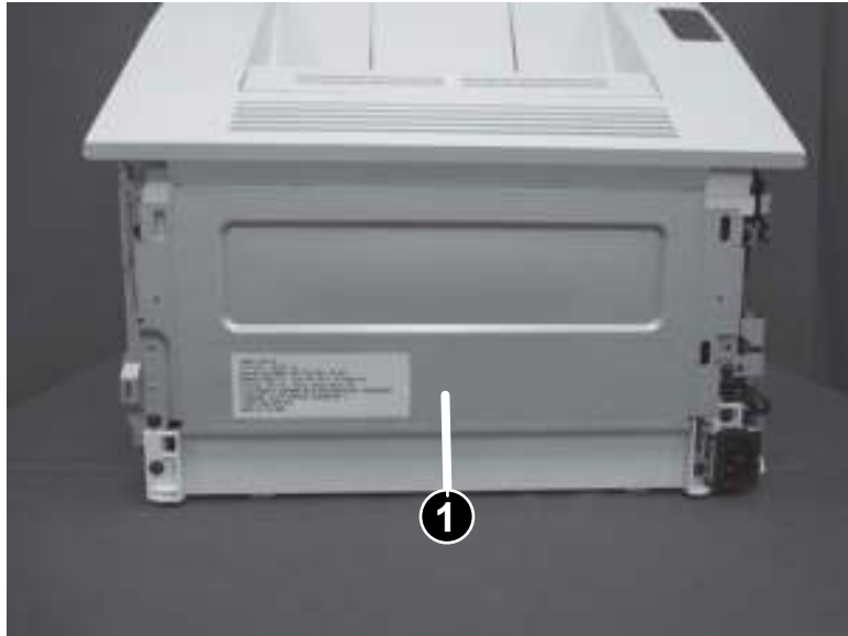
Figure 1-340 Remove the rear panel (SFP)
