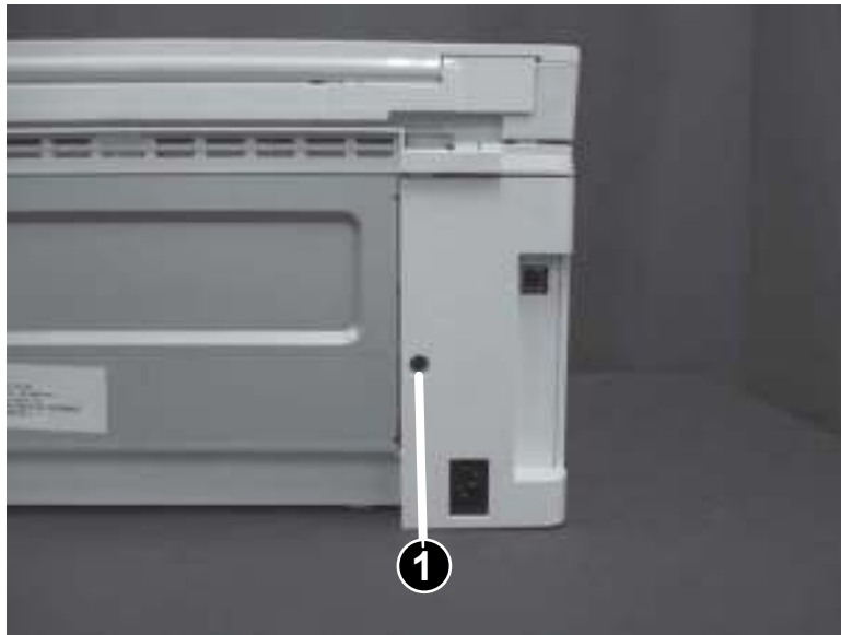
Figure 1-438 Install one screw
