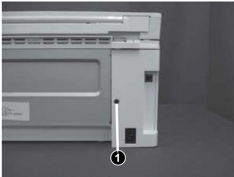
Figure 1-85 Remove one screw (MFP)
