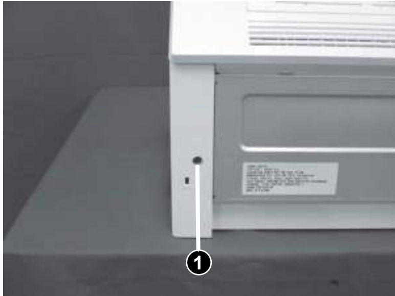
Figure 1-1012 Install one screw (SFP)
