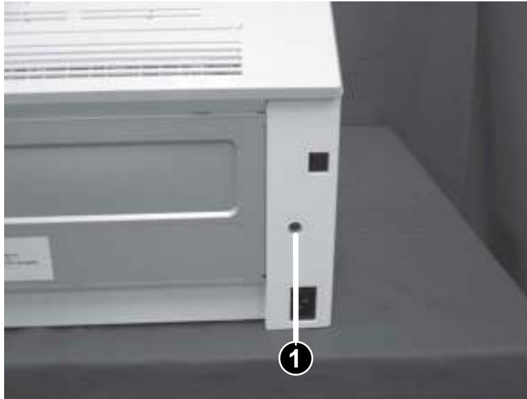
Figure 1-468 Install one screw (SFP)
