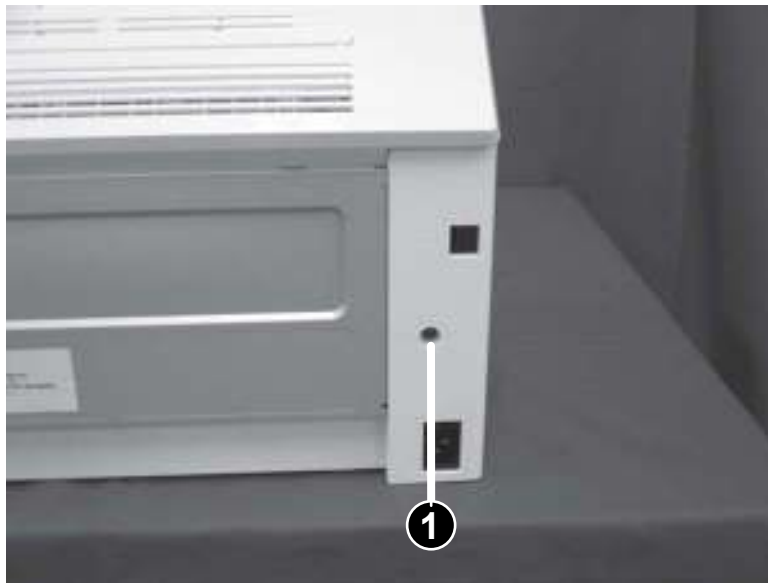
Figure 1-154 Remove one screw (SFP)
