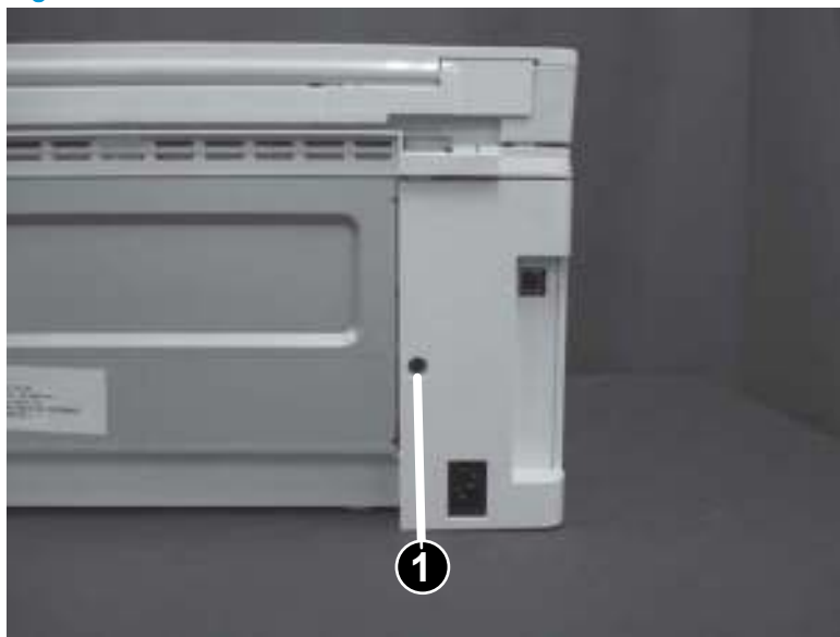
Figure 1-244 Remove one screw
