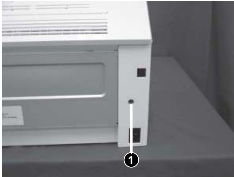
Figure 1-617 Remove one screw (SFP)
