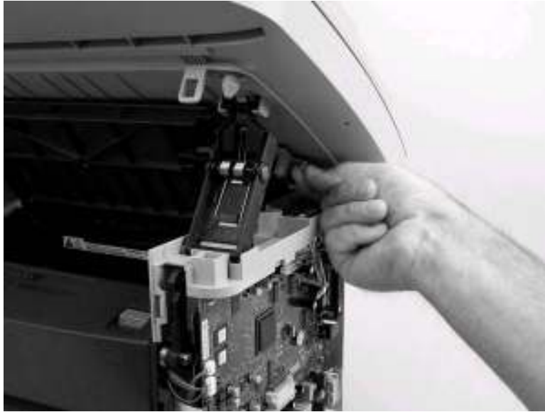
Figure 5-81. Remove the scanner assembly (7 of 13)
