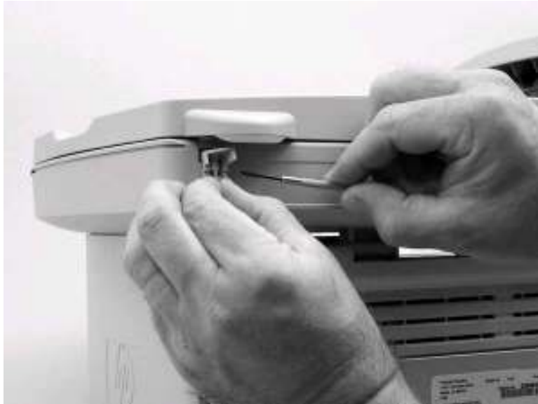
Figure 5-57. Remove the flatbed lid (4 of 5)
