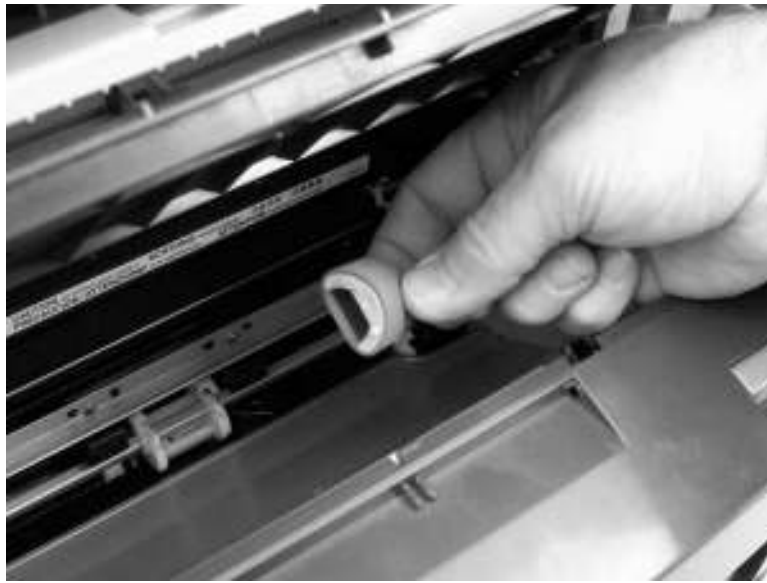
Figure 5-95. Remove the printer pickup roller (3 of 5)
