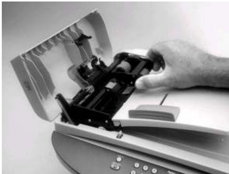
Figure 5-70. Remove the ADF pickup roller (2 of 2)
