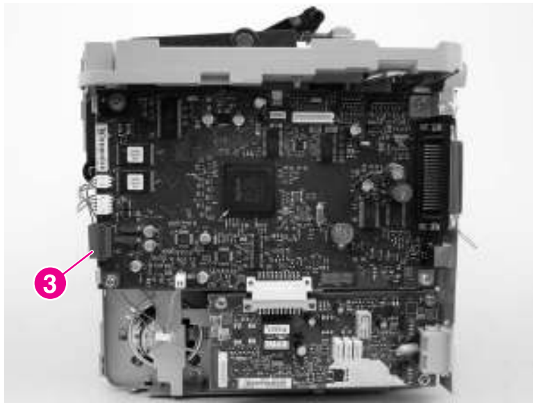
Figure 5-135. Remove the ECU (3 of 6)
