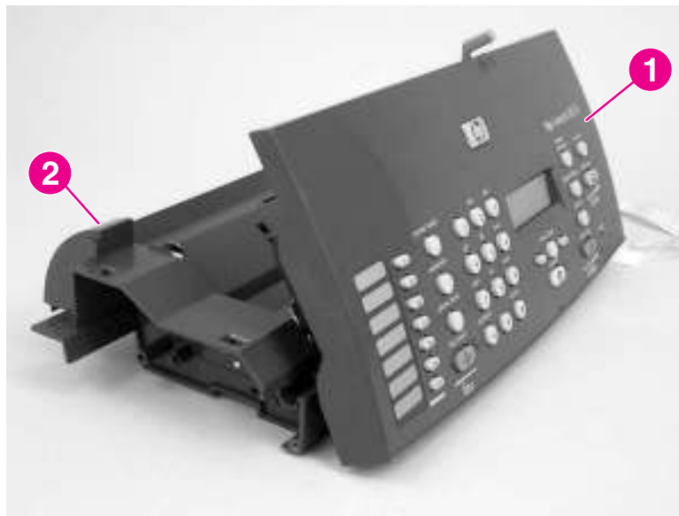
Figure 5-45. Remove the top-cover assembly (1 of 2)
