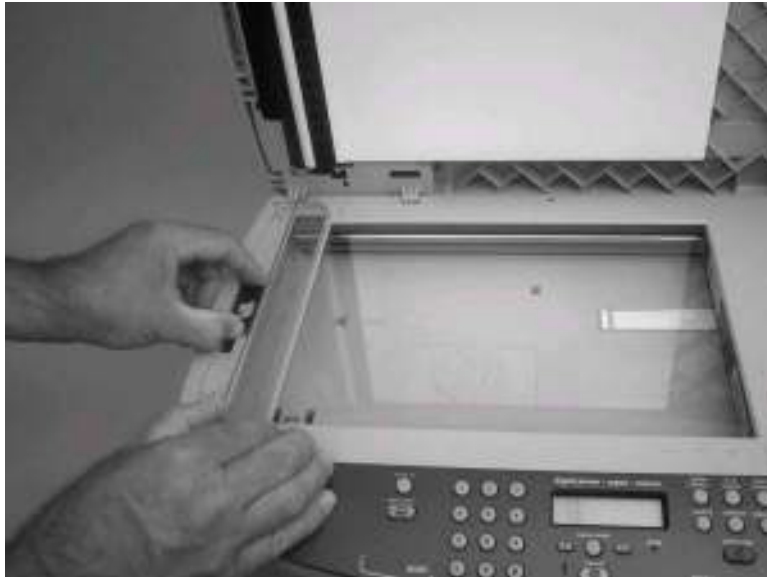
Figure 5-73. Remove the ADF scanner glass (3 of 3)
