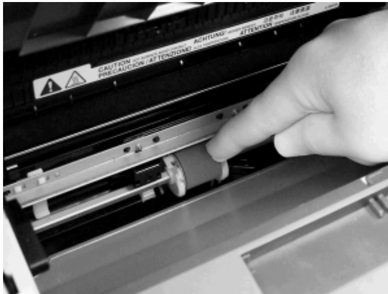
Figure 5-97. Remove the printer pickup roller (5 of 5)
