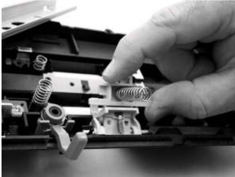
Figure 5-22. Remove the separation pad assembly (2 of 3)
