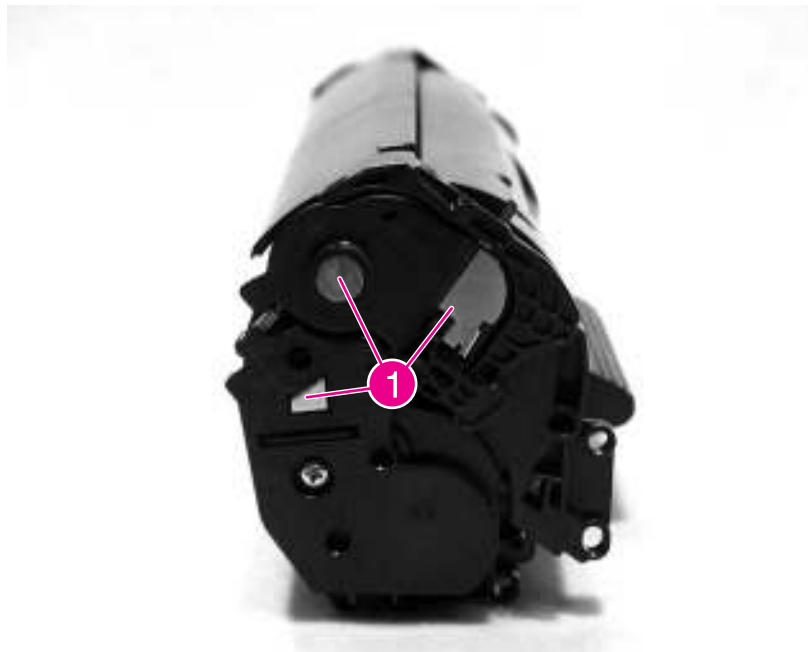
Figure 6-15. Print-cartridge high-voltage contacts
