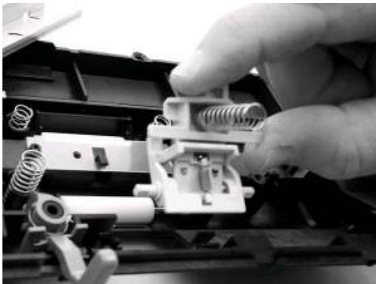
Figure 5-23. Remove the separation pad assembly (3 of 3)
