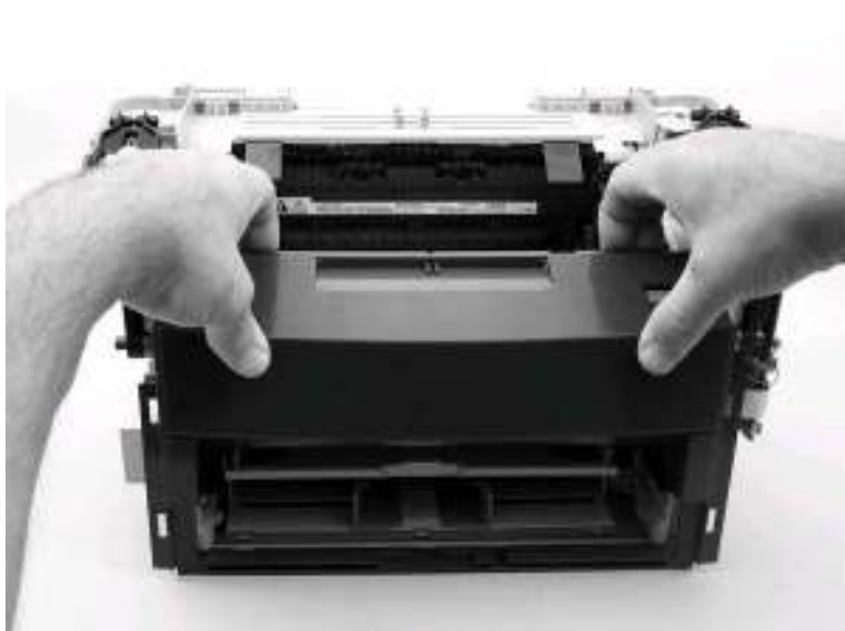
Figure 5-115. Remove the front cover (3 of 3)
