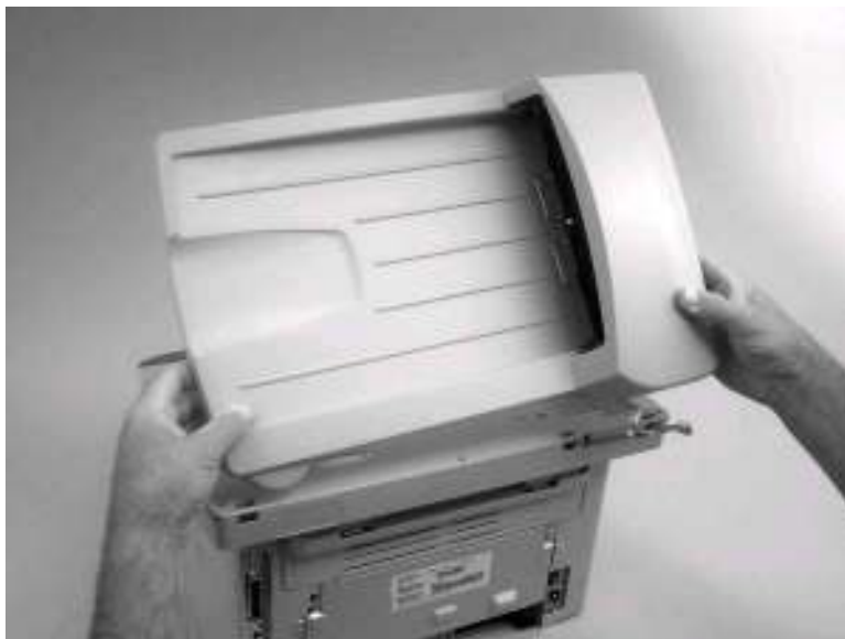
Figure 5-58. Remove the flatbed lid (5 of 5)
