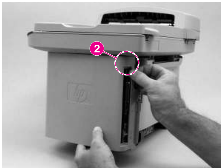
Figure 5-76. Remove the scanner assembly (2 of 13)
