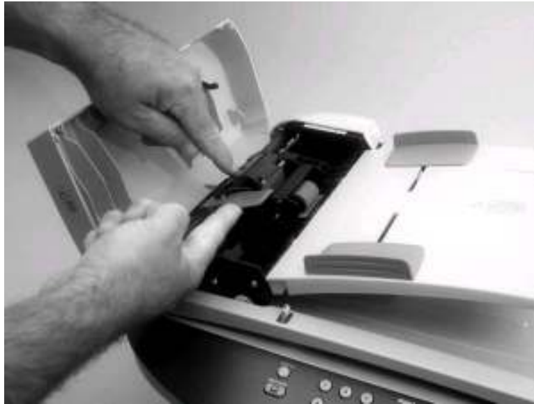
Figure 5-69. Remove the ADF pickup roller (1 of 2)
