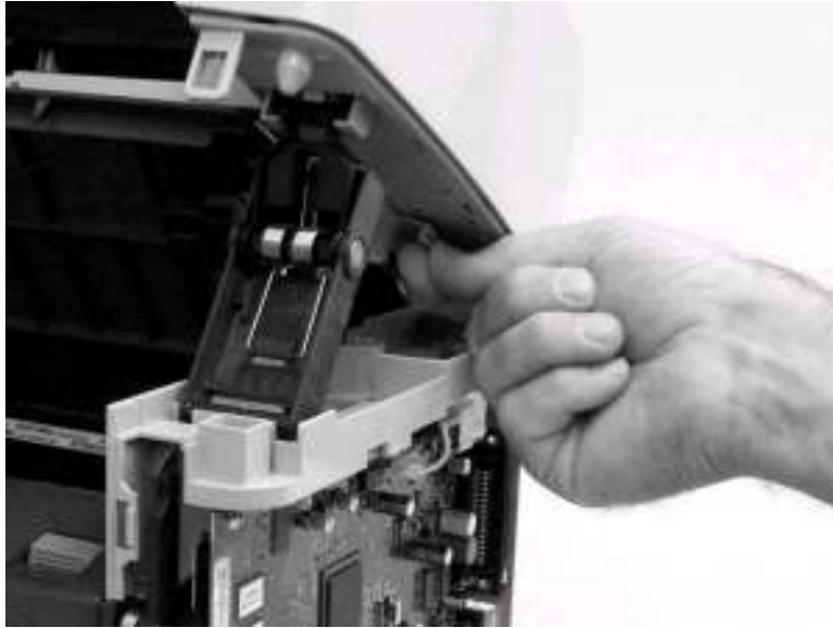
Figure 5-32. Remove the scanner assembly (9 of 15)
