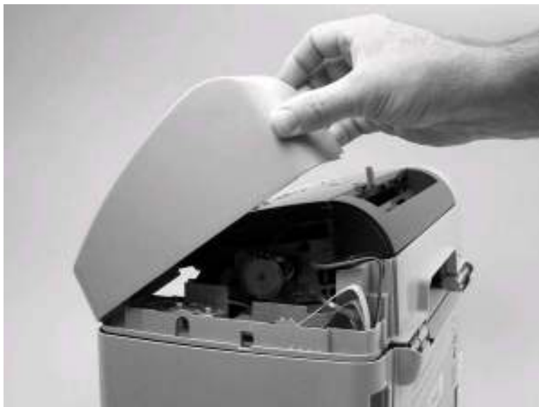
Figure 5-12. Remove the scanner side covers (3 of 3)
