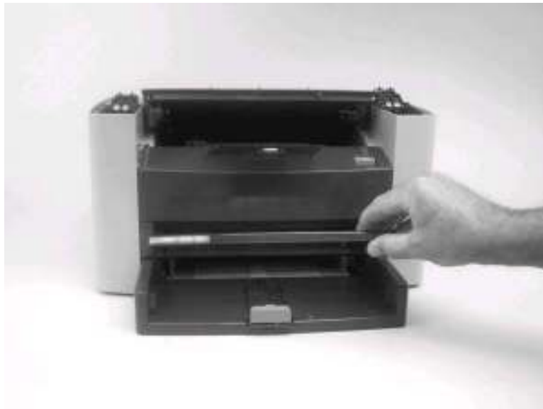
Figure 5-98. Remove the media input tray (1 of 3)
