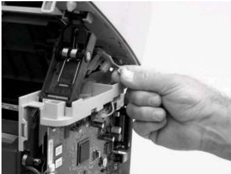
Figure 5-33. Remove the scanner assembly (10 of 15)
