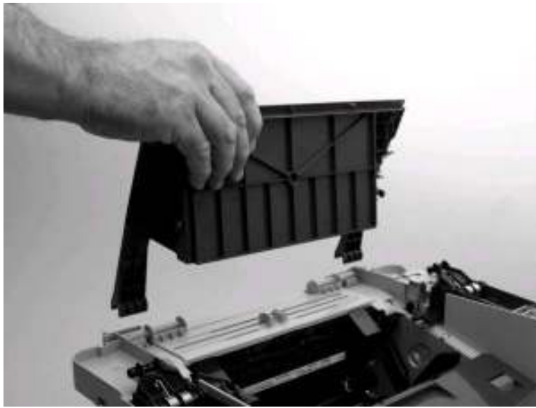
Figure 5-109. Remove the print-cartridge door (2 of 2)
