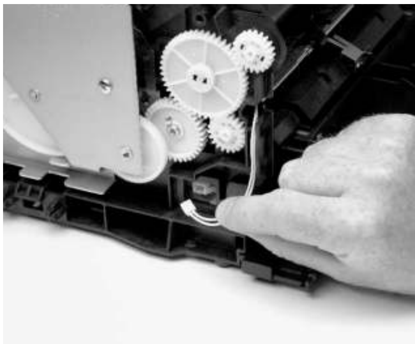
Figure 49. Fusing element removal (2 of 4)
