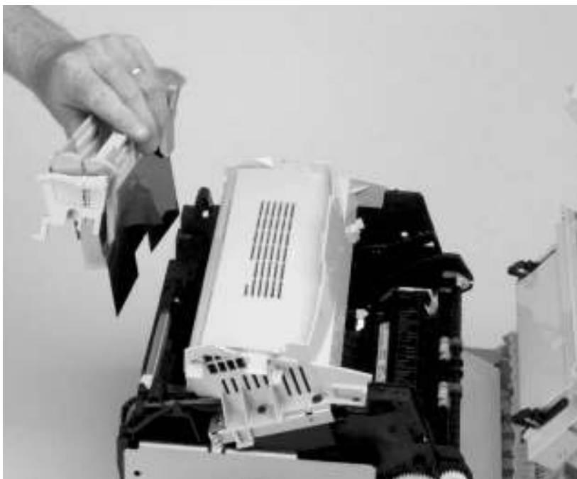
Figure 22. Internal paper guide removal
