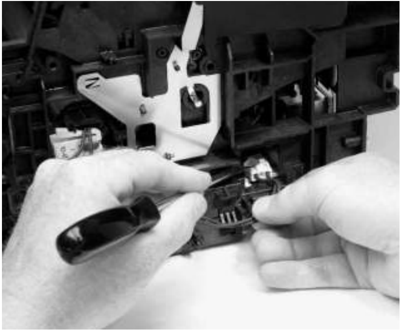
Figure 50. Fusing element removal (3 of 4)
