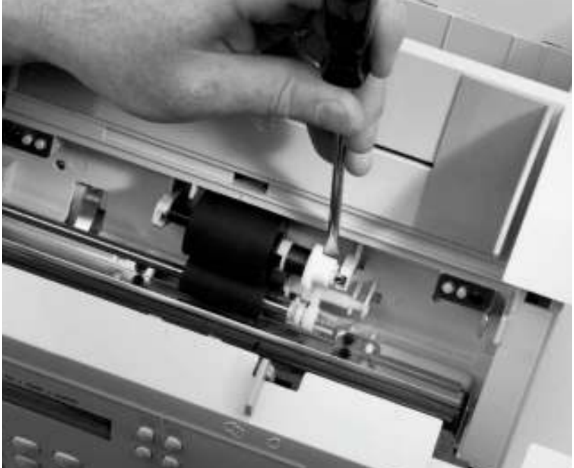
Figure 33. Document scanner pickup roller removal
