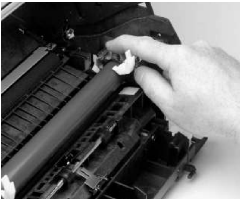
Figure 48. Fusing element metal clips reinstallation
