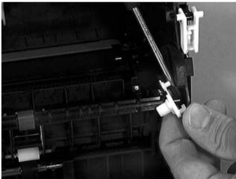
Figure 42. Output roller removal (1 of 2)
