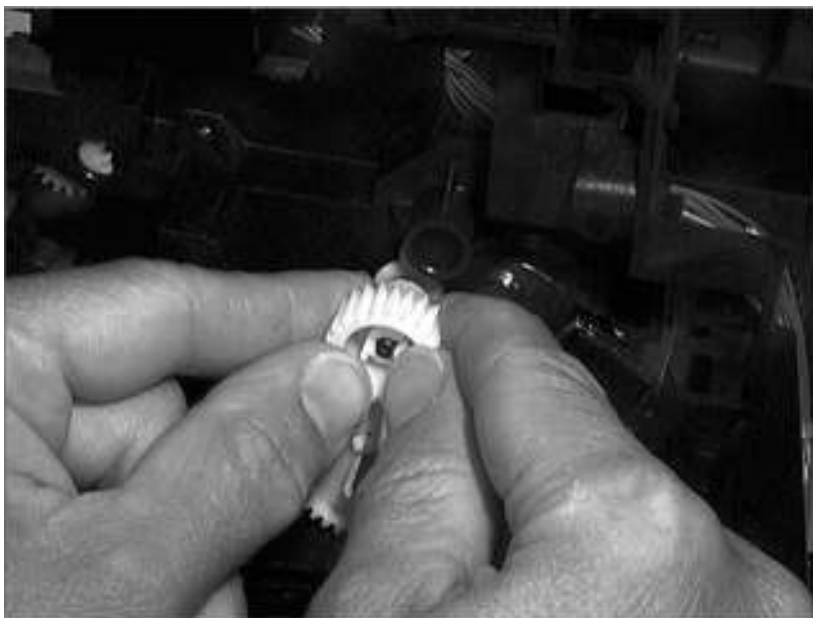
Figure 69. Paper-feed assembly removal (2 of 3)
