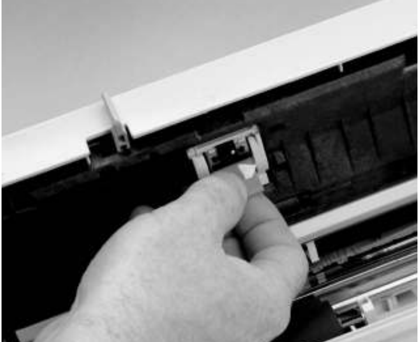
Figure 34. Document scanner separation pad removal
