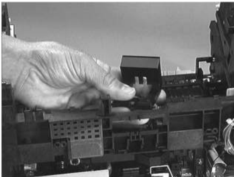
Figure 63. Separation pad removal (2 of 2)
