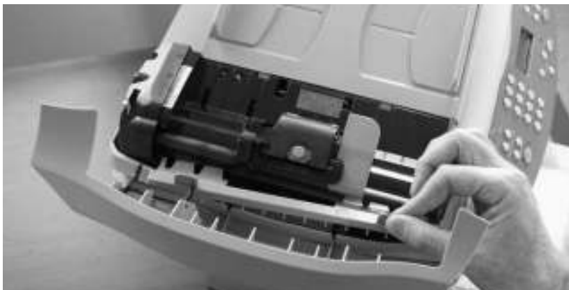
Figure 32. Removing the document feed guide (1 of 2)
