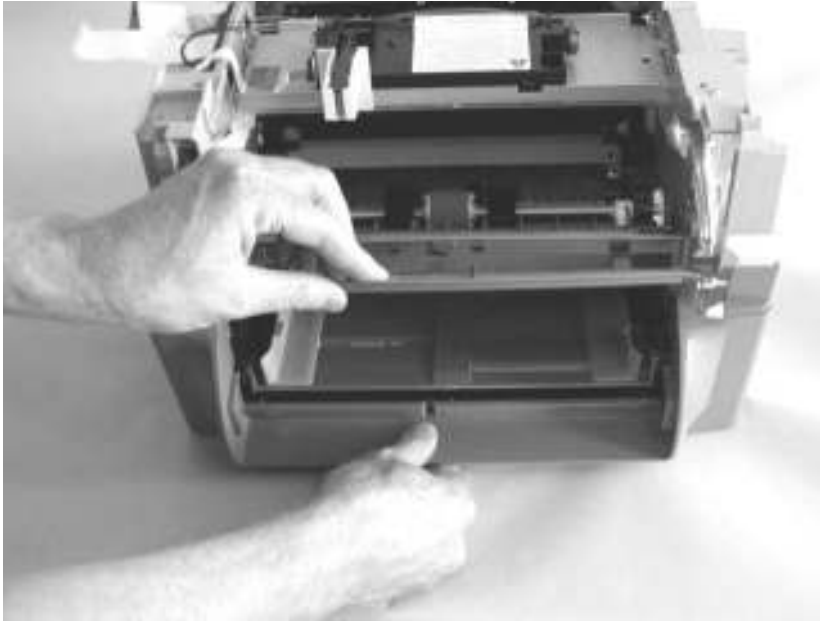
Figure 52. Removing the front cover (2 of 2)
