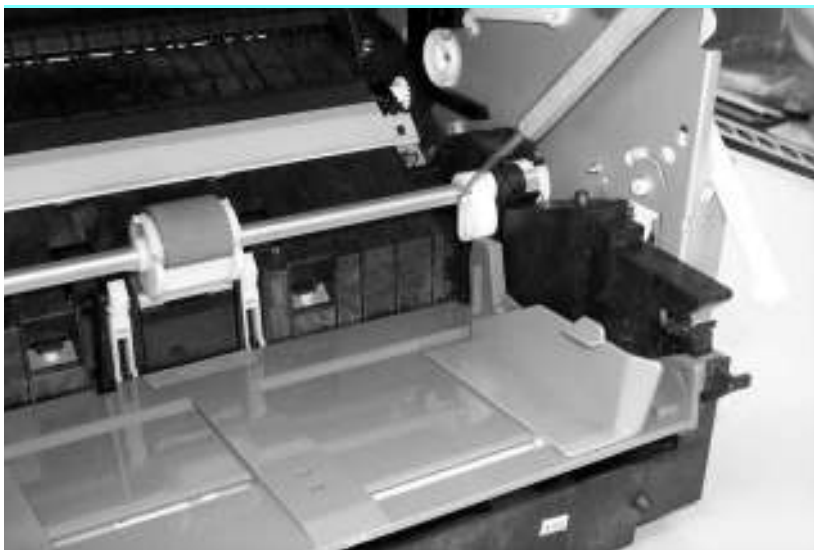
Figure 76. Removing the paper lift-plate assembly (1 of 3)
