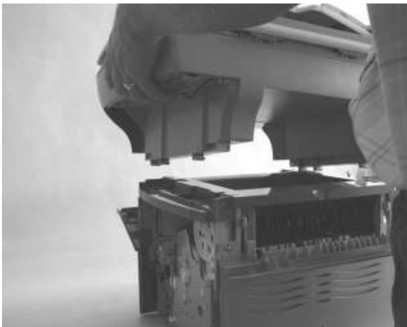
Figure 30. Separating the scanner from the printer (4 of 4)
