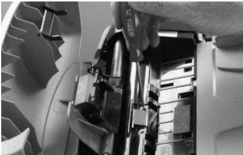
Figure 34. Removing the ADF separation pad
