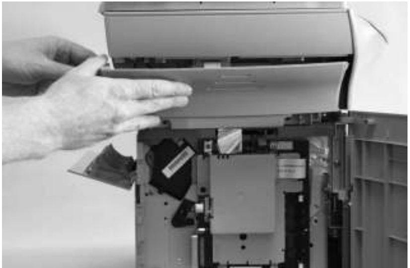
Figure 26. Removing the left scanner cover
