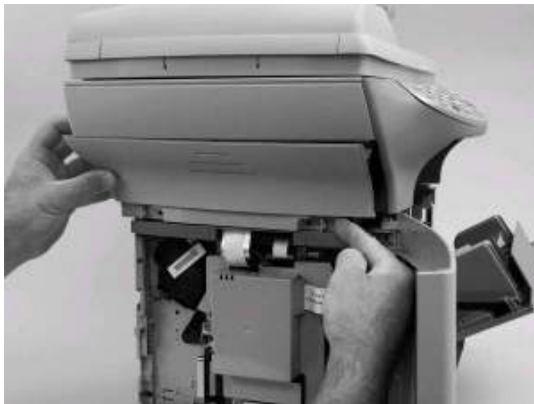
Figure 5-10. Remove the left-side scanner cover (2 of 2)
