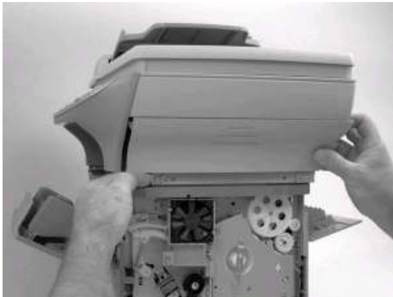
Figure 5-8. Remove the scanner right-side cover (2 of 2)
