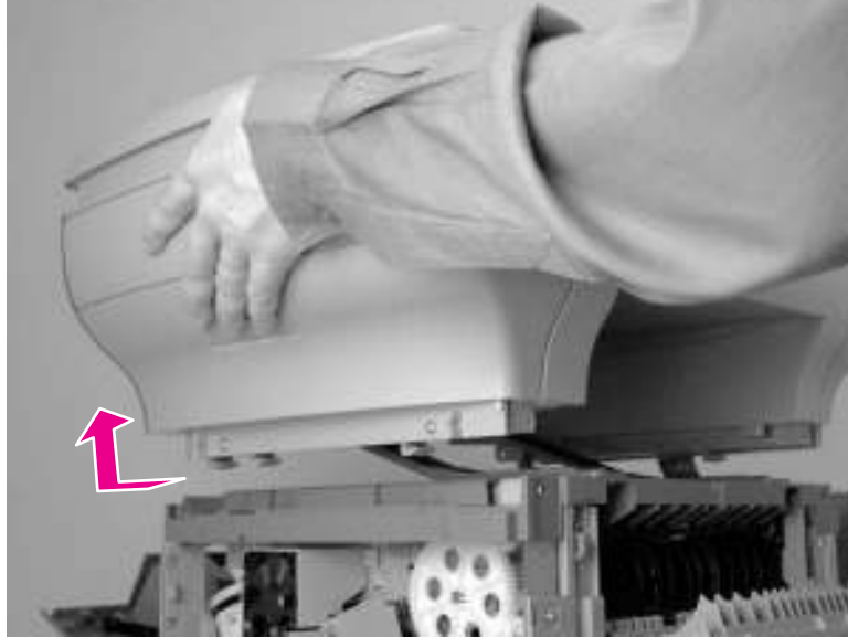
Figure 5-40. Separate the scanner from the printer (4 of 4)
