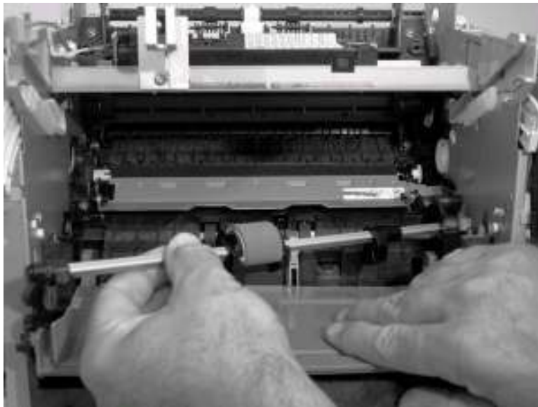
Figure 5-82. Remove the pickup roller shaft
