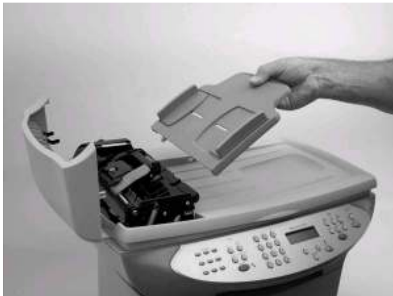
Figure 5-12. Remove the ADF pickup-roller assembly (1 of 5)
