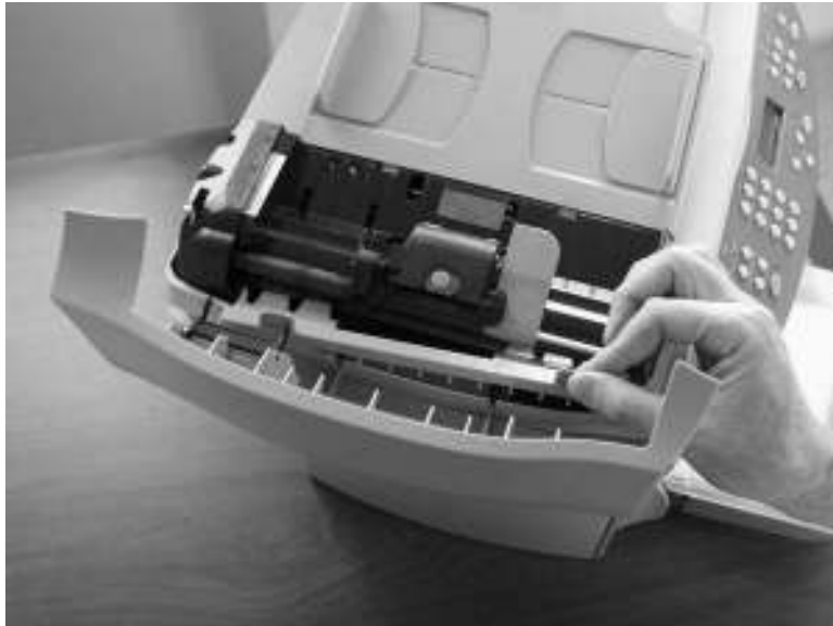
Figure 5-17. Remove the ADF document-feed guide/cleanout comb
