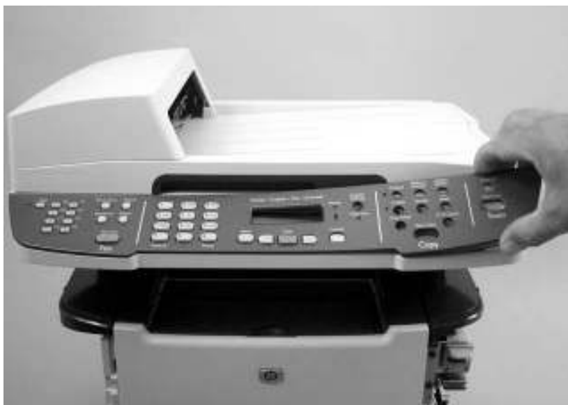
Figure 5-31 Remove the bezel and control panel (1 of 4)
