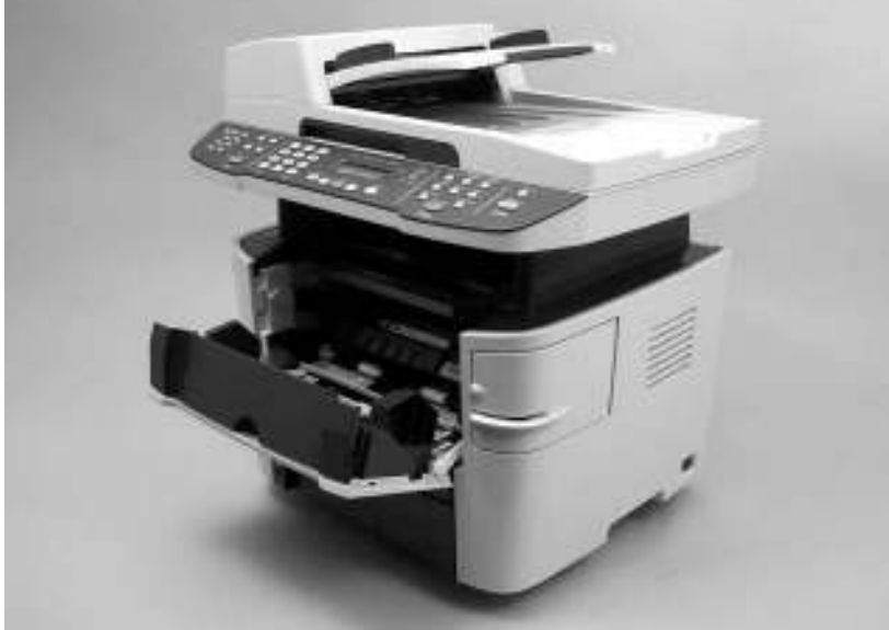
Figure 5-3 Remove the print cartridge (1 of 2)
