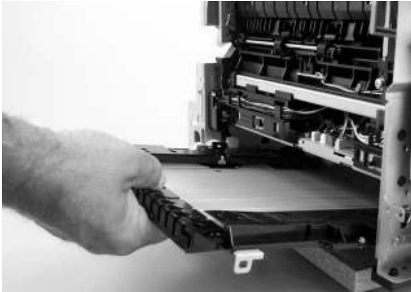
Figure 5-50 Remove the duplex assembly (3 of 3)
