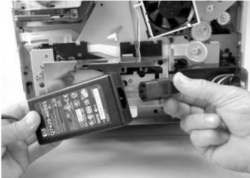
Figure 5-39 Remove the convenience-stapler power assembly (3 of 3)
