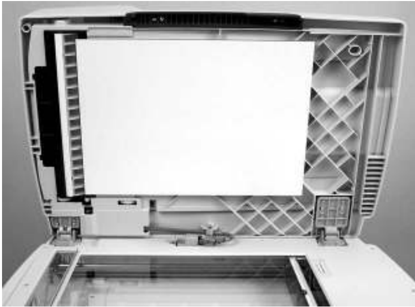
Figure 5-25 Remove the ADF assembly (1 of 3)
