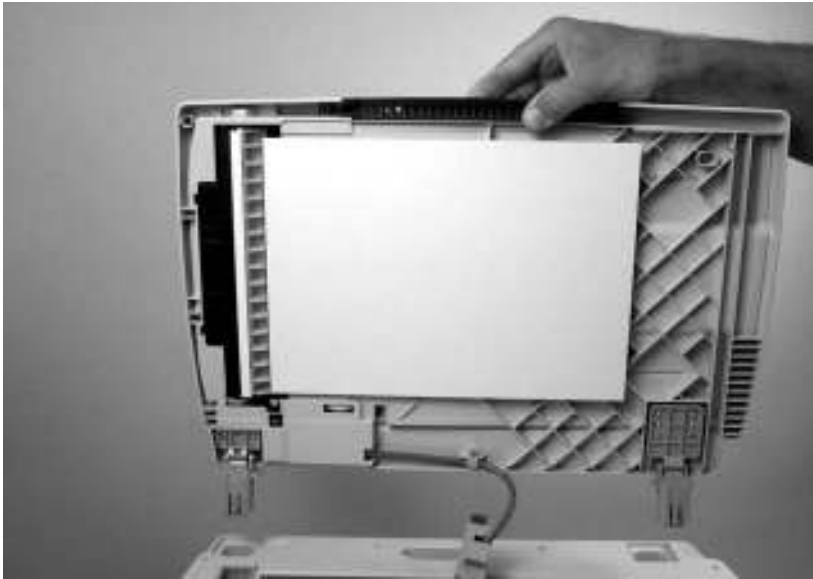
Figure 5-27 Remove the ADF assembly (3 of 3)
