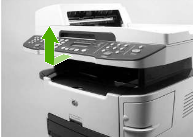
Figure 5-30 Remove the scanner/ADF assembly (3 of 3)
