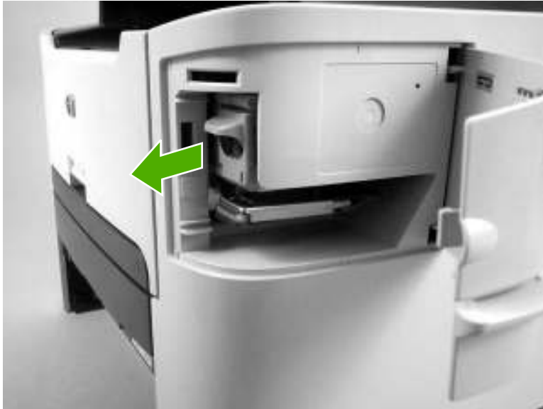
Figure 5-5 Remove the right cover (1 of 4)
