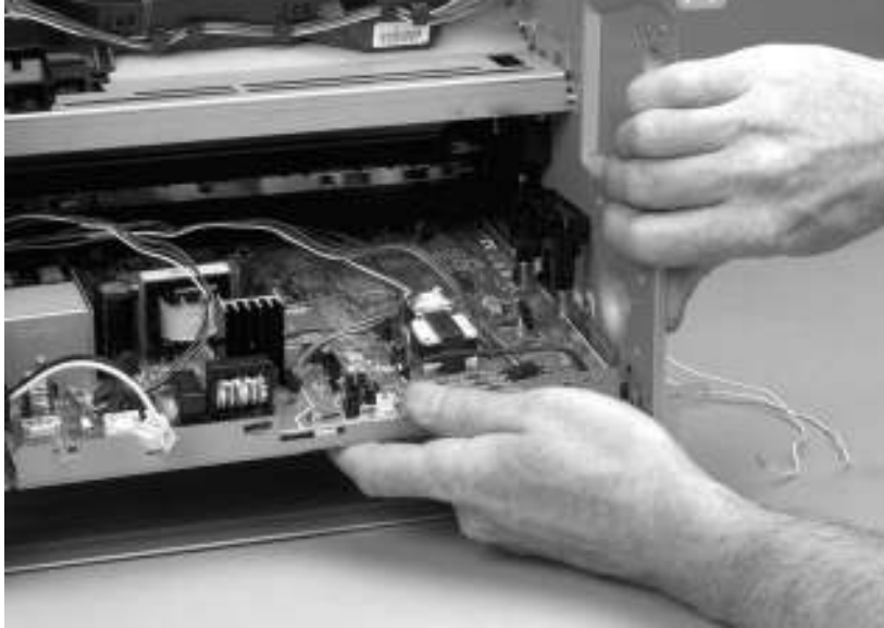
Figure 5-78 Remove the ECU (7 of 8)
