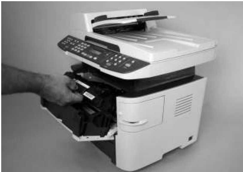
Figure 5-4 Remove the print cartridge (2 of 2)
