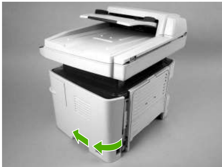
Figure 5-8 Remove the right cover (4 of 4)
