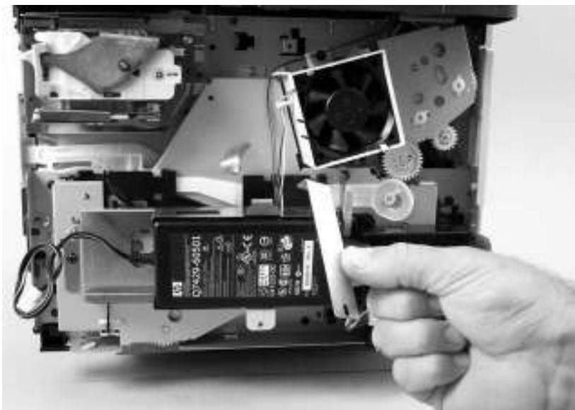
Figure 5-38 Remove the convenience-stapler power assembly (2 of 3)
