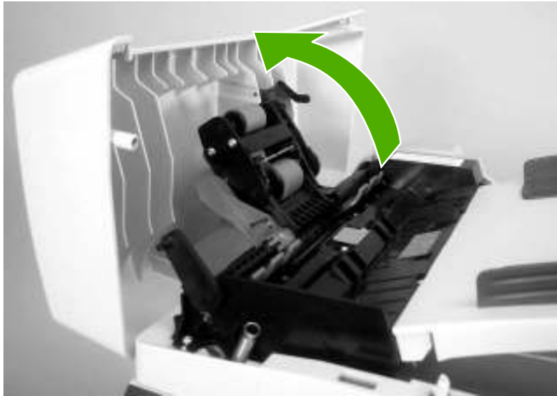
Figure 5-21 Replacing the ADF pickup-roller assembly (3 of 6)
