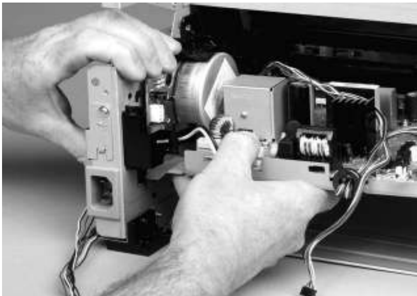
Figure 5-77 Remove the ECU (6 of 8)
