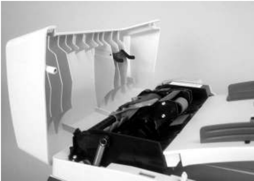
Figure 5-19 Replacing the ADF pickup-roller assembly (1 of 6)
