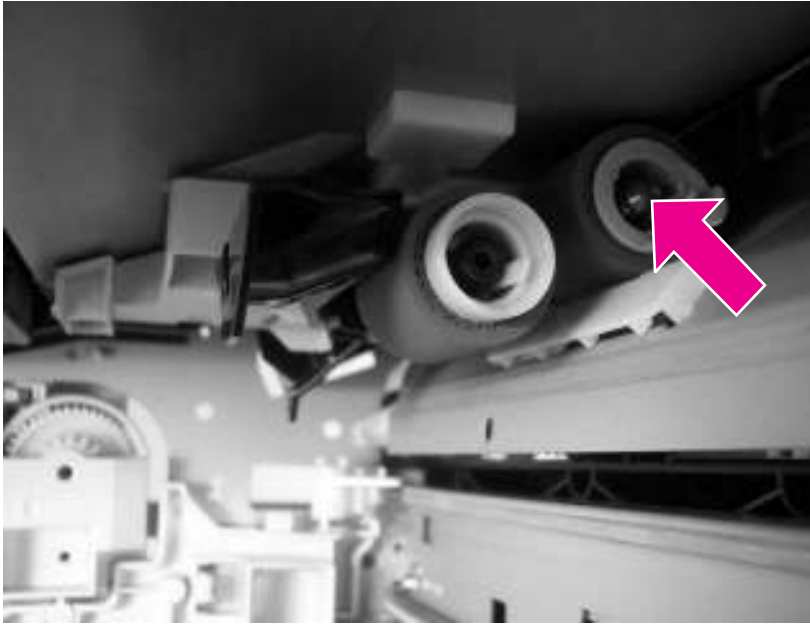
Figure 6-135 Cassette feed-roller shaft (push here while replacing the gear)
