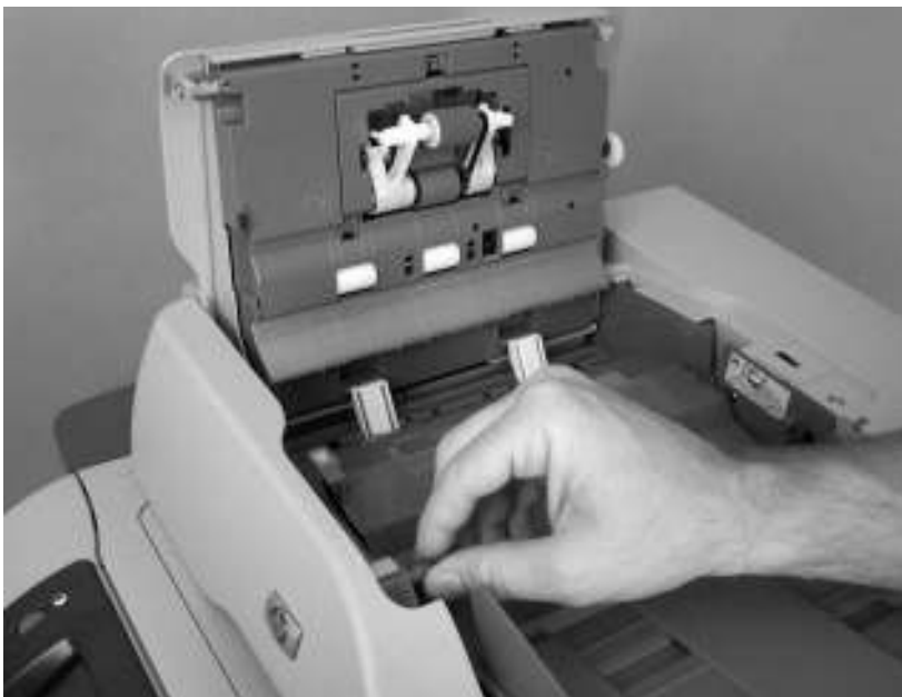
Figure 6-6 Remove the ADF input tray (2 of 3)
