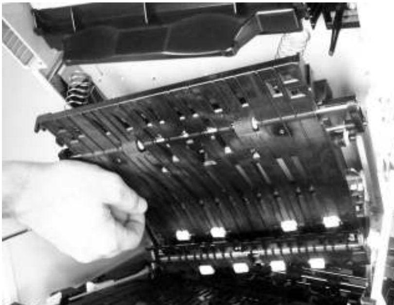
Figure 6-51 Remove the reversing-separation-guide assembly (2 of 2)
