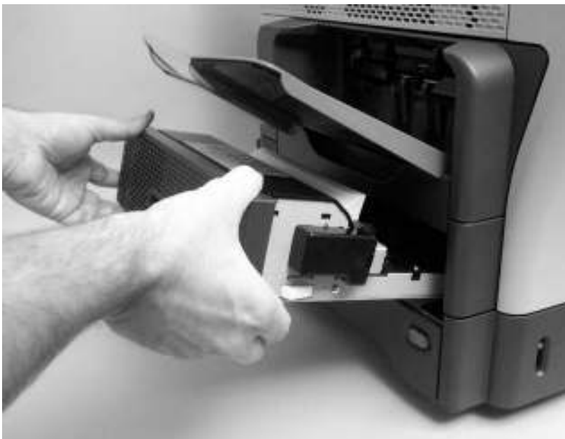
Figure 6-19 Remove the duplex-printing unit (2 of 2)
