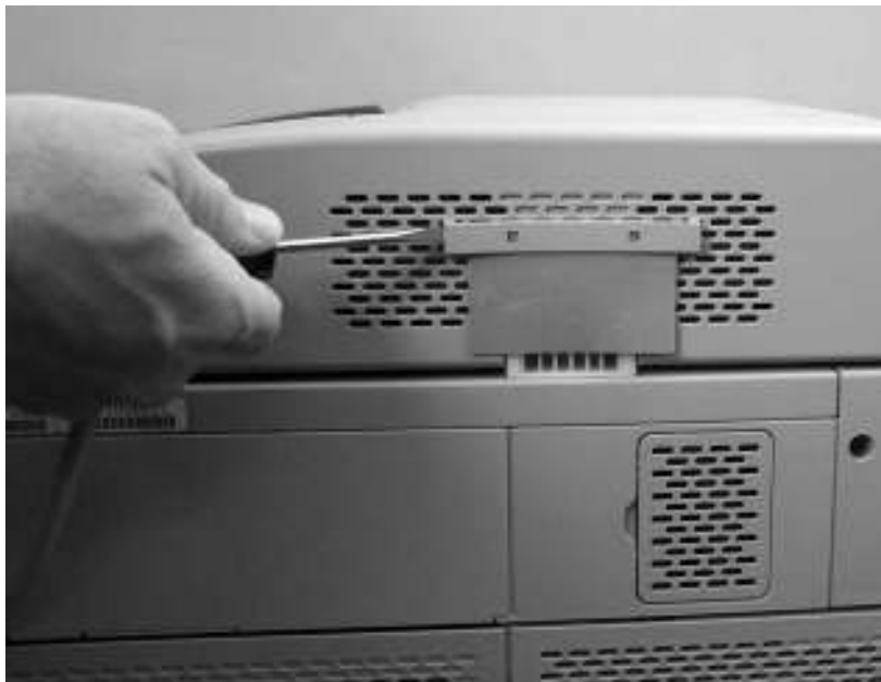
Figure 6-28 Remove the ADF-hinge flap (2 of 3)
