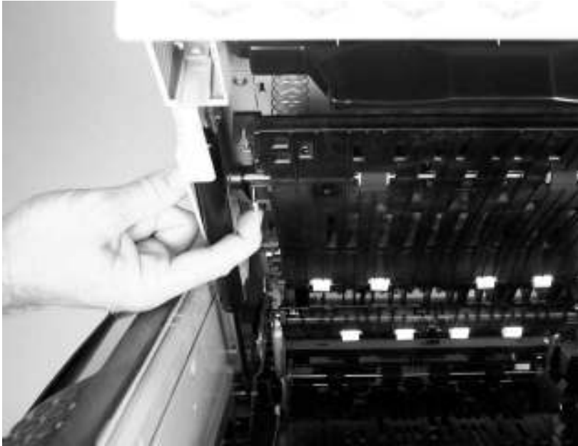
Figure 6-50 Remove the reversing-separation-guide assembly (1 of 2)
