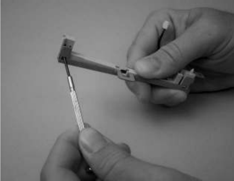
Figure 6-71 Remove the thermistor (3 of 4)
