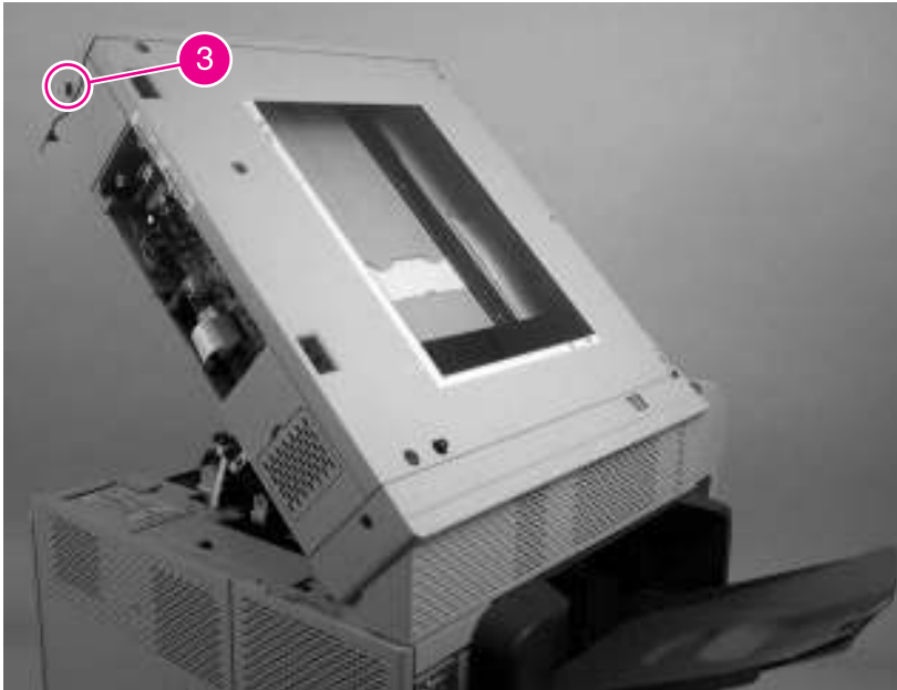
Figure 6-174 Remove the scanner assembly (3 of 8)
