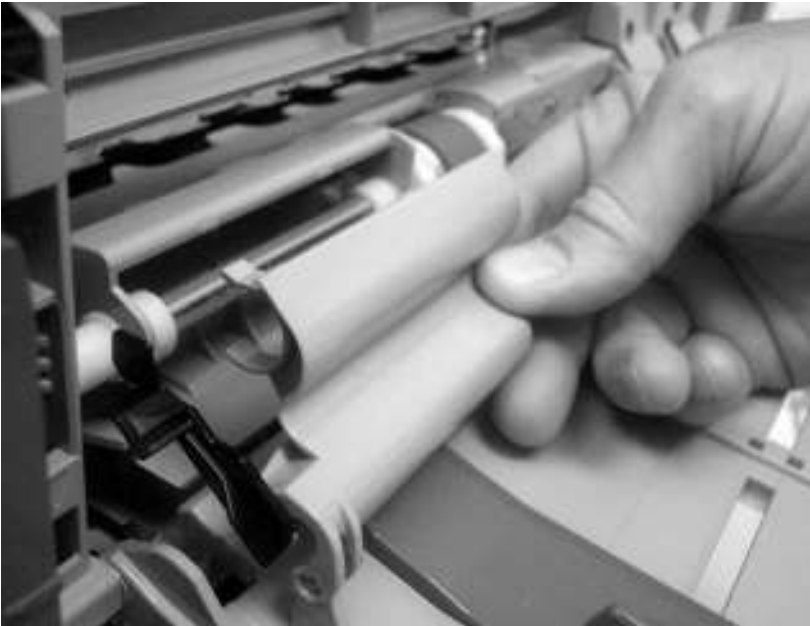
Figure 6-78 Remove the tray 1 assembly (3 of 5)
