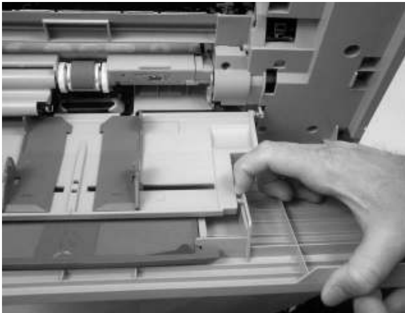
Figure 6-76 Remove the tray 1 assembly (1 of 5)
