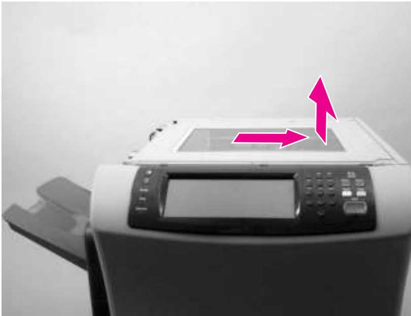
Figure 6-179 Remove the scanner assembly (8 of 8)
