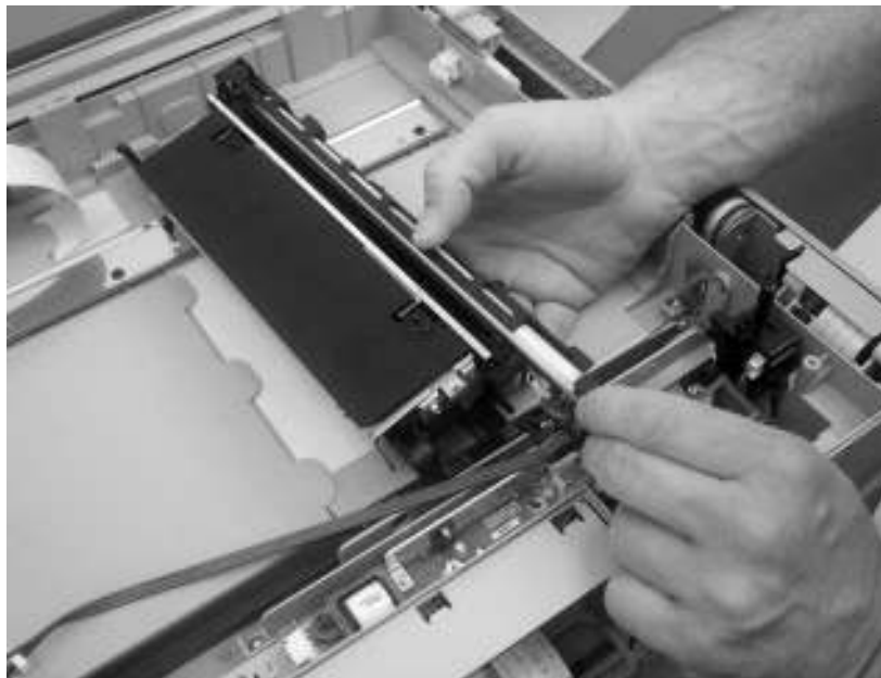
Figure 6-195 Remove the scanner bulb (2 of 2)
