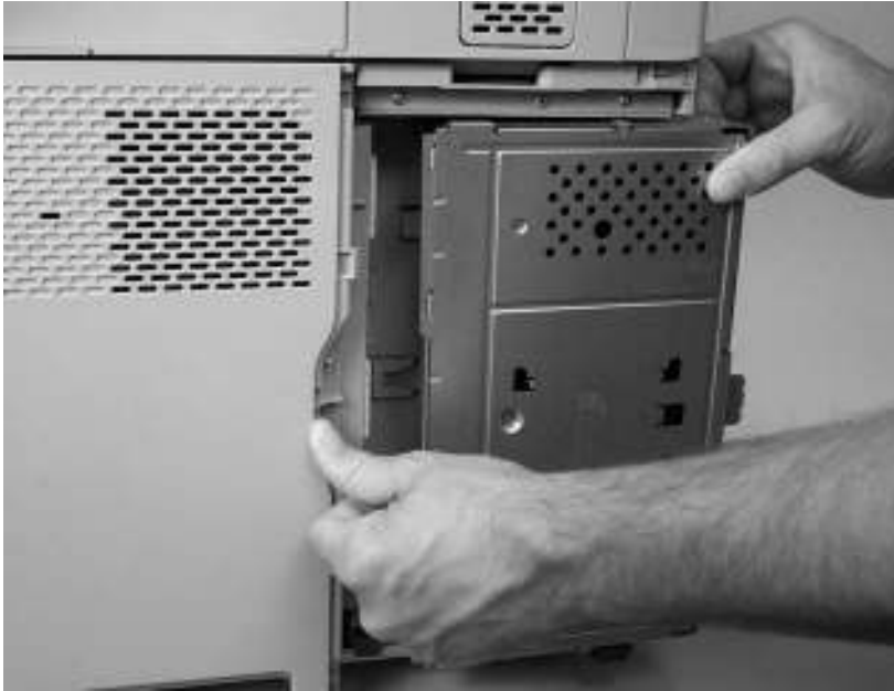
Figure 6-32 Remove the formatter cover and formatter (3 of 3)
