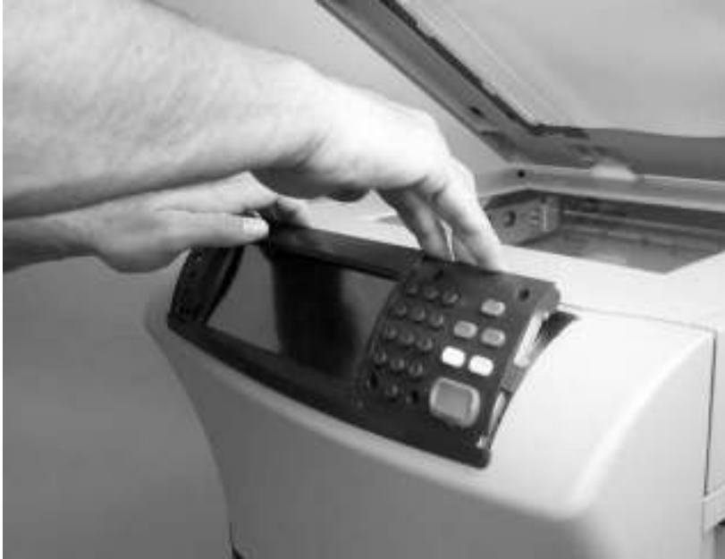
Figure 6-2 Remove the control panel (1 of 2)
