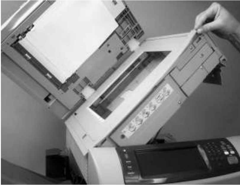
Figure 6-38 Remove the top-cover flatbed flange (1 of 2)
