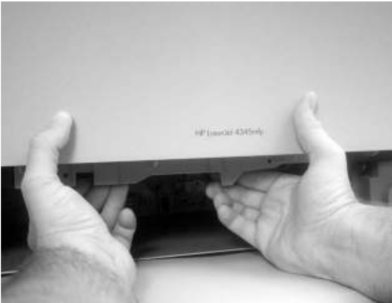
Figure 6-45 Remove the front cover (6 of 7)
