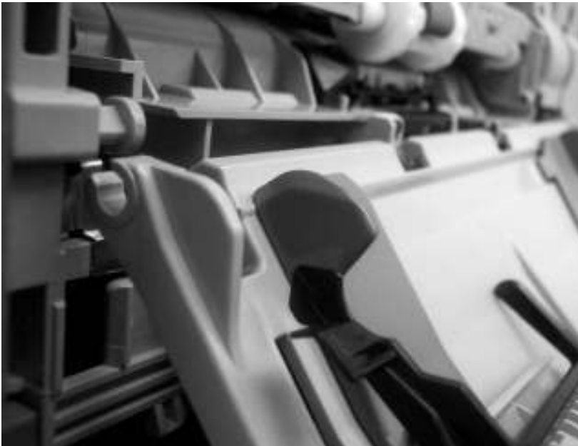
Figure 6-79 Remove the tray 1 assembly (4 of 5)
