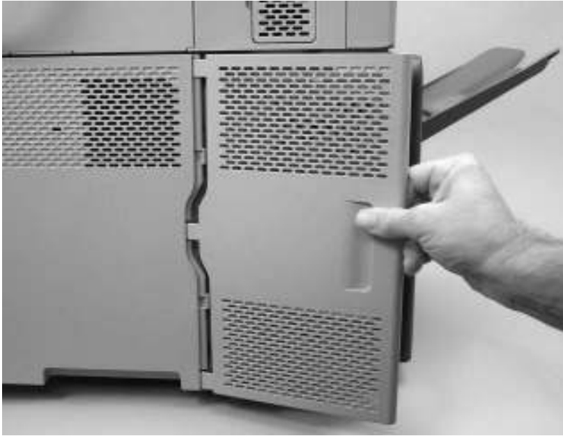
Figure 6-30 Remove the formatter cover and formatter (1 of 3)
