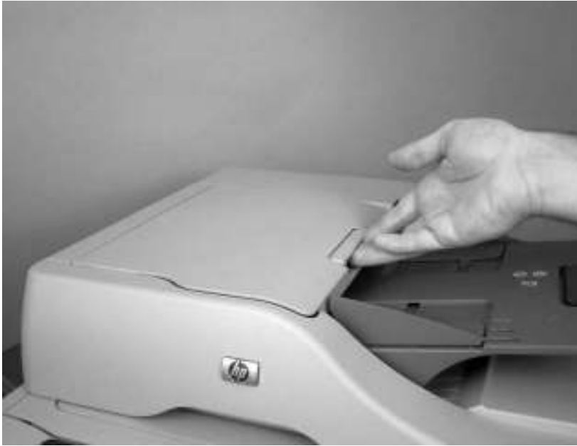
Figure 6-5 Remove the ADF input tray (1 of 3)
