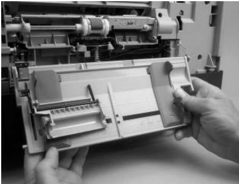
Figure 6-81 Remove the tray 1 assembly (5 of 5)
