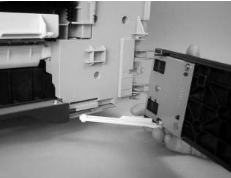
Figure 6-86 Remove the tray 1 feed-assembly (3 of 13)
