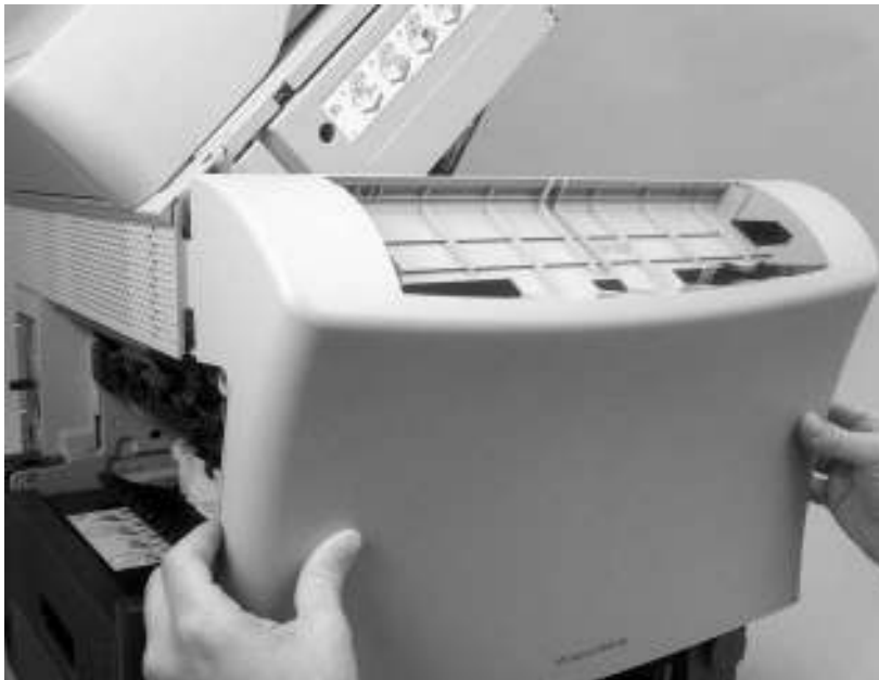
Figure 6-46 Remove the front cover (7 of 7)
