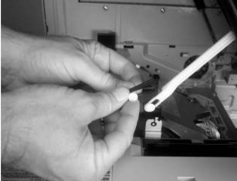
Figure 6-123 Remove the registration assembly (1 of 6)
