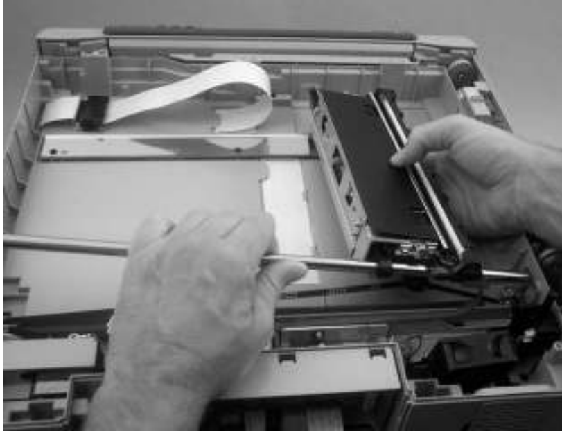
Figure 6-191 Remove the optical unit (5 of 7)
