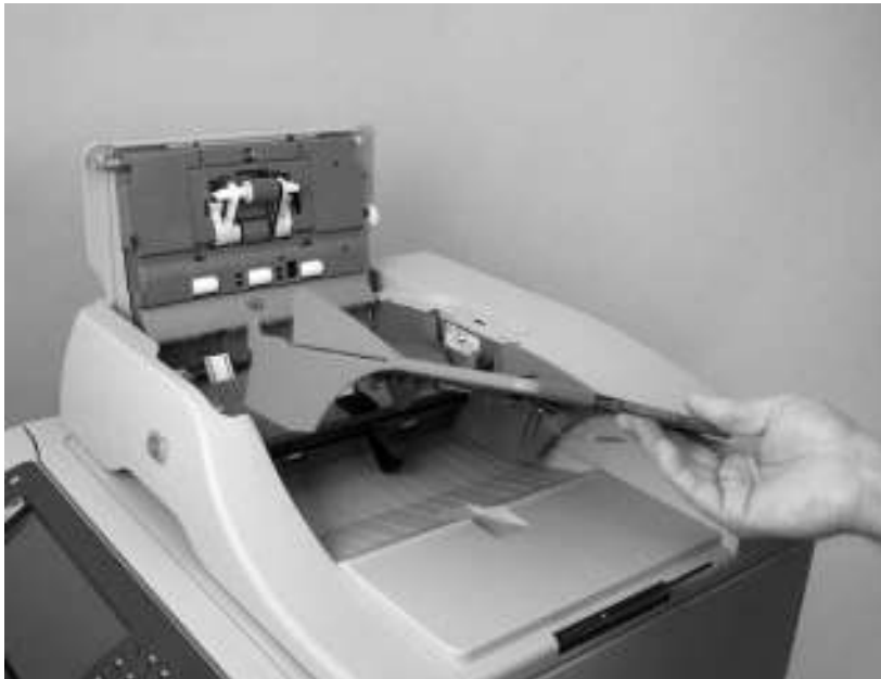
Figure 6-7 Remove the ADF input tray (3 of 3)
