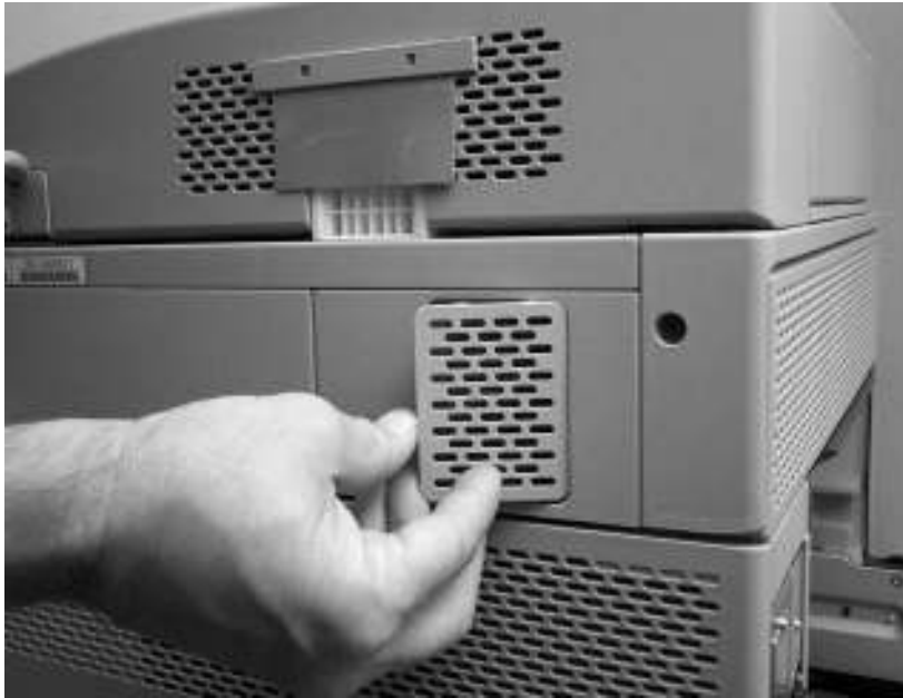
Figure 6-25 Remove the scanner filter (1 of 2)
