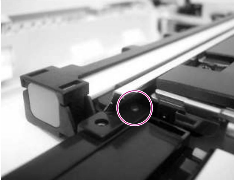
Figure 6-193 Remove the optical unit (7 of 7)
