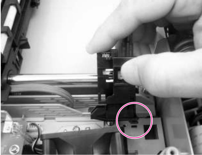
Figure 6-199 Reinstalling the scanner home-position sensor
