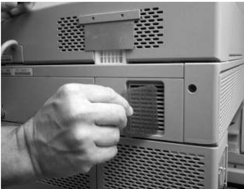
Figure 6-26 Remove the scanner filter (2 of 2)
