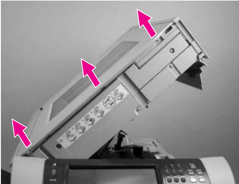
Figure 6-172 Remove the scanner assembly (1 of 8)
