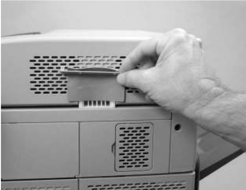
Figure 6-29 Remove the ADF-hinge flap (3 of 3)
