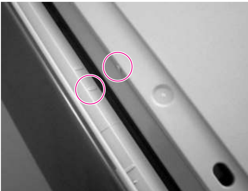
Figure 6-180 Correctly positioning the scanner assembly
