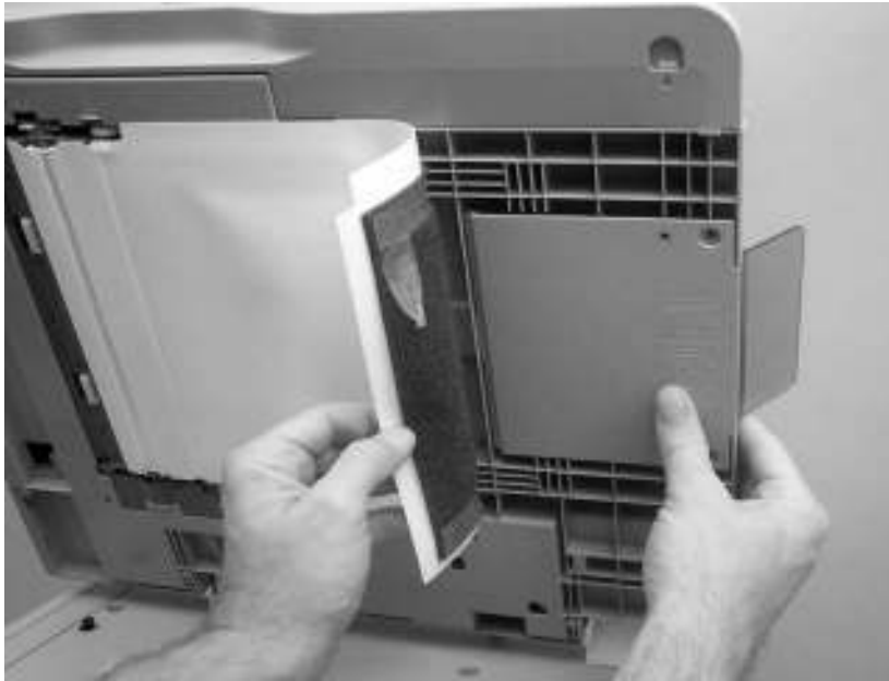
Figure 6-203 Remove the ADF output-bin extension (2 of 2)
