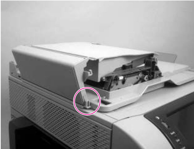
Figure 6-213 Remove the ADF left cover (2 of 2)
