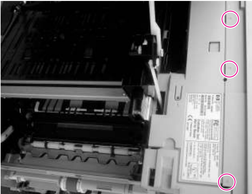
Figure 6-48 Remove the back cover (2 of 3)
