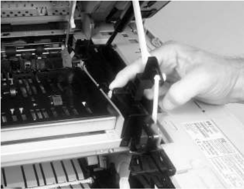
Figure 6-53 Remove the reversing assembly (2 of 8)
