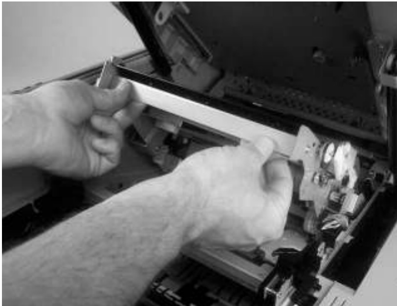
Figure 6-59 Remove the reversing assembly (8 of 8)
