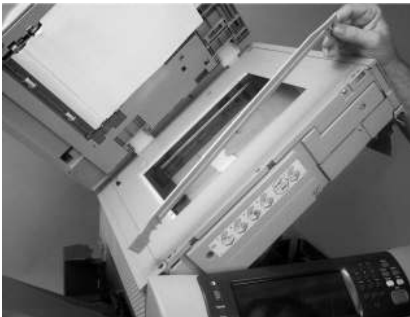
Figure 6-39 Remove the top-cover flatbed flange (2 of 2)
