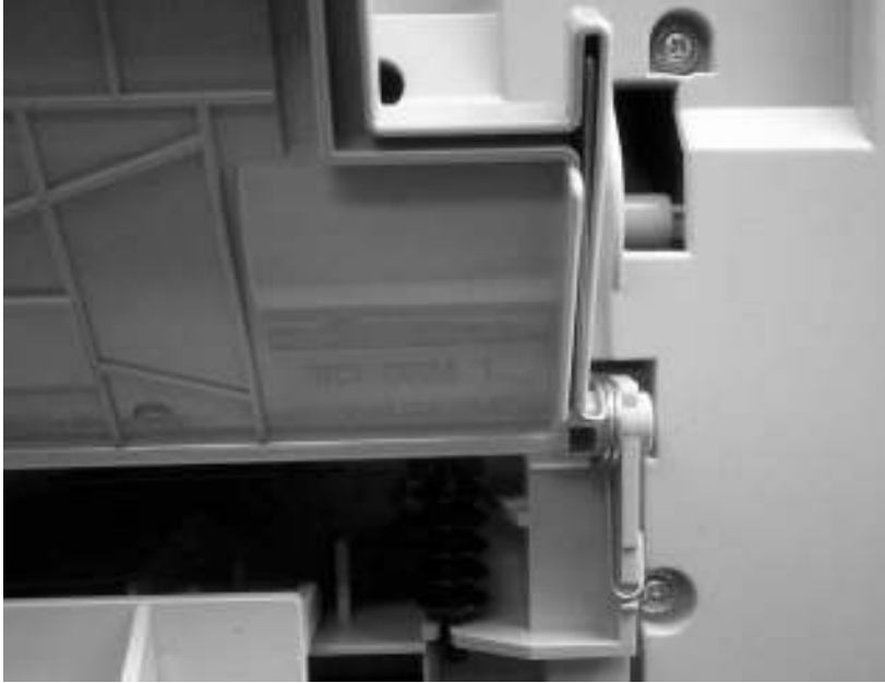
Figure 6-80 Correct tray 1 rear-hinge-spring placement
