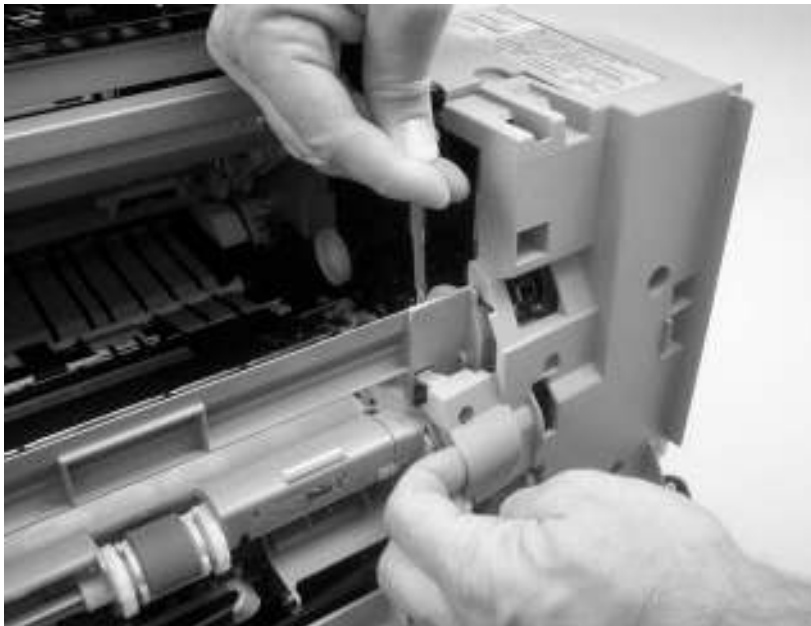
Figure 6-88 Remove the tray 1 feed-assembly (5 of 13)
