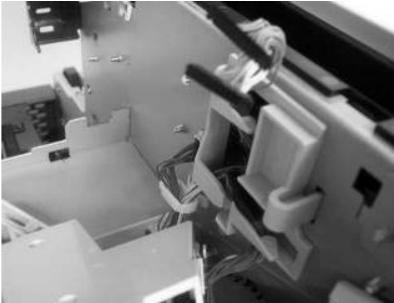
Figure 6-165 Remove the laser/scanner (1 of 2)
