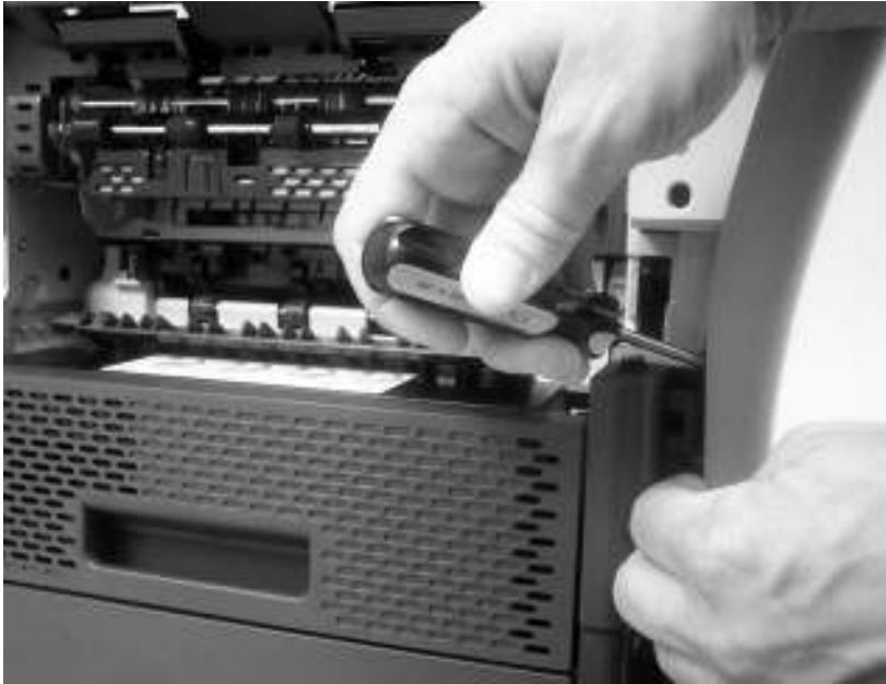
Figure 6-43 Remove the front cover (4 of 7)
