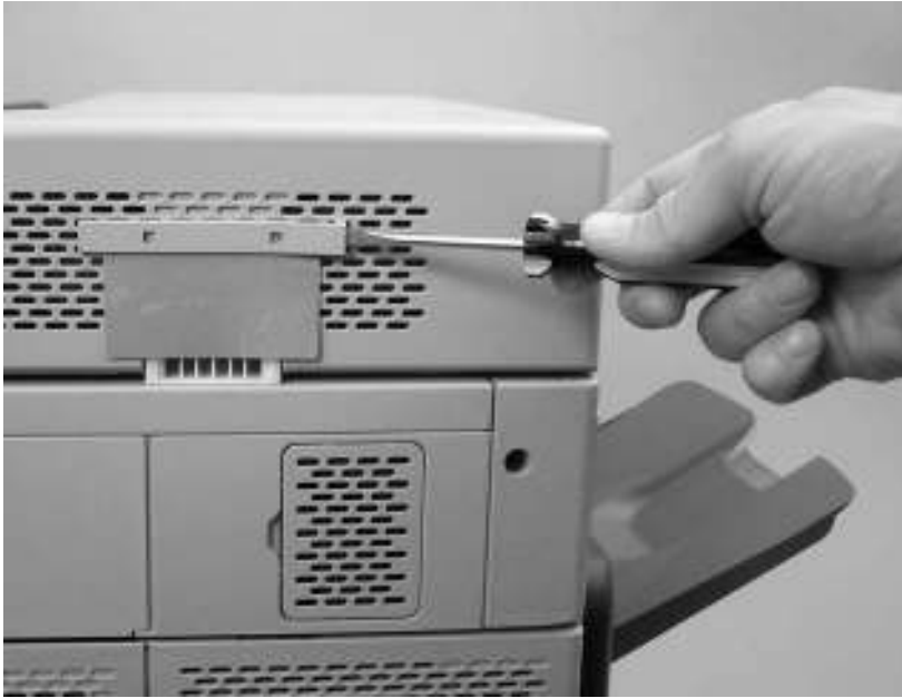
Figure 6-27 Remove the ADF-hinge flap (1 of 3)
