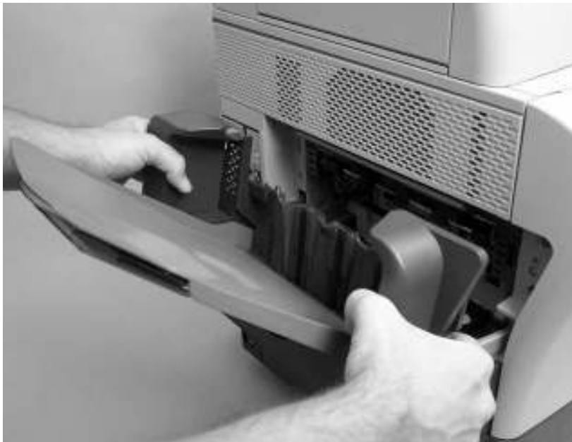
Figure 6-17 Remove the output-bin assembly (2 of 2)
