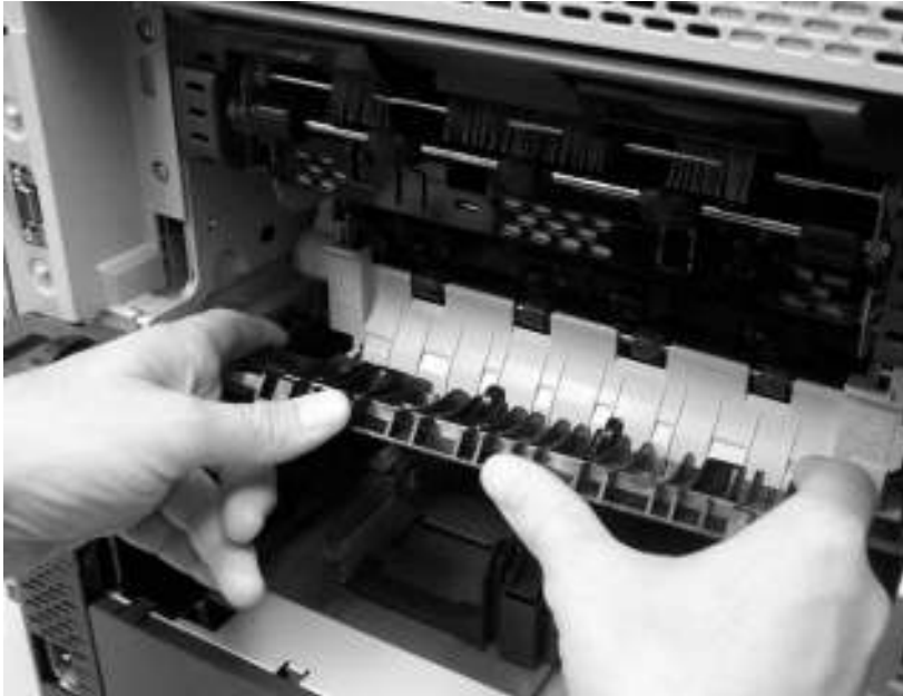
Figure 6-20 Remove the fuser-entrance guide
