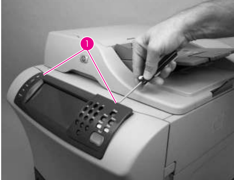
Figure 6-1 Remove the control-panel overlays
