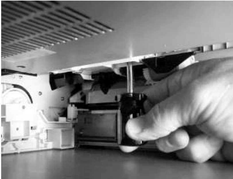
Figure 6-163 Remove the tray 2 paper-present sensor
