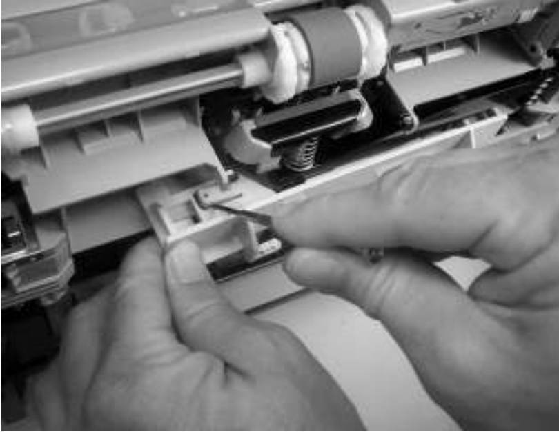
Figure 6-82 Remove the front-cover support (1 of 2)
