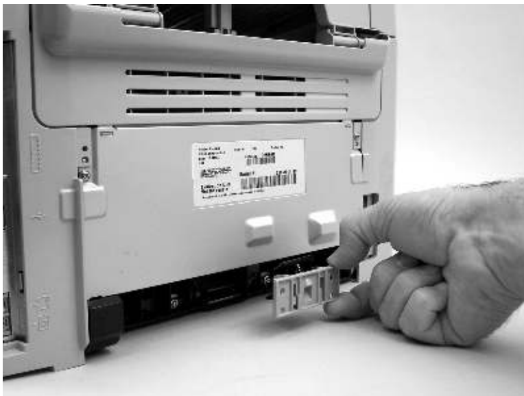
Figure 6-20 Remove the device separation pad (2 of 2)
