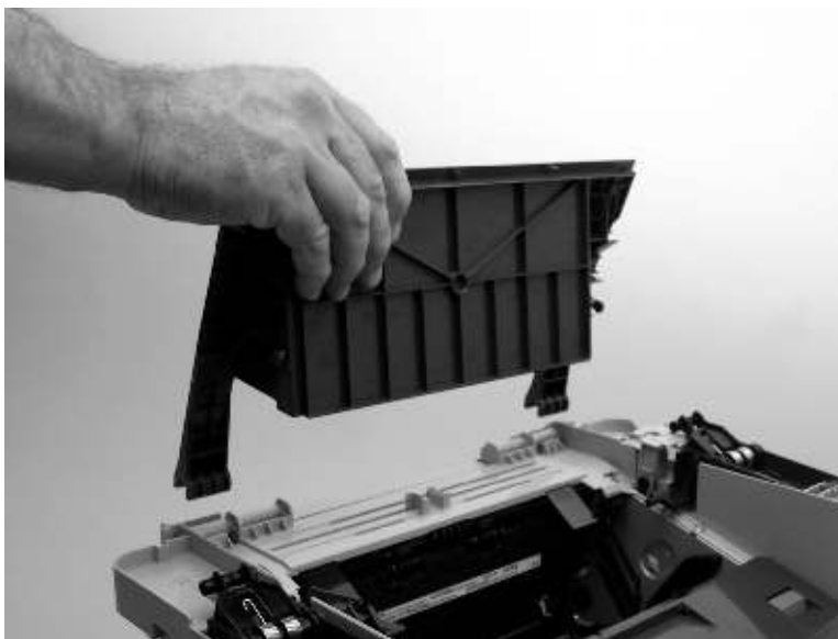
Figure 6-39 Remove the print-cartridge door (2 of 2)
