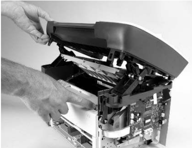
Figure 6-12 Remove the scanner assembly (5 of 11)
