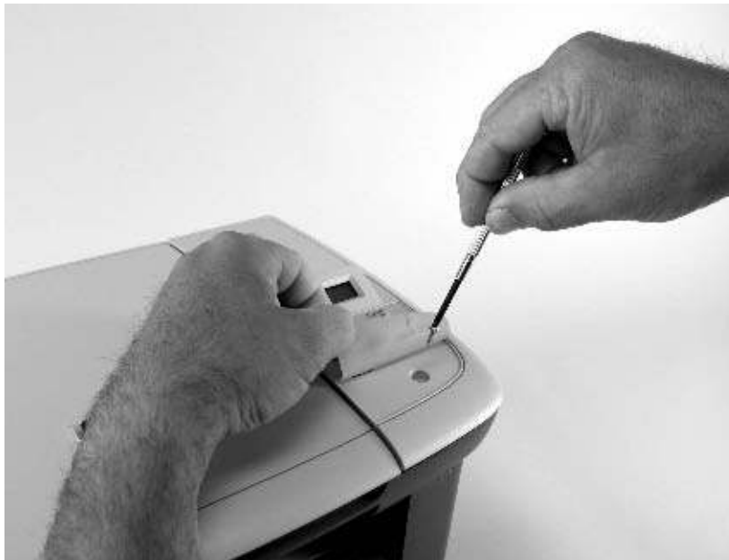
Figure 6-5 Remove the control panel (2 of 4)
