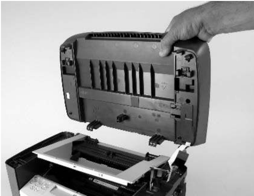
Figure 6-18 Remove the scanner assembly (11 of 11)
