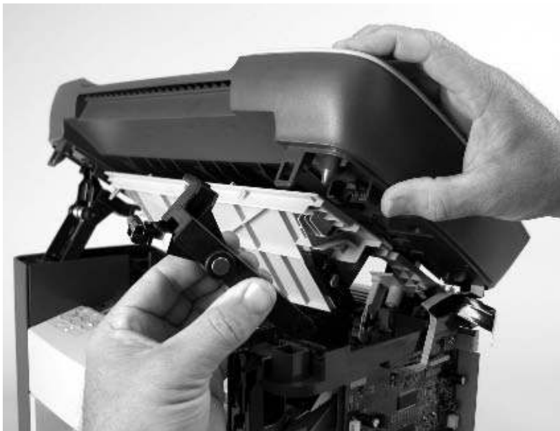
Figure 6-17 Remove the scanner assembly (10 of 11)
