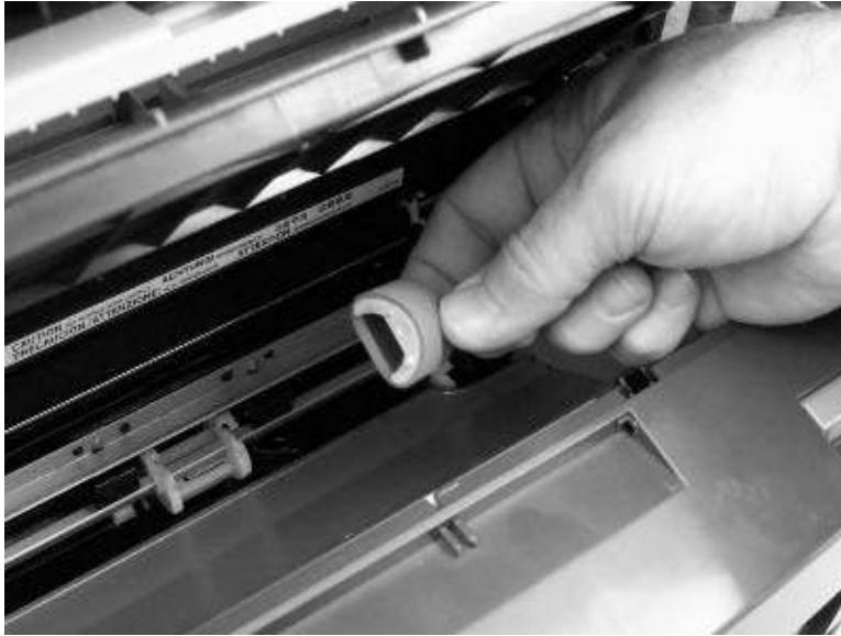
Figure 6-25 Remove the device pickup roller (3 of 5)
