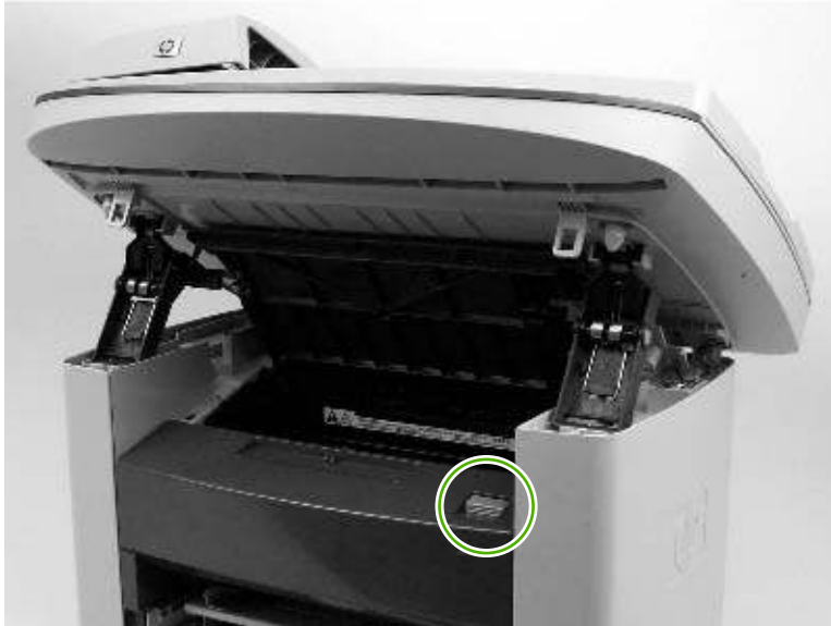
Figure 6-21 Remove the print cartridge (1 of 2)
