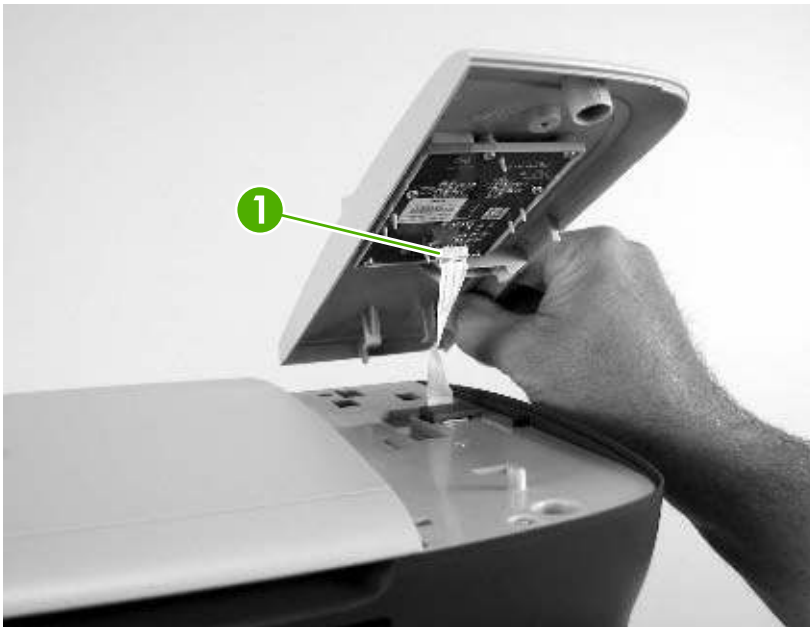
Figure 6-7 Remove the control panel (4 of 4)
