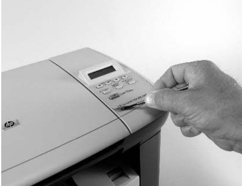
Figure 6-3 Remove the control-panel overlay
