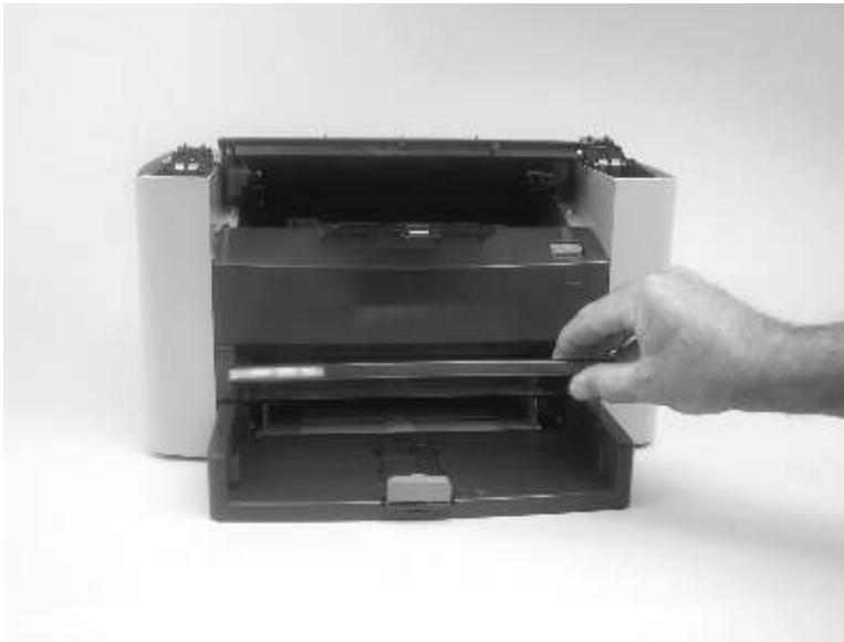
Figure 6-28 Remove the media input tray (1 of 3)
