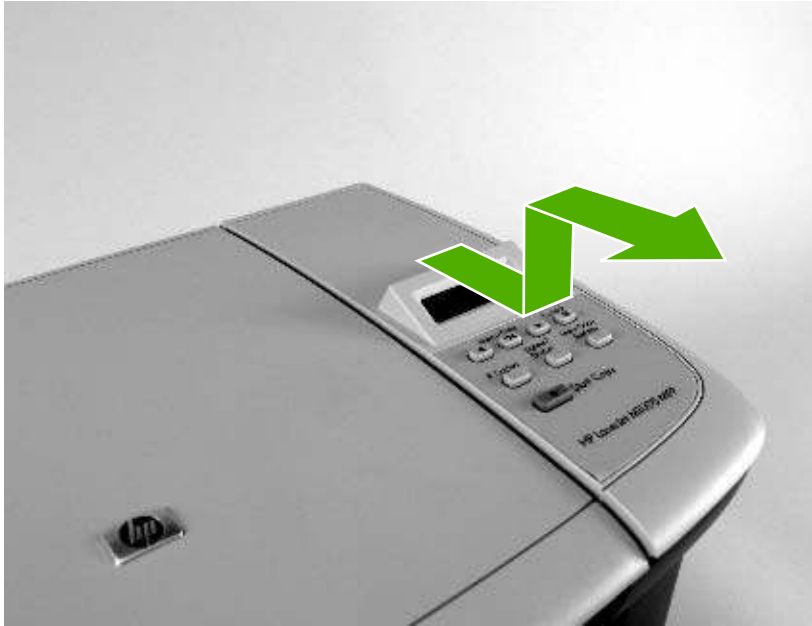
Figure 6-6 Remove the control panel (3 of 4)
