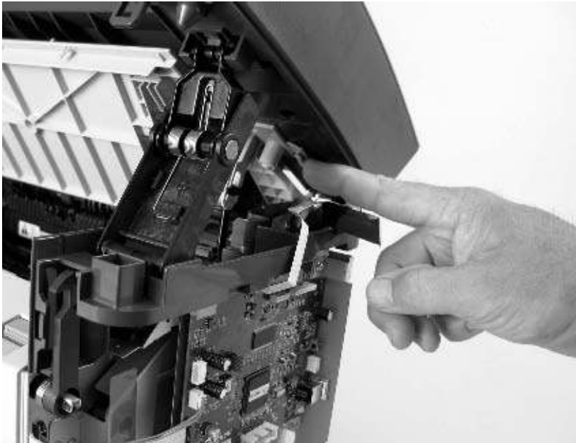
Figure 6-14 Remove the scanner assembly (7 of 11)
