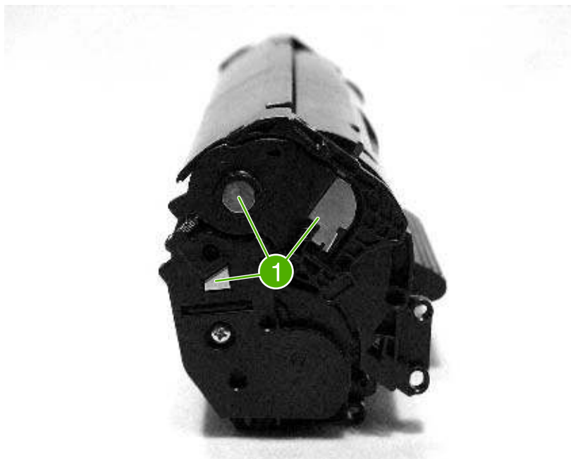
Figure 7-7 Print-cartridge high-voltage contacts
