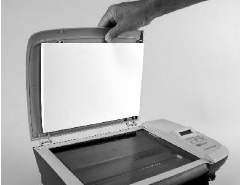
Figure 6-2 Remove the flatbed lid (1 of 2)
