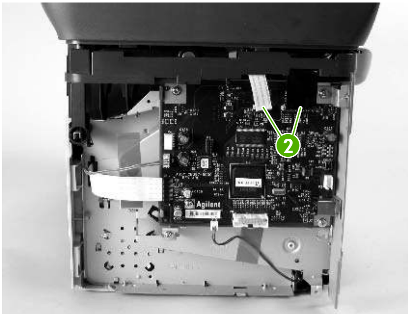
Figure 6-11 Remove the scanner assembly (4 of 11)
