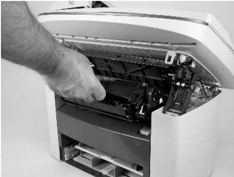
Figure 6-22 Remove the print cartridge (2 of 2)
