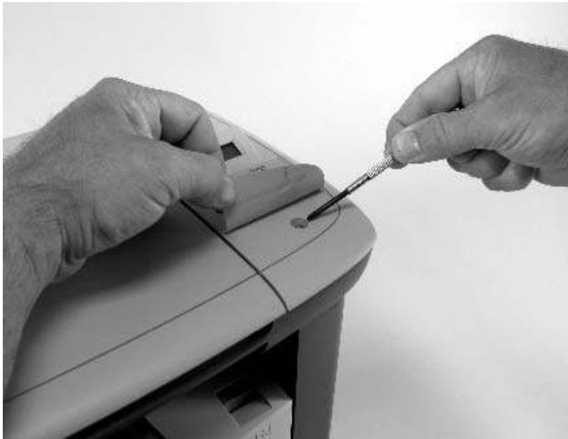
Figure 6-4 Remove the control panel (1 of 4)
