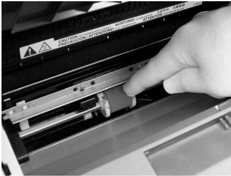
Figure 6-27 Remove the device pickup roller (5 of 5)
