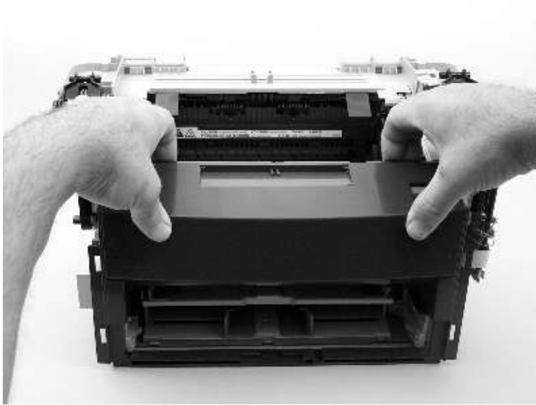
Figure 6-45 Remove the front cover (3 of 3)
