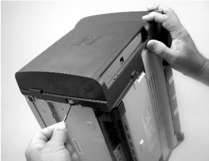
Figure 6-10 Remove the scanner assembly (3 of 11)
