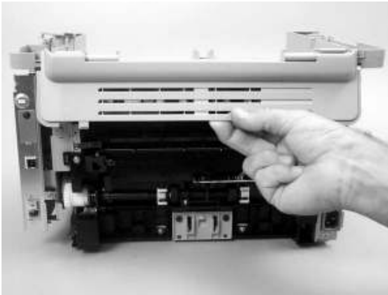
Figure 5-45 Remove the rear cover and fuser cover (3 of 3)
