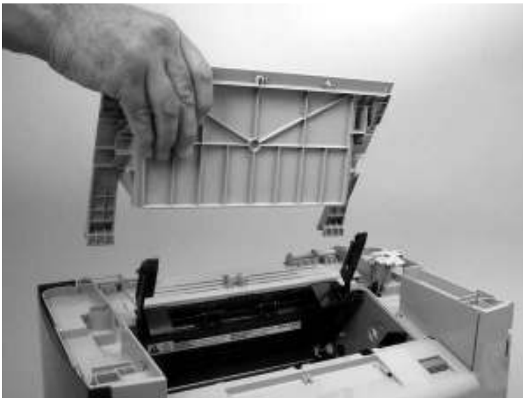
Figure 5-42 Remove the print-cartridge door (2 of 2)
