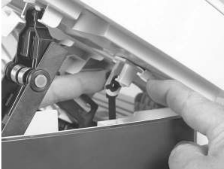
Figure 5-19 Remove the scanner assembly (7 of 10)
