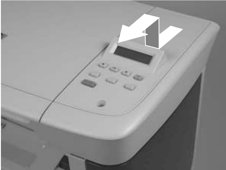
Figure 5-11 Remove the control-panel assembly (2 of 3)
