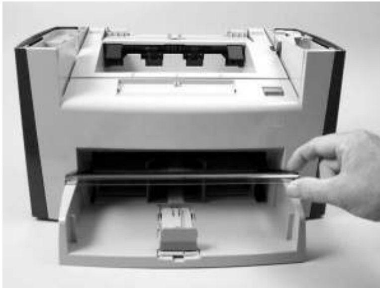
Figure 5-33 Remove the media input tray (1 of 3)
