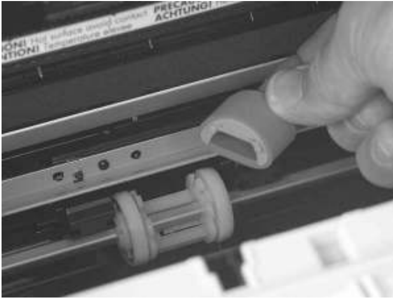
Figure 5-29 Remove the pickup roller (3 of 5)
