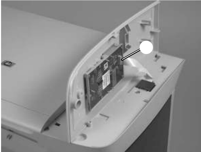
Figure 5-12 Remove the control-panel assembly (3 of 3)
