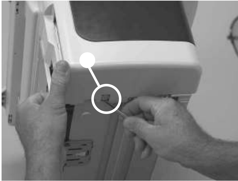
Figure 5-15 Remove the scanner assembly (3 of 10)
