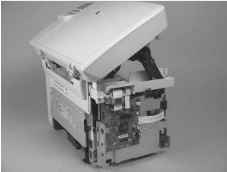
Figure 5-17 Remove the scanner assembly (5 of 10)
