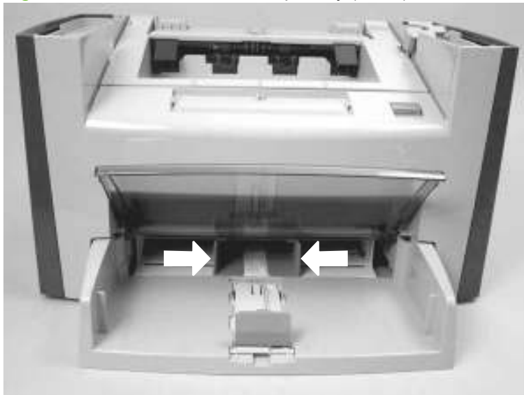
Figure 5-34 Remove the media input tray (2 of 3)
