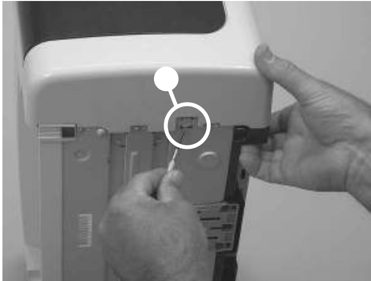
Figure 5-39 Remove the side covers (3 of 4)
