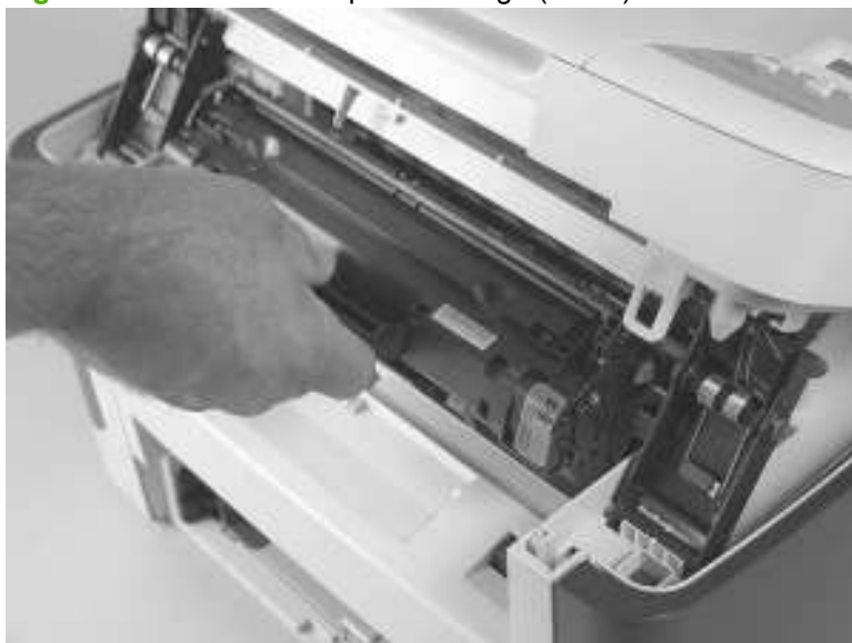
Figure 5-24 Remove the print cartridge (2 of 2)
