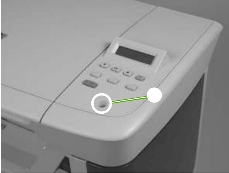
Figure 5-10 Remove the control-panel assembly (1 of 3)
