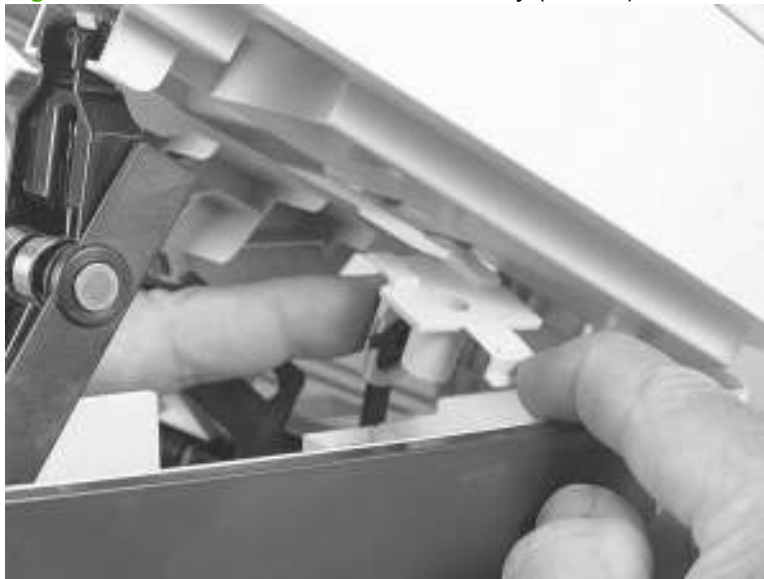
Figure 5-20 Remove the scanner assembly (8 of 10)
