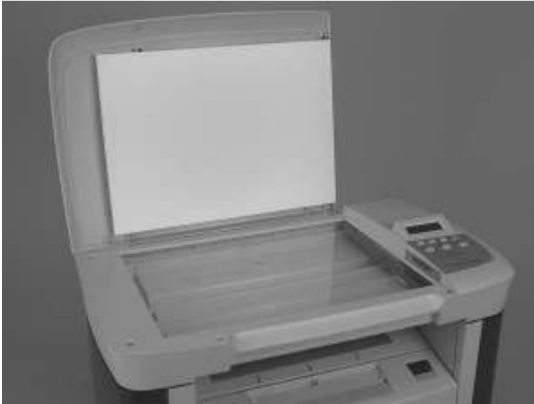
Figure 5-7 Remove the scanner lid (1 of 2)
