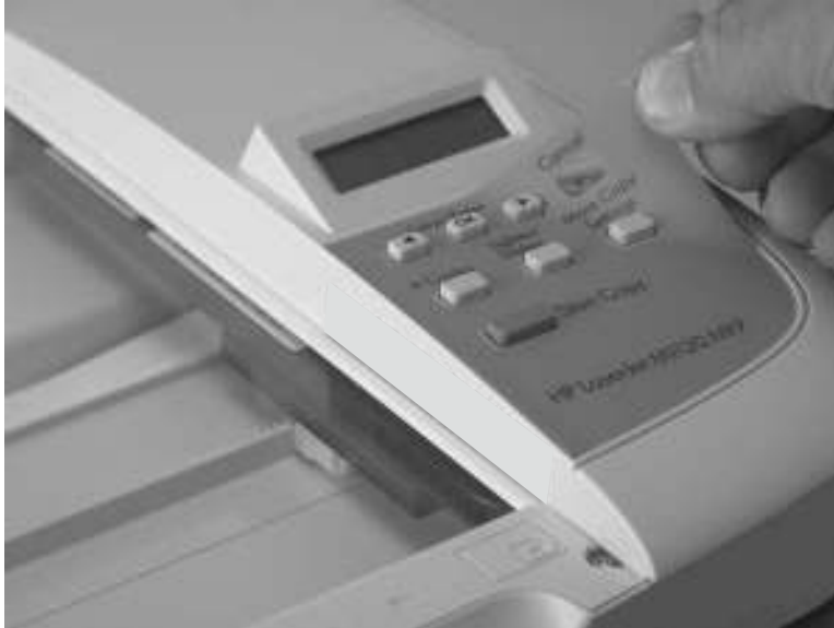
Figure 5-9 Remove the control-panel overlay
