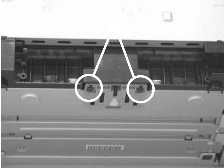
Figure 5-25 Remove the separation pad (1 of 2)
