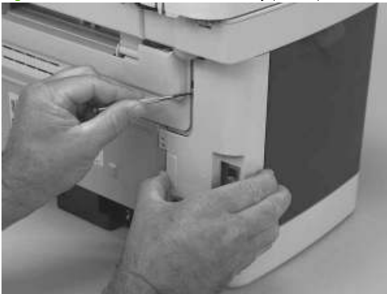
Figure 5-14 Remove the scanner assembly (2 of 10)
