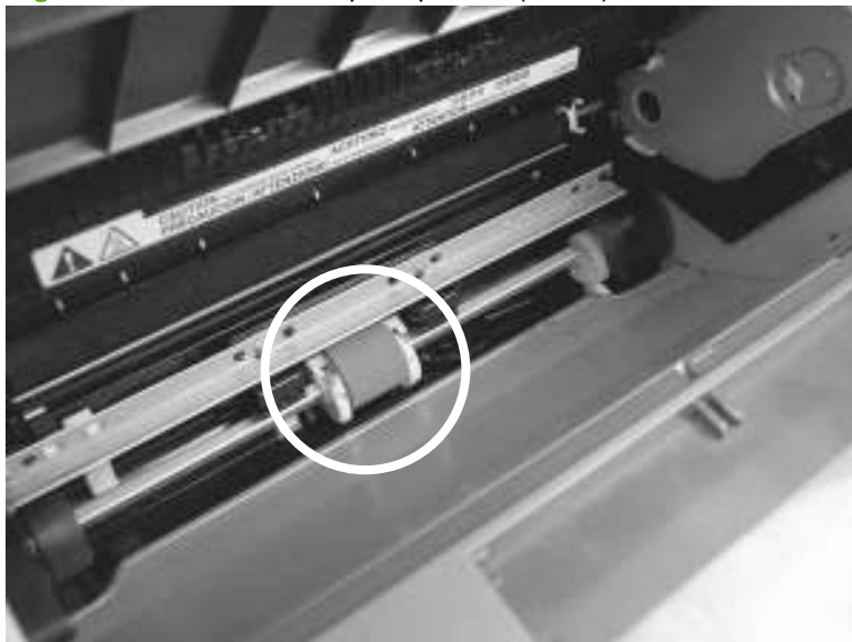
Figure 5-27 Remove the pickup roller (1 of 5)
