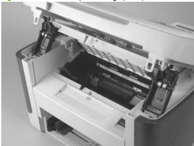
Figure 5-23 Remove the print cartridge (1 of 2)
