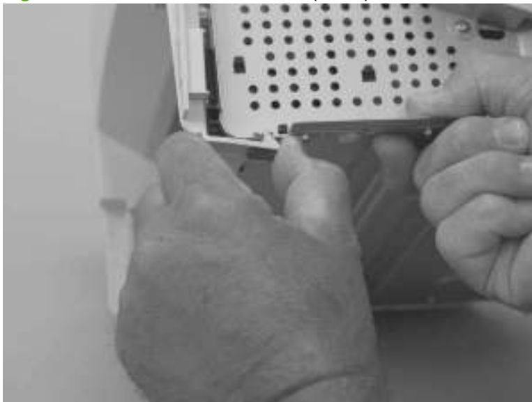
Figure 5-47 Remove the front cover (2 of 4)
