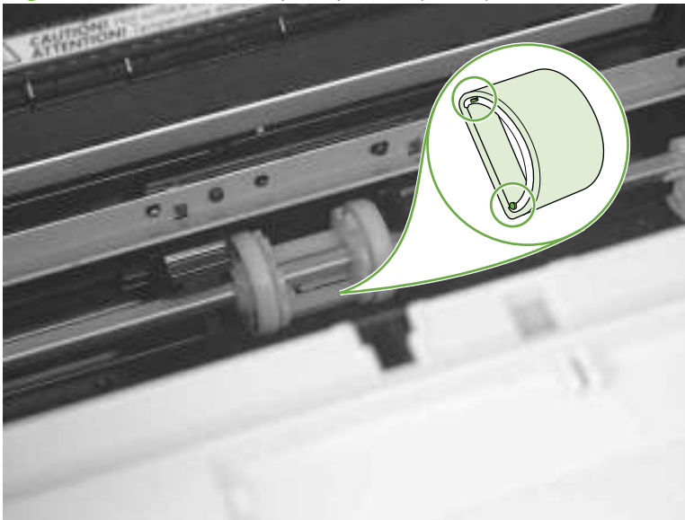
Figure 5-30 Remove the pickup roller (4 of 5)
