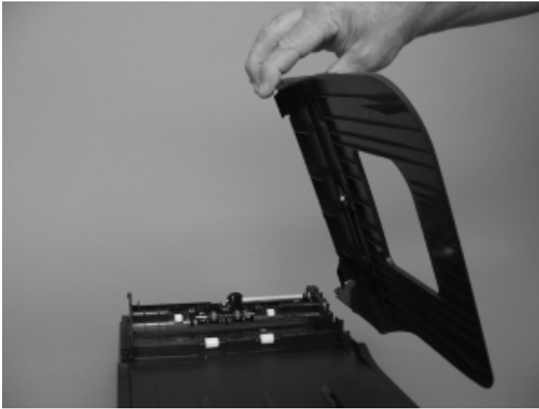
Figure 1-73 Remove the ADF tray (4 of 4)
