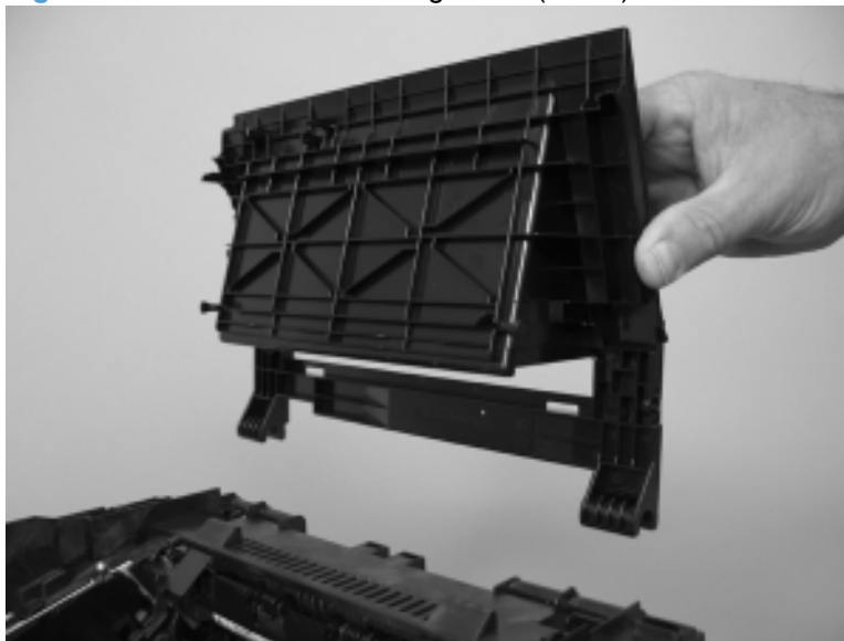
Figure 1-51 Remove the cartridge door (5 of 5)
