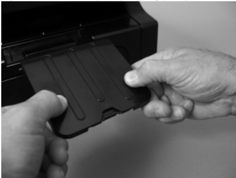
Figure 1-26 Remove the paper-pickup tray (2 of 2)
