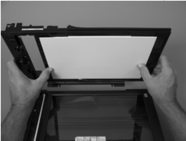
Figure 1-76 Remove the ADF base or scanner assembly lid (3 of 3)
