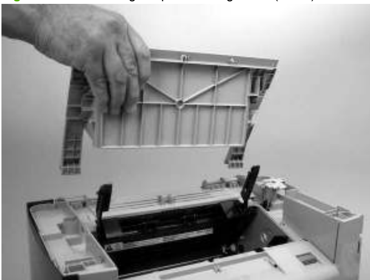
Figure 6-66 Removing the print-cartridge door (2 of 2)
