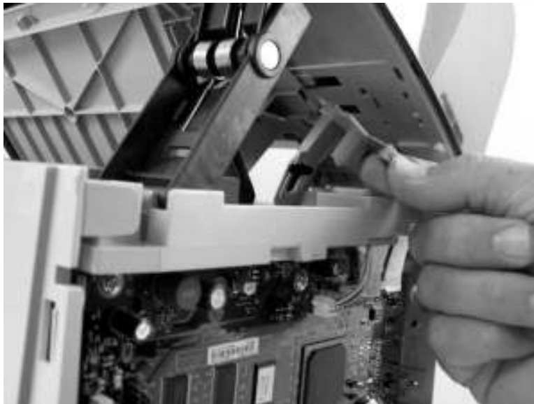
Figure 6-29 Removing the scanner assembly (10 of 14)
