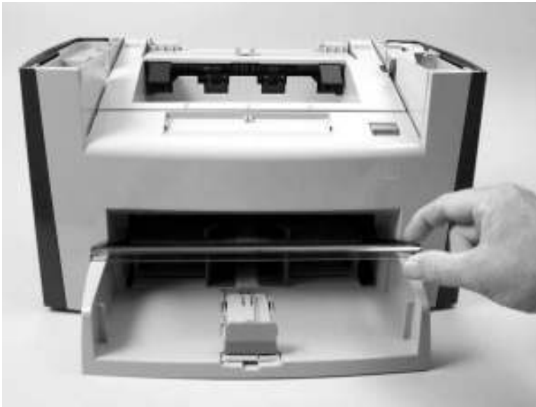
Figure 6-55 Removing the media input tray (1 of 3)
