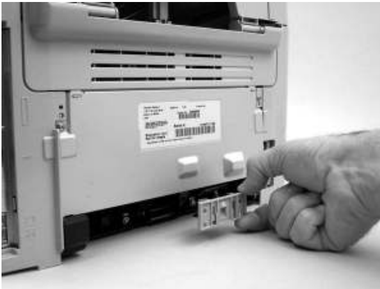
Figure 6-46 Removing the separation pad (2 of 2)
