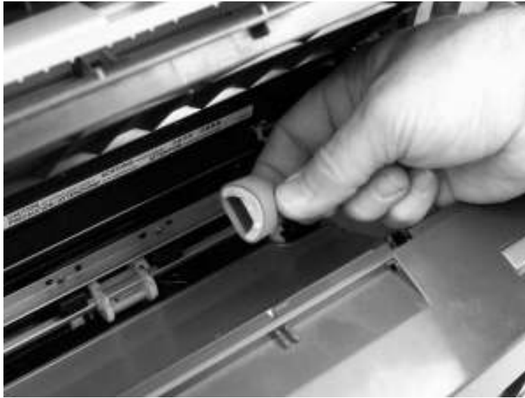
Figure 6-51 Removing the pickup roller (3 of 5)
