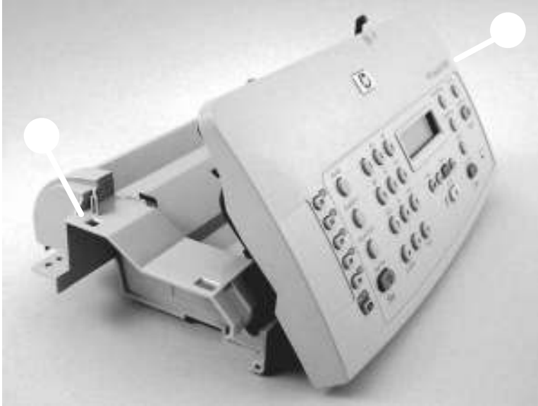
Figure 6-38 Removing the top-cover assembly (1 of 2)
