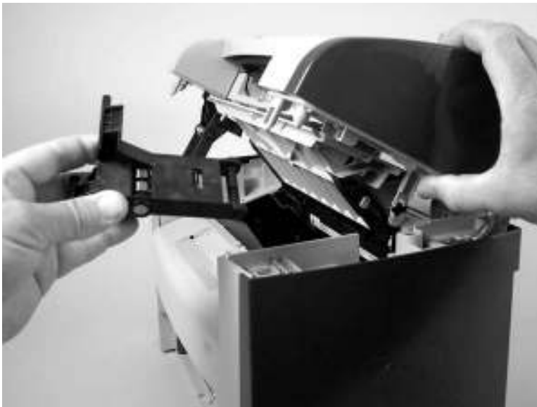
Figure 6-6 Removing the link assemblies and scanner support-frame spring (3 of 4)
