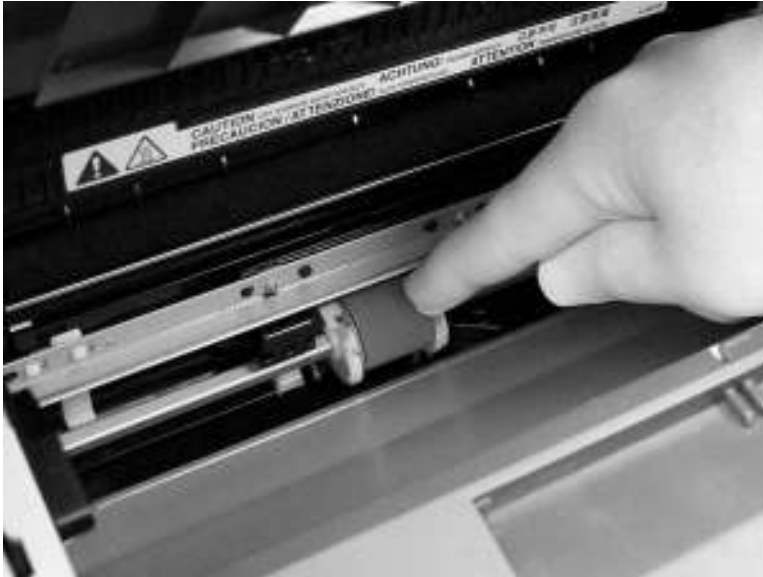
Figure 6-53 Removing the pickup roller (5 of 5)
