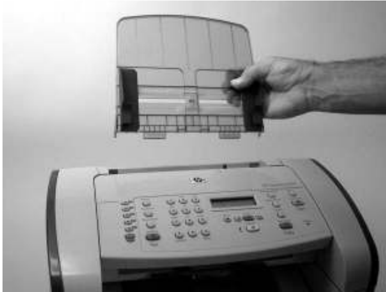
Figure 6-20 Removing the scanner assembly (1 of 14)
