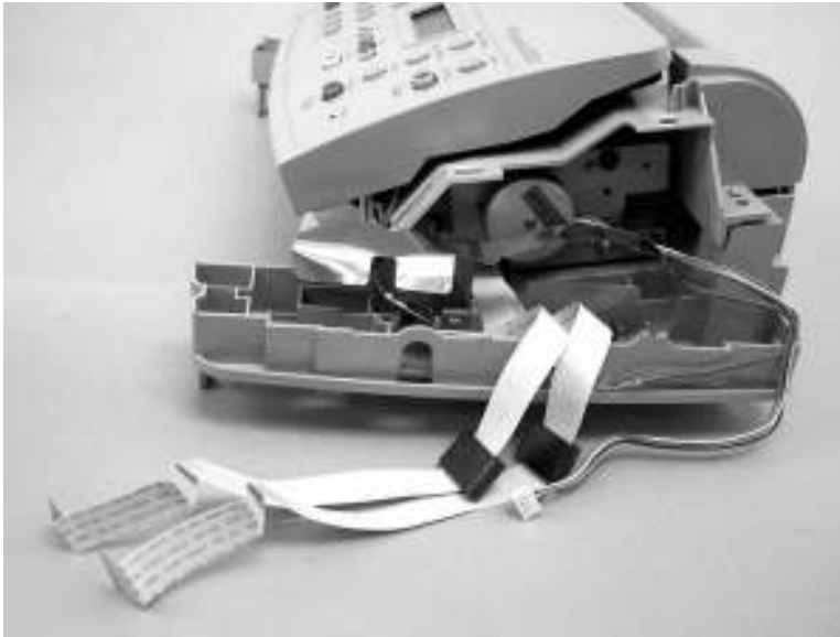
Figure 6-35 Removing the scanner assembly top cover (2 of 4)
