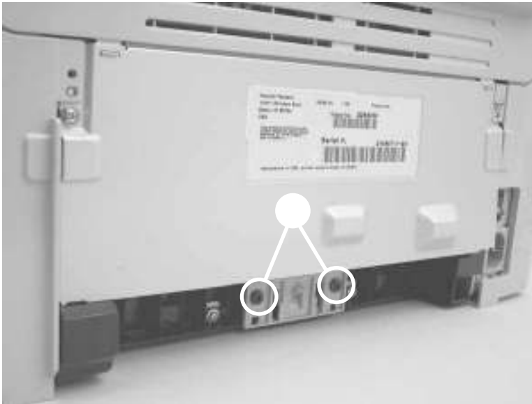
Figure 6-45 Removing the separation pad (1 of 2)
