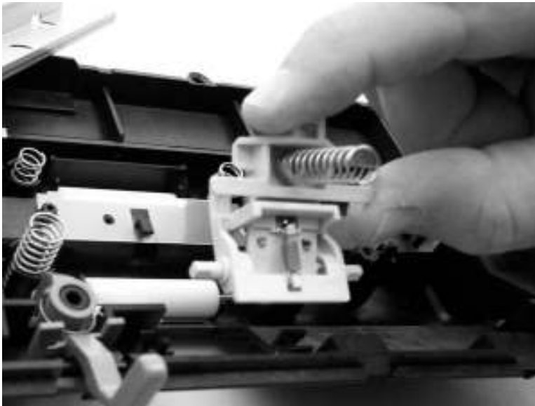
Figure 6-19 Removing the separation-pad assembly (3 of 3)
