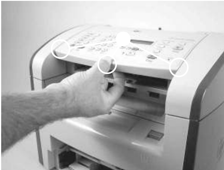
Figure 6-11 Removing the top cover, control panel (1 of 3)
