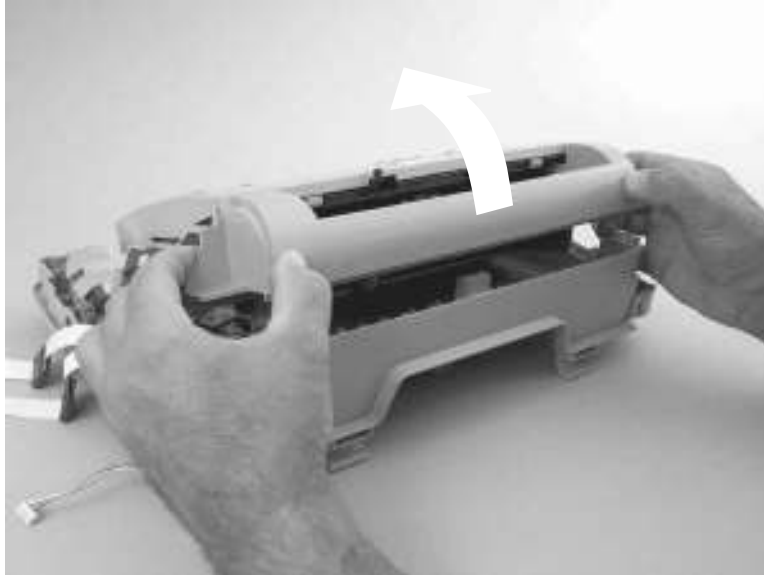
Figure 6-37 Removing the scanner assembly top cover (4 of 4)
