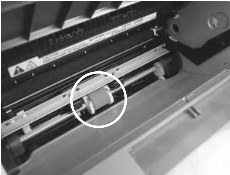
Figure 6-49 Removing the pickup roller (1 of 5)
