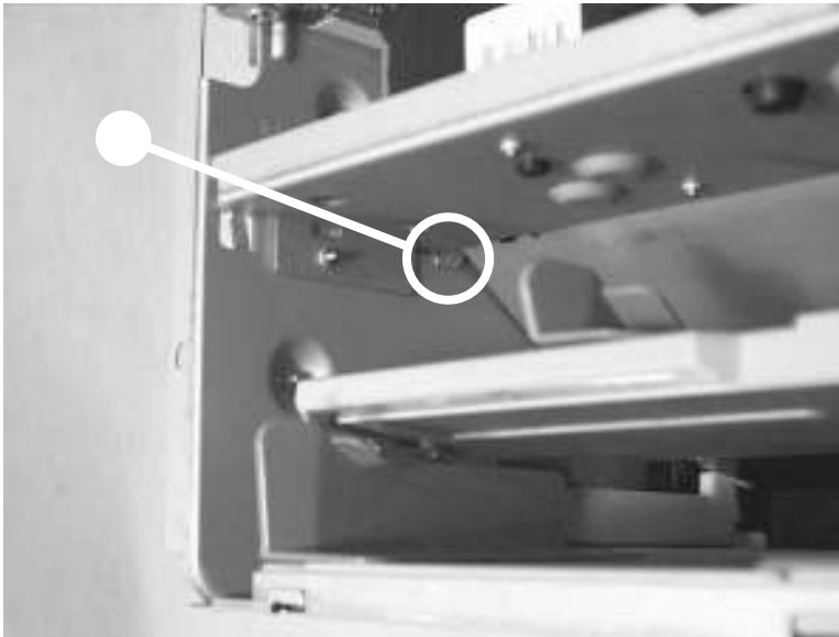
Figure 6-91 Removing the ECU (2 of 6)
