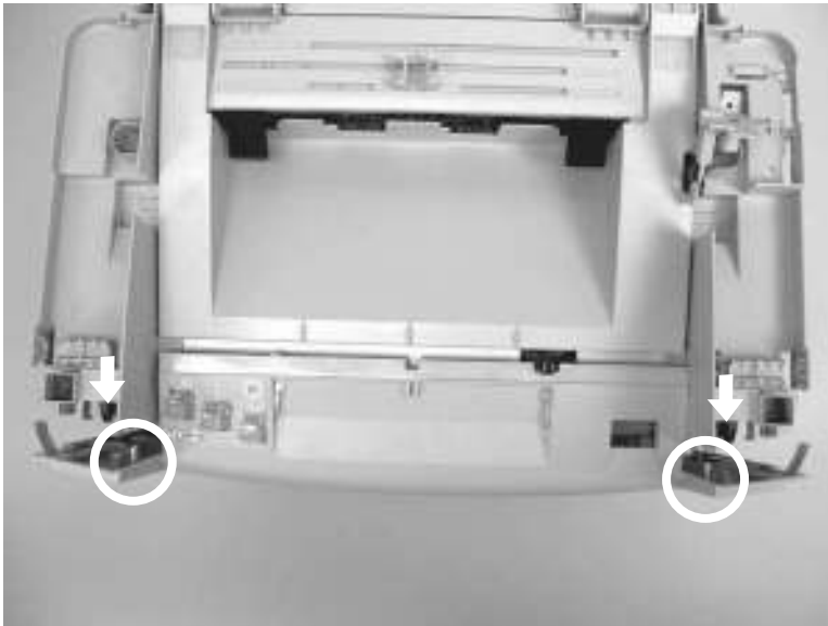
Figure 6-73 Removing the front cover (4 of 5)
