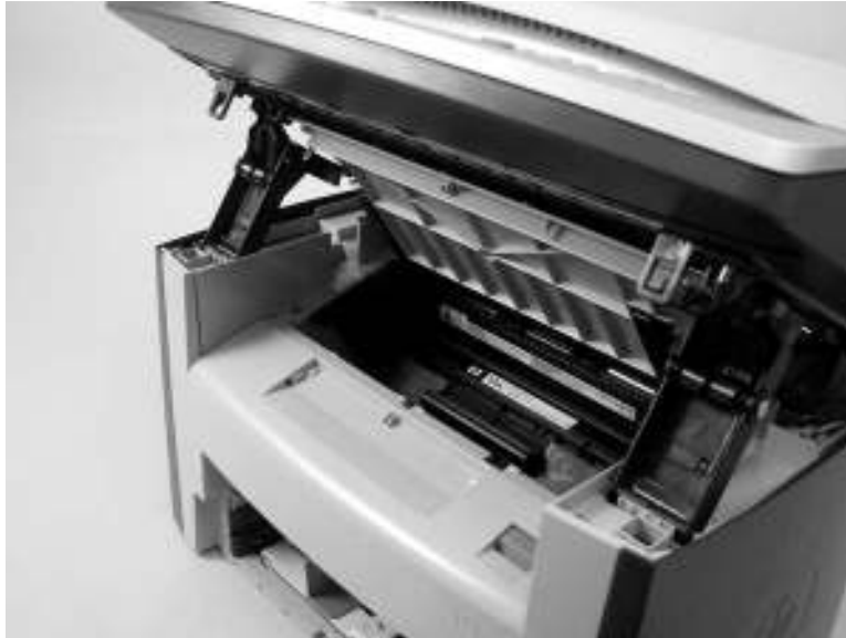
Figure 6-47 Removing the print cartridge (1 of 2)
