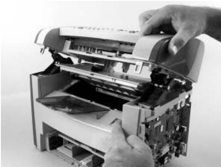
Figure 6-27 Removing the scanner assembly (8 of 14)
