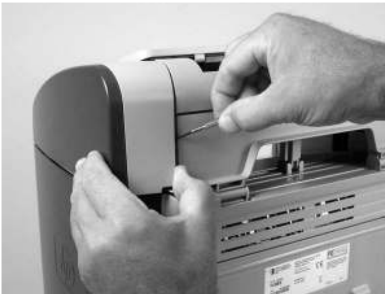
Figure 6-8 Removing the scanner side covers (1 of 2)
