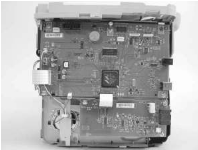
Figure 6-83 Removing the formatter (2 of 4)
