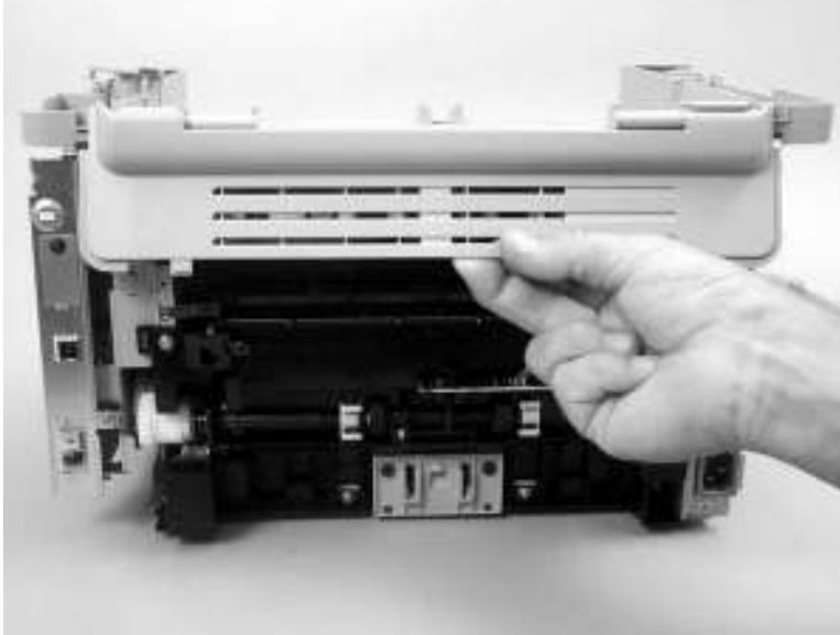
Figure 6-69 Removing the rear cover and fuser cover (3 of 3)
