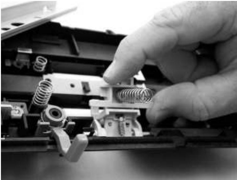
Figure 6-18 Removing the separation-pad assembly (2 of 3)
