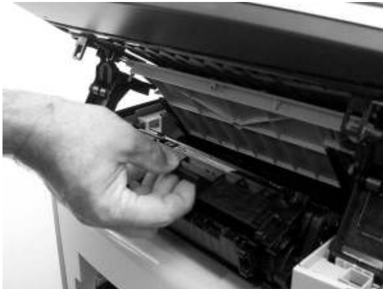
Figure 6-48 Removing the print cartridge (2 of 2)
