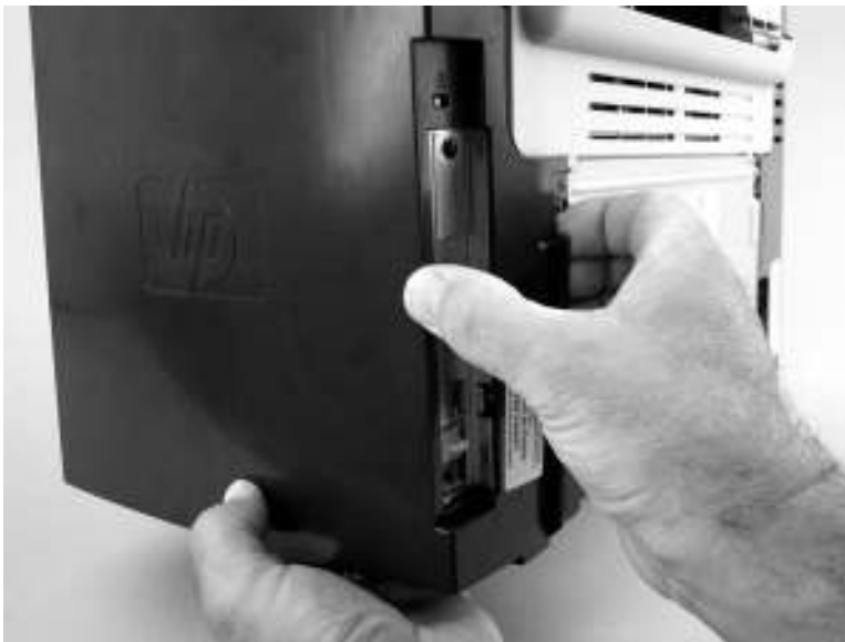
Figure 6-23 Removing the scanner assembly (4 of 14)
