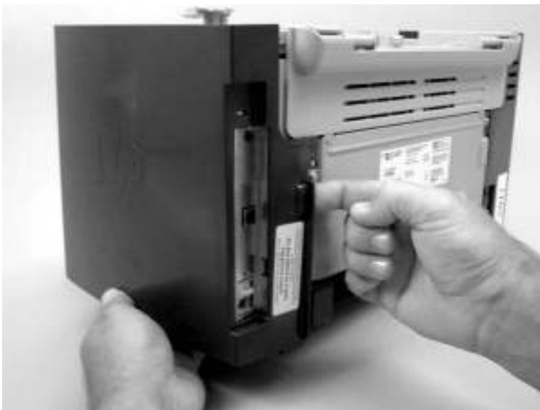
Figure 6-62 Removing the side covers (2 of 4)
