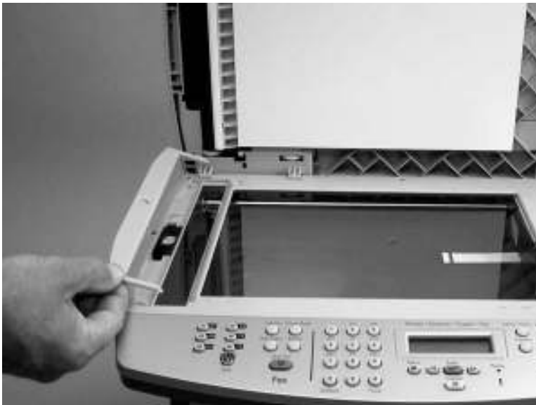
Figure 5-27 Remove the ADF scanner glass (2 of 3)
