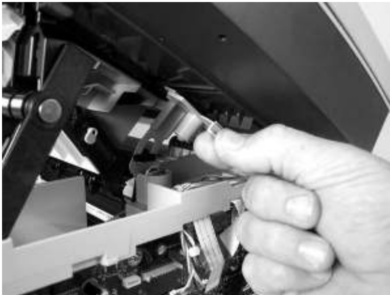
Figure 5-36 Remove the scanner assembly (8 of 10)
