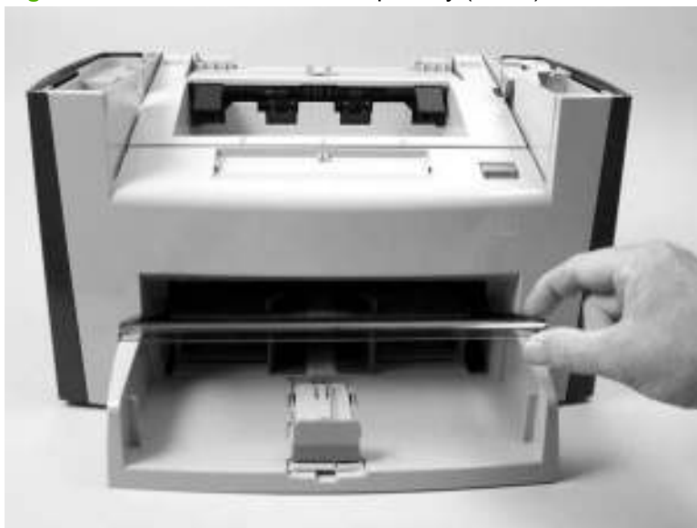
Figure 5-49 Remove the media input tray (1 of 3)
