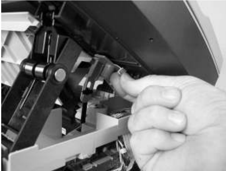
Figure 5-35 Remove the scanner assembly (7 of 10)
