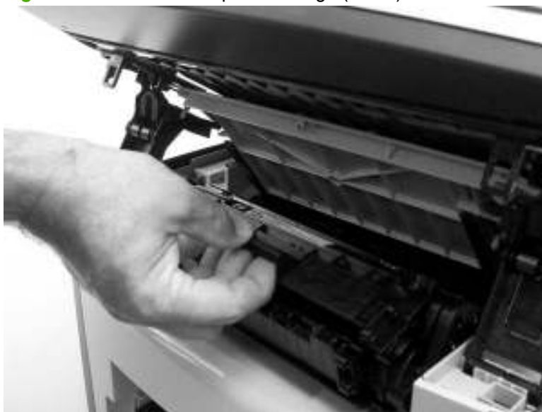
Figure 5-40 Remove the print cartridge (2 of 2)
