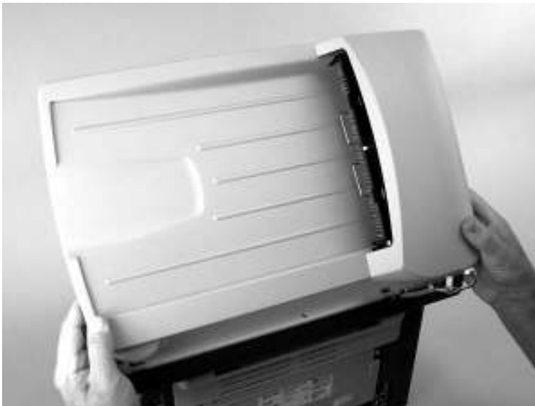
Figure 5-10 Remove the flatbed lid (5 of 5)
