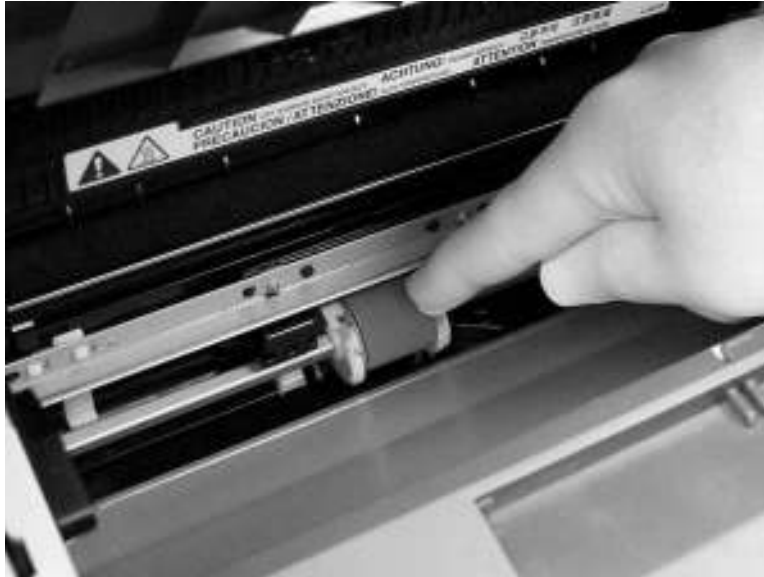
Figure 5-47 Remove the product pickup roller (5 of 5)
