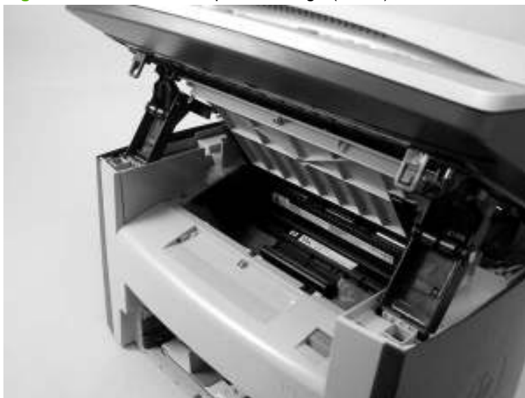
Figure 5-39 Remove the print cartridge (1 of 2)
