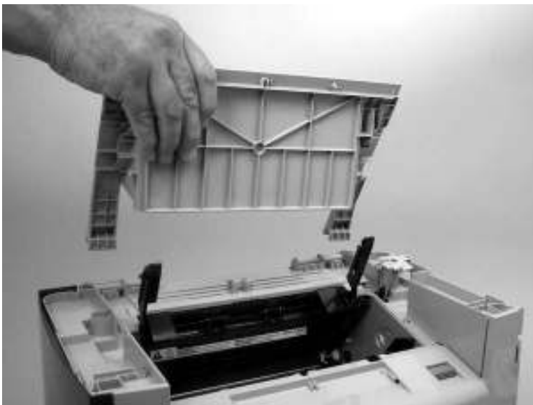
Figure 5-58 Remove the print-cartridge door (2 of 2)
