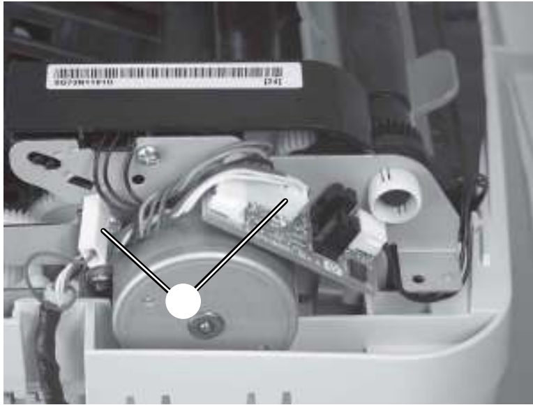
Figure 5-7 Remove the flatbed lid (2 of 5)
