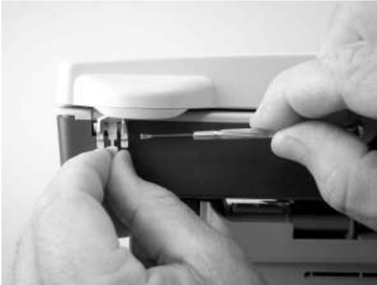
Figure 5-9 Remove the flatbed lid (4 of 5)
