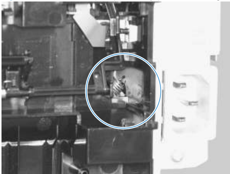
Figure 1-58 Reinstall the pickup assembly (2 of 4; incorrect ground spring position)
