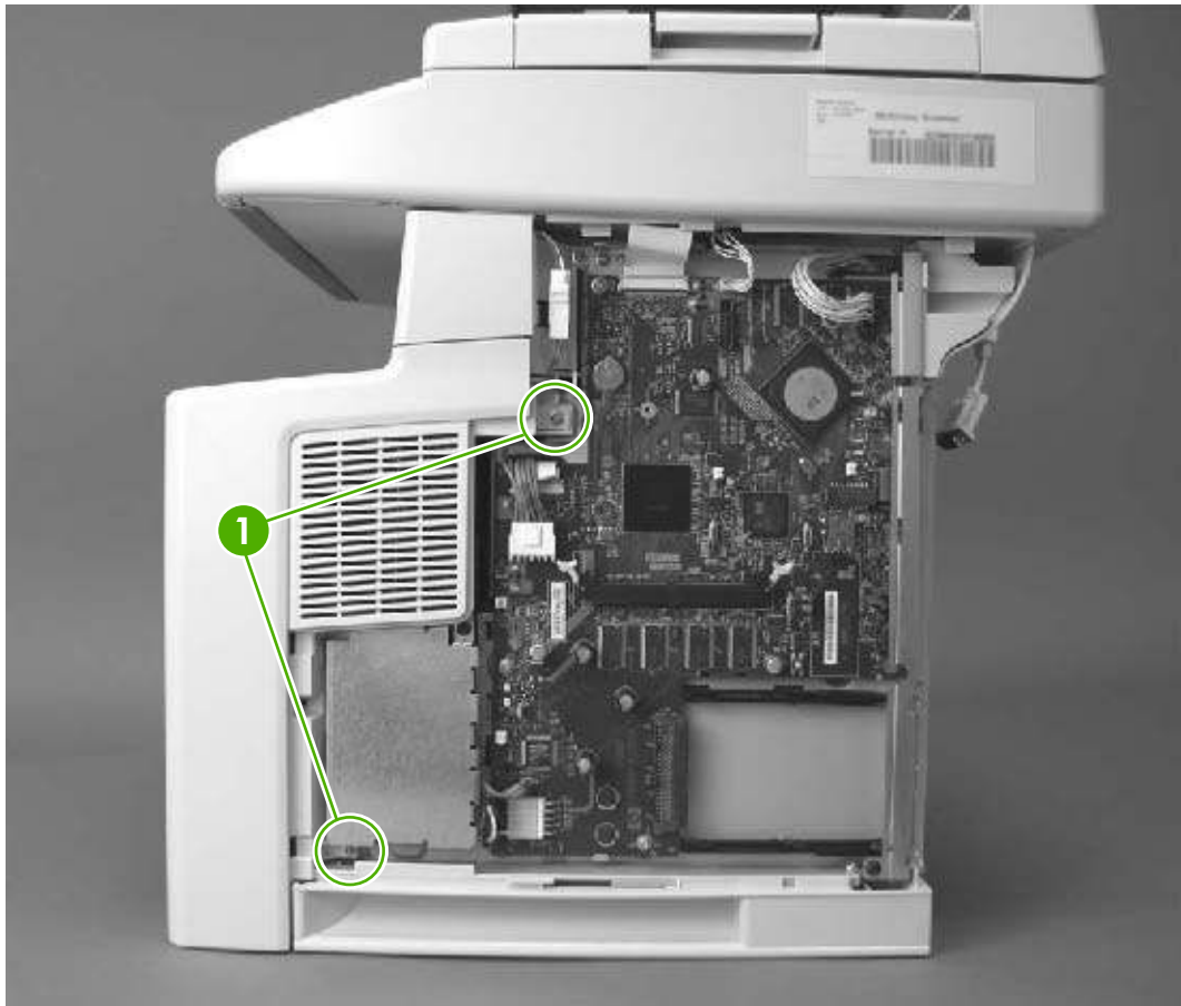
Figure 5-30 Removing the front, right cover (1 of 2)
