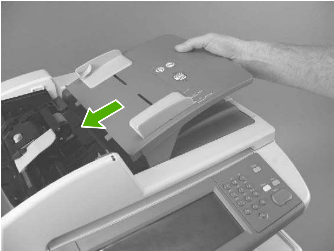
Figure 5-5 Reinstalling the ADF input tray
