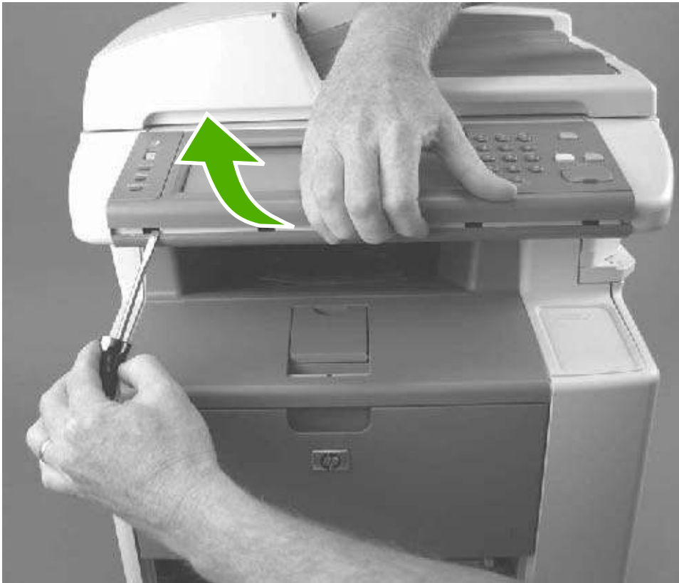
Figure 5-6 Removing the control panel (1 of 2)
