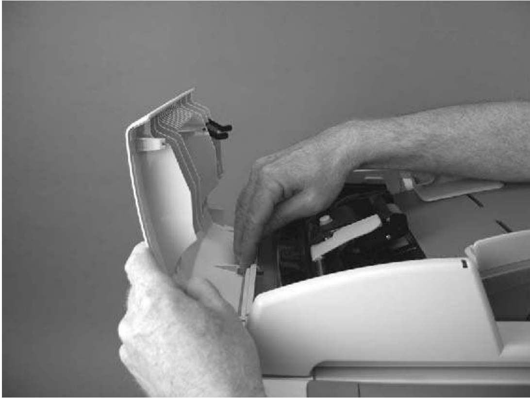
Figure 5-3 Reinstalling the ADF cover
