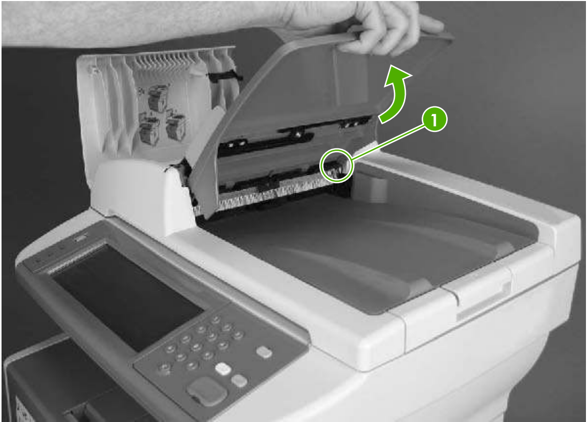
Figure 5-4 Removing the ADF input tray
