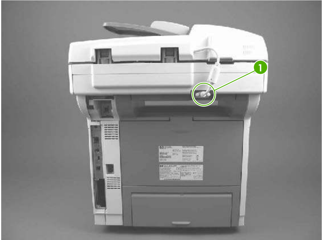
Figure 5-9 Removing the ADF (1 of 3)
