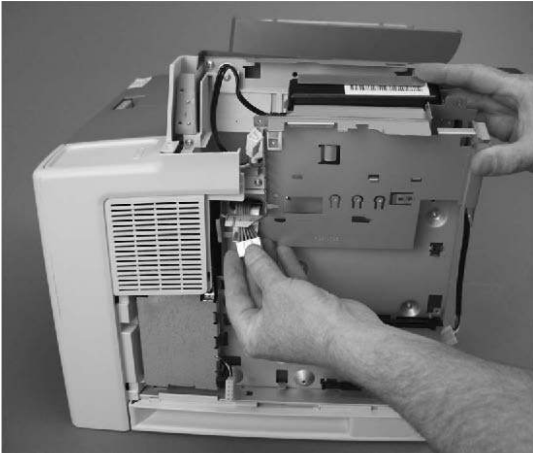
Figure 5-47 Removing the stapler power supply (4 of 5)
