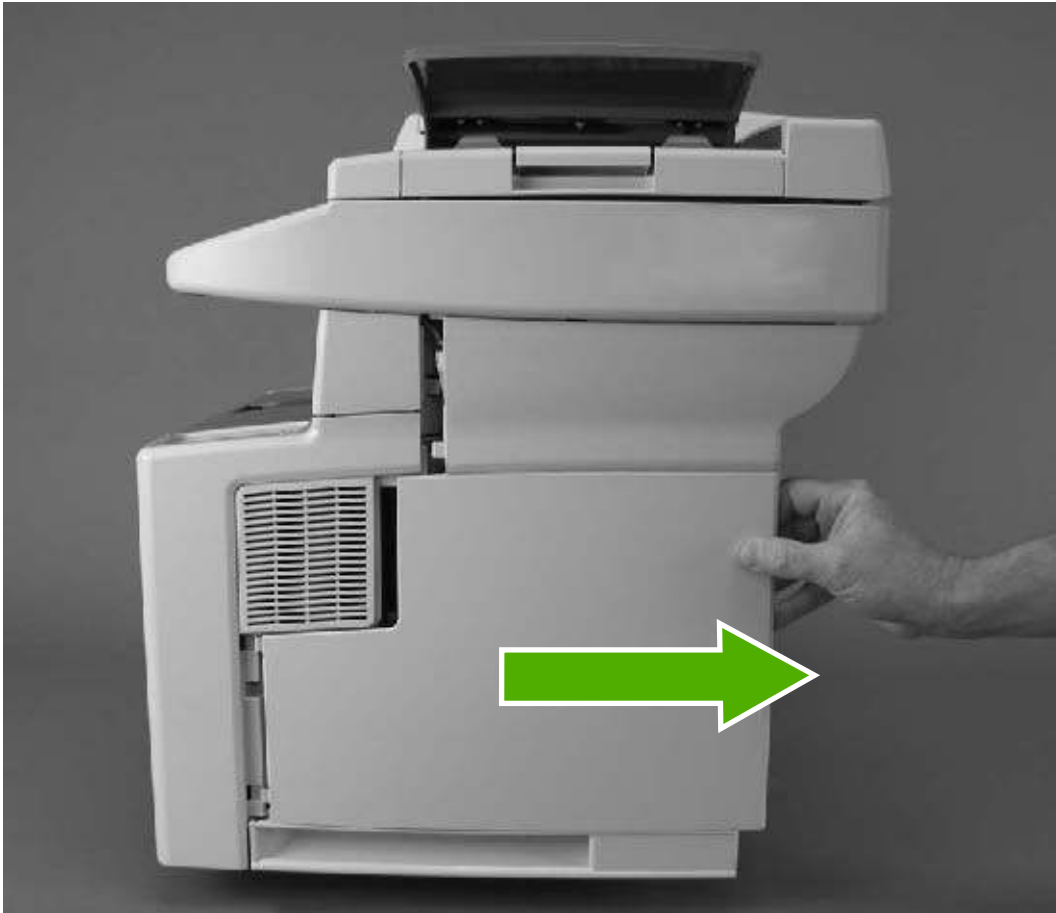
Figure 5-16 Removing the right-side cover
