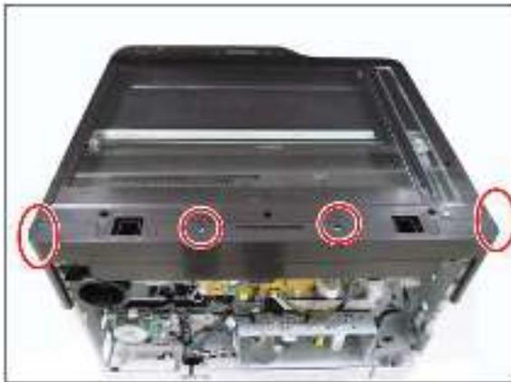
6. Remove the two cap holes and two screws. Pull up and release the left-platen cover.
