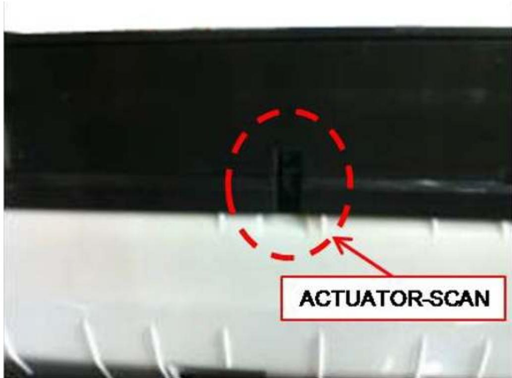
4. Re-seat the Scan Actuator Photo Sensor cable.
