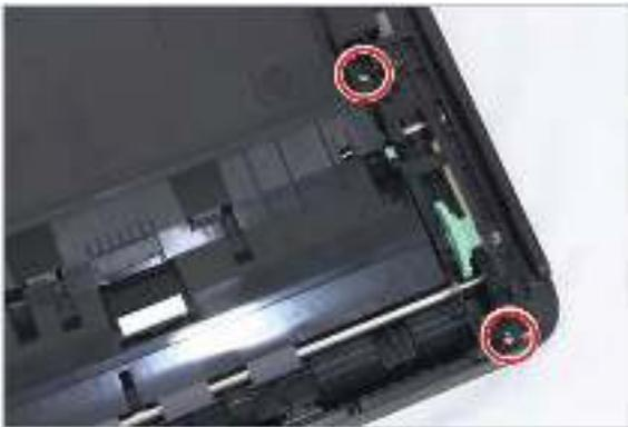
5. Lift up and release the document feeder main frame.
