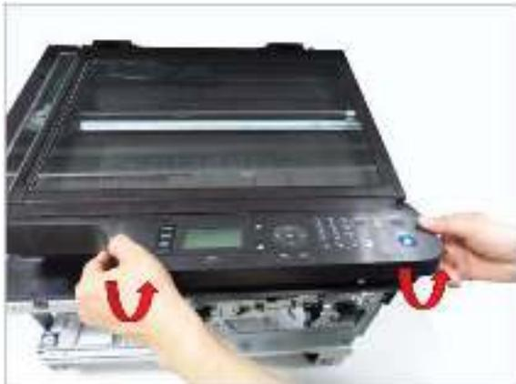
5. Release the OPE unit after unplugging the connector.
