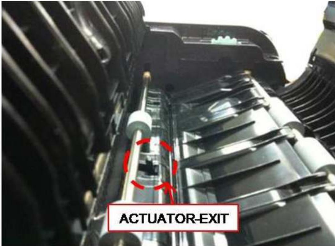
4. Re-seat the Exit Actuator Photo Sensor cable.
