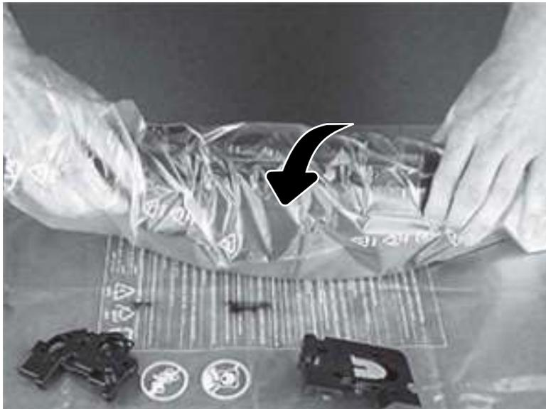
19. Remove the developer unit from the bag, carefully fold up bag and then dispose of the bag and toner.
