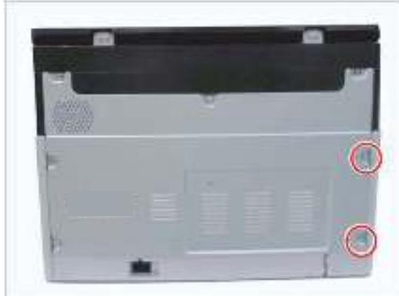
2. Remove the left cover after removing six cap-holes and six screws.
