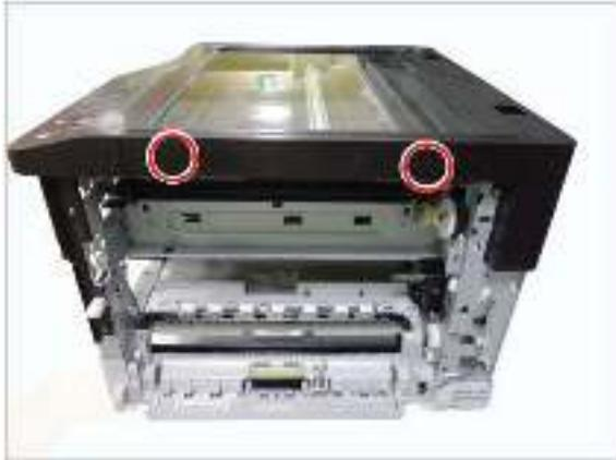
5. Remove four cap holes and four screws. Remove the rear platen cover.
