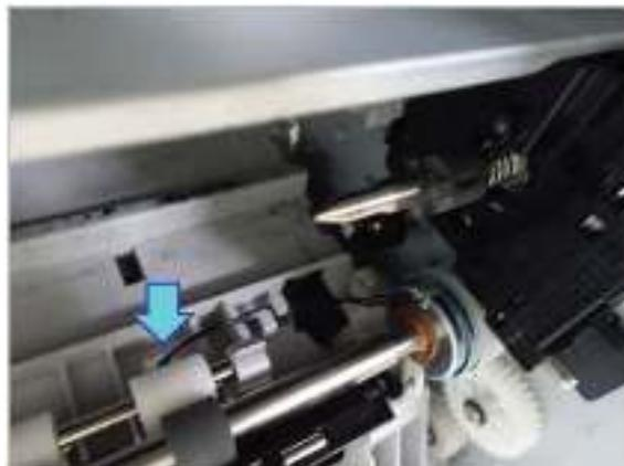
6. Remove the registration shaft assembly by pulling it to the left, then out (callouts 1 and 2).
