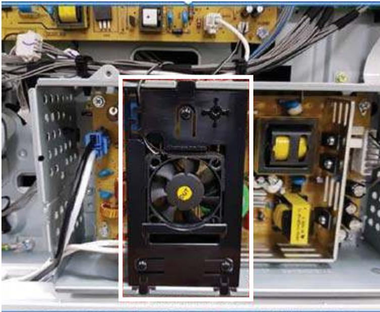
3. Unplug all connectors on the SMPS (LVPS) board. Remove four screws. Remove the SMPS (LVPS) board.
