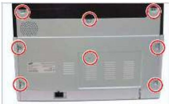
2. Open the document feeder unit. Remove six screw-caps, and then remove six screws.
