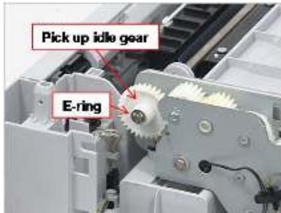
5. Remove the e-ring. Release the bushing.
