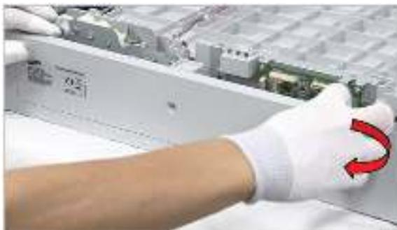
4. Unplug all connectors from the SCF board. Remove four screws. Release the SCF board.
