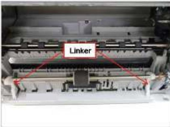
10. Release the MP pickup assembly.
