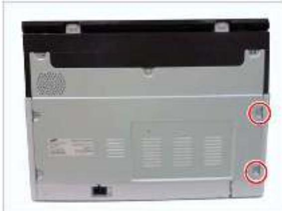
2. Remove the left cover after removing the six cap holes and screws.
