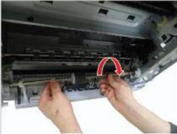
11. Remove the MP pickup roller by pulling the tabs (callouts 1 and 2).
