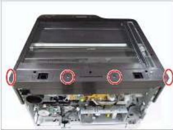
4. Unplug the connector. Remove two screws. Remove the exit motor.
