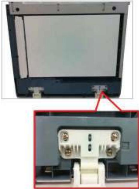
2. Adjust the position of the document feeder hinge as the skew status.
