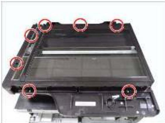
7. Lift up and release the upper platen.
