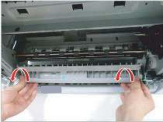
5. Remove the rear-dummy cover after removing two screws.
