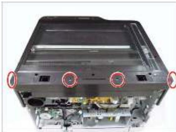
4. Remove two screws. Release the support hooks. Remove the HVPS board.
