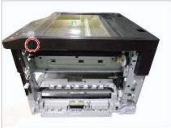
3. Release the left scan-cover after removing two screws.
