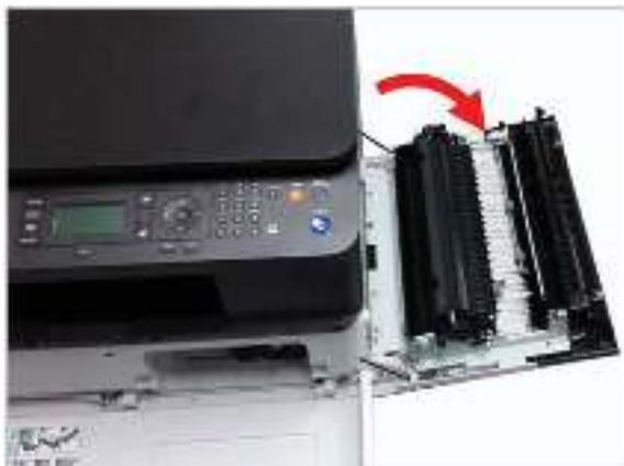
4. Remove the toner cartridge while pushing both hooks.
