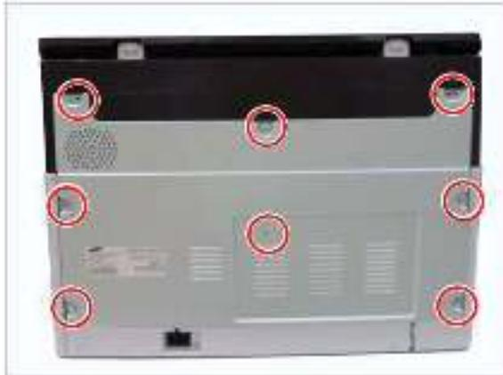
2. Remove the document feeder unit or platen cover.
