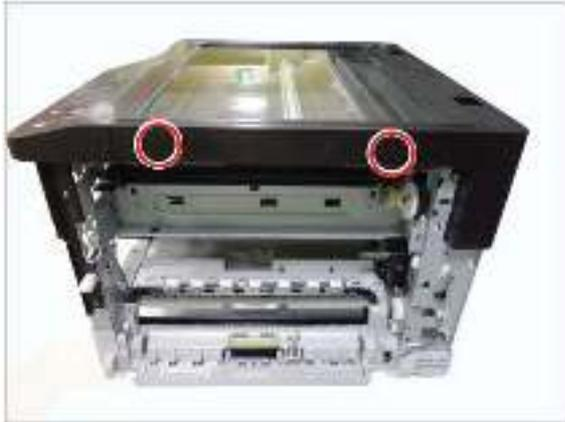
5. Remove the four cap holes and four screws. Remove the rear-platen cover.
