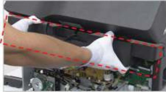
5. Remove one screw. Unplug the document feeder cable.
