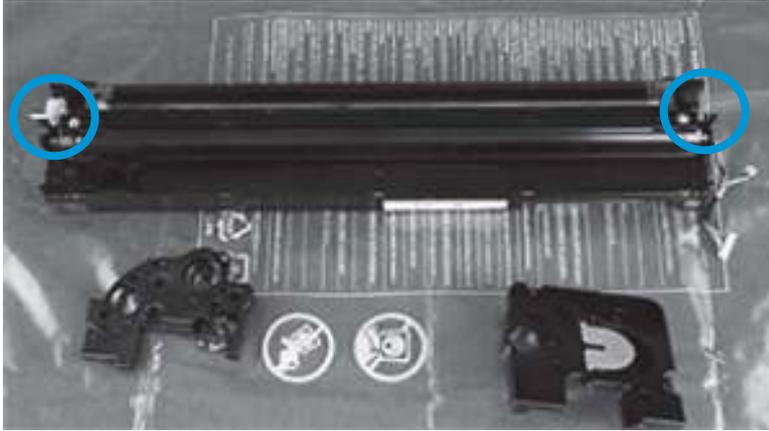
24. Remove the replacement drum unit from the shipping package.
