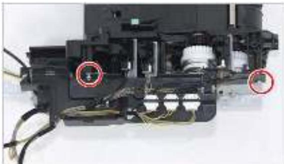
7. Unplug the connector. Remove four screws. Release the motor.
