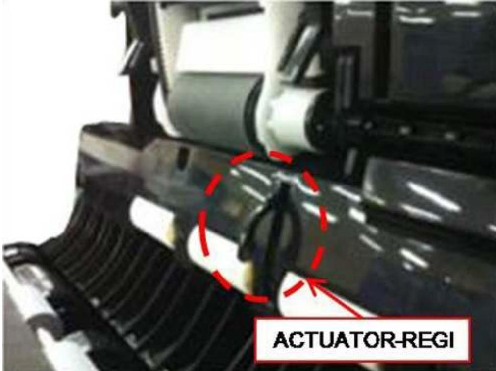
4. Re-seat the Actuator Registration Photo Sensor cable.
