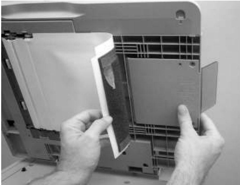
Remove the ADF output-bin extension (2 of 2)
