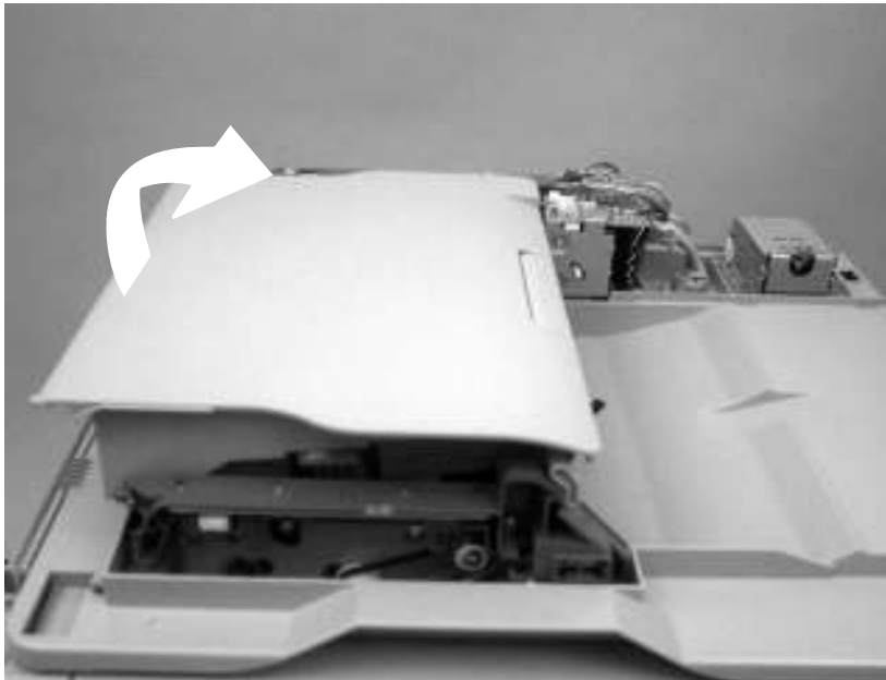
Remove the ADF jam-access cover and latch (1 of 3)
