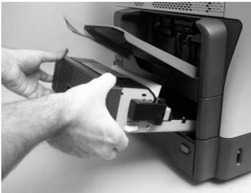
Remove the duplex-printing unit (2 of 2)
