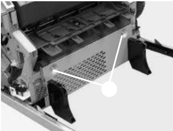
Remove the bottom cover (1 of 2)
