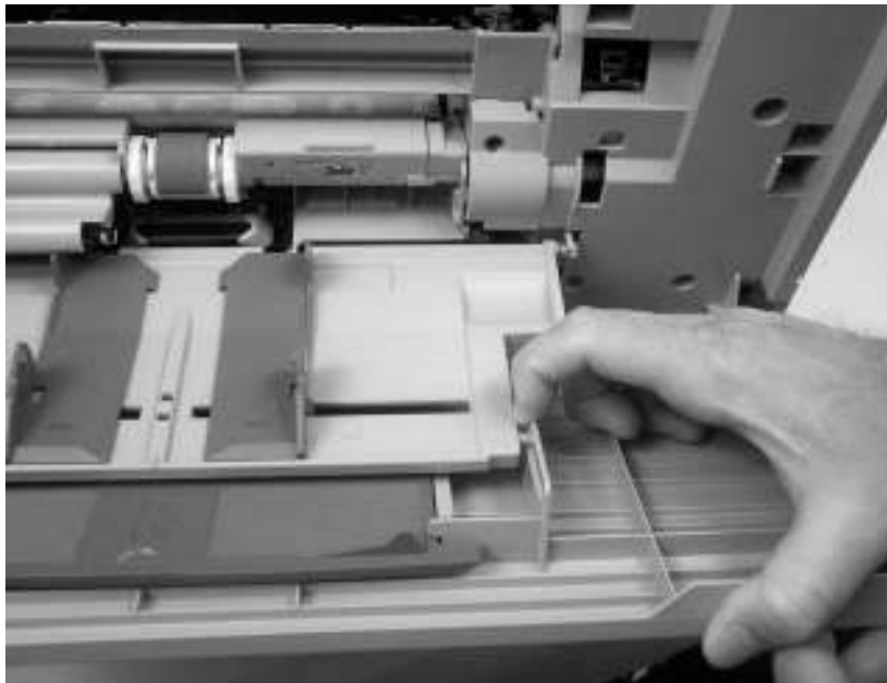
Remove the tray 1 assembly (1 of 5)
