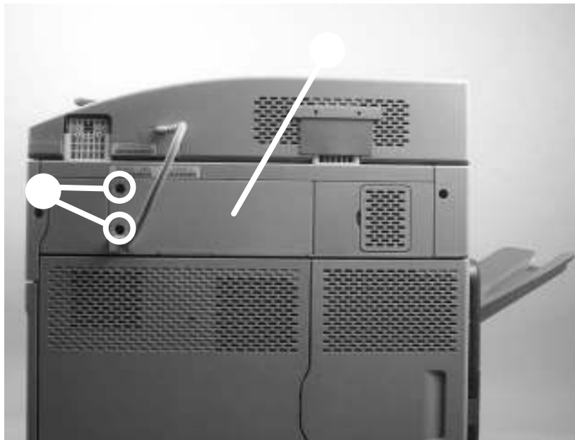
Remove the ADF assembly (1 of 3)
