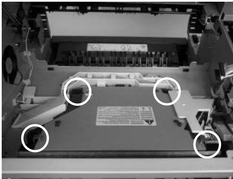
Remove the laser/scanner (1 of 2)
