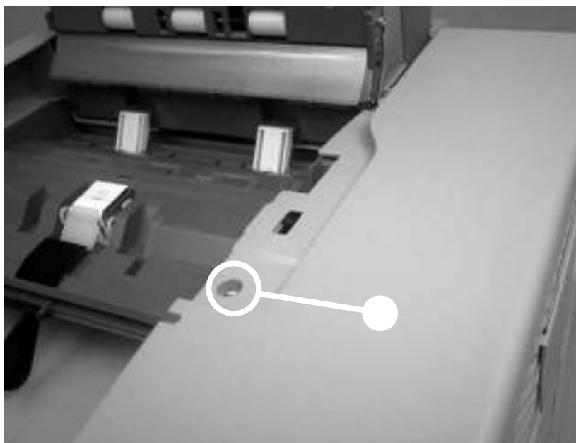
Remove the ADF rear cover (1 of 2)
