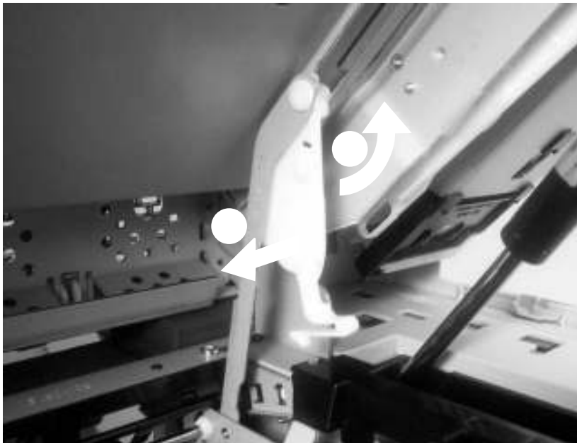
Remove the reversing assembly (6 of 8)
