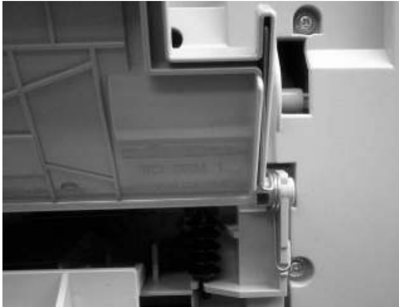
Correct tray 1 rear-hinge-spring placement
