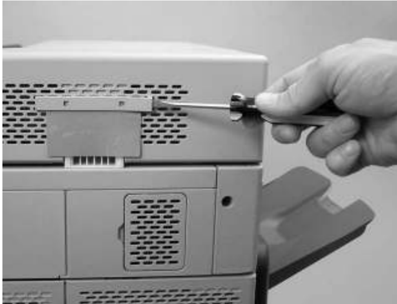
Remove the ADF-hinge flap (1 of 3)
