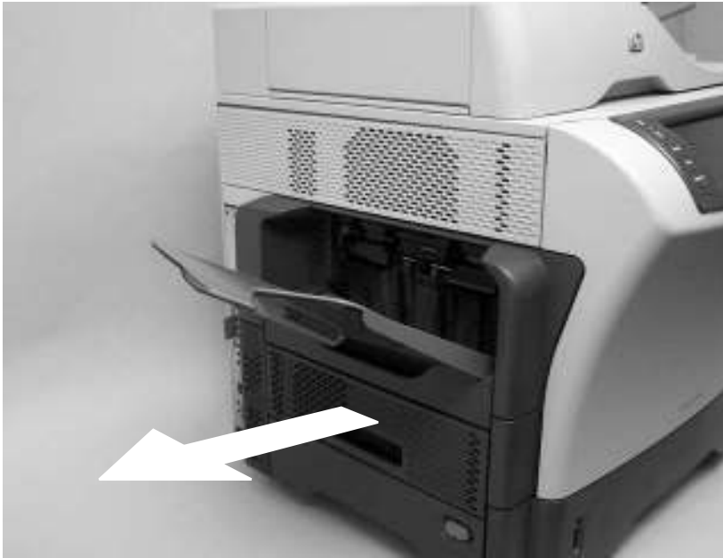
Remove the duplex-printing unit (1 of 2)
