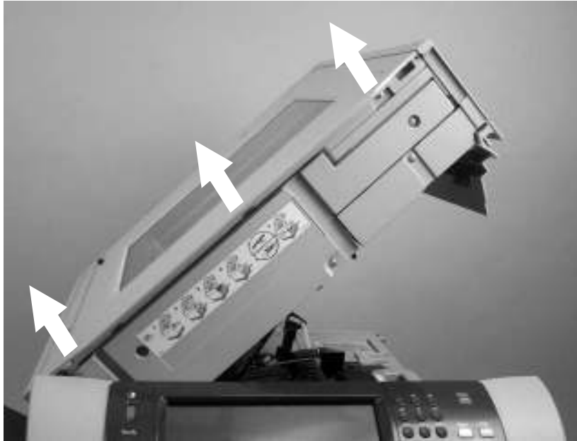
Remove the scanner assembly (1 of 8)
