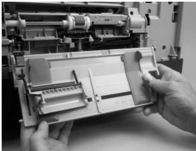
Remove the tray 1 assembly (5 of 5)
