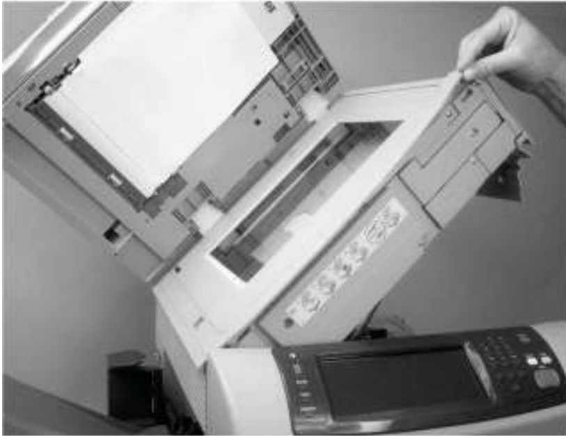
Remove the top-cover flatbed flange (1 of 2)
