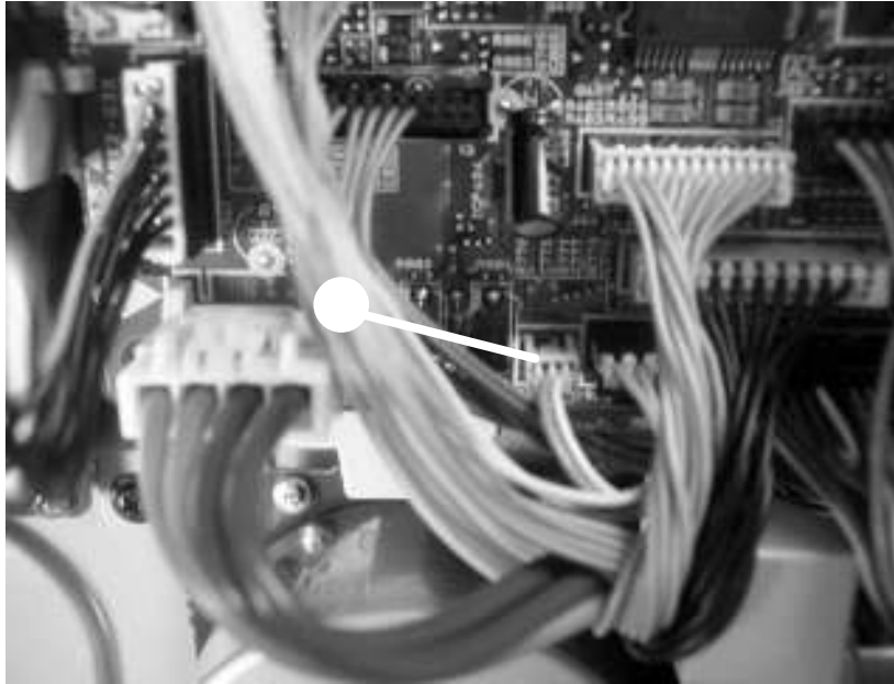
Remove the lifter-drive assembly (5 of 5)
