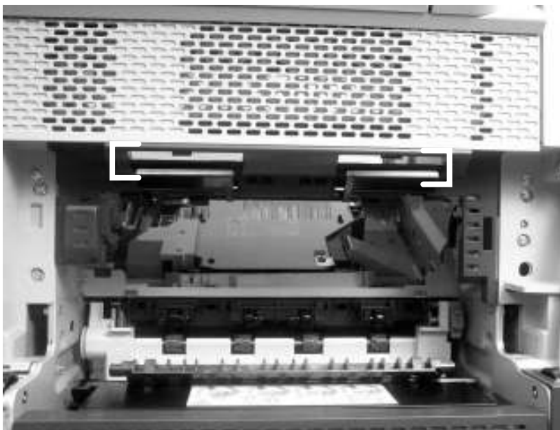
Correct installation of the output-bin-full sensor
