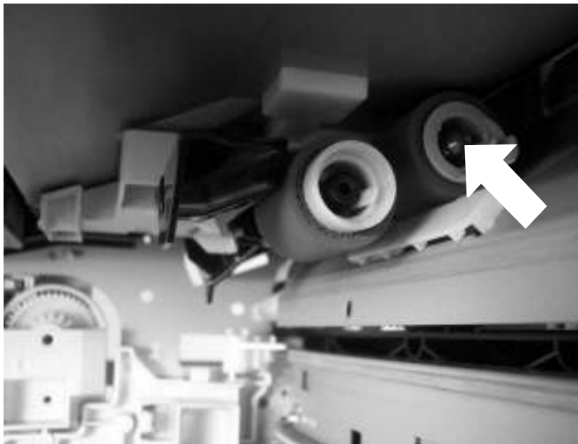
Cassette feed-roller shaft (push here while replacing the gear)
