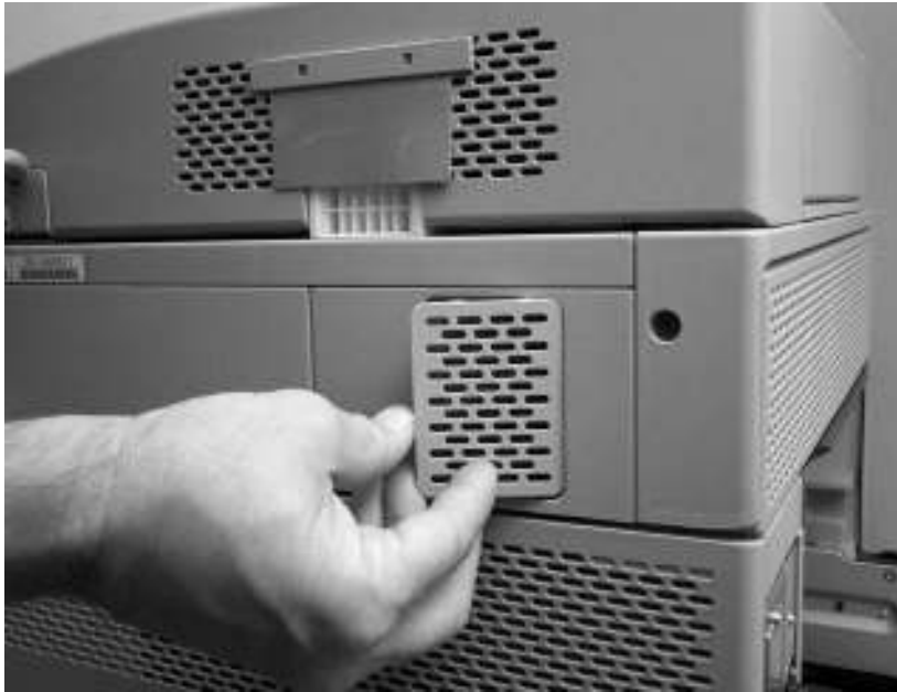
Remove the scanner filter (1 of 2)
