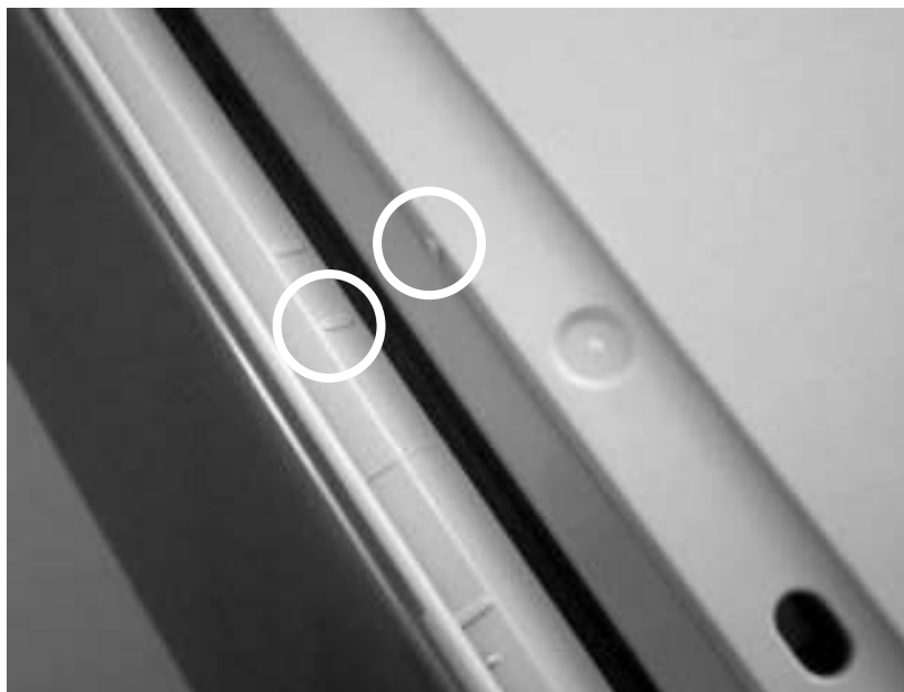
Correctly positioning the scanner assembly
