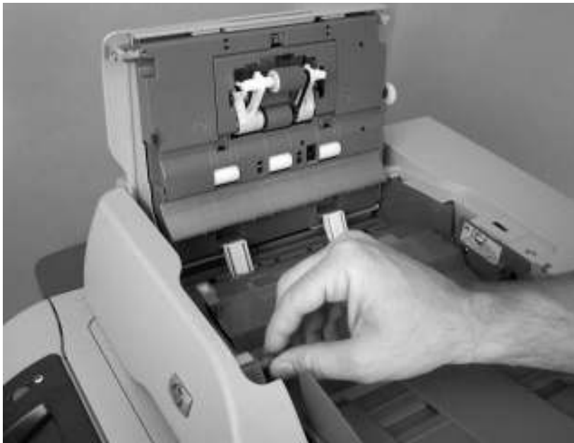
Remove the ADF input tray (2 of 3)
