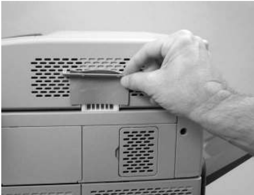
Remove the ADF-hinge flap (3 of 3)
