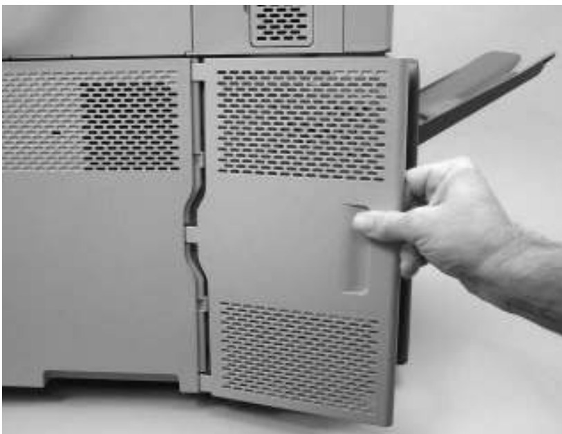
Remove the formatter cover and formatter (1 of 3)
