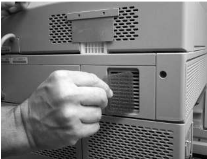
Remove the scanner filter (2 of 2)
