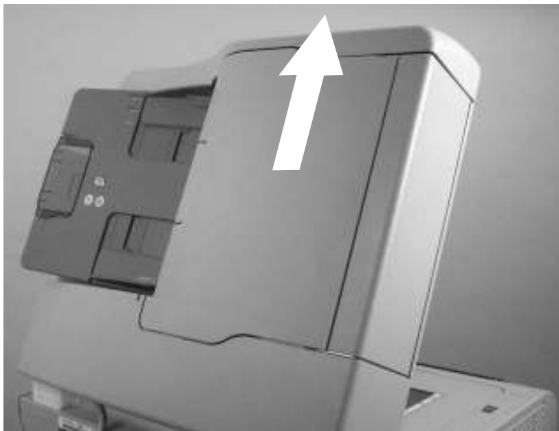
Remove the ADF assembly (3 of 3)
