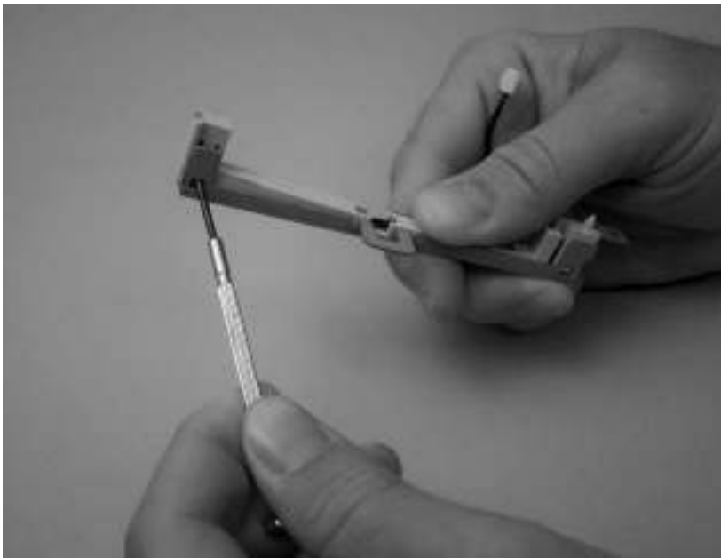
Remove the thermistor (3 of 4)
