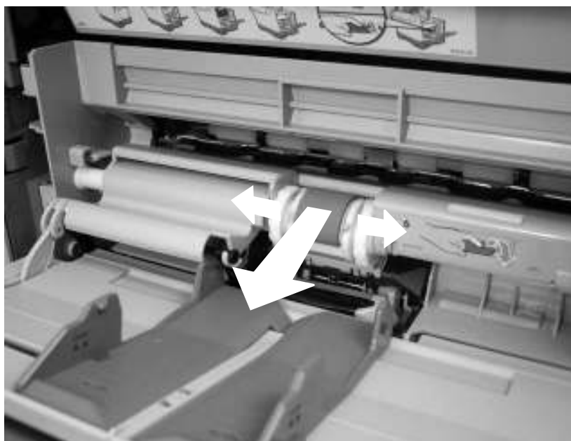
Remove the tray 1 pickup roller
