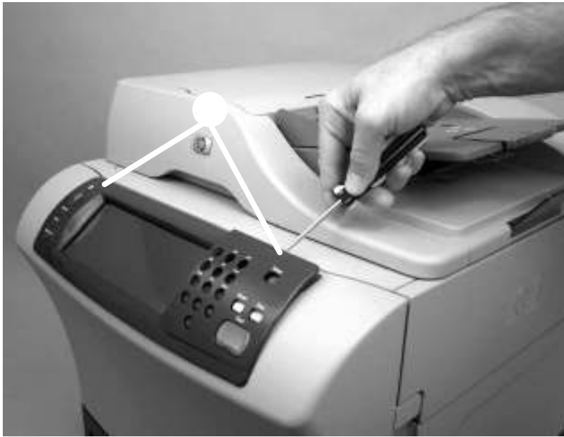
Remove the control-panel overlays
