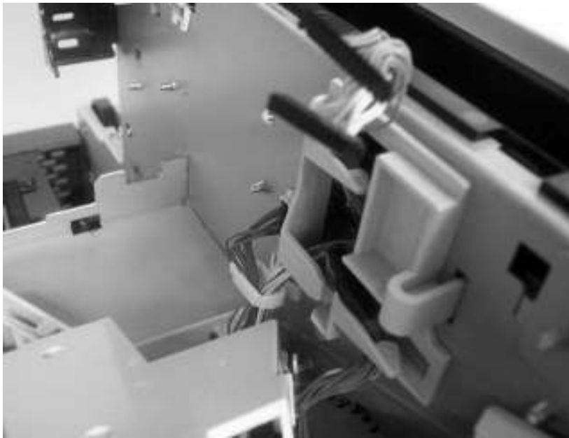
Remove the laser/scanner (1 of 2)
