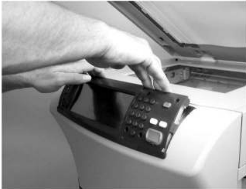
Remove the control panel (1 of 2)
