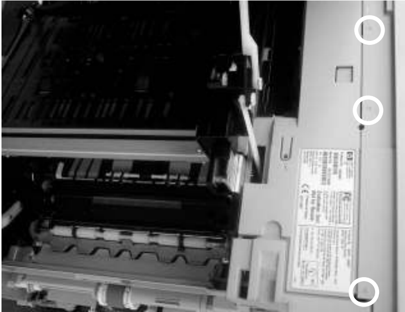
Remove the back cover (2 of 3)
