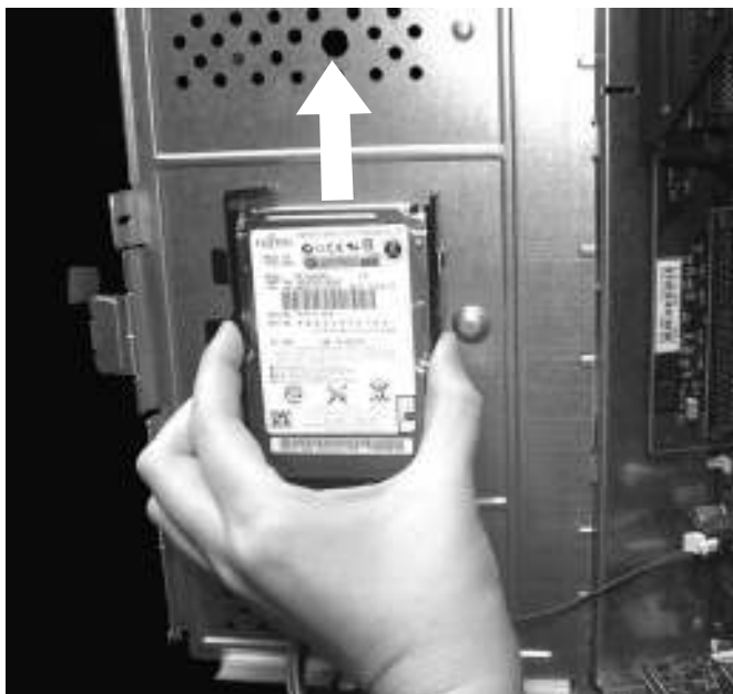
Remove the hard drive (2 of 2)
