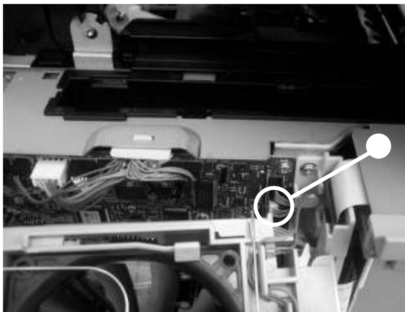
Remove the PFC power supply (3 of 8)
