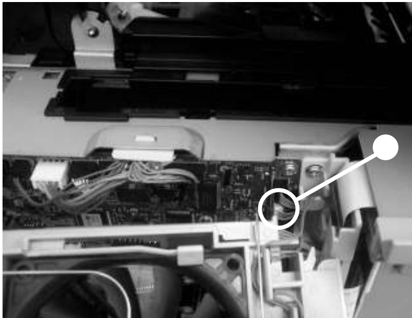
Remove the DC controller (3 of 6)
