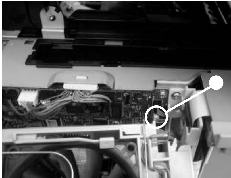
Remove the tray 1 feed-assembly (11 of 13)
