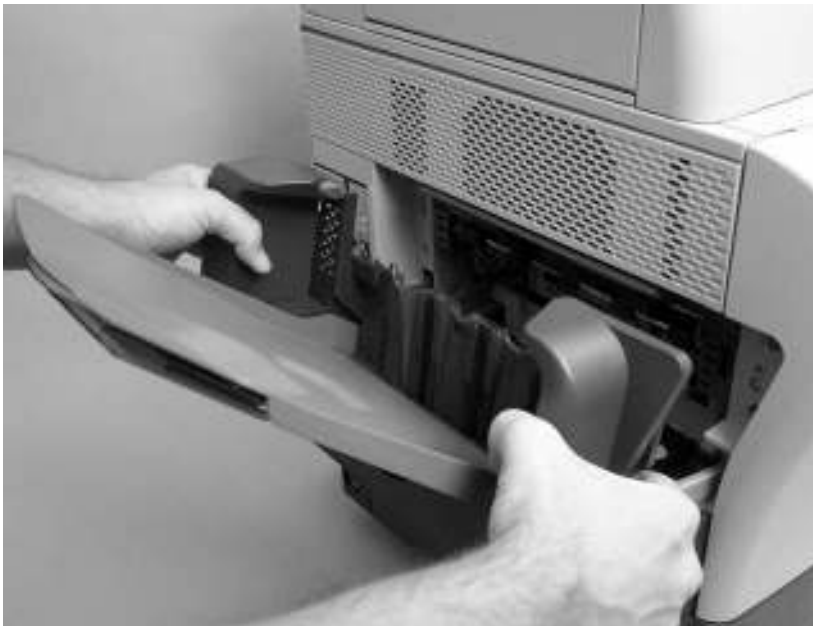
Remove the output-bin assembly (2 of 2)
