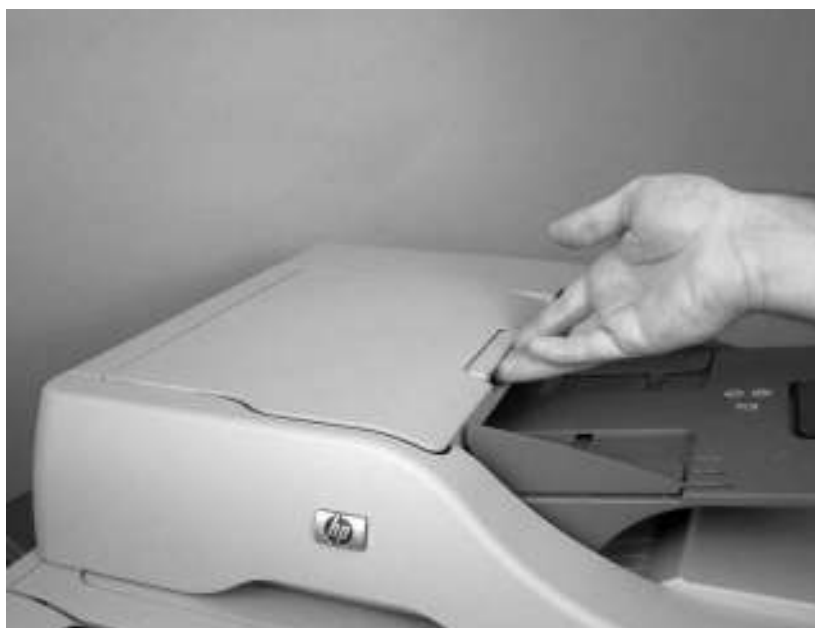
Remove the ADF input tray (1 of 3)
