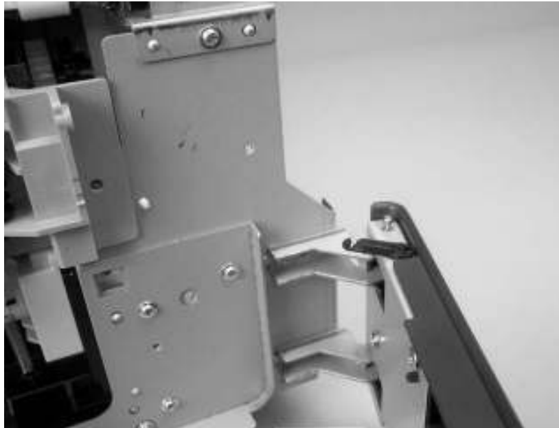
Remove the tray 1 feed-assembly (1 of 13)
