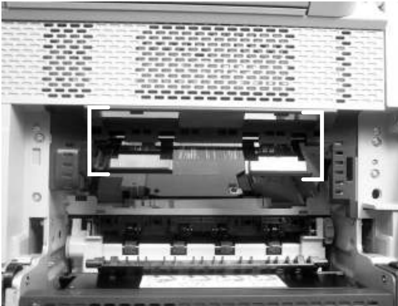
Incorrect installation of the output-bin-full sensor
