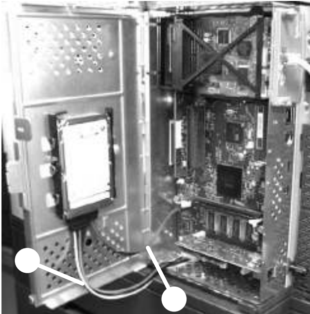
Remove the hard drive (1 of 2)
