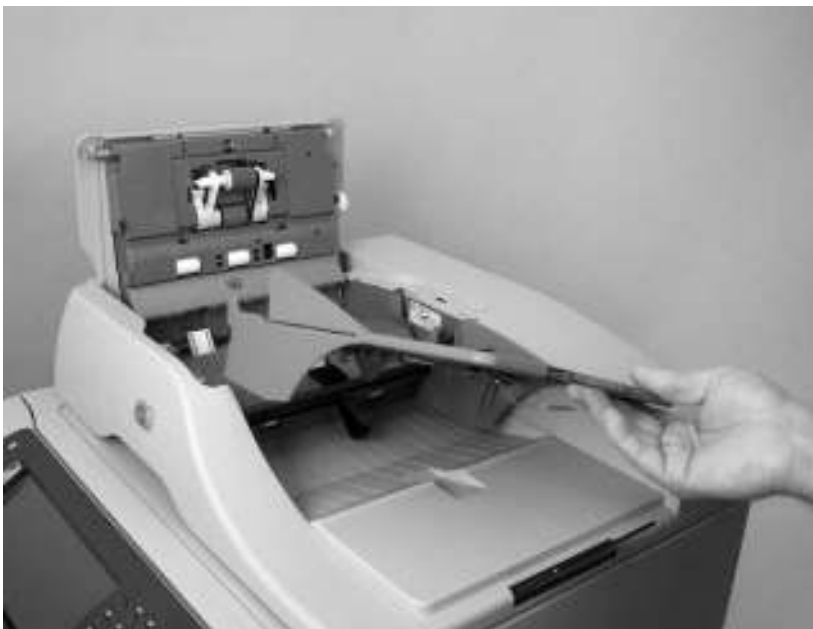
Remove the ADF input tray (3 of 3)
