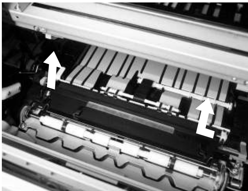
Remove the transfer roller
