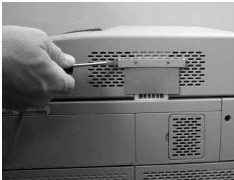
Remove the ADF-hinge flap (2 of 3)
