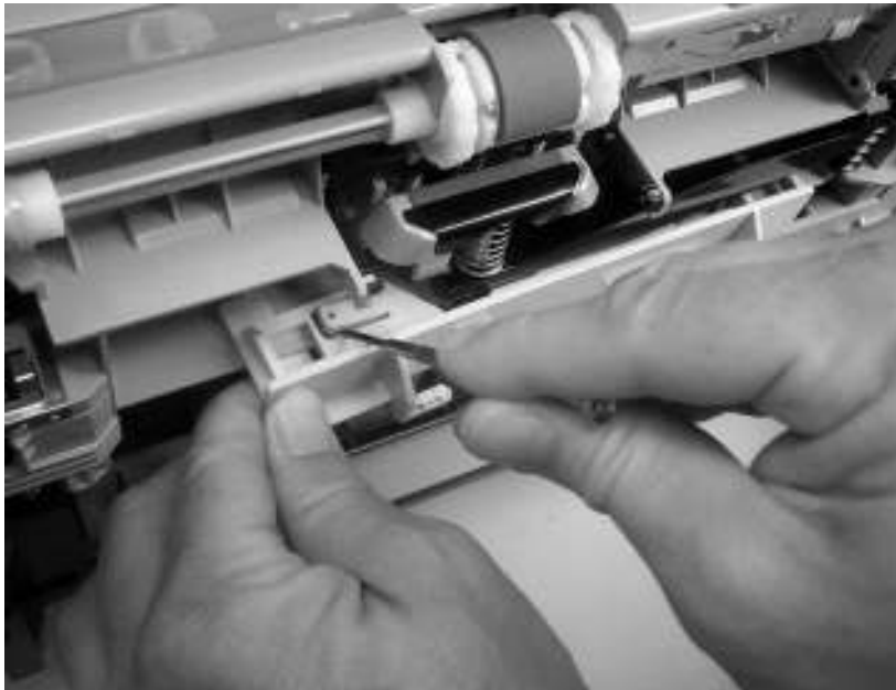
Remove the front-cover support (1 of 2)
