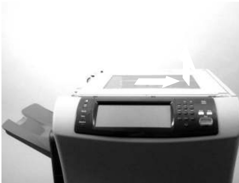
Remove the scanner assembly (8 of 8)
