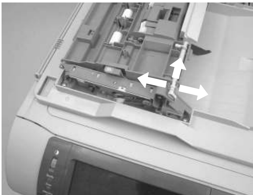
Remove the ADF jam-access cover and latch (2 of 3)
