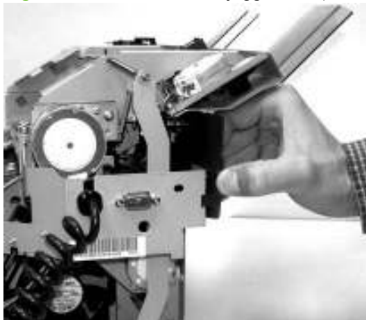
Figure 5-210 Remove the jogger unit (1 of 7)
