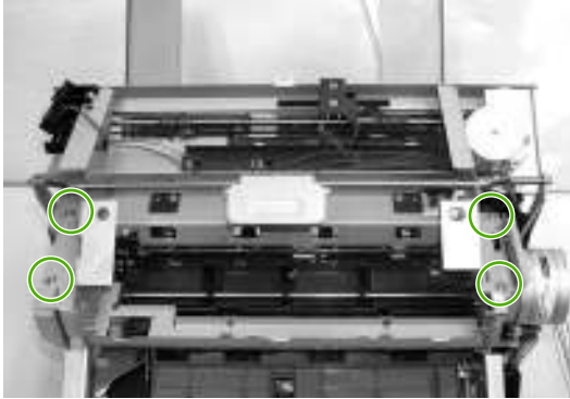
Figure 5-215 Remove the jogger unit (6 of 7)
