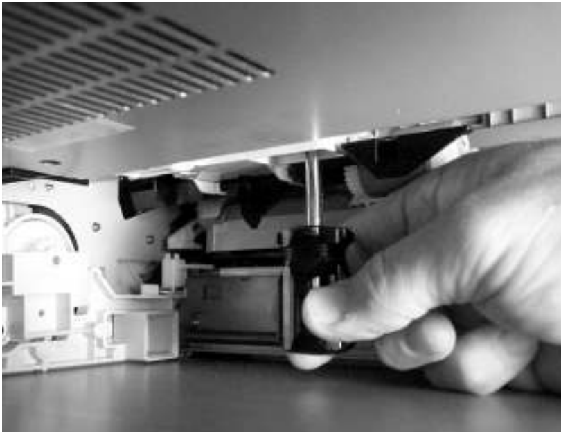
Figure 5-162 Remove the tray 2 paper-present sensor
