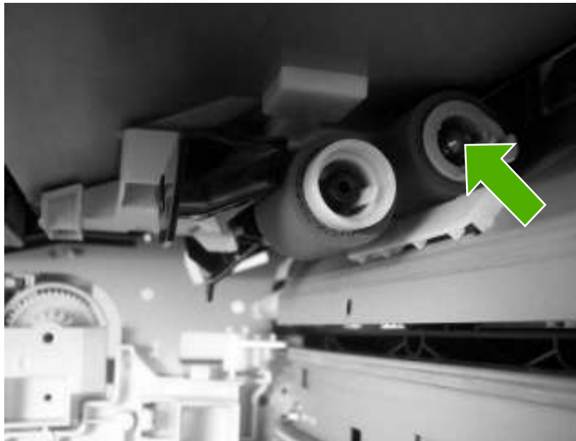
Figure 5-134 Cassette feed-roller shaft (push here while replacing the gear)
