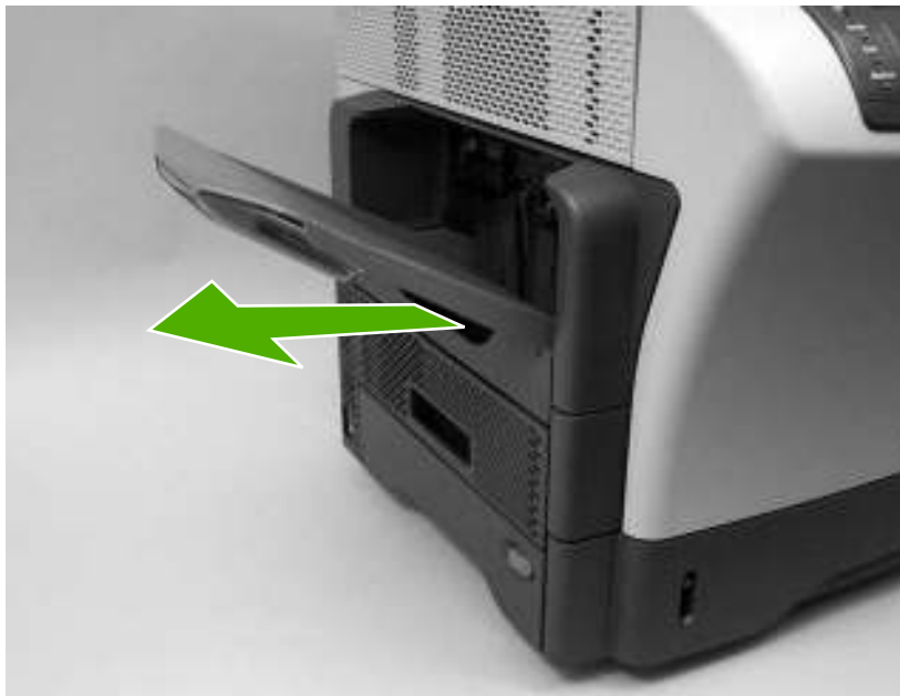
Figure 5-16 Remove the output-bin assembly (1 of 2)
