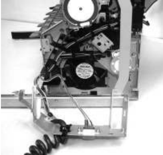
Figure 5-212 Remove the jogger unit (3 of 7)
