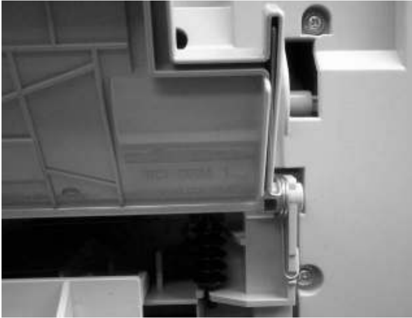
Figure 5-79 Correct tray 1 rear-hinge-spring placement
