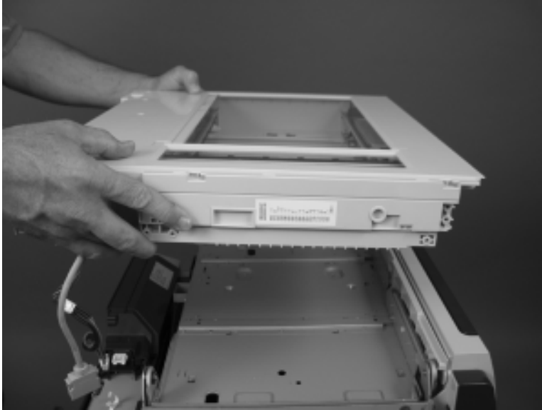
Figure 2-204 Remove the scanner assembly (4 of 4)
