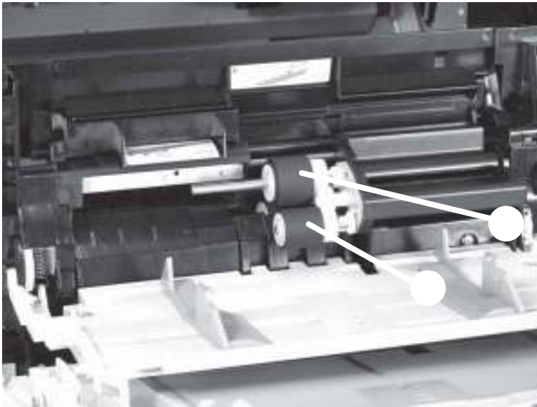
Figure 2-29 Remove the Tray 1 pickup and feed rollers (2 of 2)
