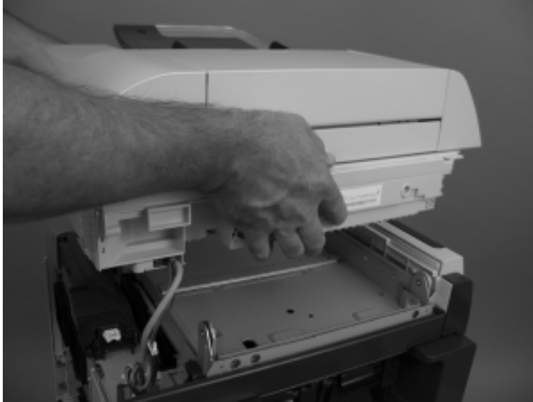
Figure 2-86 Remove the document feeder (4 of 4)
