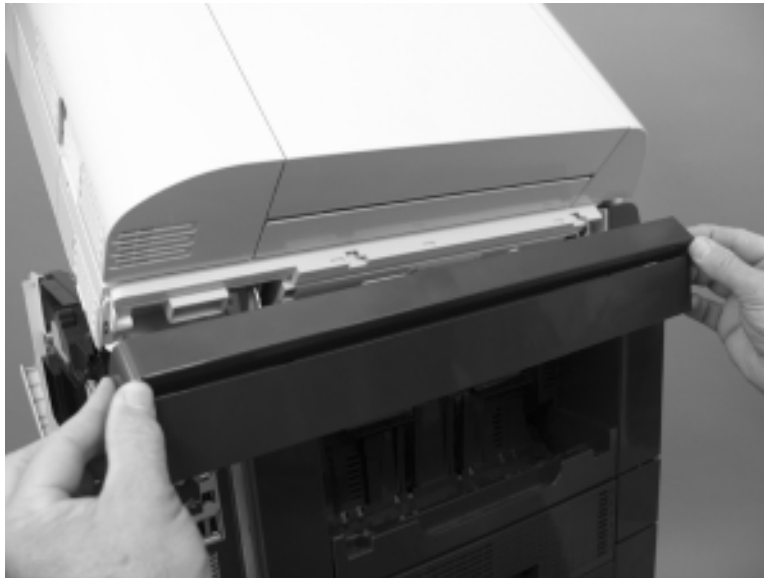
Figure 2-81 Remove the document feeder hinge cover (3 of 3)
