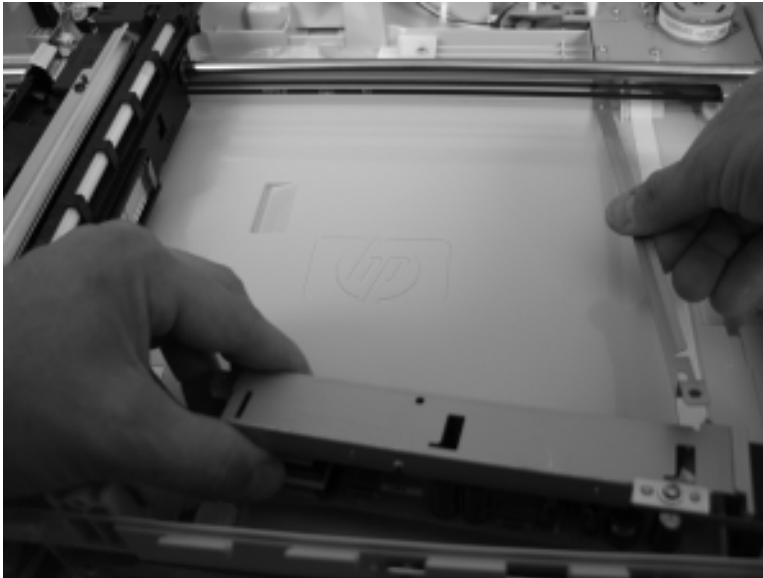
Figure 2-219 Remove the inverter (2 of 2)
