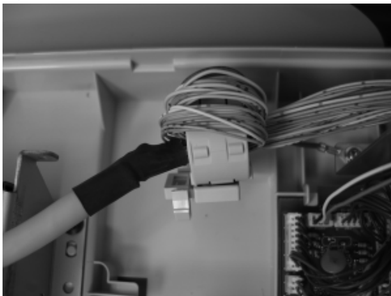
Figure 2-192 Reinstall the document feeder cable
