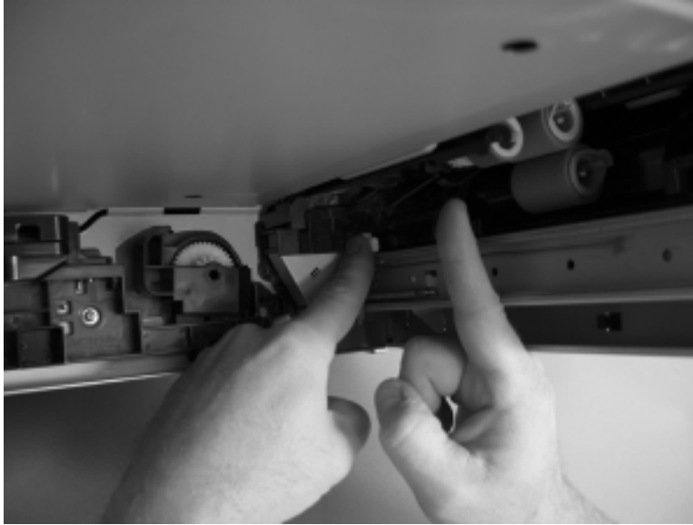
Figure 3-21 Test the PS107/PS907 Tray 2 paper surface sensor
