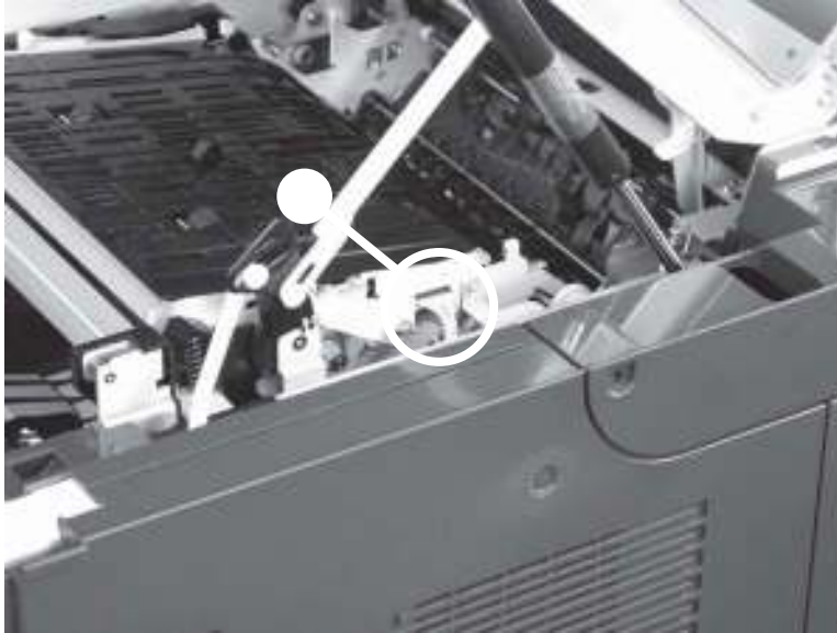
Figure 2-94 Remove the switchback assembly (3 of 6)
