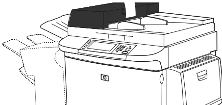
Figure 4-20 Clean the ADF rollers (4 of 6)
