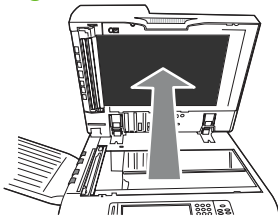
Figure 4-10 Clean the ADF delivery system (3 of 5)
