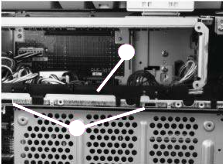
Figure 6-120 Remove the scanner controller board (3 of 5)
