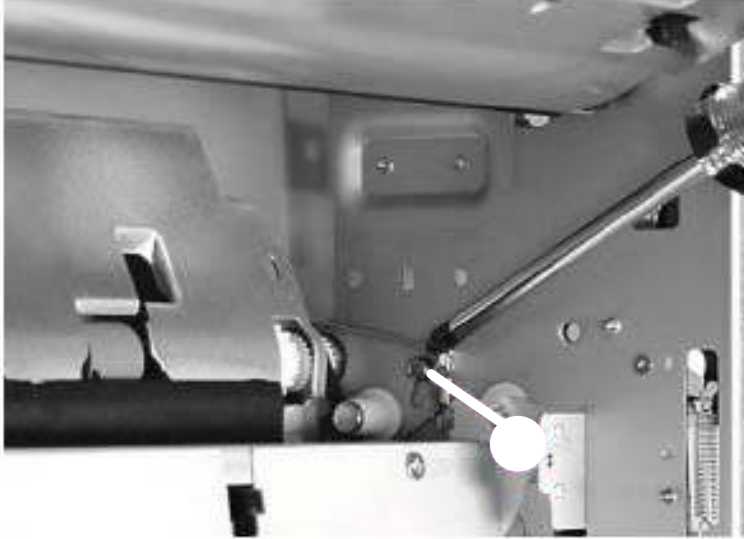
Figure 6-101 Remove the lower registration roller assembly (11 of 11)
