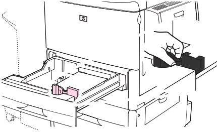
Figure 3-20 Load custom media in Trays 2, 3, and 4 (5 of 6)
