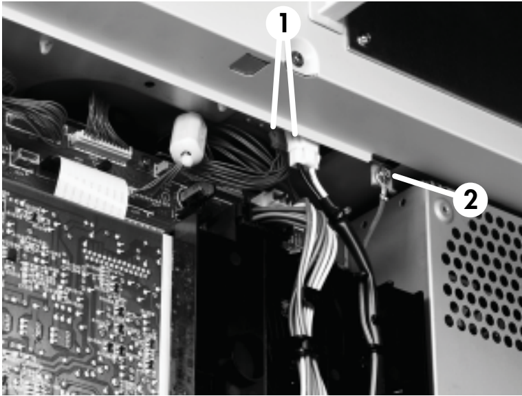
Figure 6-124 Remove the scan engine (1 of 7)
