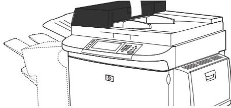
Figure 4-13 Clean the top ADF glass strip (1 of 4)
