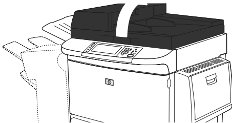
Figure 4-8 Clean the ADF delivery system (1 of 5)
