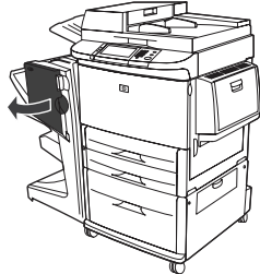
Figure 7-56 Clear a staple jam from the multifunction finisher (1 of 11)
