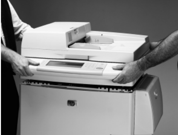
Figure 6-129 Remove the scan engine (6 of 7)
