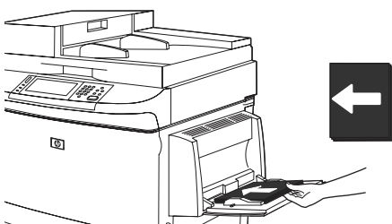
Figure 3-2 Load Tray 1 (2 of 3)
