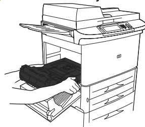
Figure 7-22 Clear jams in the duplex printing accessory (6 of 6)
