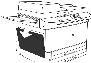
Figure 7-78 Clear jams in the left door (2 of 4)
