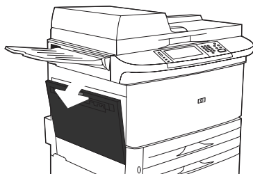
Figure 7-18 Clear jams in the duplex printing accessory (2 of 6)
