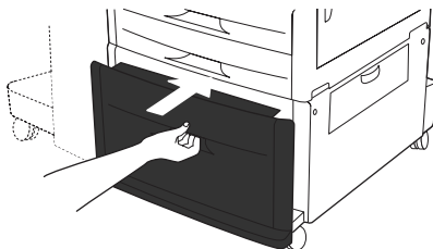
Figure 7-33 Clear jams in Tray 4 (3 of 4)
