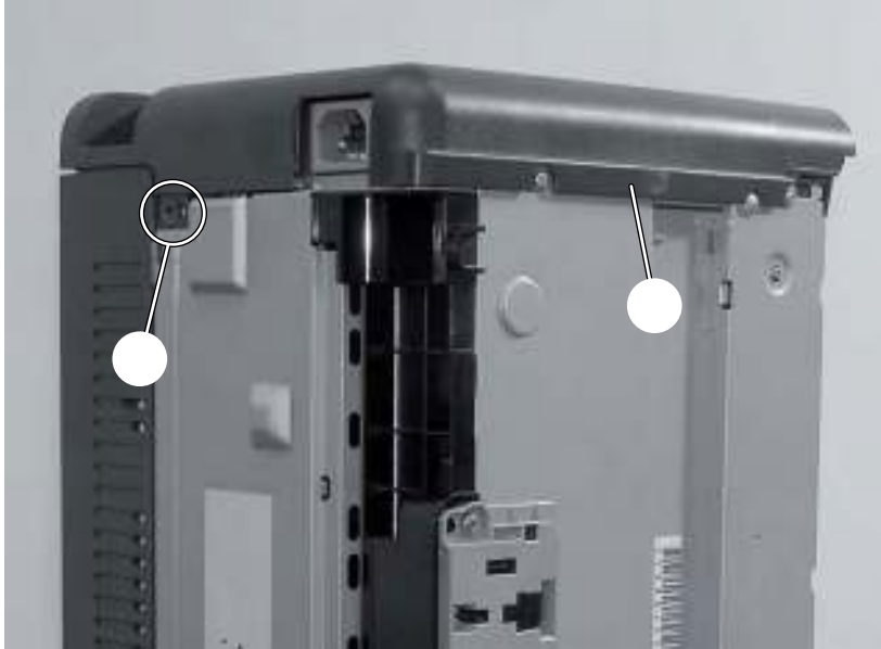
Figure 4-5 Remove side covers (3 of 4)
