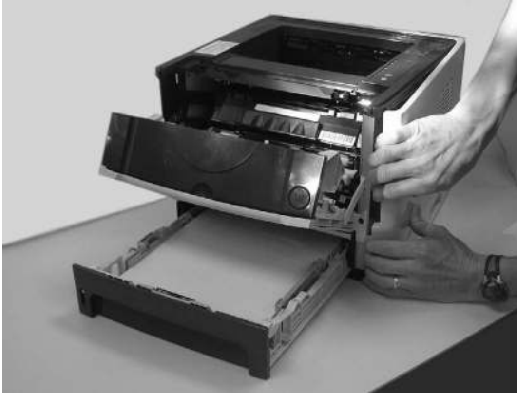
Removing the right-side cover
