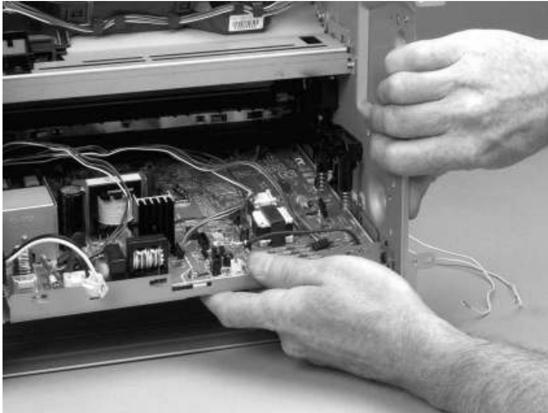
Removing the ECU (6 of 7)
