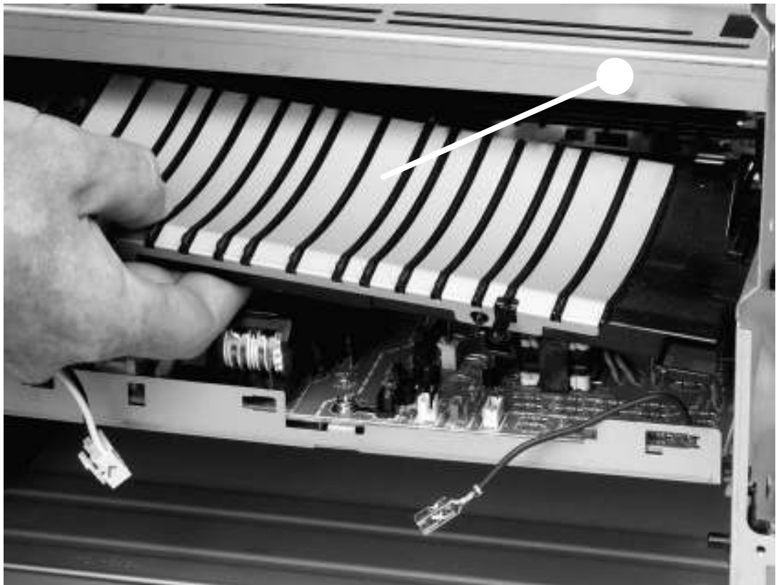
Removing the ECU (1 of 7)
