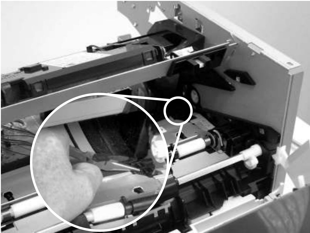
Removing the transfer roller
