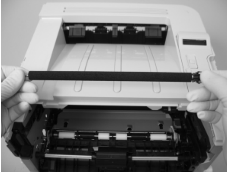
Figure 6-20 Remove the transfer roller (5 of 5)
