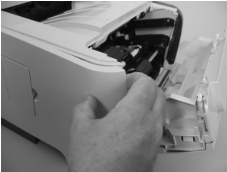
Figure 6-30 Remove the left cover (2 of 4)
