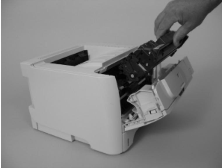
Figure 6-2 Remove the print cartridge
