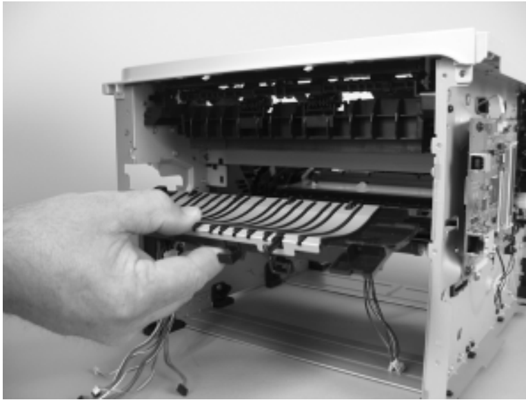
Figure 6-114 Remove the paper-feed-guide assembly (2 of 2)
