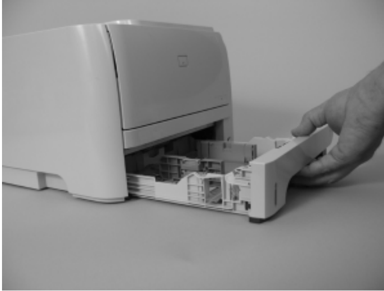
Figure 6-3 Remove the Tray 2 cassette
