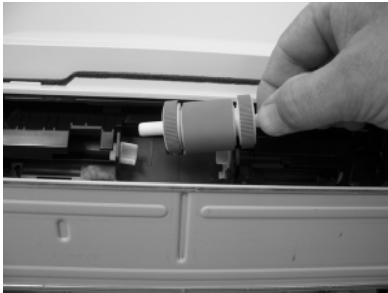
Figure 6-13 Remove the pickup roller; Tray 2 (5 of 5)
