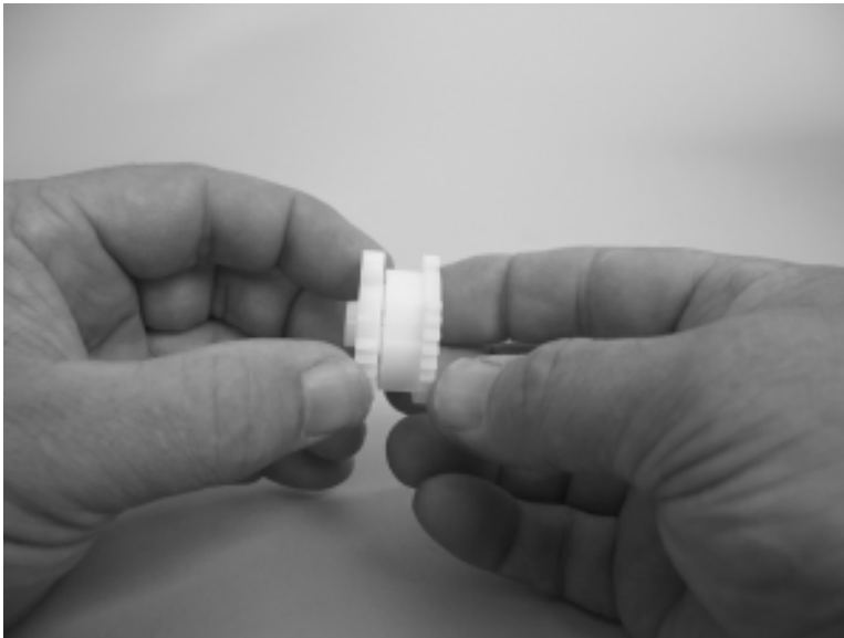
Figure 6-58 Reinstall the paper-pickup-gear assembly (3 of 3)
