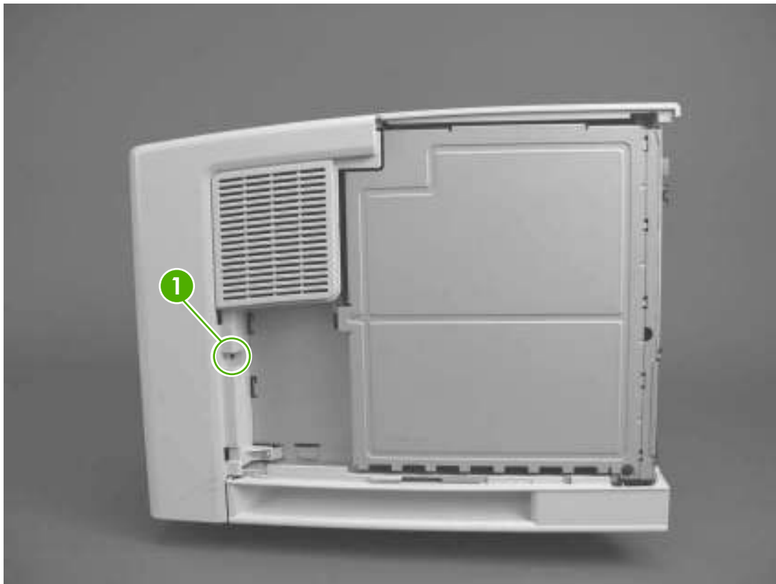
Figure 6-3 Locating the engine-test-page switch
