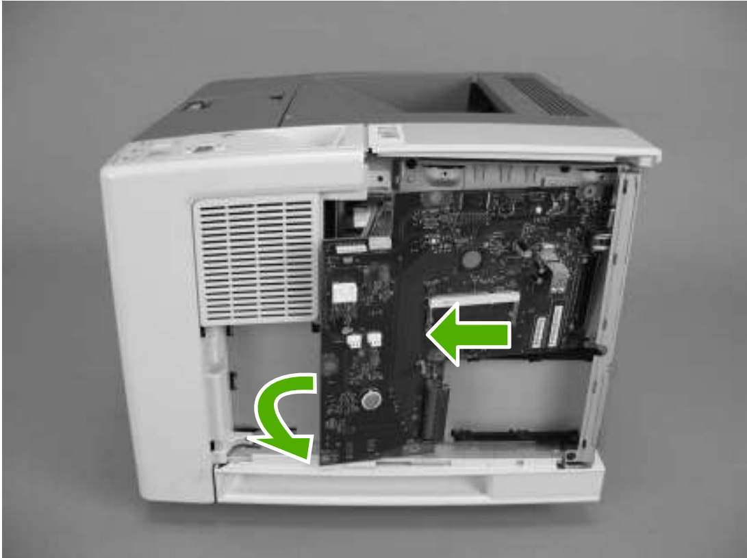
Figure 5-15 Removing the formatter (3 of 3)
