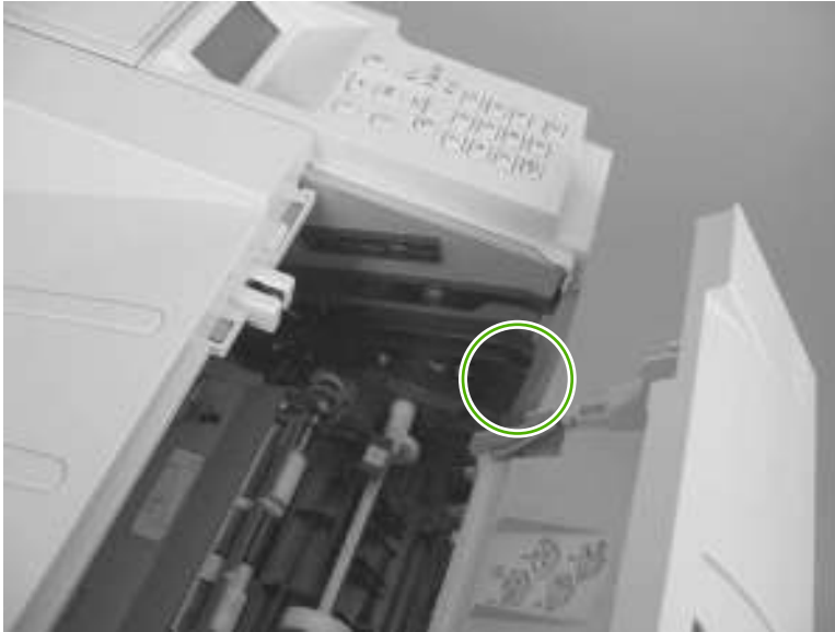
Figure 3-11 Test the cartridge-door open switch
