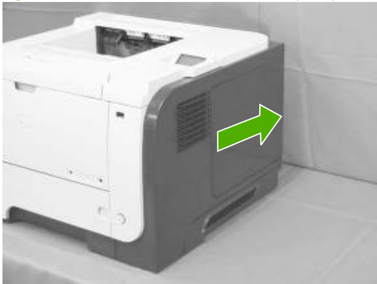
Figure 2-11 Remove the DIMM cover and DIMM (1 of 3)
