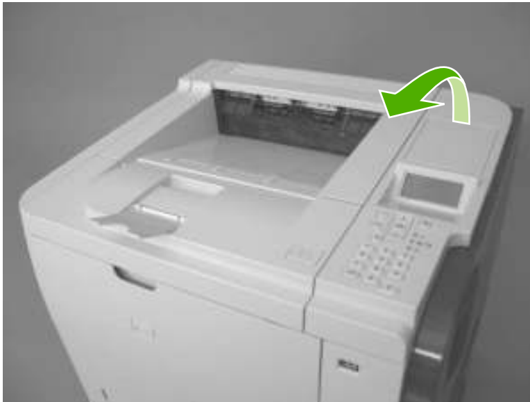
Figure 2-8 Remove the sub cover
