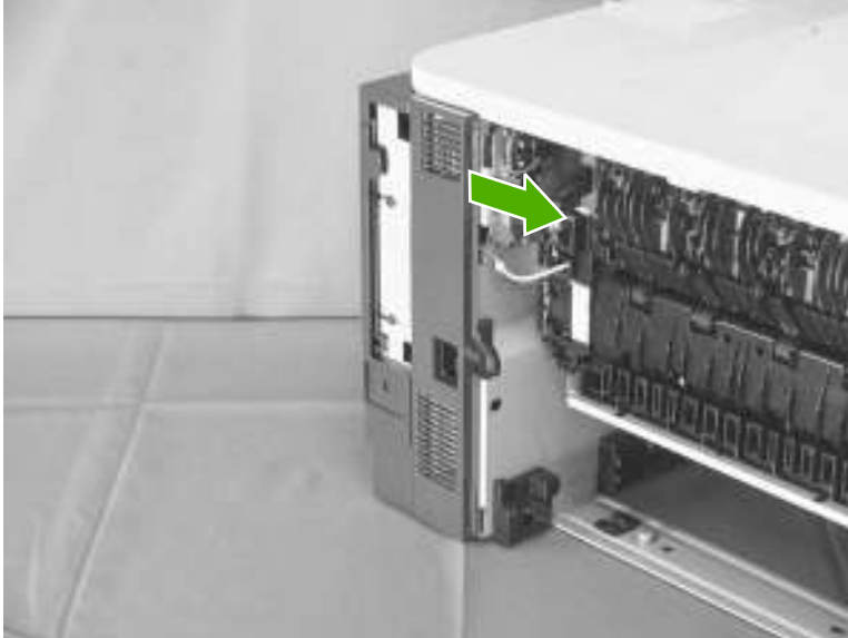
Figure 2-32 Remove the right-rear cover (1 of 2)
