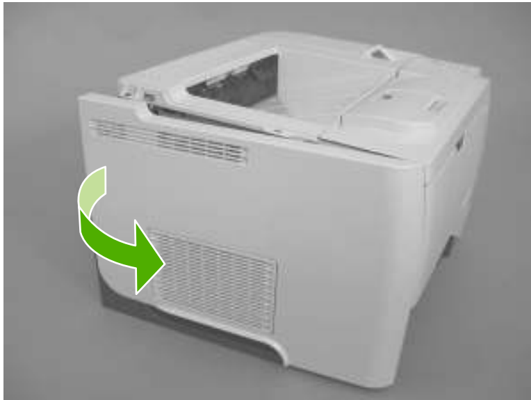
Figure 2-31 Remove the left cover (4 of 4)
