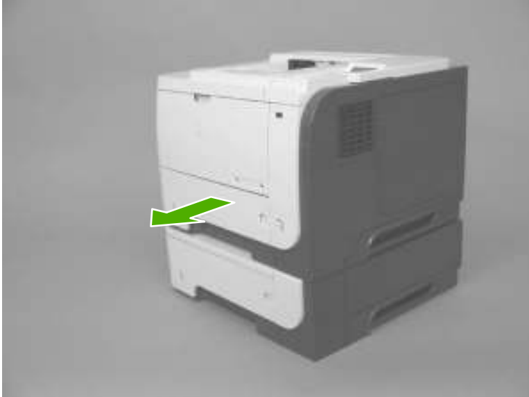
Figure 2-6 Remove the tray cassette (1 of 2)
