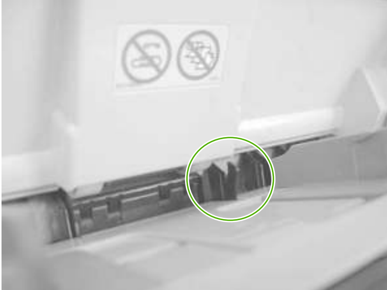
Figure 3-14 Test the Tray 1 (multipurpose tray) media-presence sensor
