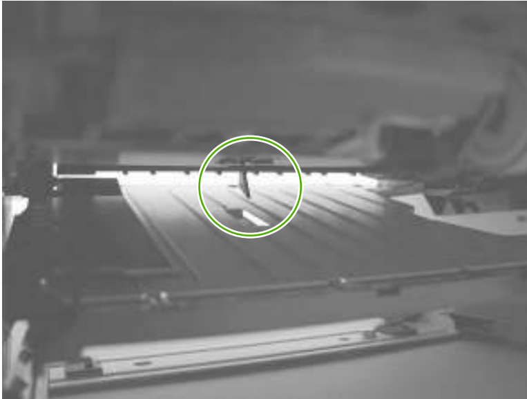
Figure 3-5 Test the duplex media-feed sensor
