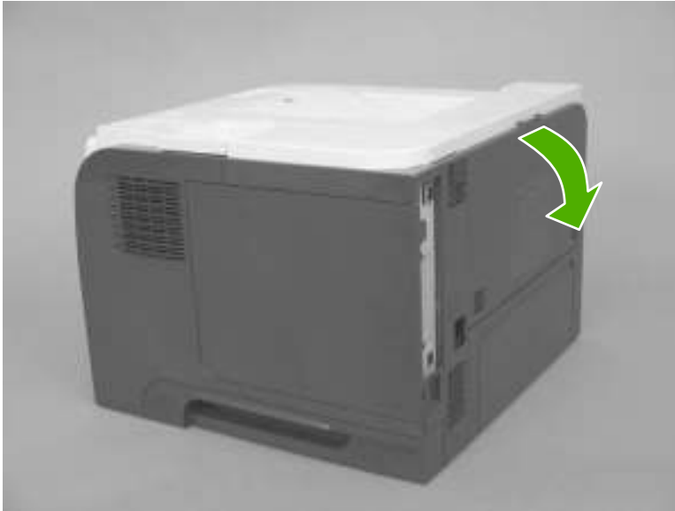
Figure 2-20 Remove the rear-door assembly (1 of 8)
