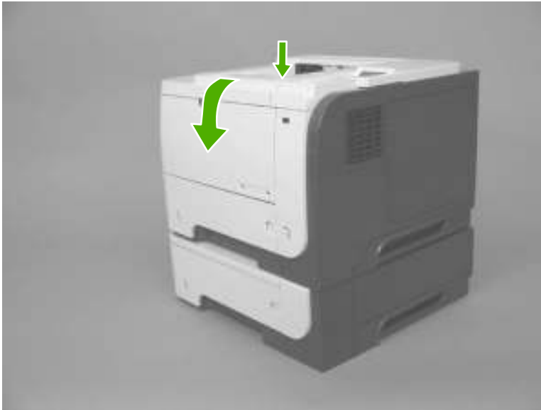
Figure 2-70 Remove the transfer roller (1 of 3)
