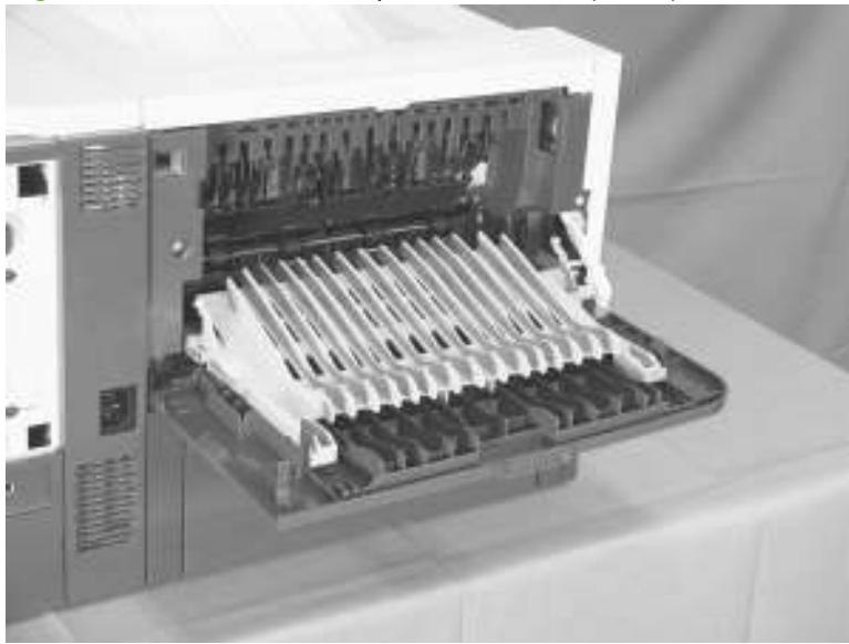
Figure 3-13 Test the face-up detect sensor (2 of 2)
