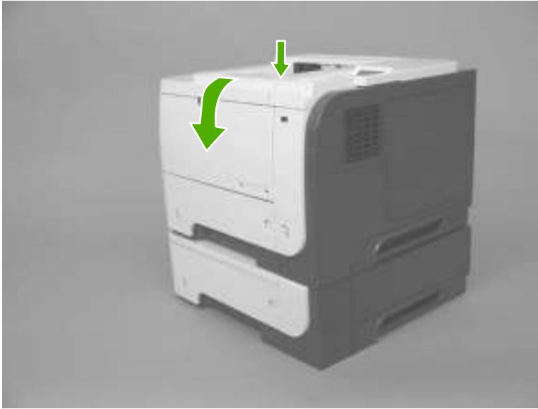
Figure 2-60 Remove the Tray 1 (MP tray) pickup roller (1 of 2)
