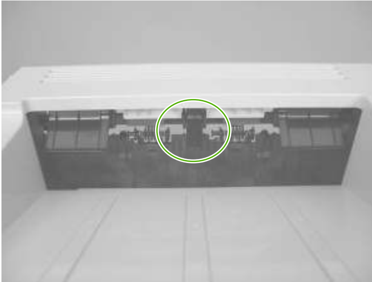
Figure 3-9 Test the face-down media tray media-full sensor
