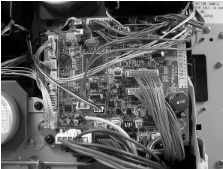
Figure 6-76 Remove the DC controller PCA (1 of 4)
