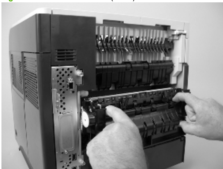
Figure 6-24 Remove the fuser (2 of 2)
