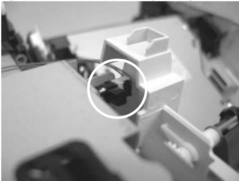
Figure 6-127 Reinstall the paper-delivery assembly
