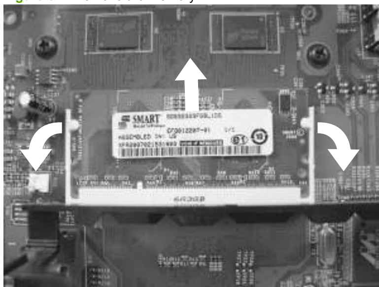
Figure 6-7 Remove the memory DIMM
