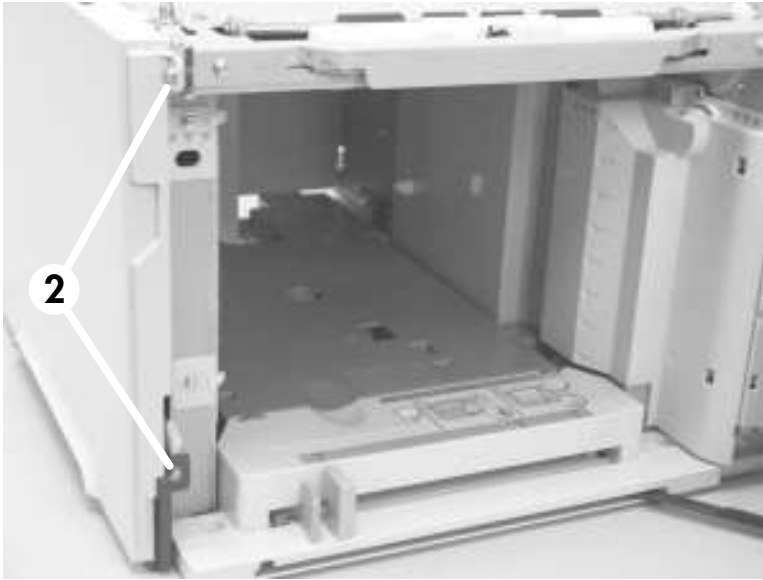
Figure 6-136 Remove the 1,500-sheet feeder left-side cover (3 of 5)
