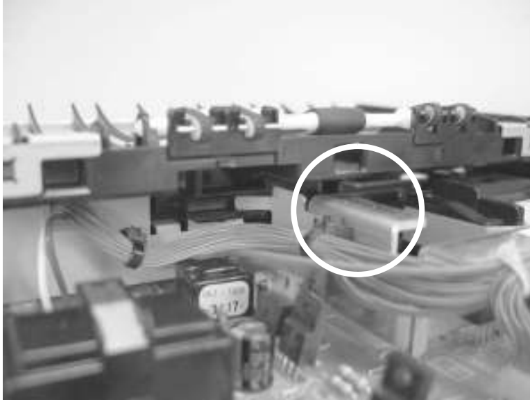
Figure 6-114 Reinstall the feed-guide assembly
