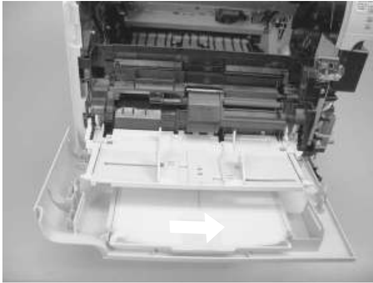
Figure 6-59 Remove the front cover (2 of 2)
