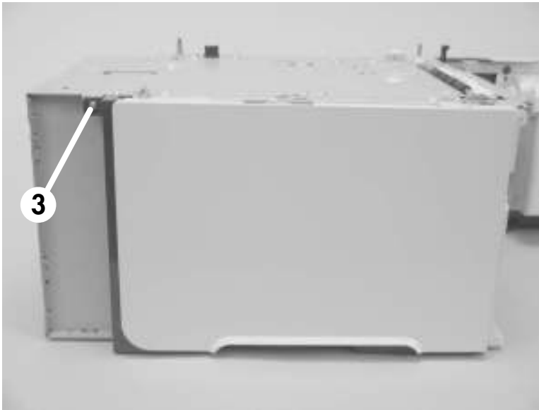
Figure 6-137 Remove the 1,500-sheet feeder left-side cover (4 of 5)
