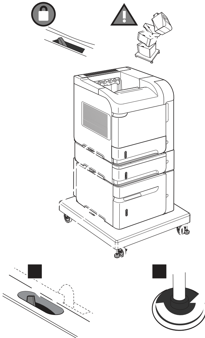
Figure 6-3 Product input trays and cabinet wheel locks
