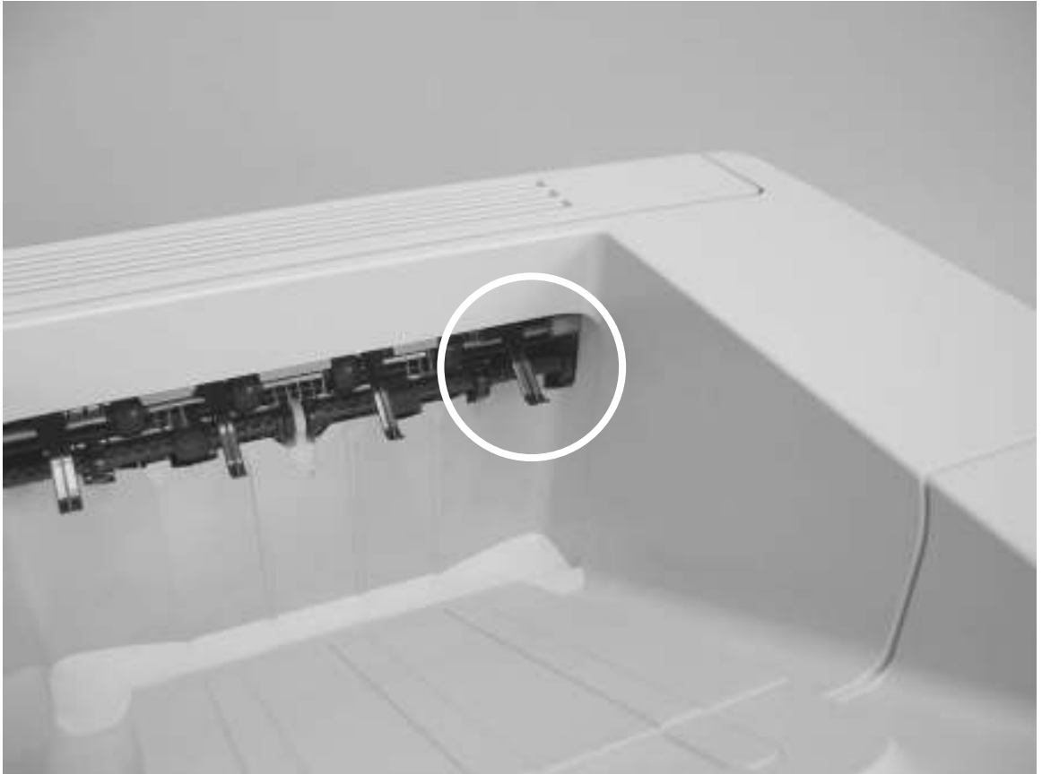
Figure 7-3 Checking the output bin full sensor
