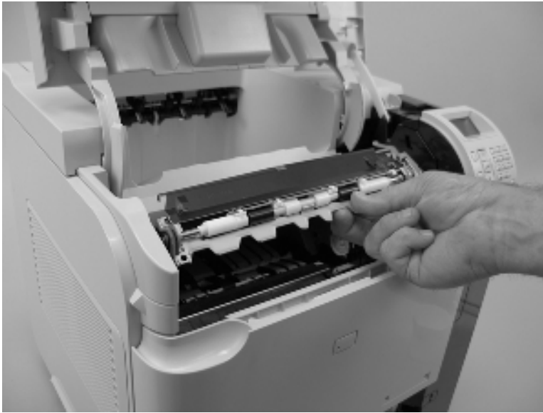
Figure 6-36 Remove the registration assembly (3 of 4)
