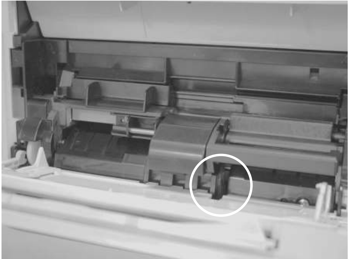
Figure 7-4 Checking the Tray 1 paper present sensor
