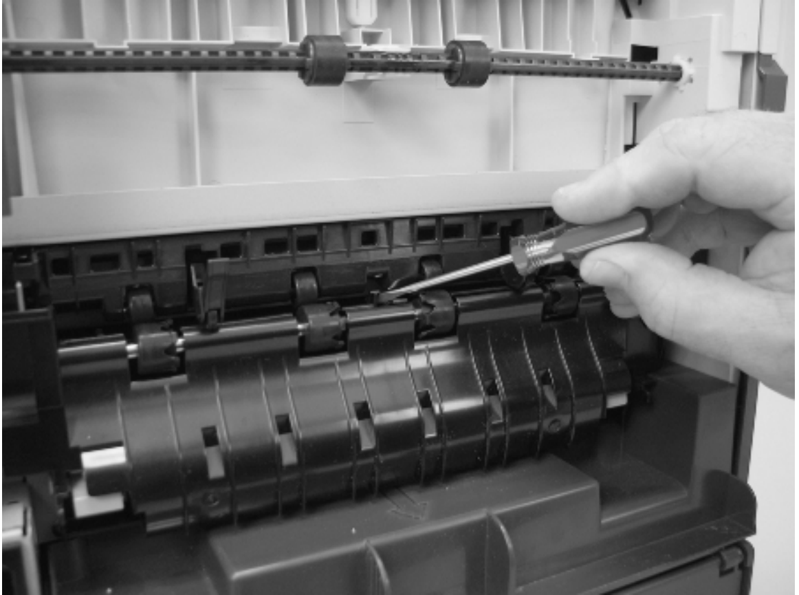
Figure 7-5 Checking the fuser delivery sensor
