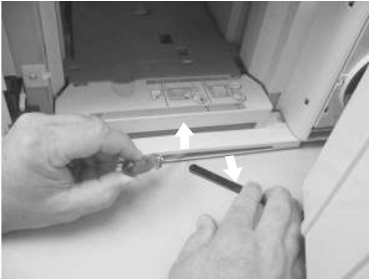
Figure 6-140 Remove the 1,500-sheet feeder door (2 of 3)
