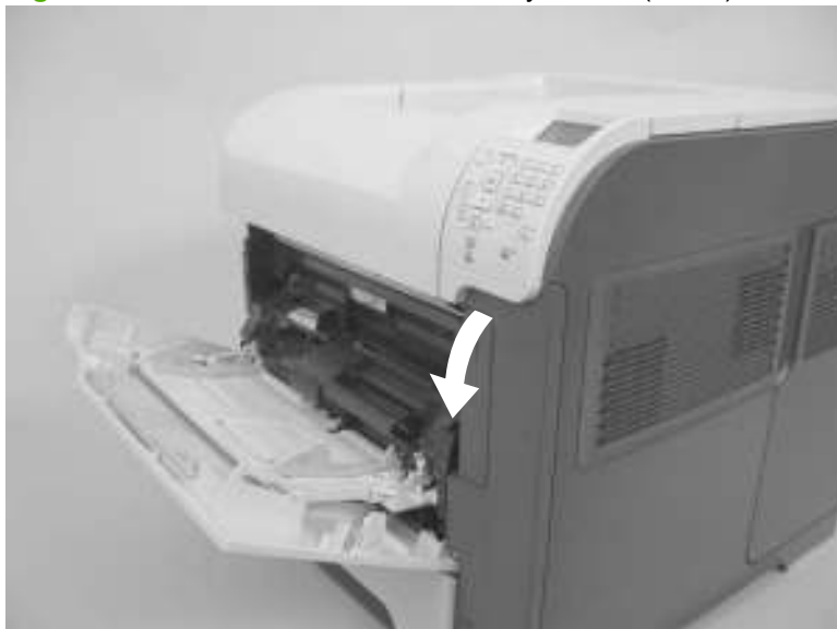
Figure 6-16 Remove the front accessory covers (2 of 2)
