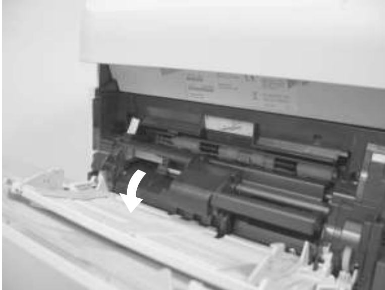
Figure 6-31 Remove the Tray 1 separation roller (1 of 3)
