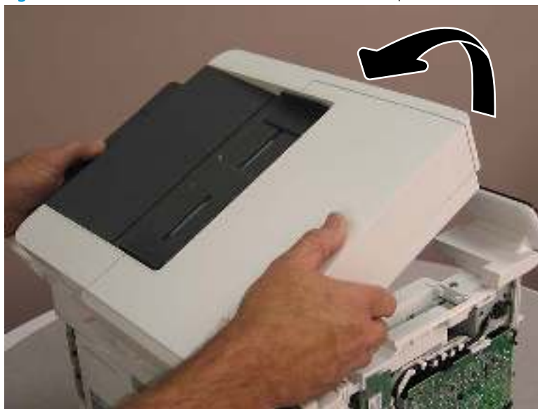
Figure 1-154 Rotate the ISA towards the rear of the printer
