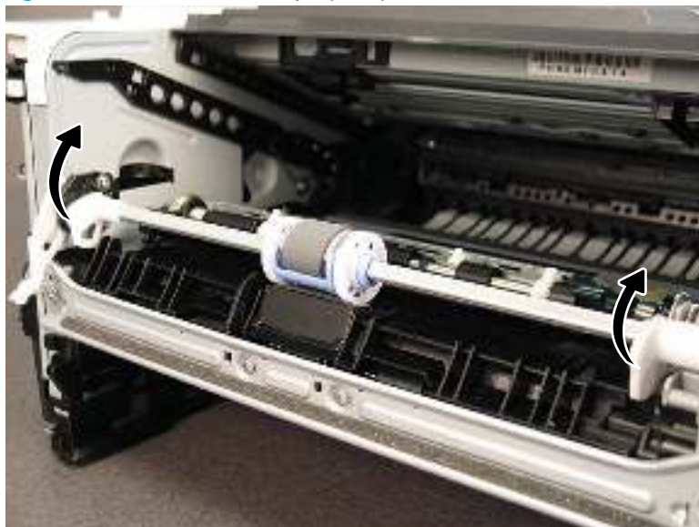
Figure 1-1038 Rotate the Tray 1 pickup roller shaft
