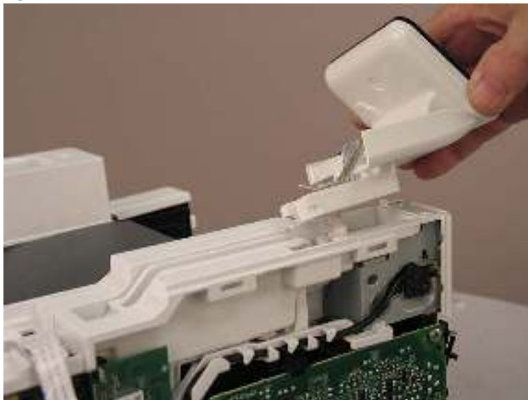
Figure 1-993 Lift up the control-panel assembly
