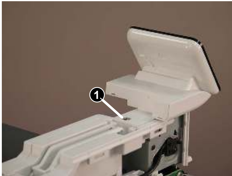
Figure 1-988 Remove one screw
