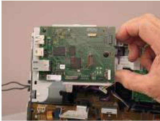
Figure 1-795 Remove the bracket
