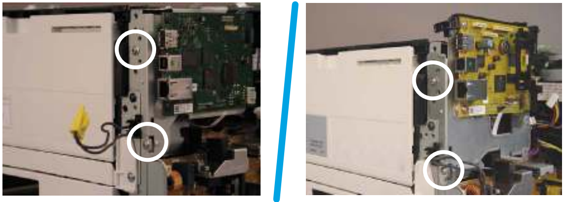
Figure 1-952 Remove two screws
