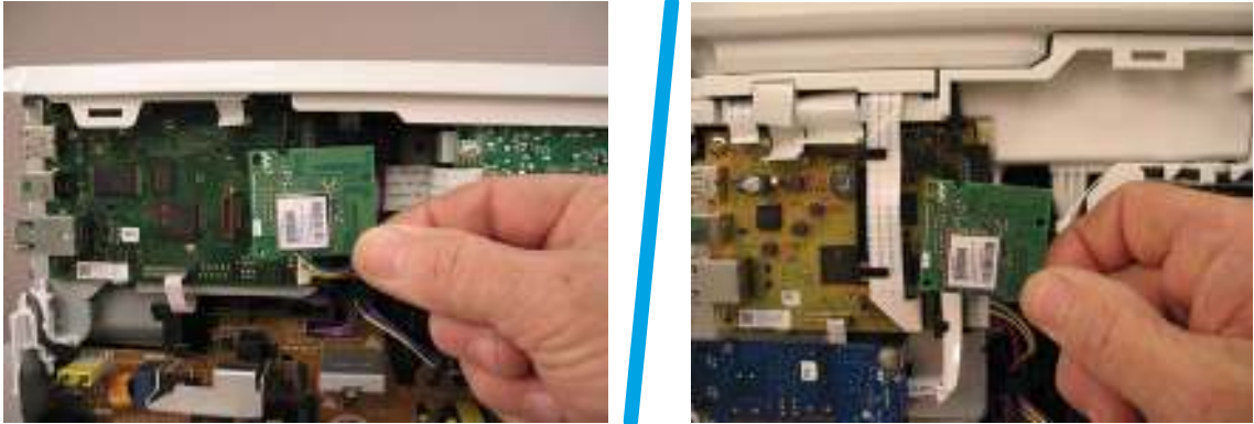
Figure 1-456 Remove the wireless PCA
