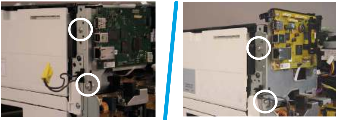
Figure 1-640 Remove two screws
