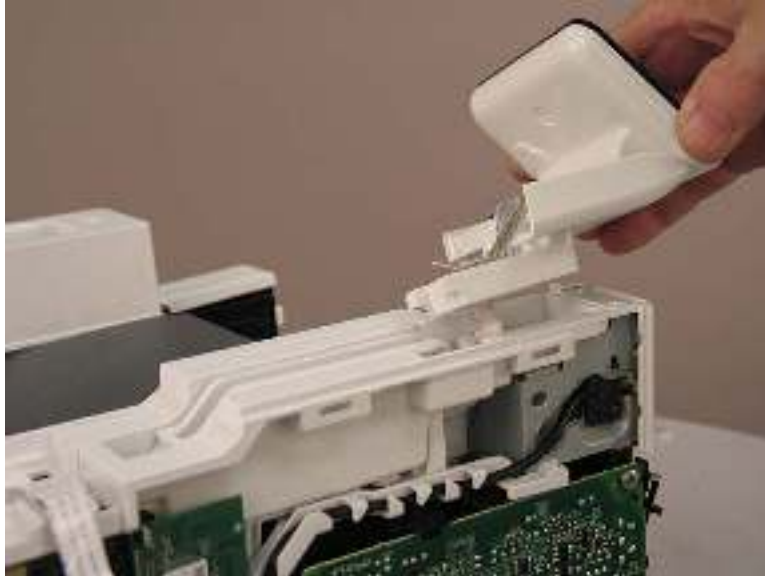
Figure 1-561 Lift up the control-panel assembly
