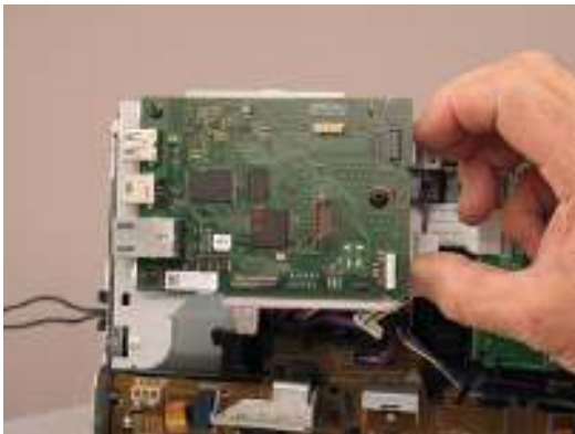
Figure 1-955 Remove the bracket
