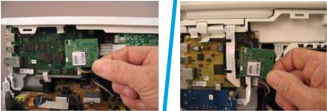
Figure 1-443 Remove the wireless PCA
