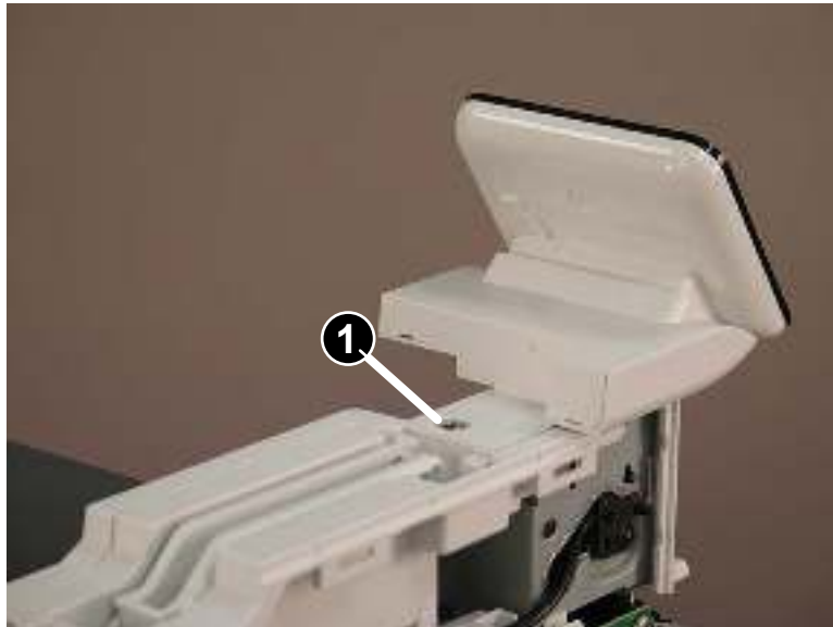
Figure 1-516 Remove one screw
