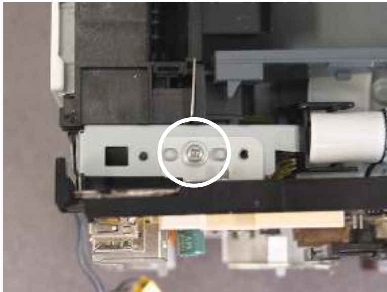
Figure 1-843 Remove one screw
