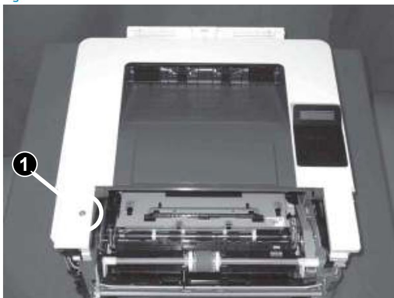
Figure 1-888 Remove one screw
