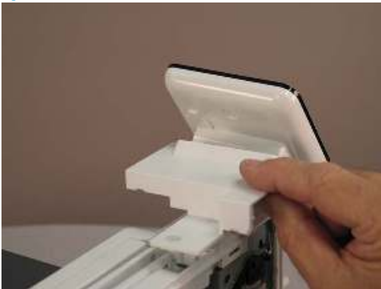
Figure 1-518 Remove the cover
