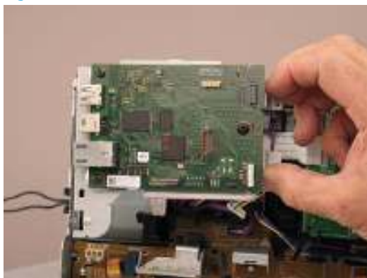
Figure 1-643 Remove the bracket
