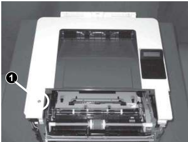
Figure 1-682 Remove one screw
