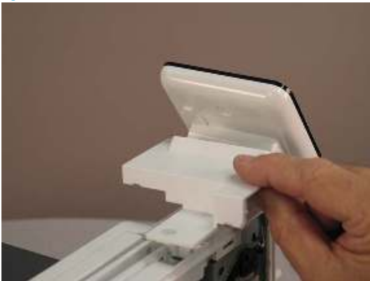
Figure 1-160 Remove the cover
