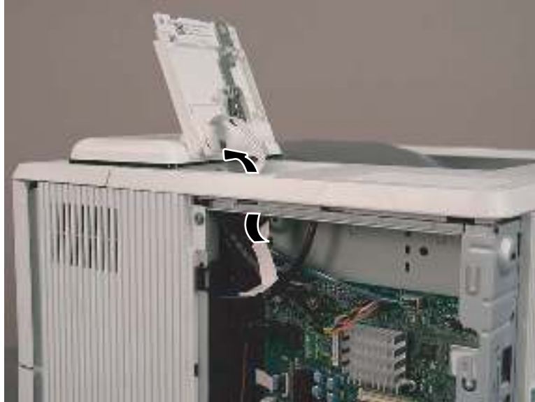
Figure 1-807 Remove the control panel (M507/E50145)
