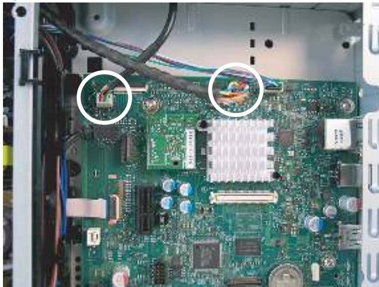
Figure 1-319 Disconnect two connectors
