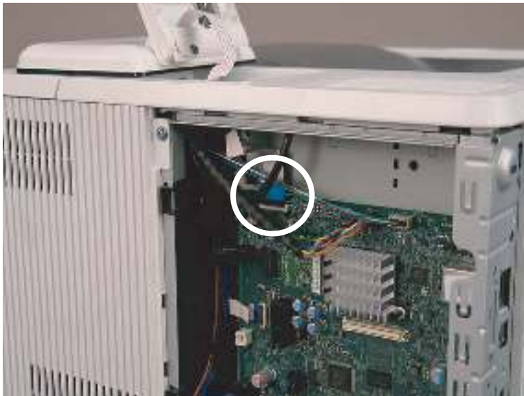
Figure 1-806 Disconnect one FFC (M507/E50145)
