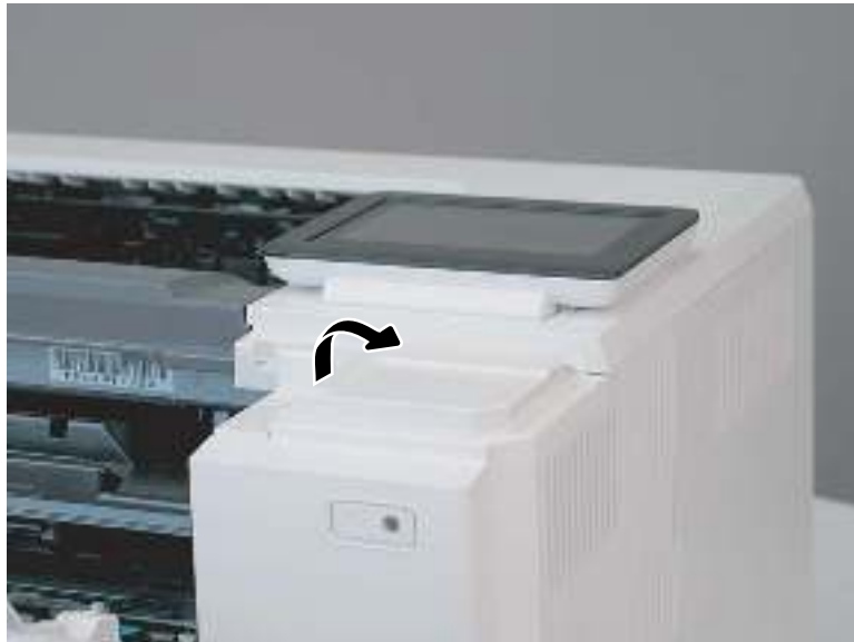
Figure 1-495 Remove the cover
