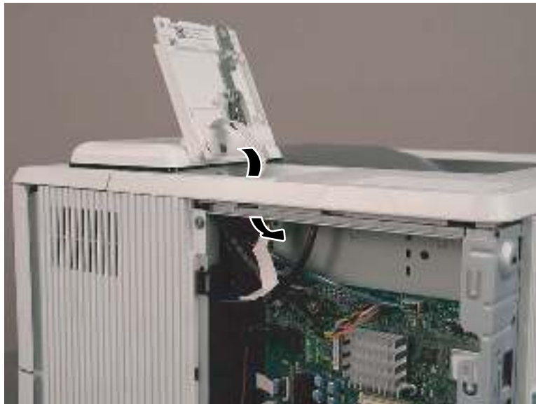
Figure 1-81 Install the FFC (M507/E50145)
