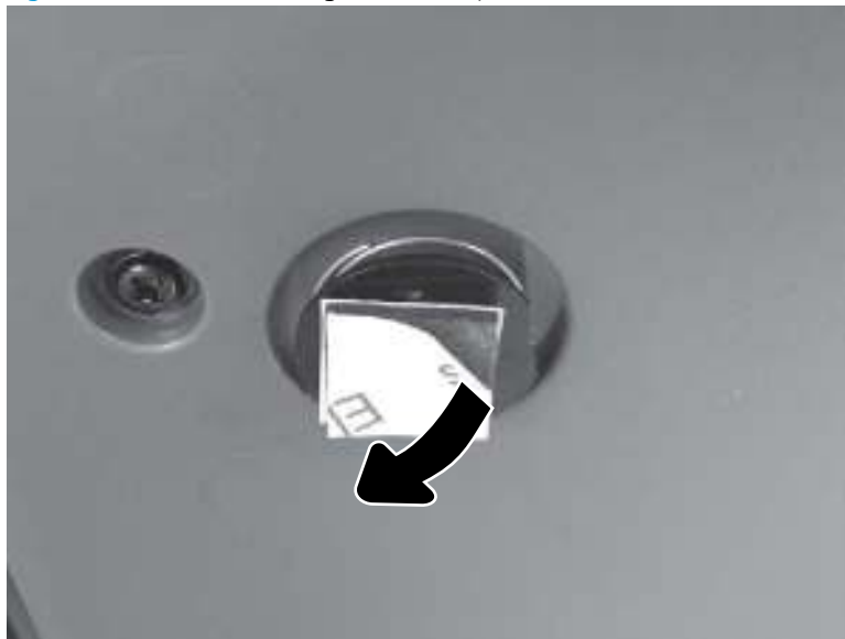
Figure 1-153 White backing adhesive squares
