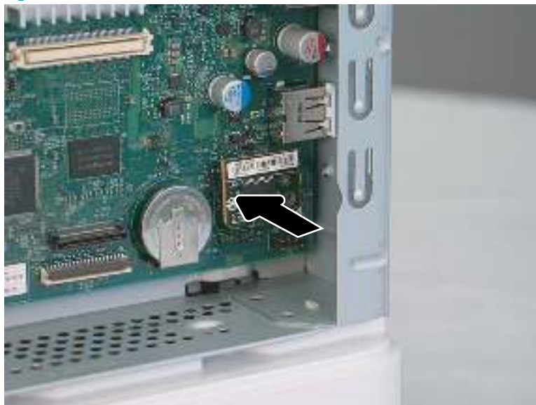
Figure 1-1172 Install the TPM (M507/E50145)
