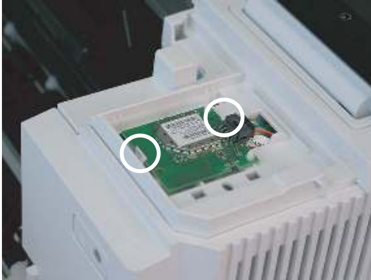
Figure 1-496 Release the PCA
