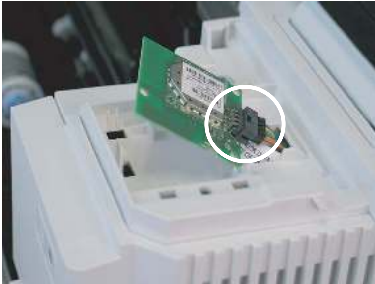
Figure 1-497 Remove the WiFi PCA
