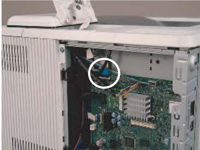
Figure 1-287 Disconnect one FFC (M507/E50145)
