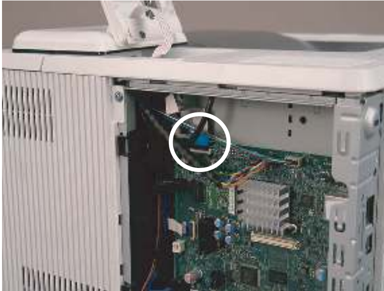
Figure 1-540 Disconnect one FFC (M507/E50145)
