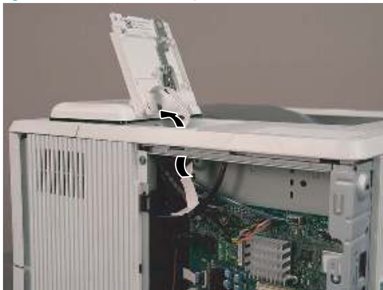
Figure 1-1003 Remove the control panel (M507/E50145)
