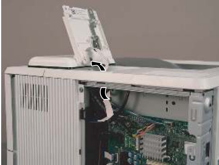
Figure 1-79 Remove the control panel (M507/E50145)
