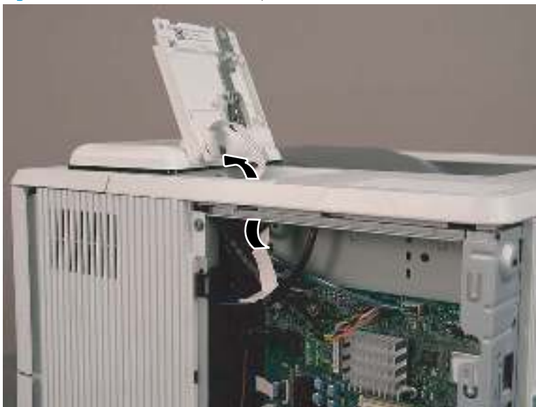
Figure 1-541 Remove the control panel (M507/E50145)
