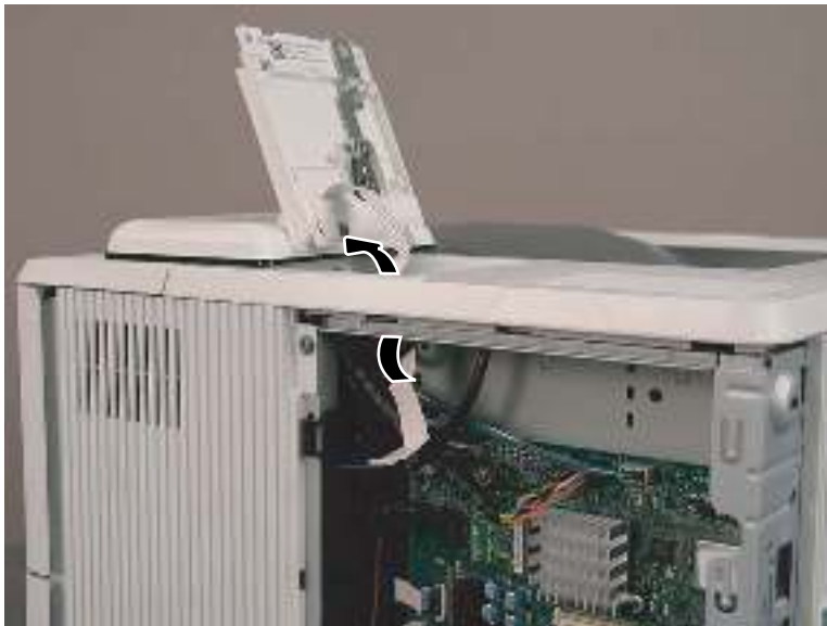
Figure 1-895 Remove the control panel (M507/E50145)
