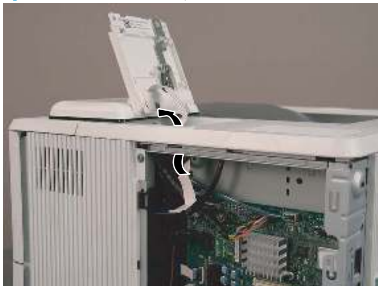
Figure 1-720 Remove the control panel (M507/E50145)
