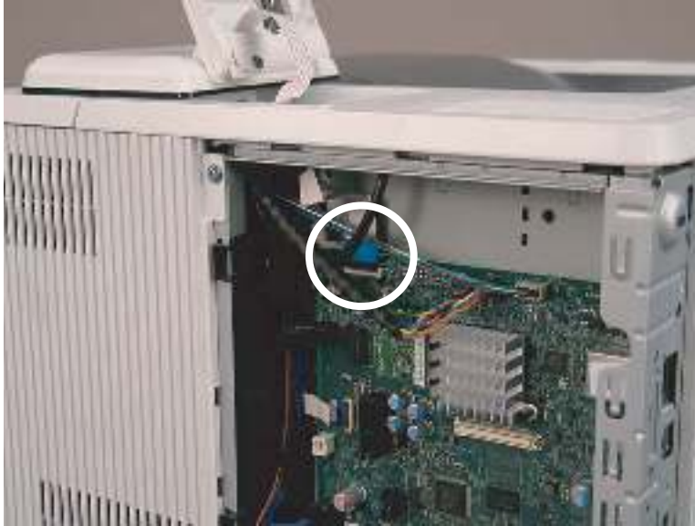
Figure 1-82 Connect one FFC (M507/E50145)
