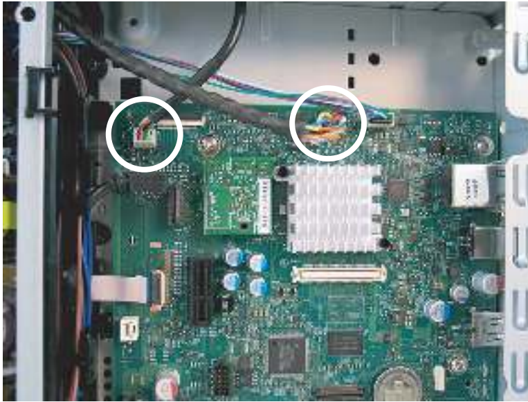
Figure 1-783 Disconnect two connectors
