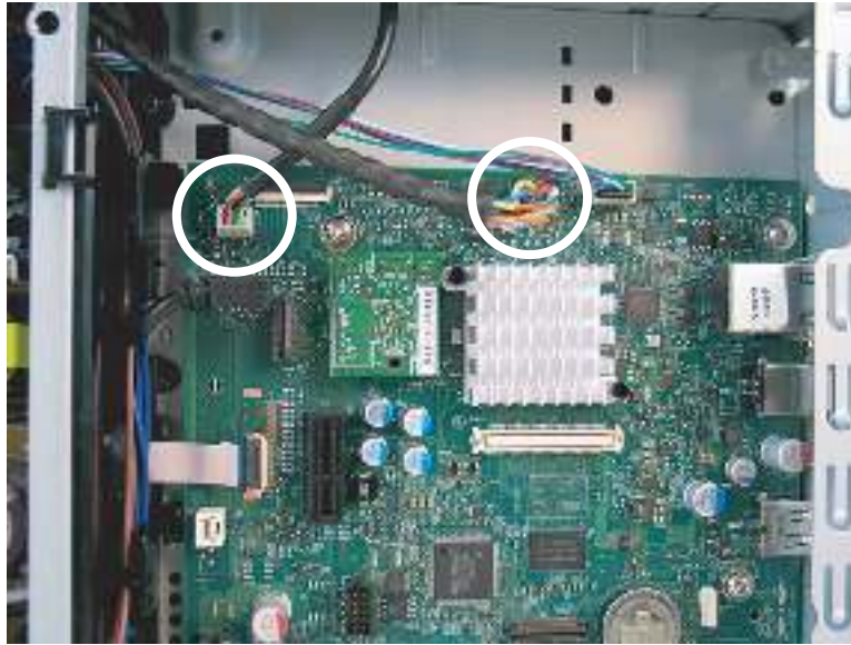
Figure 1-870 Disconnect two connectors
