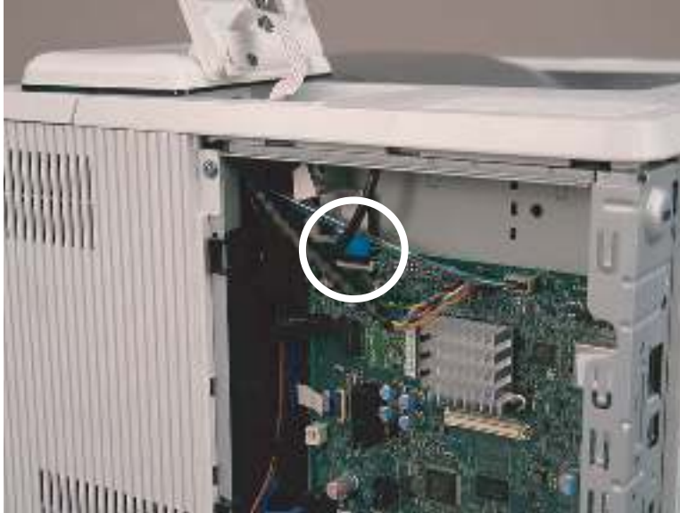
Figure 1-894 Disconnect one FFC (M507/E50145)
