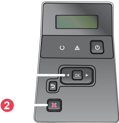
Figure 2-1 Control panel 2ndary Service test access buttons
