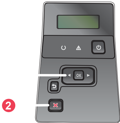
Figure 2-20 Control panel 2ndary Service test access buttons
