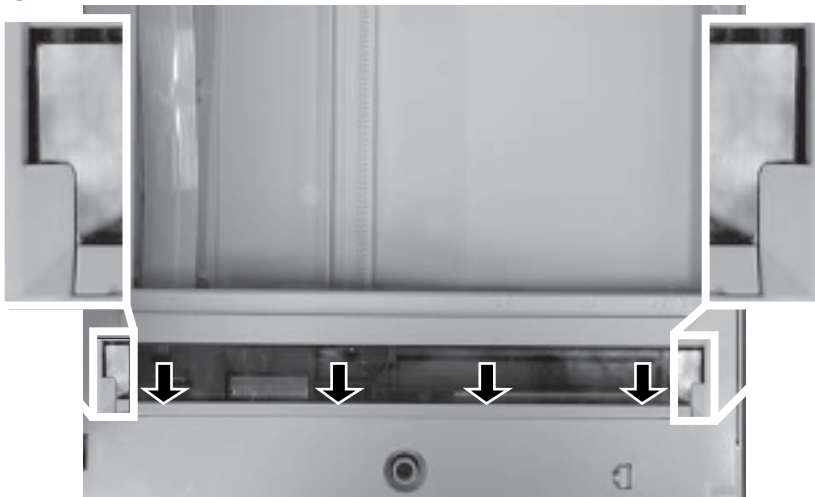
Figure 1-27 Engage the tabs
