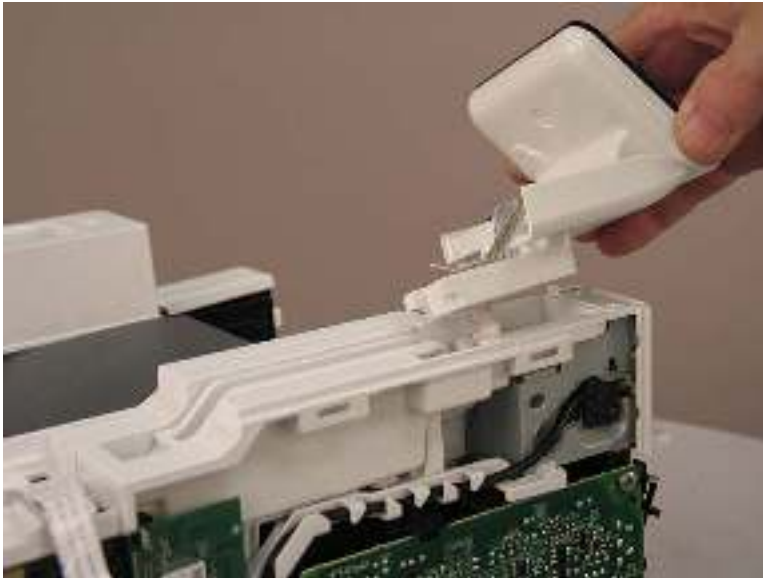
Figure 1-269 Lift up the control-panel assembly
