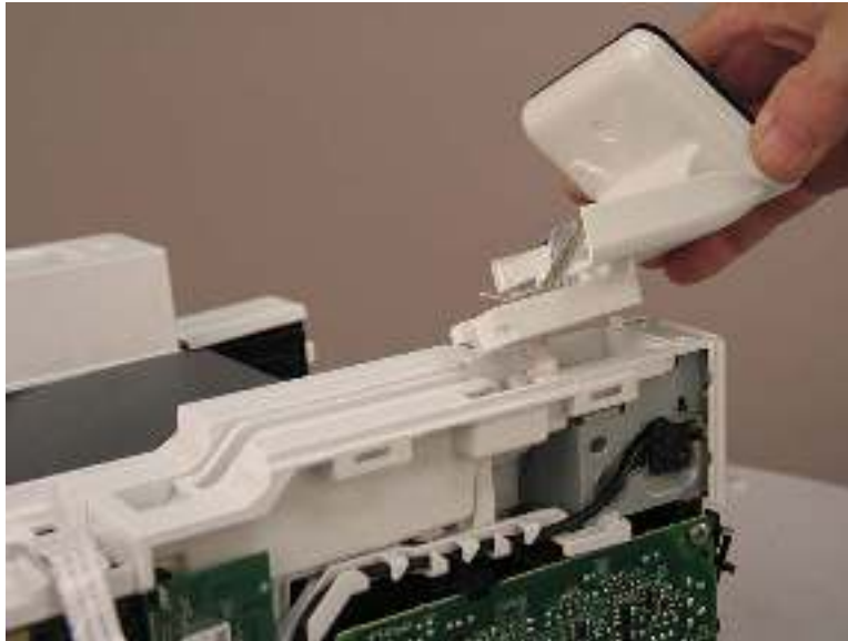
Figure 1-561 Lift up the control-panel assembly
