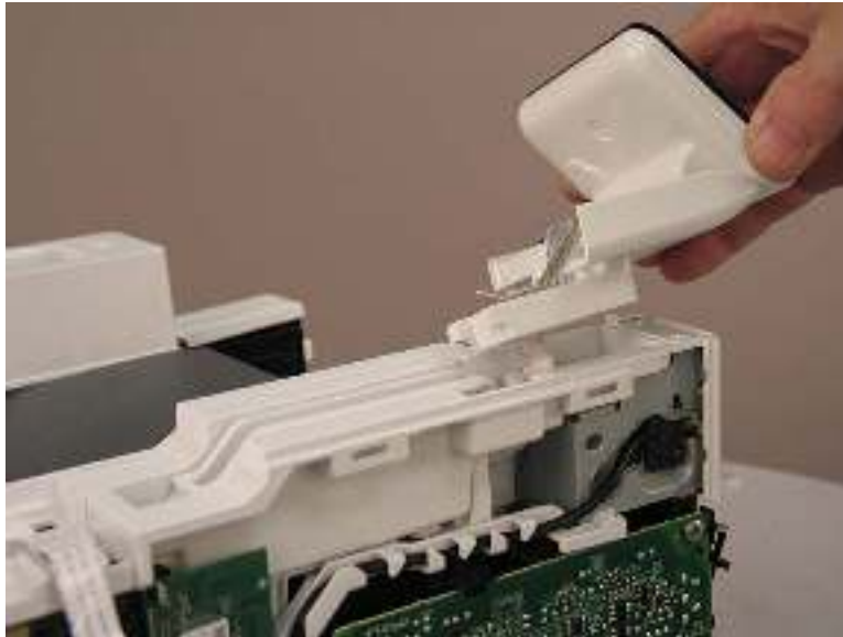
Figure 1-357 Lift up the control-panel assembly
