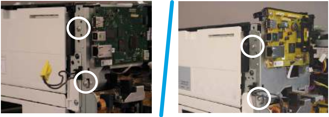
Figure 1-691 Remove two screws
