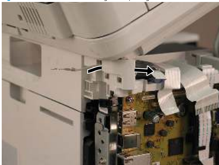
Figure 1-293 Pass the wire through the opening
