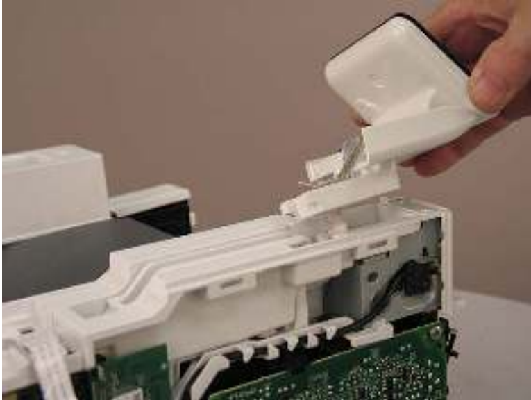
Figure 1-163 Lift up the control-panel assembly
