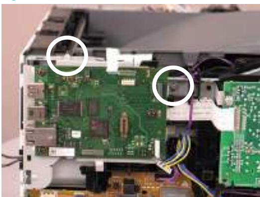
Figure 1-794 Remove two screws
