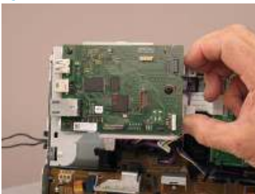
Figure 1-955 Remove the bracket
