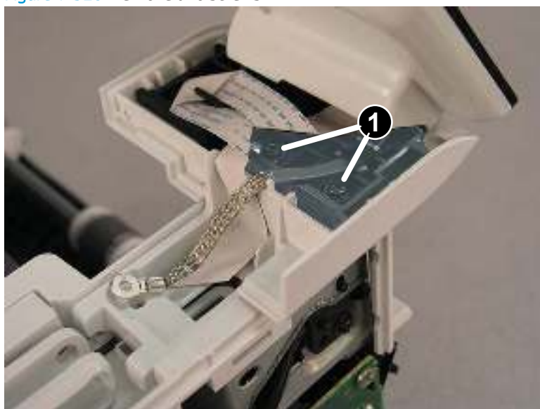
Figure 1-520 Remove two screws
