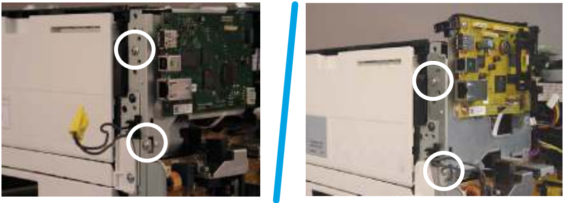
Figure 1-640 Remove two screws
