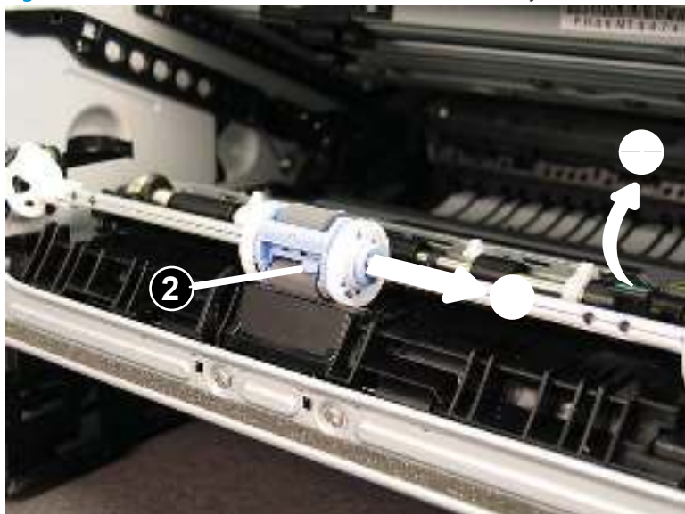
Figure 1-1039 Slide the roller and holder out of the way
