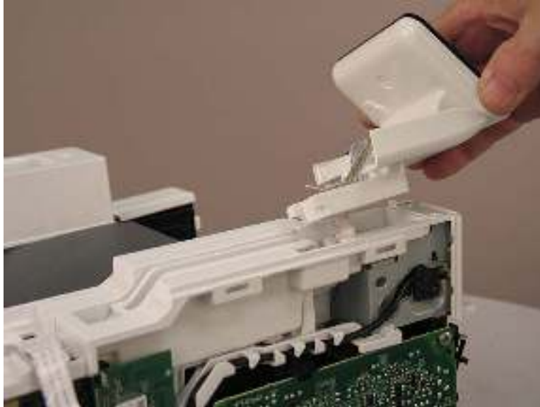
Figure 1-778 Lift up the control-panel assembly
