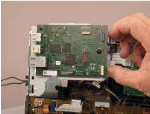
Figure 1-845 Remove the bracket
