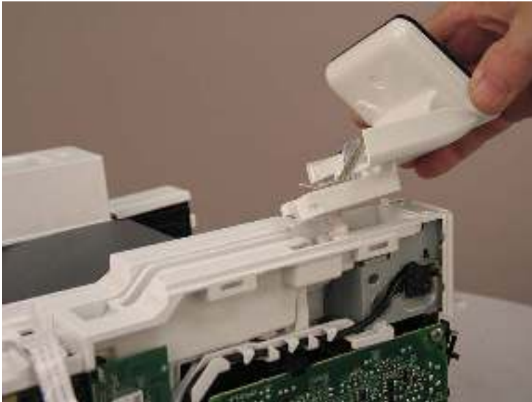
Figure 1-187 Lift up the control-panel assembly
