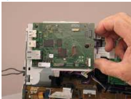
Figure 1-643 Remove the bracket
