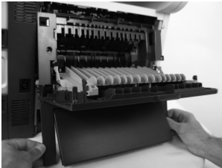
Figure 1-31 Remove the rear cover assembly (8 of 8)
