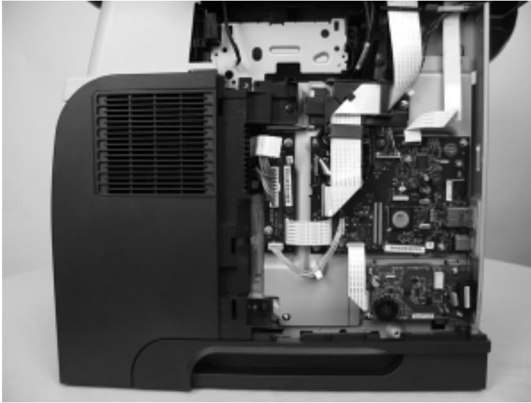
Figure 1-59 Remove the document feeder/scanner assembly (1 of 7)
