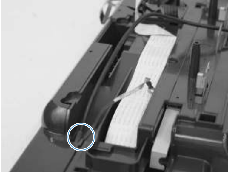
Figure 1-95 Remove the USB cable and USB grounding cable (5 of 5)
