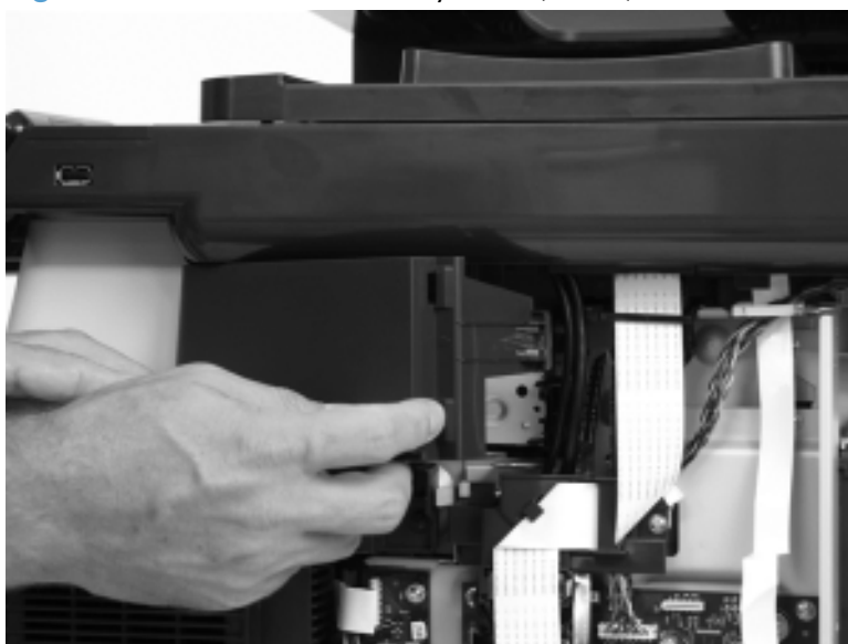
Figure 1-23 Remove the dummy cover (2 of 2)
