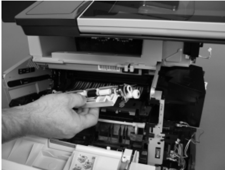
Figure 1-127 Removing the registration roller assembly (3 of 3)
