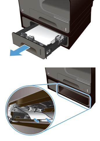
3. If the jam cannot be cleared at the tray, try clearing the jam from the Tray 3 left door.
