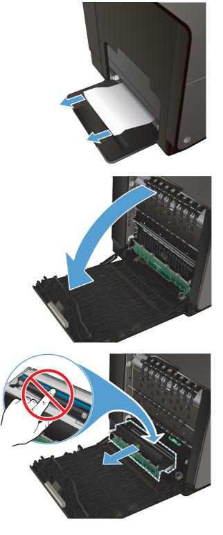
4. Lower the platen by pressing down on the green tab. This will cause the product to try to feed the sheet through the print zone. You might need to gently pull on the sheet if it does not feed. Remove the sheet.
