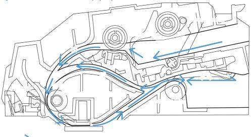
Figure 1-15 Document feeder paper path and sensors
