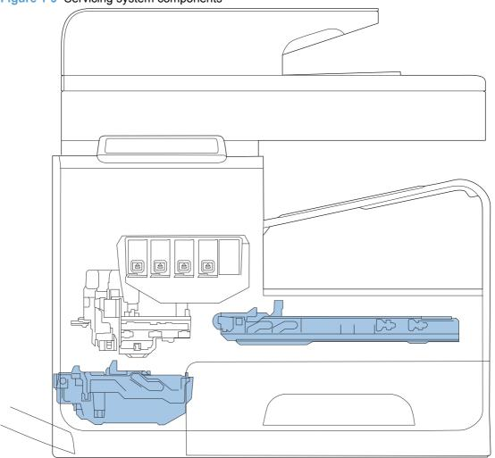
Figure 1-9 Servicing system components
