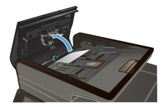
3. Lift the document feeder roller assembly, and gently pull the jammed paper out.
