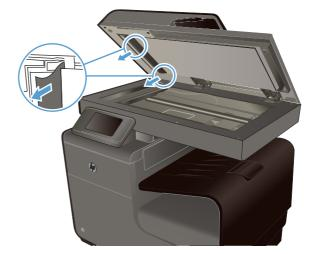
5. Open the scanner lid. If paper is jammed behind the white plastic backing, gently pull it out.
