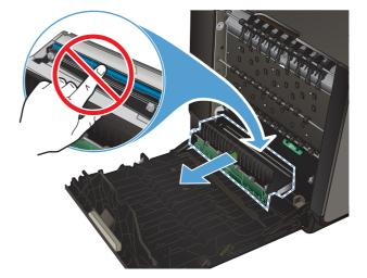
4. Lower the platen by pressing down on the green tab. This will cause the product to try to feed the sheet through the print zone. You might need to gently pull on the sheet if it does not feed. Remove the sheet.
