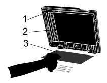
In the ADF unit, clean the white bar (1) and the glass strip (2) underneath it with a soft lint-free cloth moistened with water.
