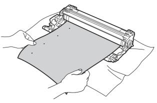
Turn the drum unit gear by hand while looking at the surface of the OPC drum (1).
