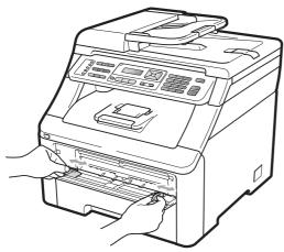
Using both hands, put one blank sheet of paper in the manual feed slot until the front edge of the paper touches the paper feed roller. Wait until the machine automatically feeds the paper. When you feel the machine pull in the paper, let go.
