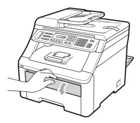
Using both hands, slide the manual feed slot paper guides to the width of the paper that you are going to use.
