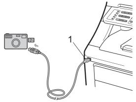
Turn on the camera. Make sure your camera is in PictBridge mode. When the machine has recognized the camera, the LCD shows the following messages, depending on which mode the machine is in:
