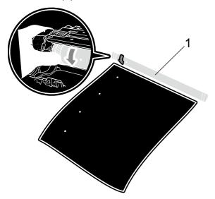
When you have found the mark on the drum that matches the print sample, wipe the surface of the OPC drum with a dry cotton swab until the dust or glue on the surface comes off.
