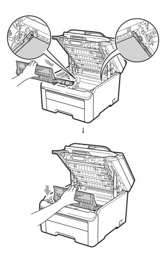
6 Slide each drum unit and toner cartridge assembly into the machine. Make sure that you match the toner cartridge color to the same color label on the machine. Repeat this for all the drum unit and toner cartridge assemblies.
