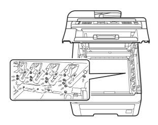
4 Push down the green-labeled lock lever (1) and take the toner cartridge out of the drum unit.
