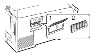
6 Put the metal (2) and then the plastic (1) SO-DIMM covers back on.
