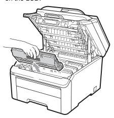
4 Push down the green-labeled lock lever (1) and take the toner cartridge out of the drum unit.
