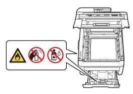
DO NOT attempt to operate this product with a paper jam or with stray pieces of paper inside the product. Prolonged contact of the paper with the drum unit could cause a fire.
