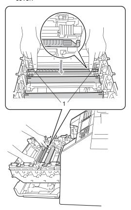
5 Clean the corona wires inside the drum unit by gently sliding the green tabs from left to right and right to left several times.
