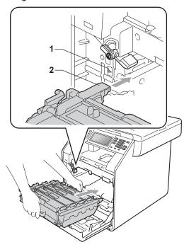
12 Turn the green lock lever (1) clockwise to the lock position.
