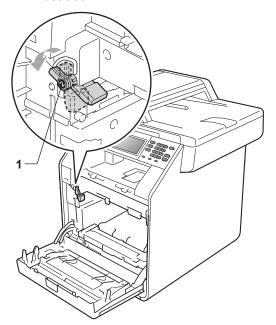
Match the guide ends (2) of the drum unit to the ► marks (1) on both sides of the machine, then gently slide the drum unit into the machine until it stops at the green lock lever.
