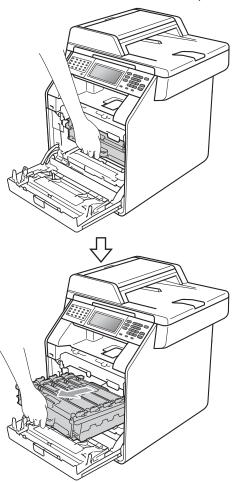
Turn the green lock lever (1) at the left of the machine counterclockwise to the release position. Holding the green handles of the drum unit, lift the front of the drum unit and remove it from the machine.
