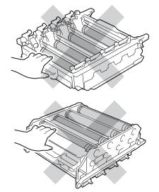
Wait to unpack the new drum unit until immediately before you put it in the machine. Exposure to direct sunlight or room light may damage the drum unit.
