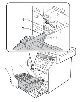
10 Turn the green lock lever (1) clockwise to the lock position.
