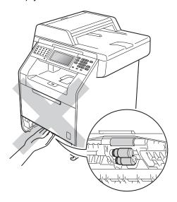
If paper is not caught inside the machine, turn the paper tray over and check underneath the paper tray.
