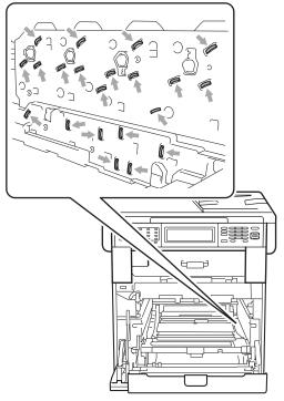
Hold the green handles of the drum unit when you carry it. DO NOT hold the sides of the drum unit.  To avoid print quality problems, DO NOT touch the shaded parts shown in the illustrations.
